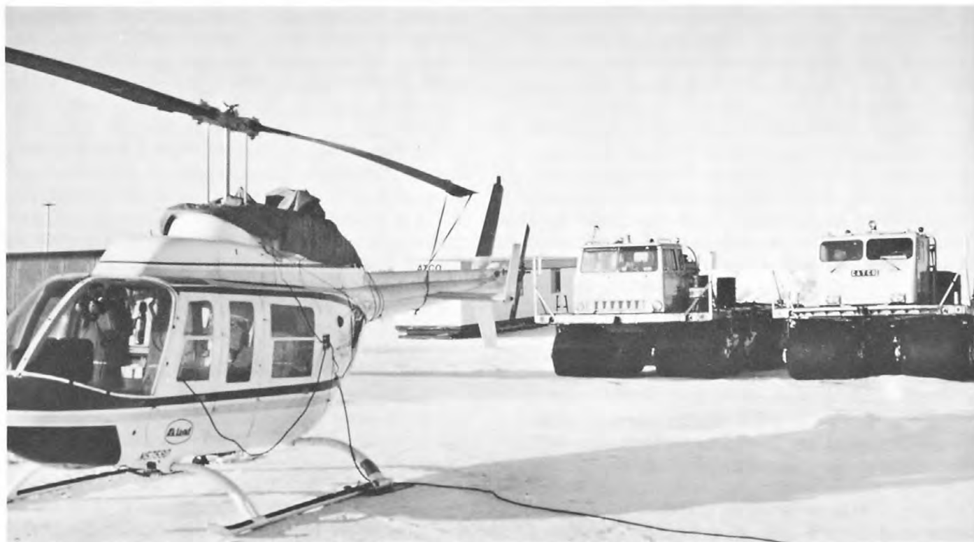
FIGURE 33. --Vehicles used to support Arctic oil and gas operations. Low-pressure tires on ground vehicles are designed for use on permafrost. (Photograph by Fritts Golden, Rogers, Golden & Halpern.)
