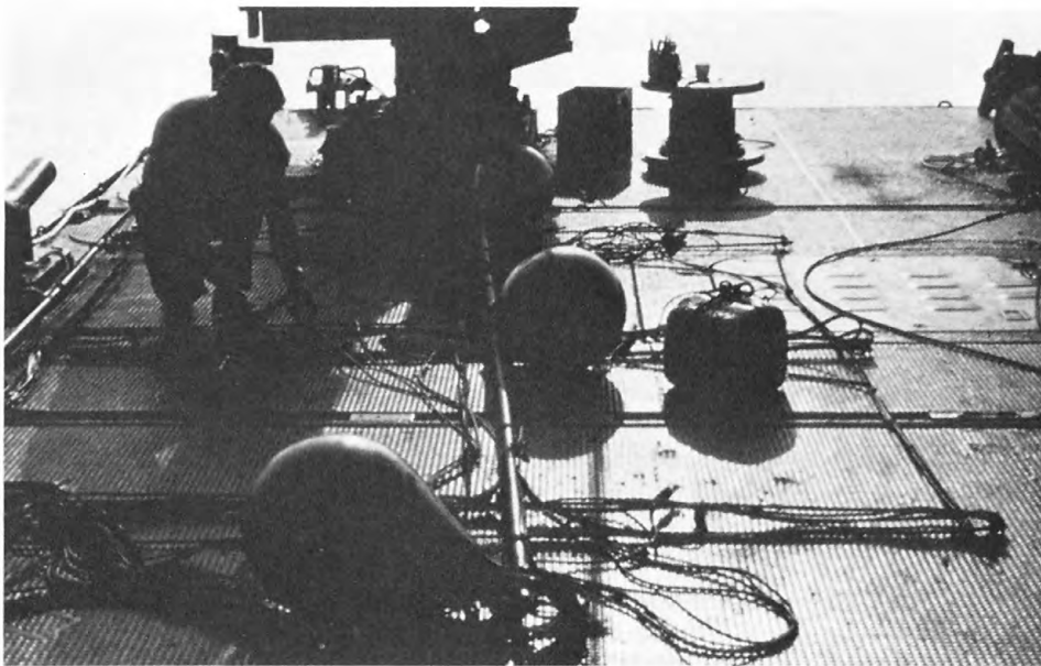
FIGURE 76.—Pressure field measurement array under test on deck of experiment barge
