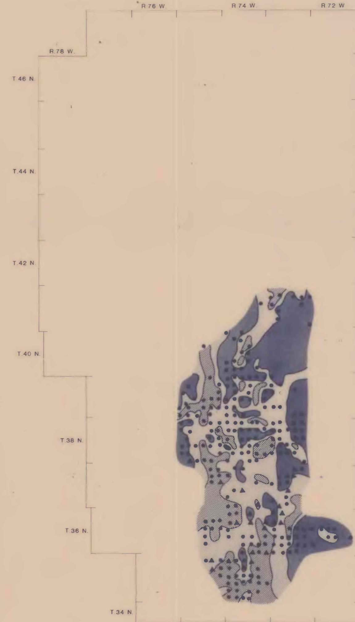
FIGURE 3. FACIES MAP OF ZONE B, 0-93m (0-300ft.) BELOW BASE OF THE SCHOOL HOUSE COAL.
