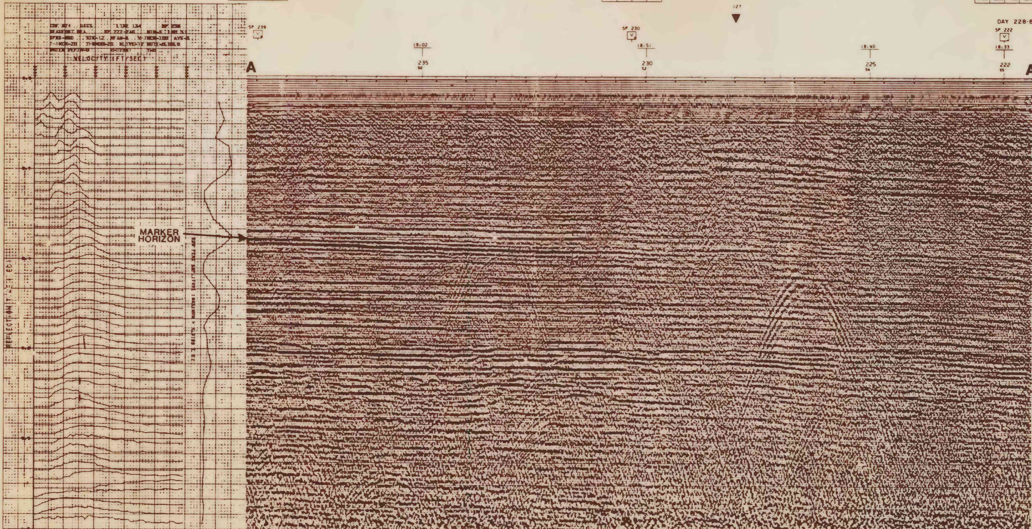
TWELVE-CHANNEL CDP SEISMIC PROFILE WITH VELOCITY ANALYSIS AND RECORDING PARAMETERS.
