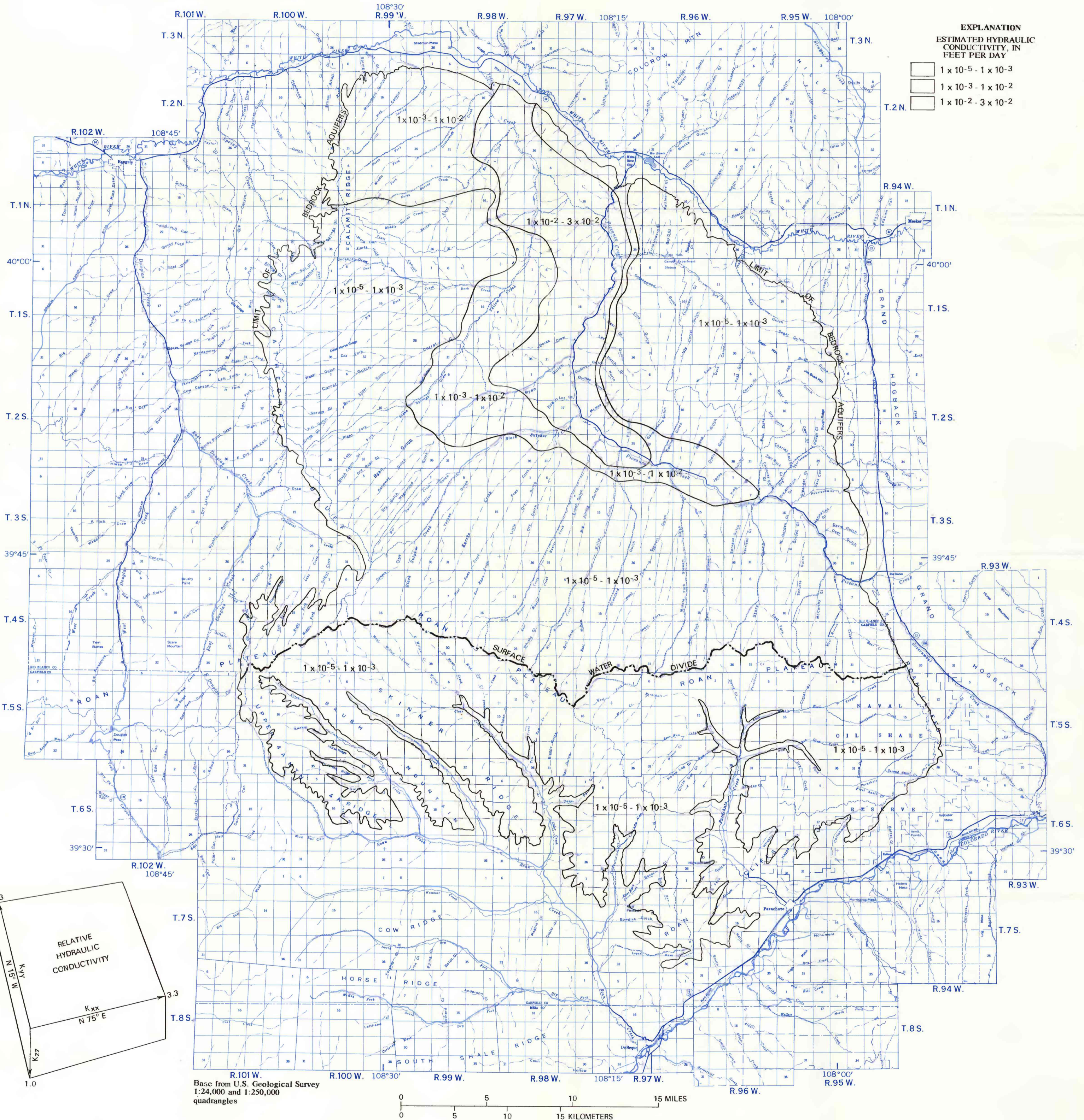
MAP SHOWING ESTIMATED VERTICAL HYDRAULIC CONDUCTIVITY OF LAYER 3, MAHOGANY ZONE OF GREEN RIVER FORMATION
