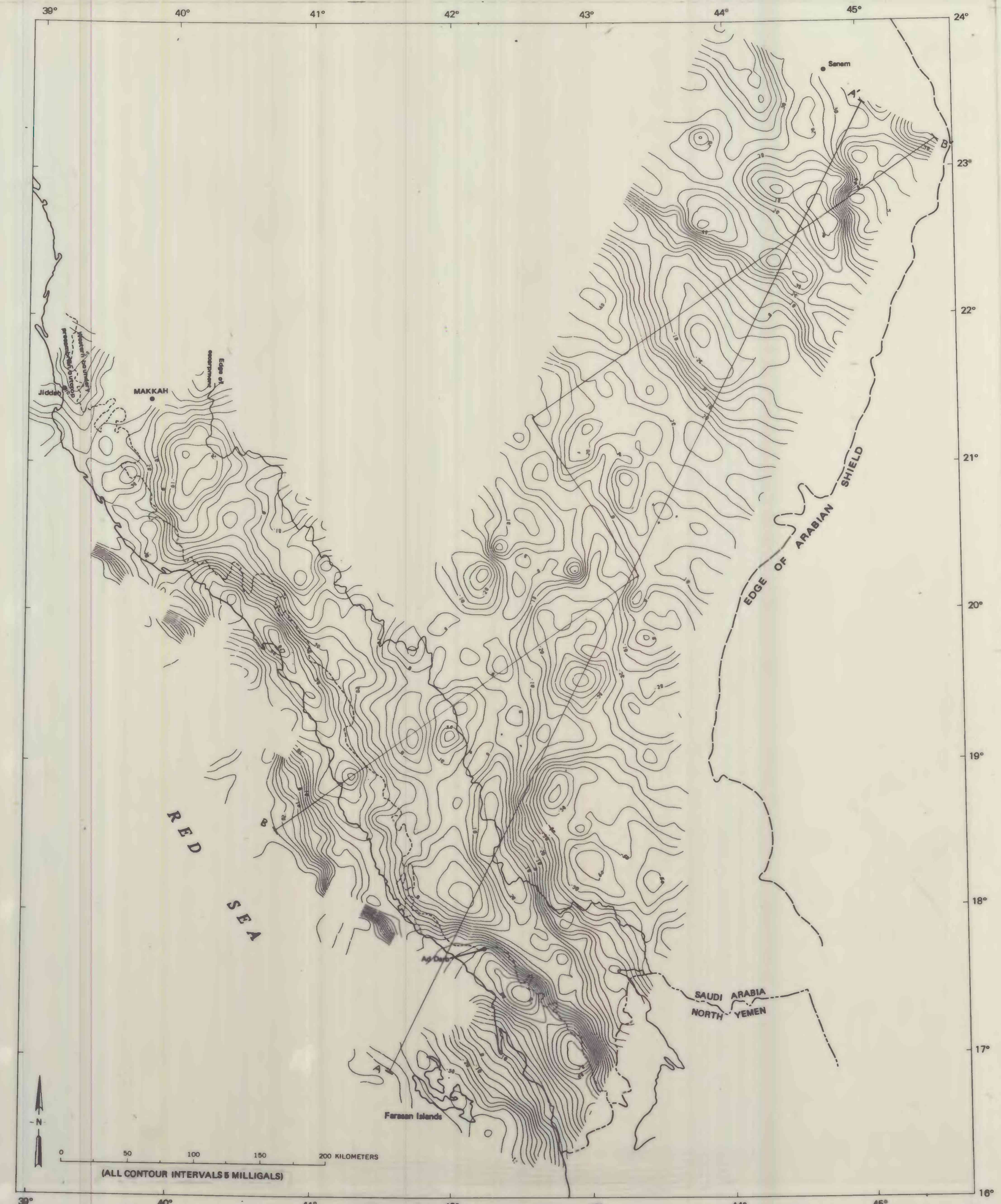
B. Uncorrected isostatic gravity anomaly map. Gravity profiles A-A' and B-B' demonstrating the northeast-trending regional gravity gradient, are shown in figure 12.
