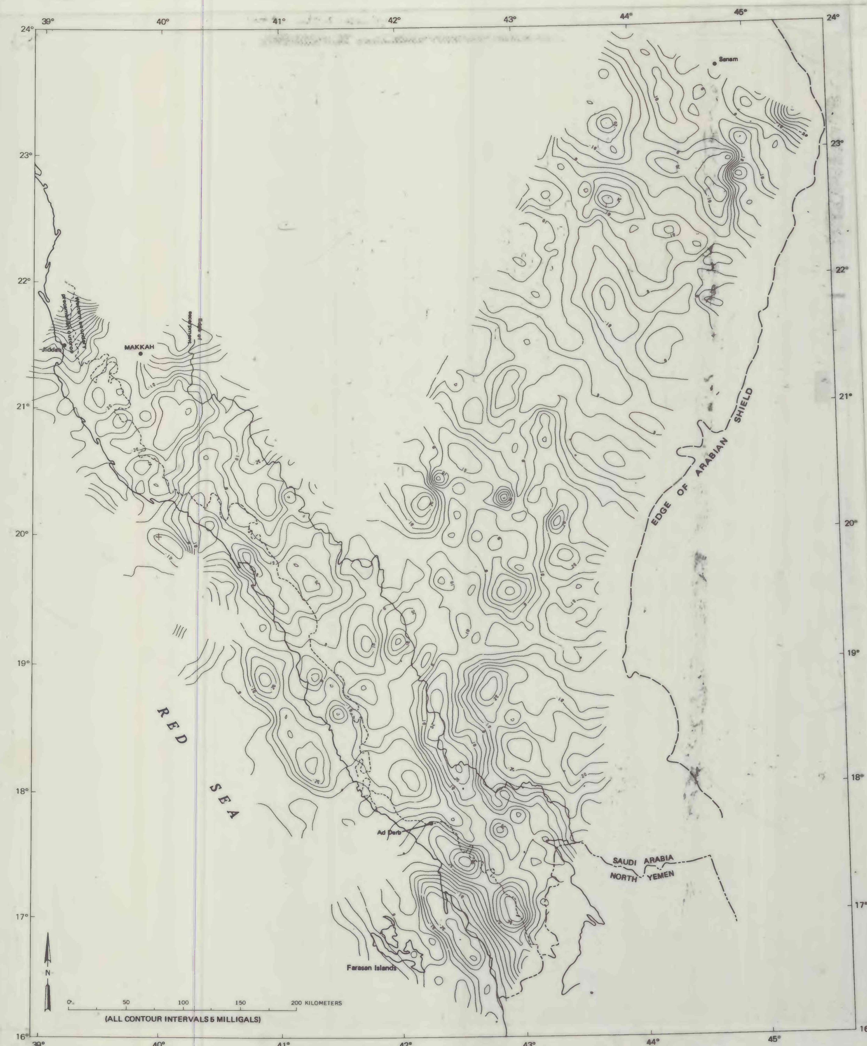
C. Final isostatic gravity anomaly map after correction for model geologic provinces shown in B.
