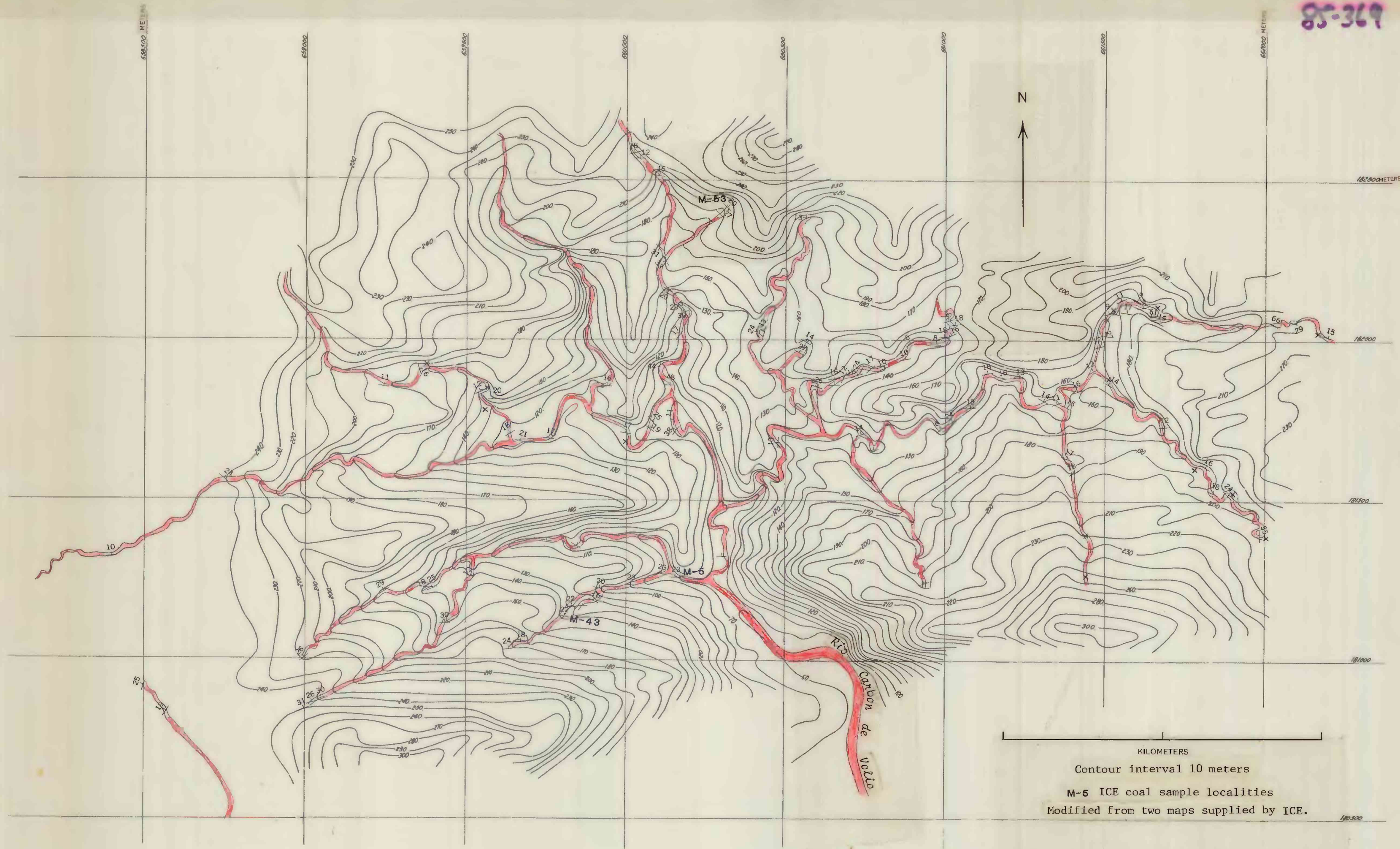
Figure 11. Composite map of the southern part of the drainage basin of Rio Carbon de Volio, showing topography, and location and attitude of coal outcrops.
