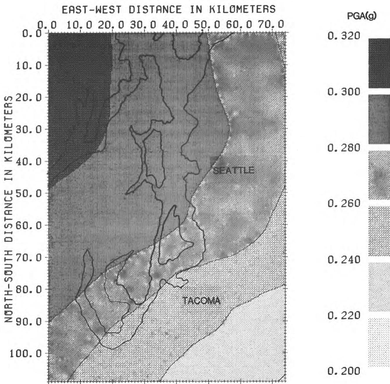
FIGURE TWO - Contour map of peak horizontal ground acceleration in Puget Sound region. Shades represent the PGA for which there is a 95% chance of non-exceedence in 250 years. The shores of Puget Sound are outlined for reference.
