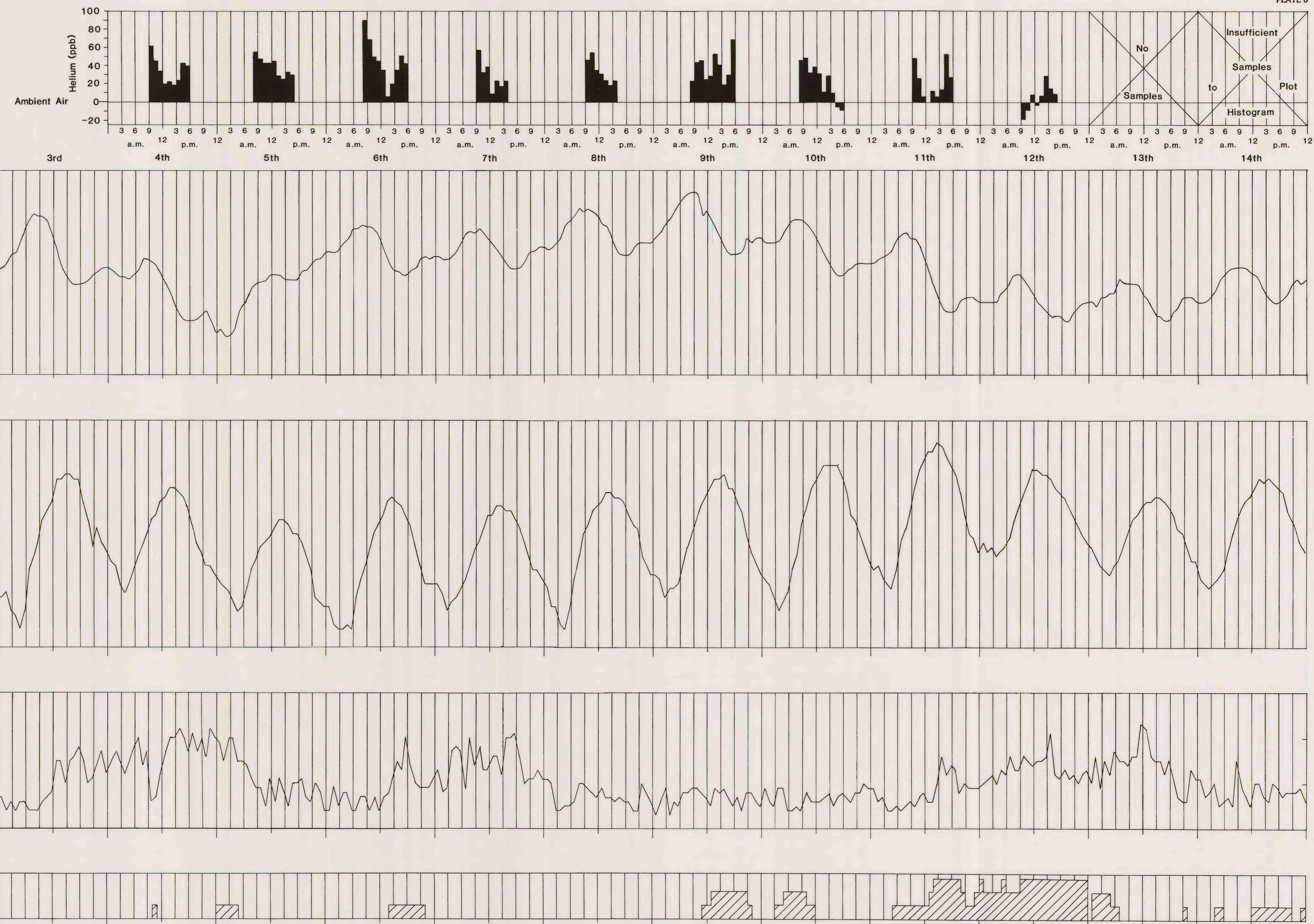
Plate 6. Variations in soil-gas-helium concentration on the Hualapai Indian Reservation as a result of changing meteorologic conditions during June 1982.
