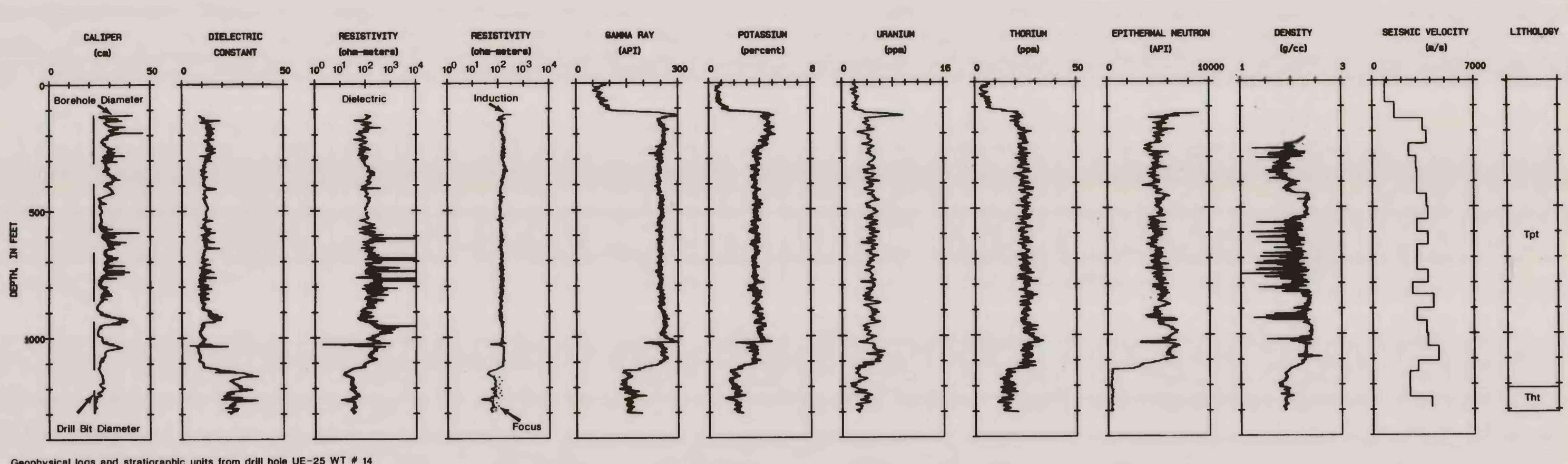
Geophysical logs and stratigraphic units from drill hole UE-25 WT # 14
