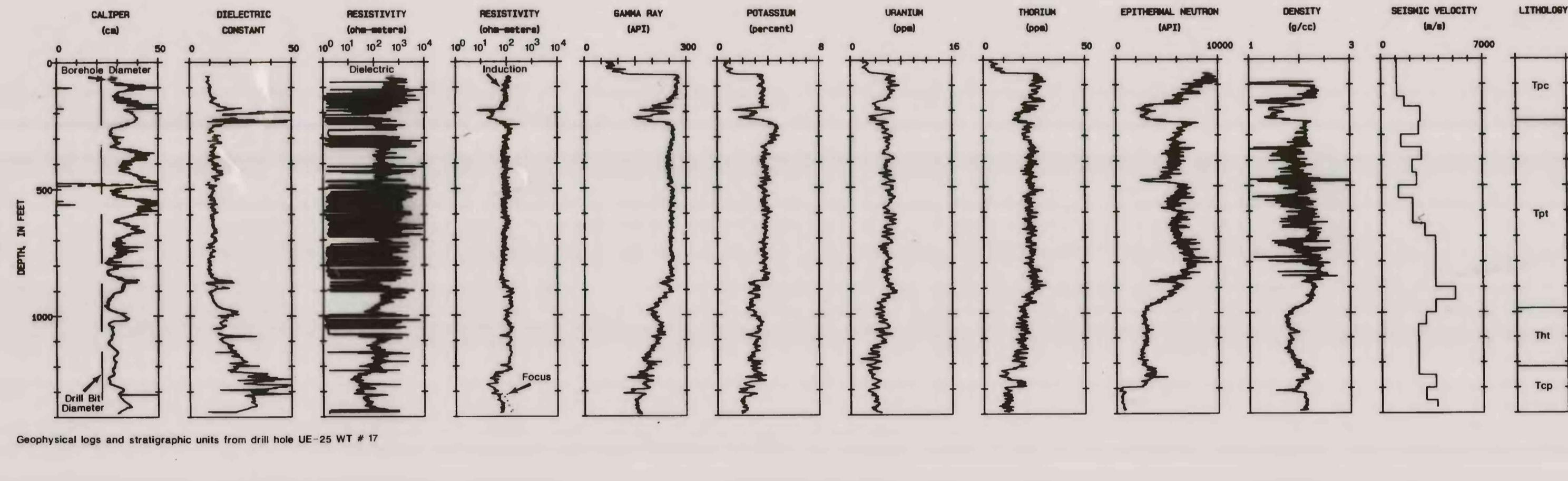
Geophysical logs and stratigraphic units from drill hole UE-25 WT # 17
