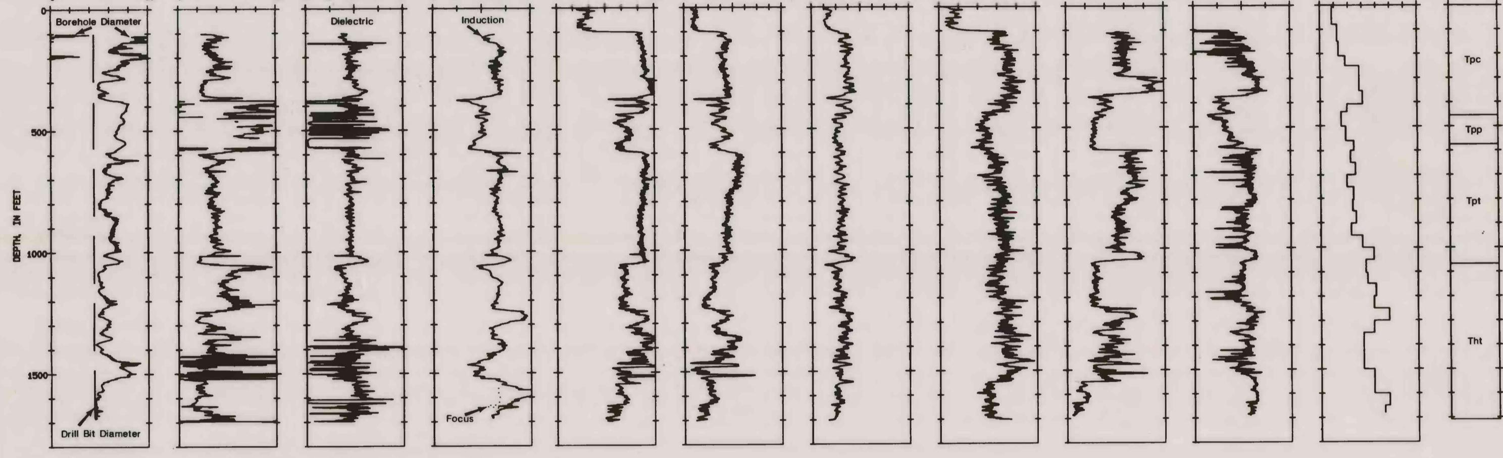
Geophysical logs and stratigraphic units from drill hole UE-25 WT # 16
