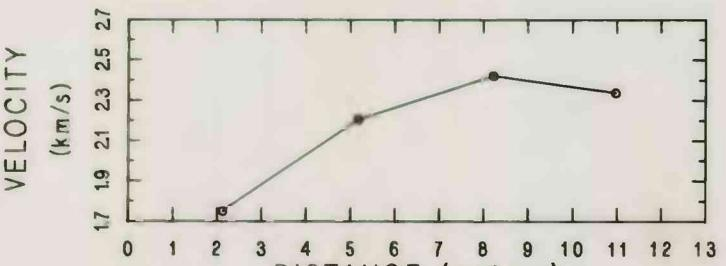
Figure 20.--Results of crosshole seismic velocity surveys in the Ball Room. Distances between holes are shown proportionally with results of surveys centered between holes for which data are representative. Distances refer to distances from the collar of the shothole--3 and 5 in the back, 3 and 4 in the floor.
