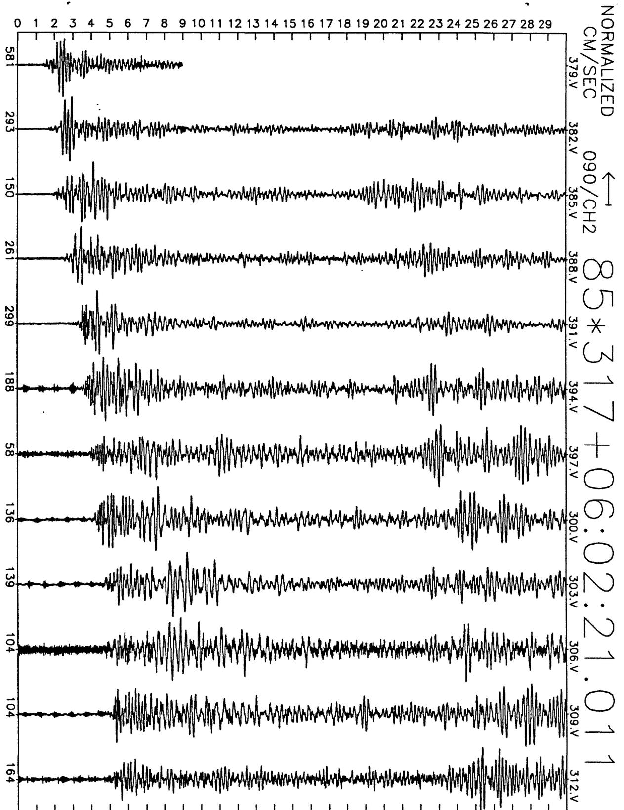
Figure A23(e), shot point 14: 30 second N25E velocity record. Abscissa is labeled with maximum counts in record (multiply by  $\frac{10}{2^{24}-2^8} \approx 6 \times 10^{-7}$  to get cm/sec). Times are unreduced beginning at time indicated.
