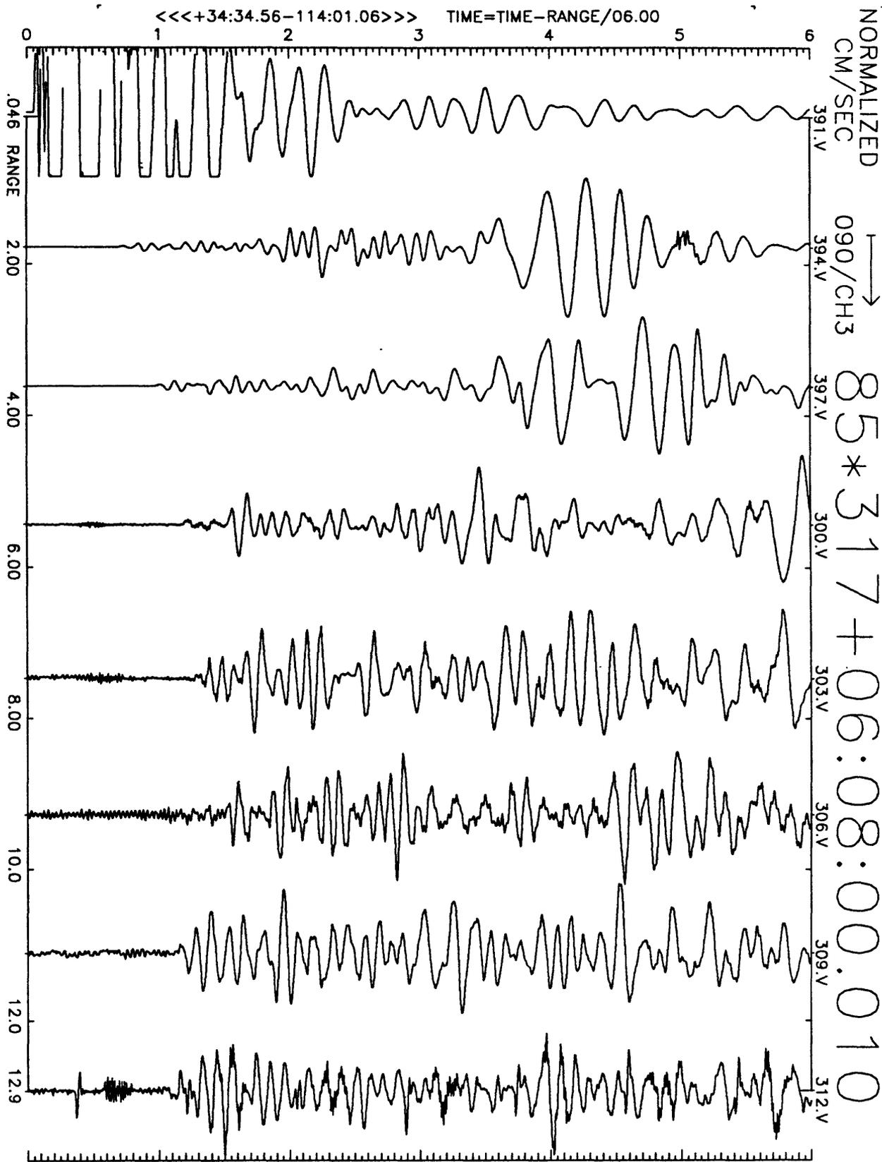
Figure A26(f), shot point 6X, NE stations: 6 second velocity record. Positive N115E motion is to right. Abscissa is distance to shot point. Top of trace is labeled with station number. Times are reduced by 6 km/sec. Shot time is indicated.
