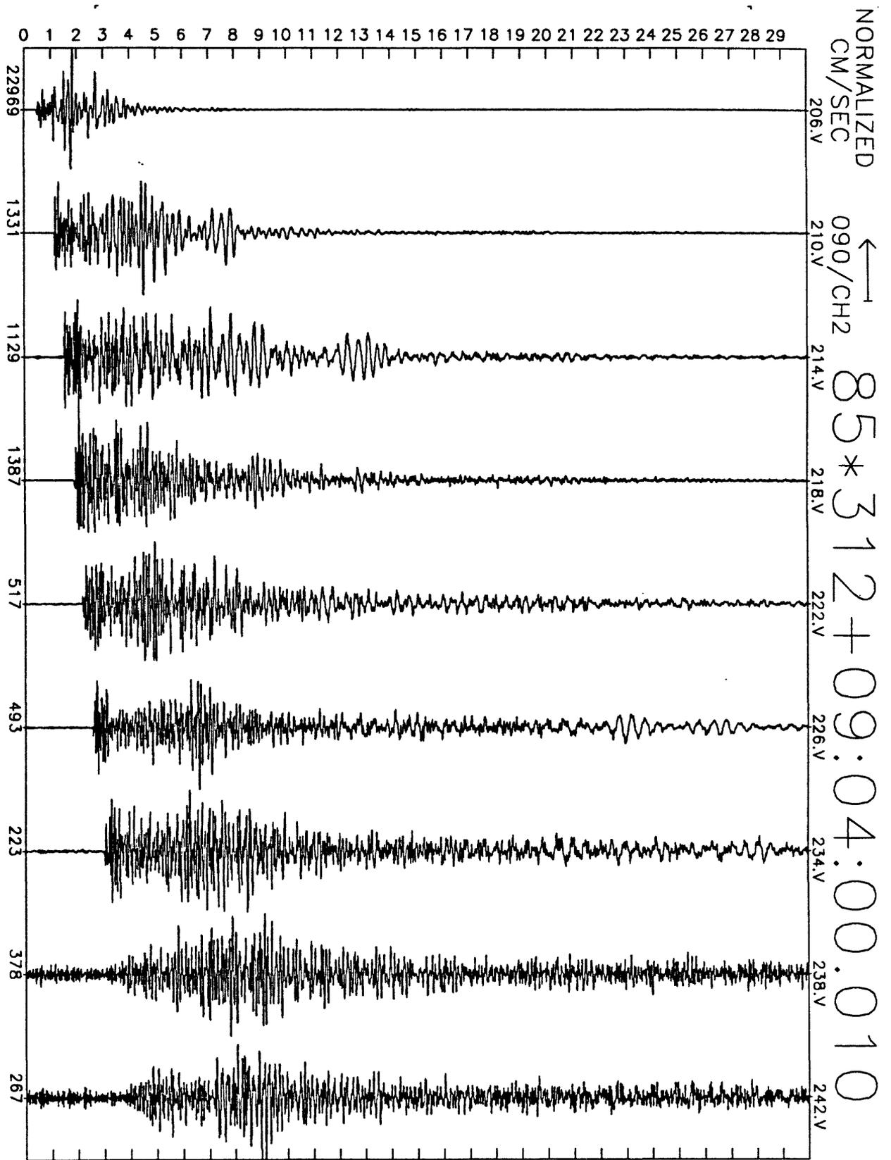
Figure A20(e), shot point 4B: 30 second N20E velocity record. Abscissa is labeled with maximum counts in record (multiply by  $\frac{10}{2^{24}-2^0} \approx 6 \times 10^{-7}$  to get cm/sec). Times are unreduced beginning at time indicated.
