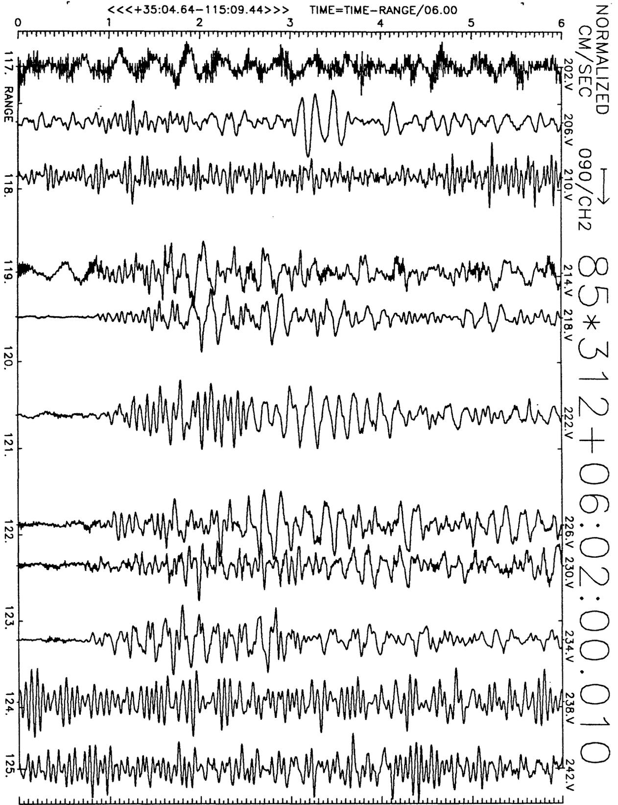
Figure A12(b), shot point 11: 6 second velocity record. Positive N20E motion is to right. Abscissa is distance to shot point. Top of trace is labeled with station number. Times are reduced by 6 km/sec. Shot time is indicated.
