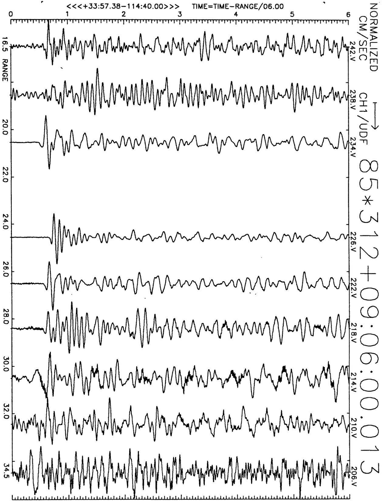
Figure A21(a), shot point 1X: 6 second velocity record. Positive vertical motion is to right. Abscissa is distance to shot point. Top of trace is labeled with station number. Times are reduced by 6 km/sec. Shot time is indicated.
