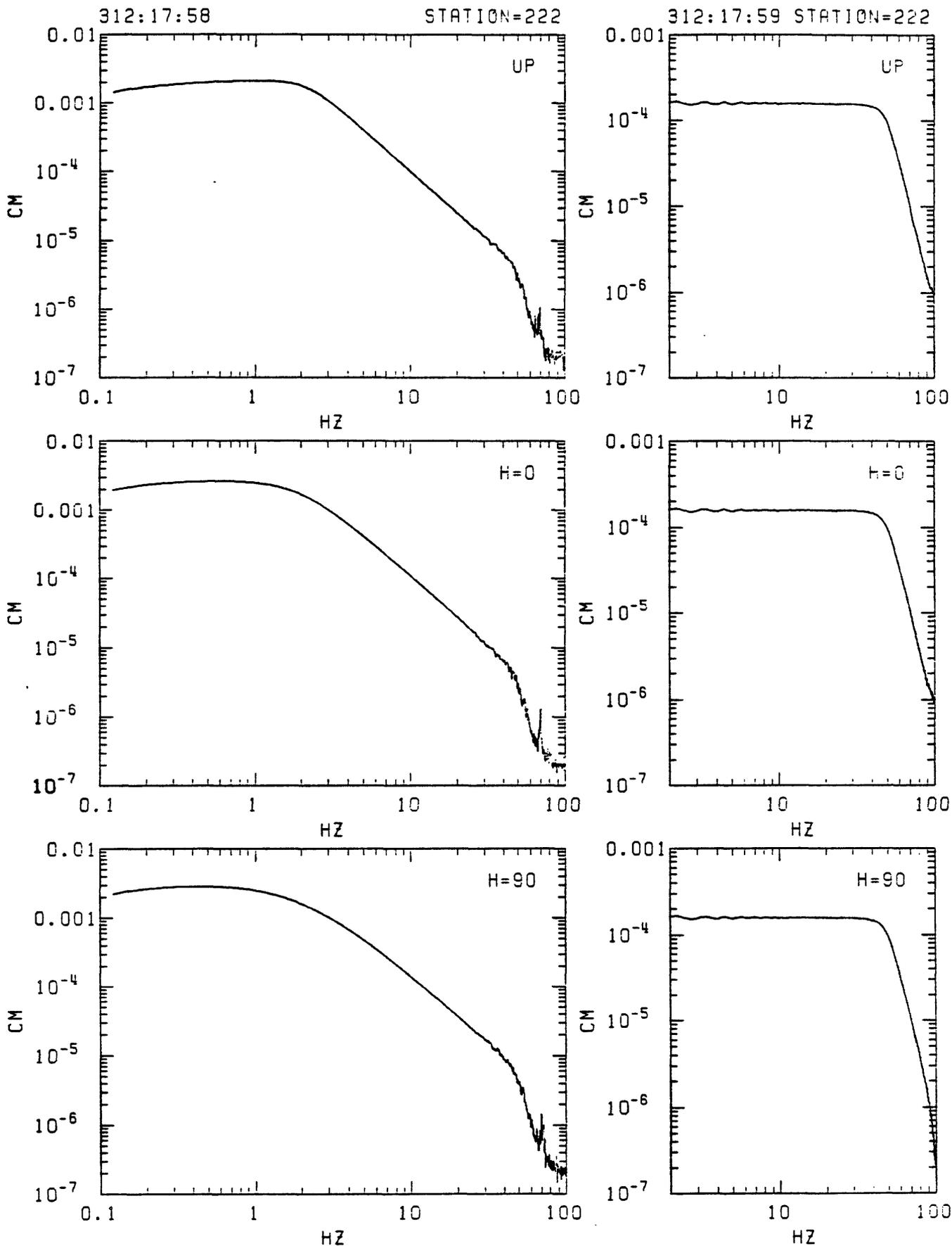
Figure C16. Station 222 in-situ velocity calibration spectra. Left: response to step in acceleration (seismometer mass released from rest at offset position). Right: response to delta function in velocity (voltage impulse applied to recorder input). From top: vertical, N20E and N110E.
