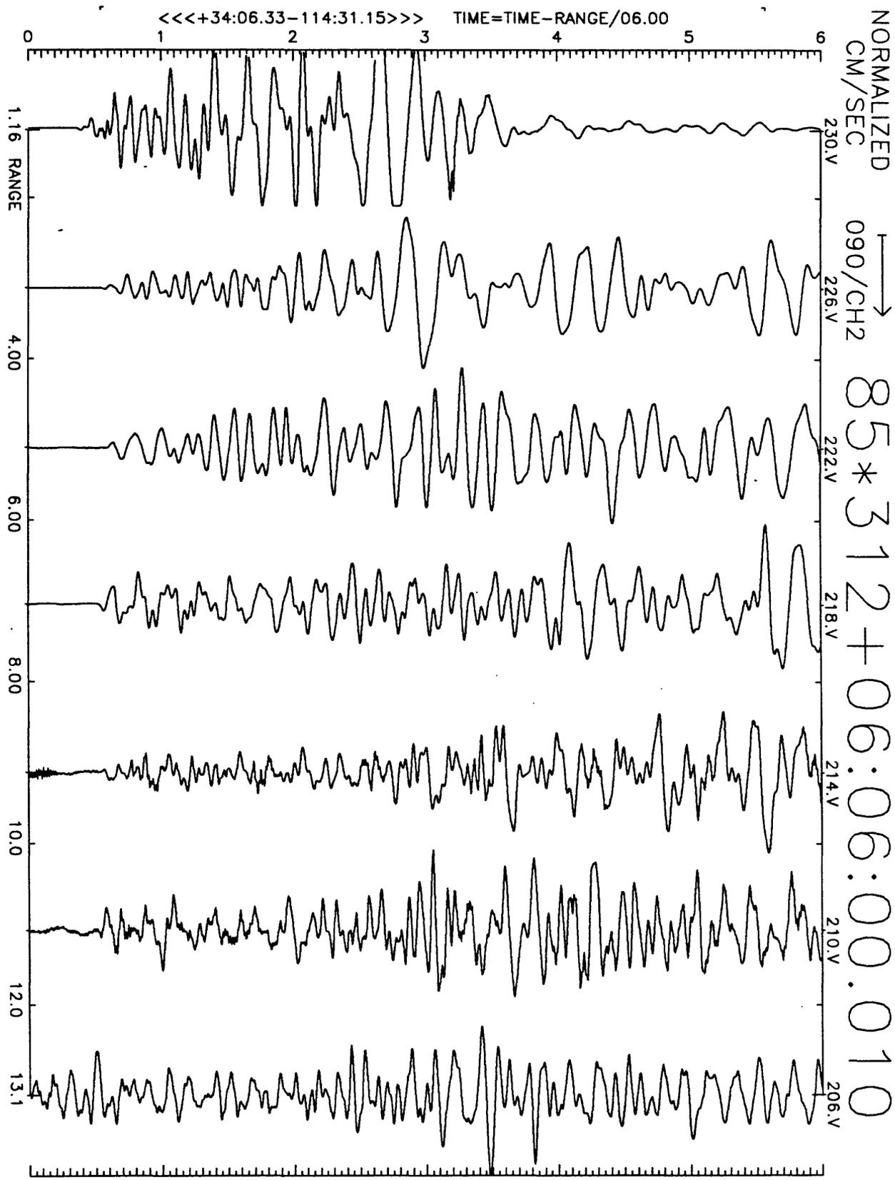
Figure A14(e), shot point 3, NE stations: 6 second velocity record. Positive N20E motion is to right. Abscissa is distance to shot point. Top of trace is labeled with station number. Times are reduced by 6 km/sec. Shot time is indicated.
