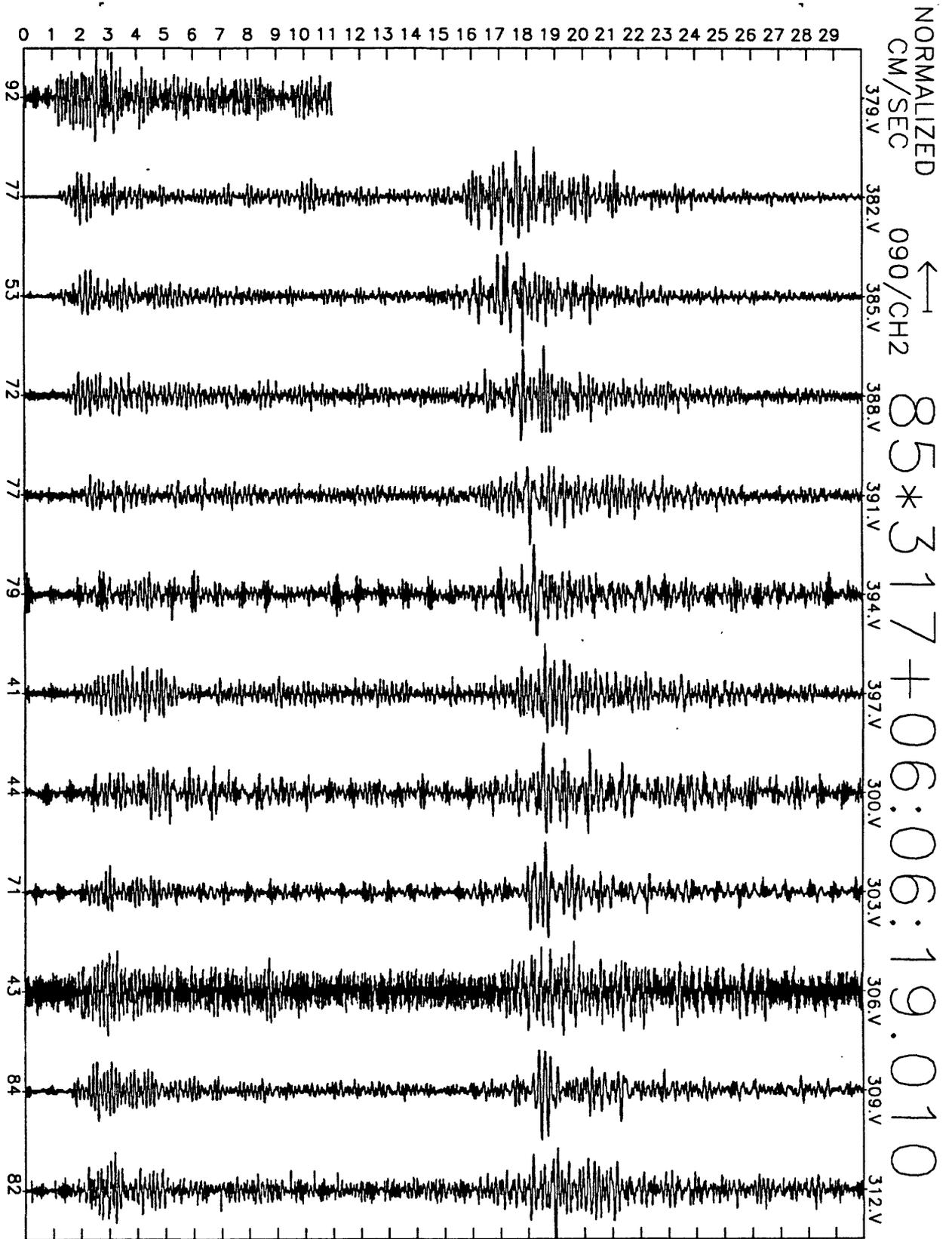
Figure A25(e), shot point 11: 30 second N25E velocity record. Abscissa is labeled with maximum counts in record (multiply by  $\frac{10}{224-25} \approx 6 \times 10^{-7}$  to get cm/sec). Times are unreduced beginning at time indicated.
