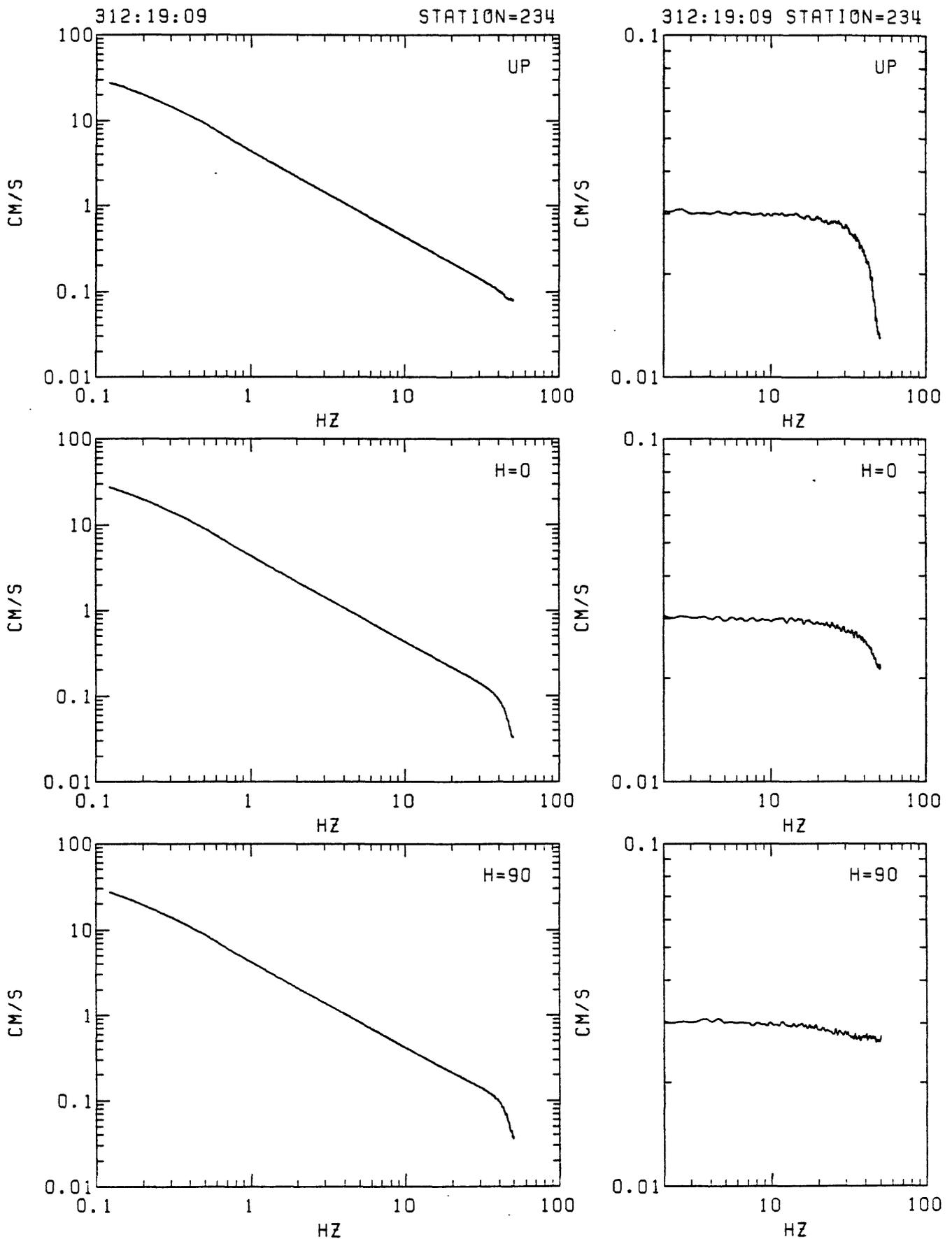
Figure D5. Station 234 in-situ 18db acceleration calibration spectra. Left: response to step in acceleration (reset FBA servo amplifier reference voltage from non-zero). Right: response to delta function in acceleration (voltage impulse applied to recorder input). From top: vertical, N20E and N110E.
