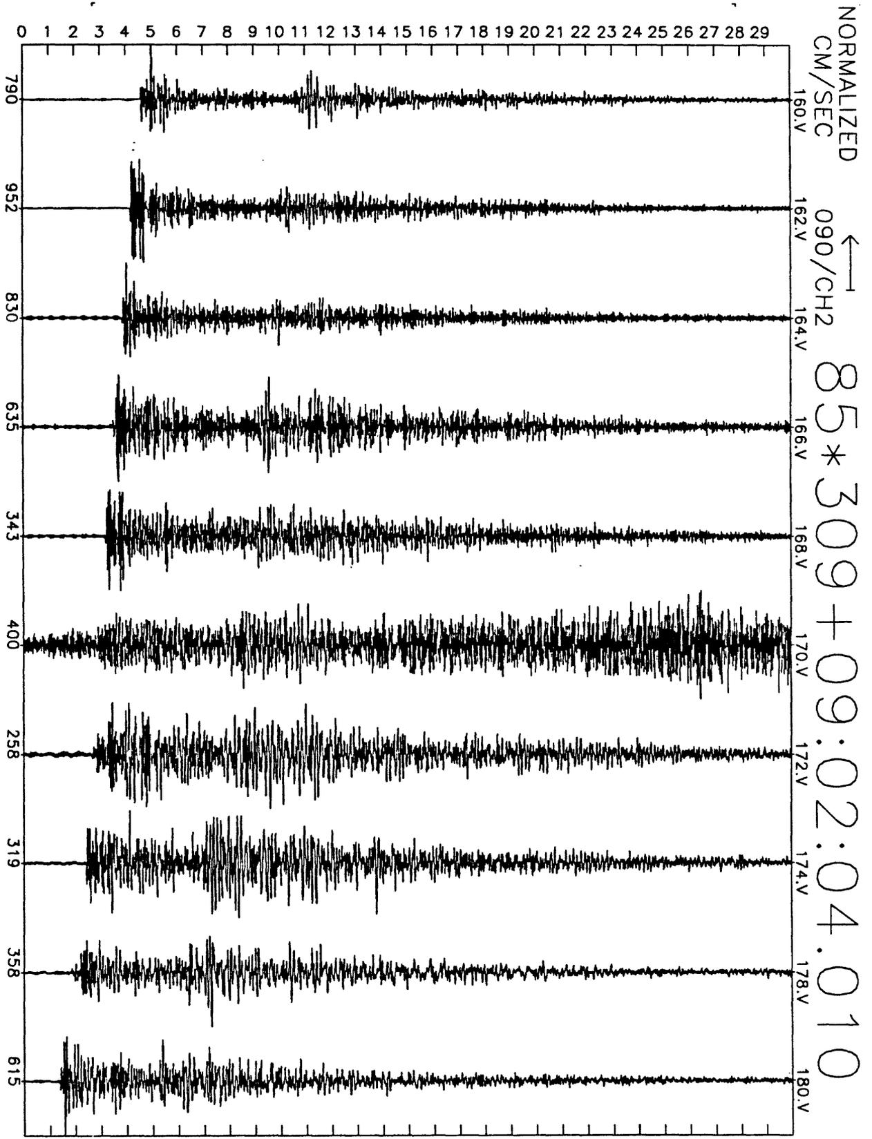
Figure A7(e), shot point 10: 30 second N33W velocity record. Abscissa is labeled with maximum counts in record (multiply by  $\frac{10}{2^{24}-2^8} \approx 6 \times 10^{-7}$  to get cm/sec). Times are unreduced beginning at time indicated.
