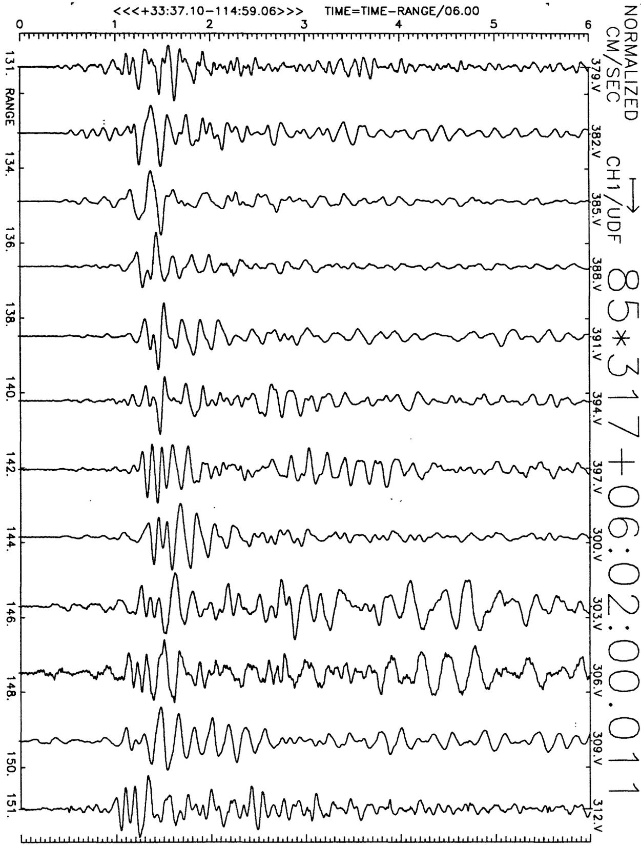
Figure A23(a), shot point 14: 6 second velocity record. Positive vertical motion is to right. Abscissa is distance to shot point. Top of trace is labeled with station number. Times are reduced by 6 km/sec. Shot time is indicated.
