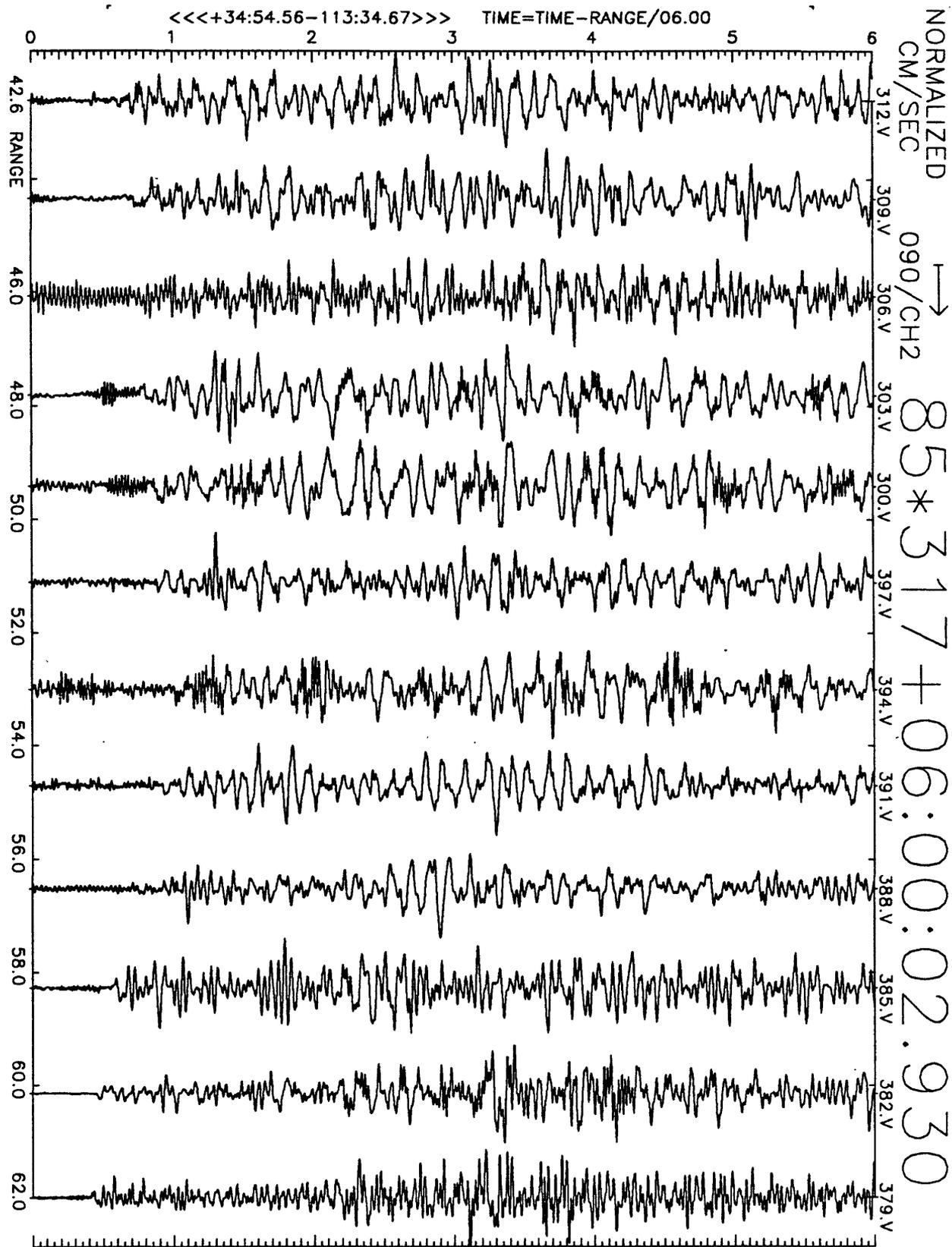
Figure A22(b), shot point 12: 6 second velocity record. Positive N25E motion is to right. Abscissa is distance to shot point. Top of trace is labeled with station number. Times are reduced by 6 km/sec. Shot time is indicated.
