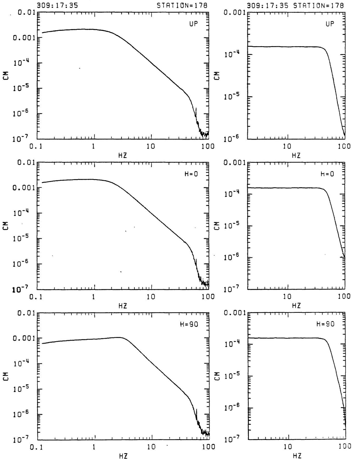
Figure C9. Station 178 in-situ velocity calibration spectra. Left: response to step in acceleration (seismometer mass released from rest at offset position). Right: response to delta function in velocity (voltage impulse applied to recorder input). From top: vertical, N33W and N57E.
