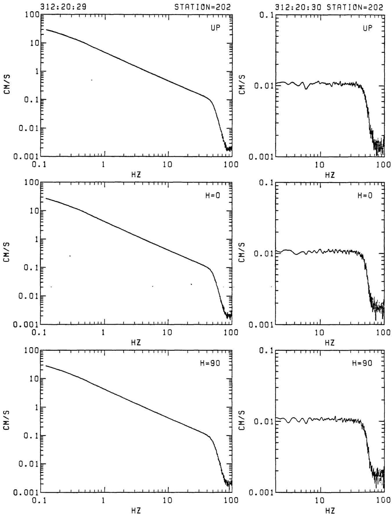
Figure D4. Station 202 in-situ 12db acceleration calibration spectra. Left: response to step in acceleration (reset FBA servo amplifier reference voltage from non-zero). Right: response to delta function in acceleration (voltage impulse applied to recorder input). From top: vertical, N20E and N110E.
