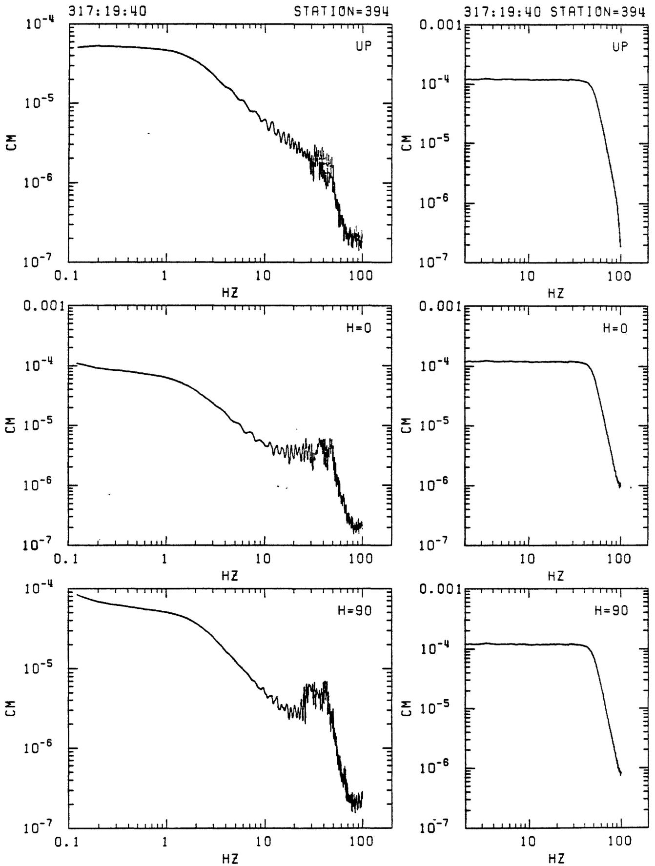
Figure C25. Station 394 in-situ velocity calibration spectra. Left: response to step in acceleration (seismometer mass released from rest at offset position). Right: response to delta function in velocity (voltage impulse applied to recorder input). From top: vertical, N25E and N115E.
