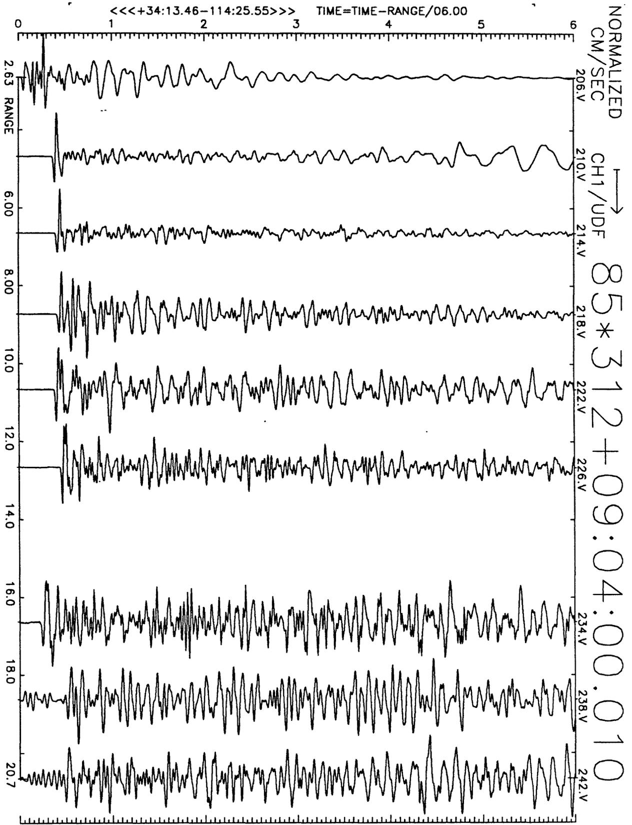
Figure A20(a), shot point 4B: 6 second velocity record. Positive vertical motion is to right. Abscissa is distance to shot point. Top of trace is labeled with station number. Times are reduced by 6 km/sec. Shot time is indicated.
