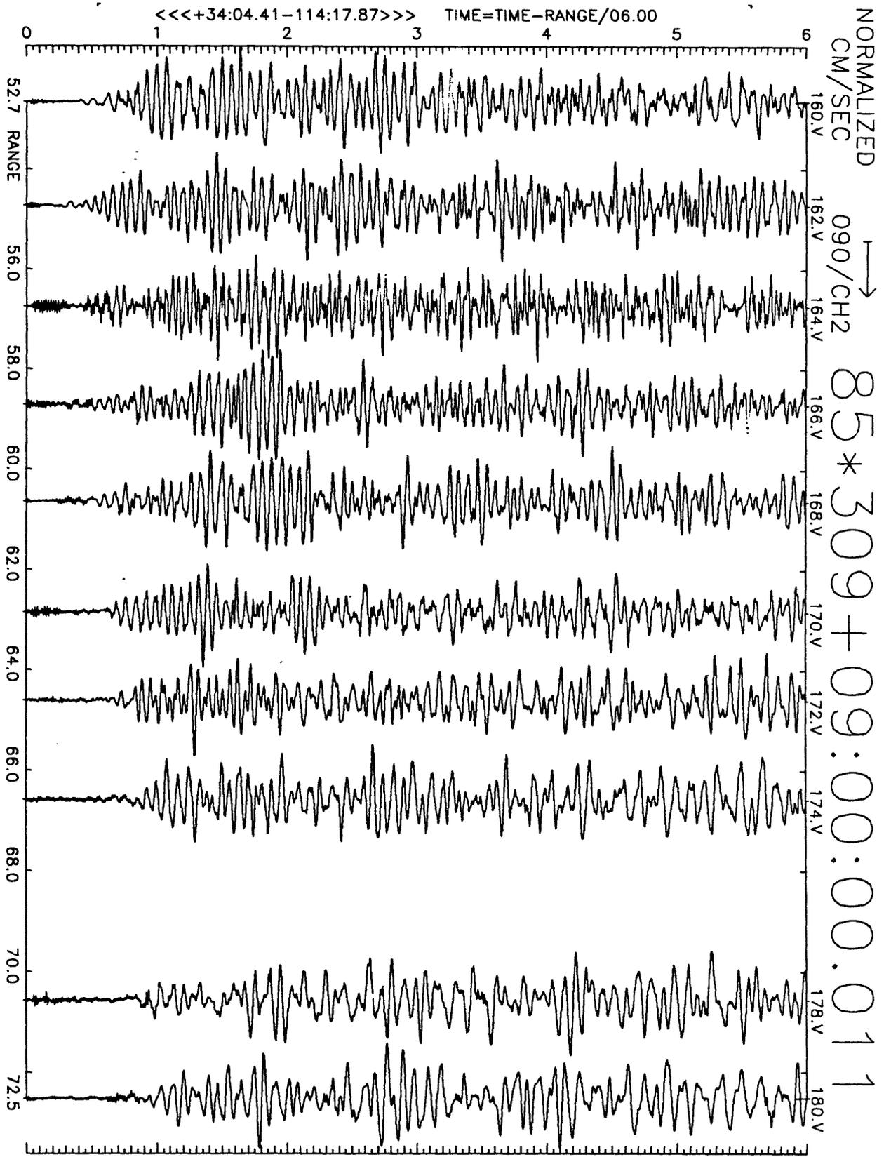
Figure A6(b), shot point 8X: 6 second velocity record. Positive N33W motion is to right. Abscissa is distance to shot point. Top of trace is labeled with station number. Times are reduced by 6 km/sec. Shot time is indicated.
