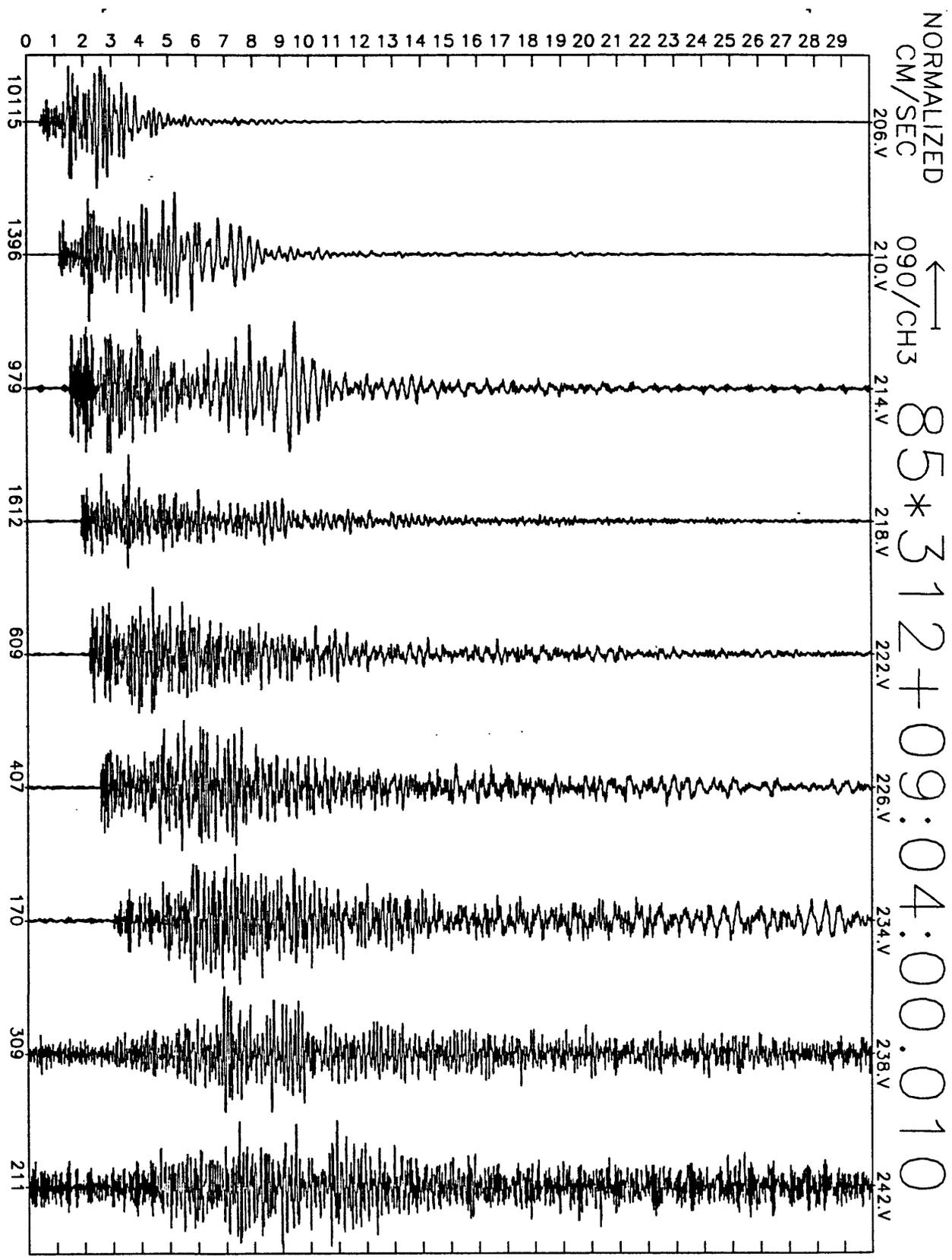
Figure A20(f), shot point 4B: 30 second N110E velocity record. Abscissa is labeled with maximum counts in record (multiply by  $\frac{10}{2^{24}-2^8} \approx 6 \times 10^{-7}$  to get cm/sec). Times are unreduced beginning at time indicated.
