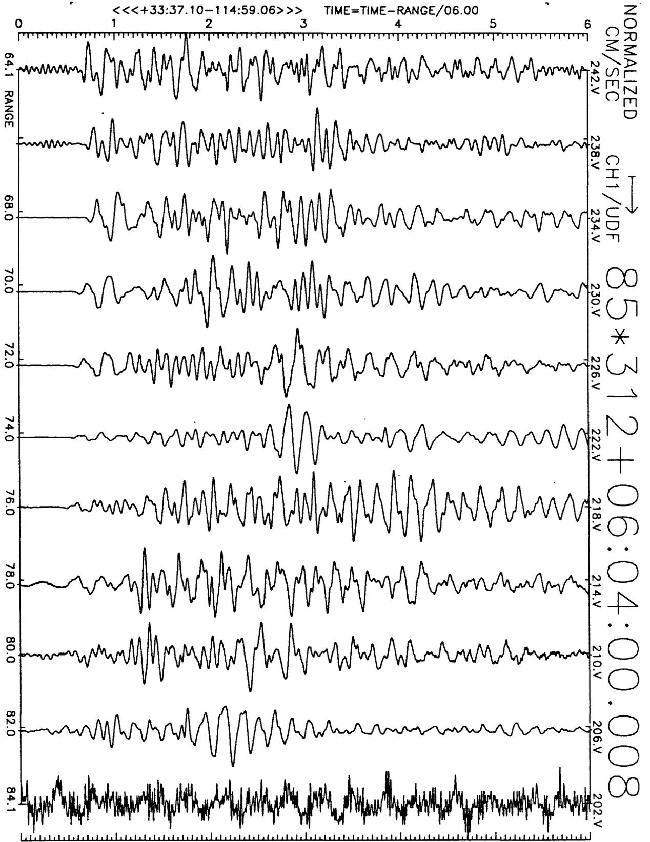
Figure A13(a), shot point 14: 6 second velocity record. Positive vertical motion is to right. Abscissa is distance to shot point. Top of trace is labeled with station number. Times are reduced by 6 km/sec. Shot time is indicated.
