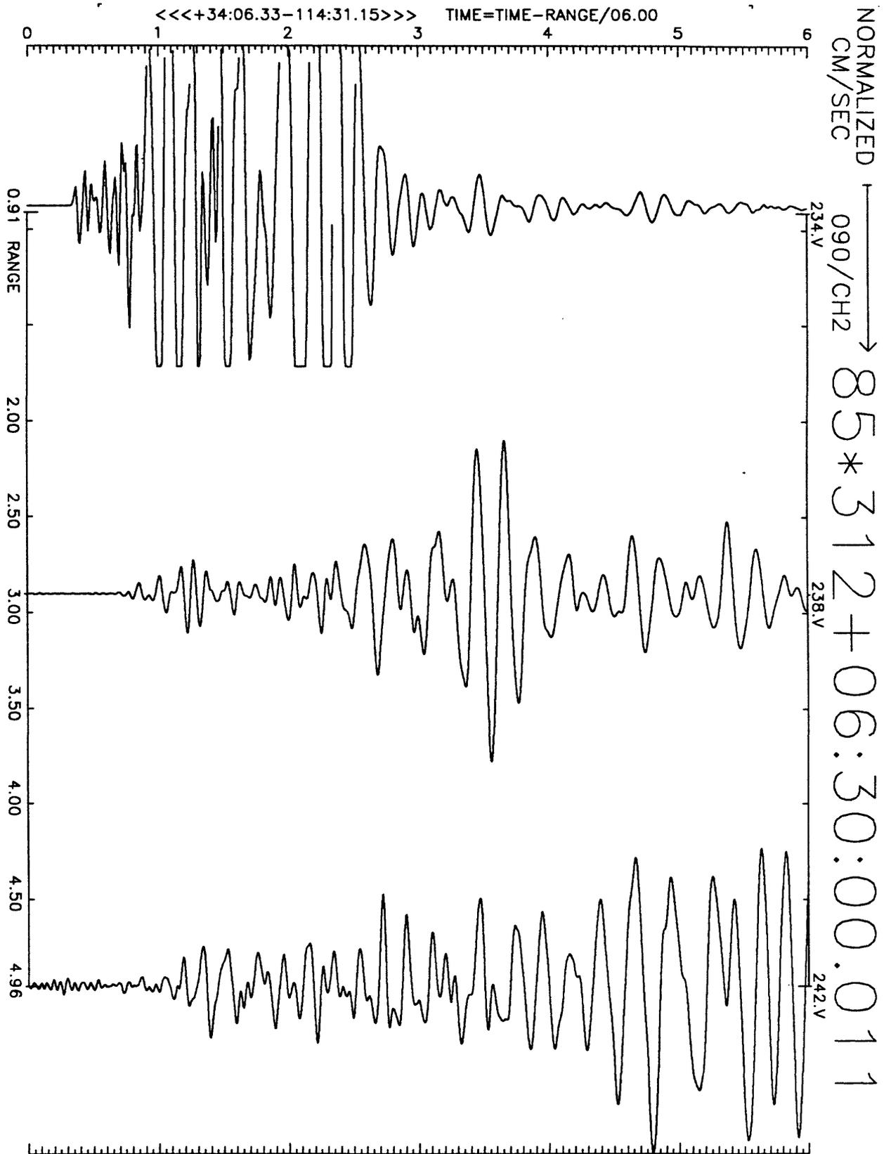
Figure A16(b), shot point 3', SW stations: 6 second velocity record. Positive N20E motion is to right. Abscissa is distance to shot point. Top of trace is labeled with station number. Times are reduced by 6 km/sec. Shot time is indicated.
