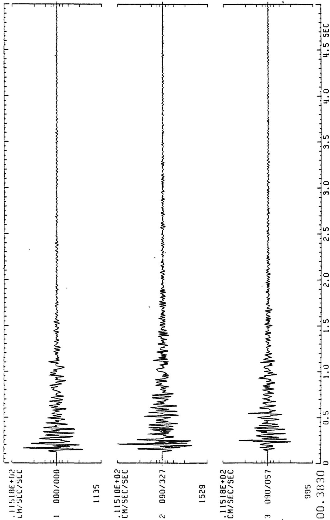
Figure B1(a), shot point 9: Three component accelerogram for station 164. Lower traces show horizontal motion. Azimuths are indicated immediately to the left of the traces. Start time is arbitrary.
