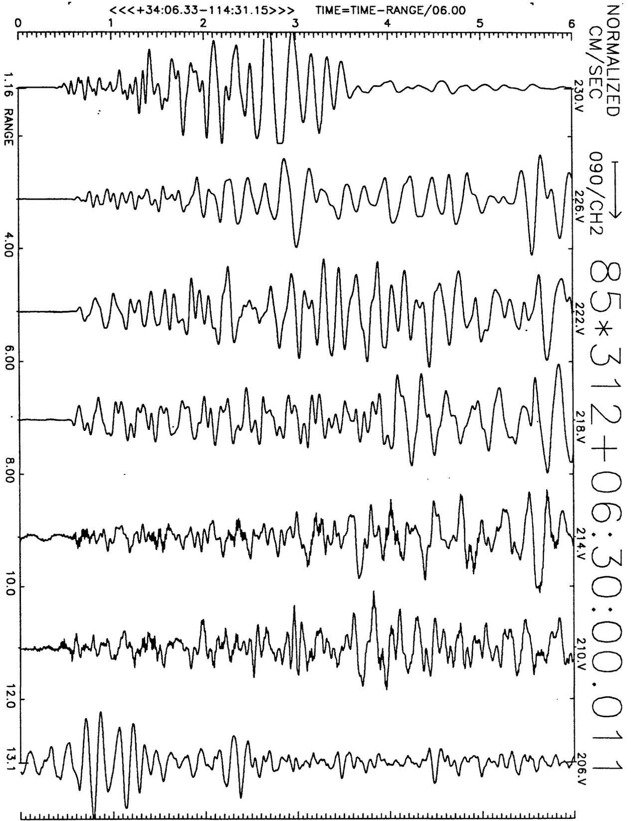
Figure A16(e), shot point 3', NE stations: 6 second velocity record. Positive N20E motion is to right. Abscissa is distance to shot point. Top of trace is labeled with station number. Times are reduced by 6 km/sec. Shot time is indicated.
