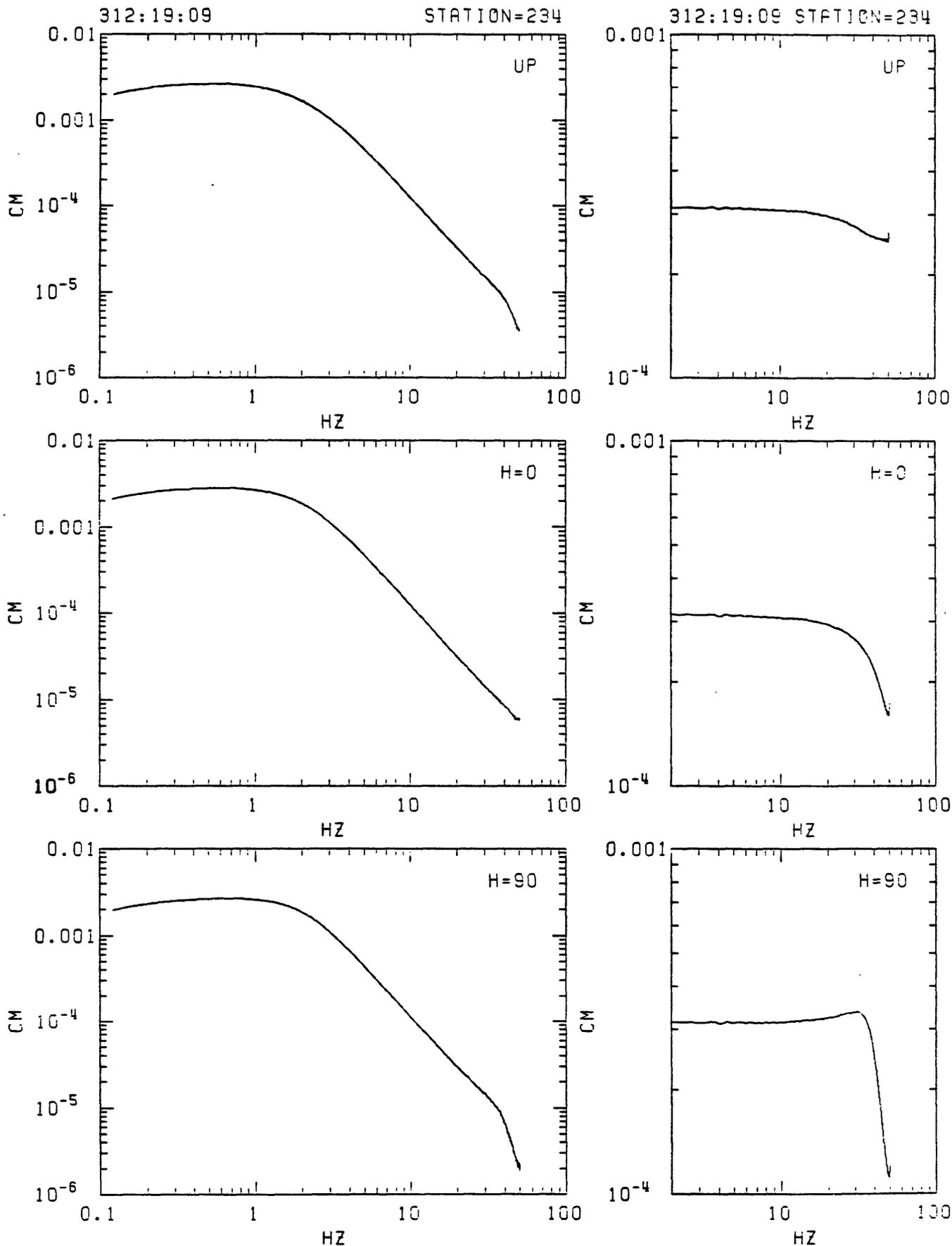
Figure C18. Station 234 in-situ velocity calibration spectra. Left: response to step in acceleration (seismometer mass released from rest at offset position). Right: response to delta function in velocity (voltage impulse applied to recorder input). From top: vertical, N20E and N110E.
