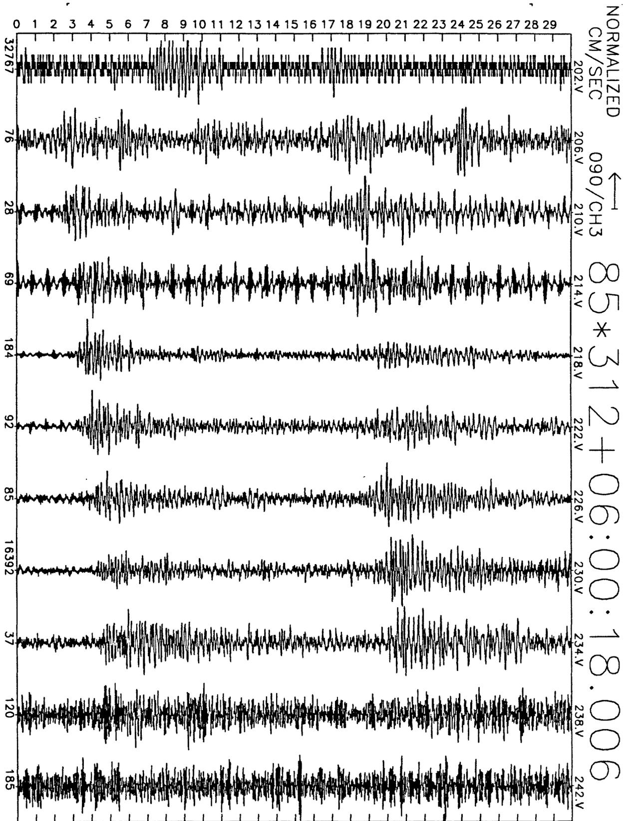
Figure A11(f), shot point 12: 30 second N110E velocity record. Abscissa is labeled with maximum counts in record (multiply by  $\frac{10}{2^{24}-2^8} \approx 6 \times 10^{-7}$  to get cm/sec). Times are unreduced beginning at time indicated.
