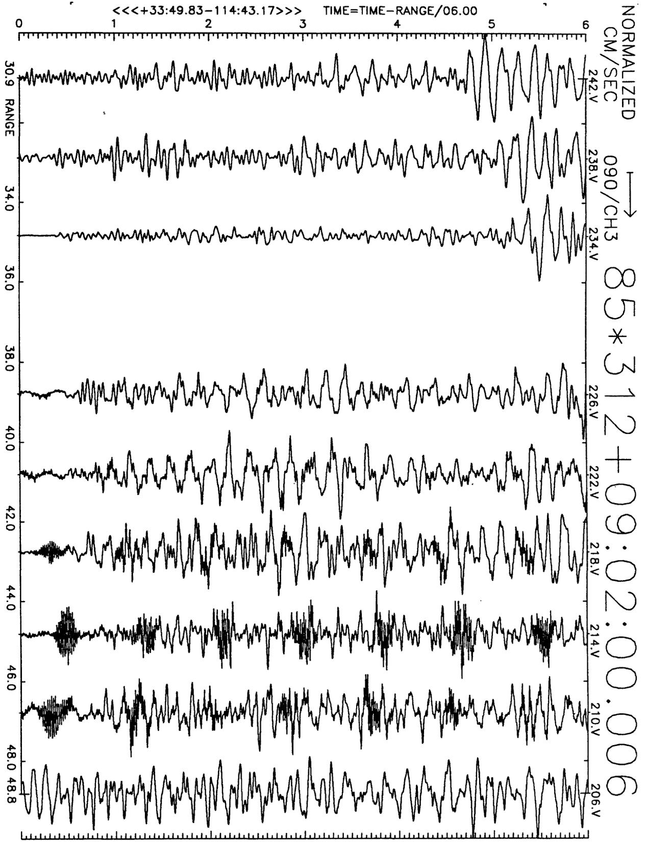
Figure A19(c), shot point 1: 6 second velocity record. Positive N110E motion is to right. Abscissa is distance to shot point. Top of trace is labeled with station number. Times are reduced by 6 km/sec. Shot time is indicated.
