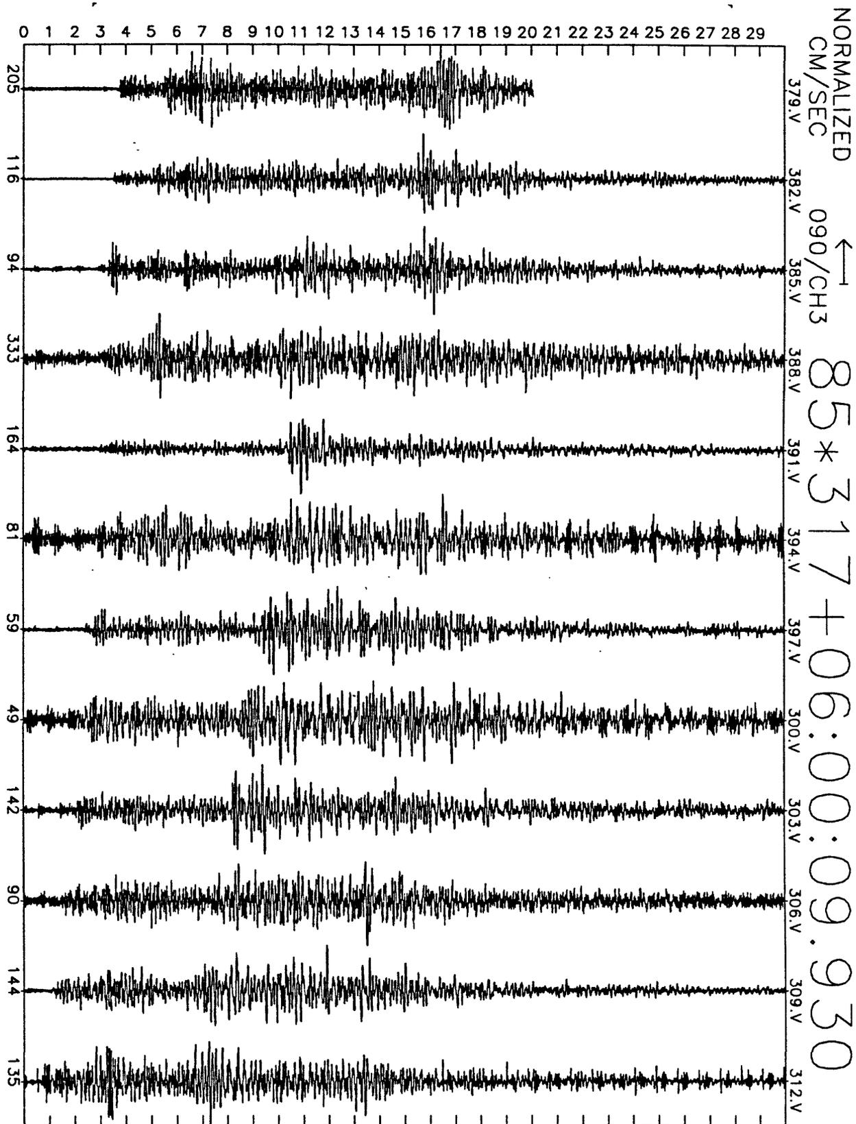
Figure A23(d), shot point 14: 30 second vertical velocity record. Abscissa is labeled with maximum counts in record (multiply by  $\frac{10}{2^{14}-2^5} \approx 6 \times 10^{-7}$  to get cm/sec). Times are unreduced beginning at time indicated.
