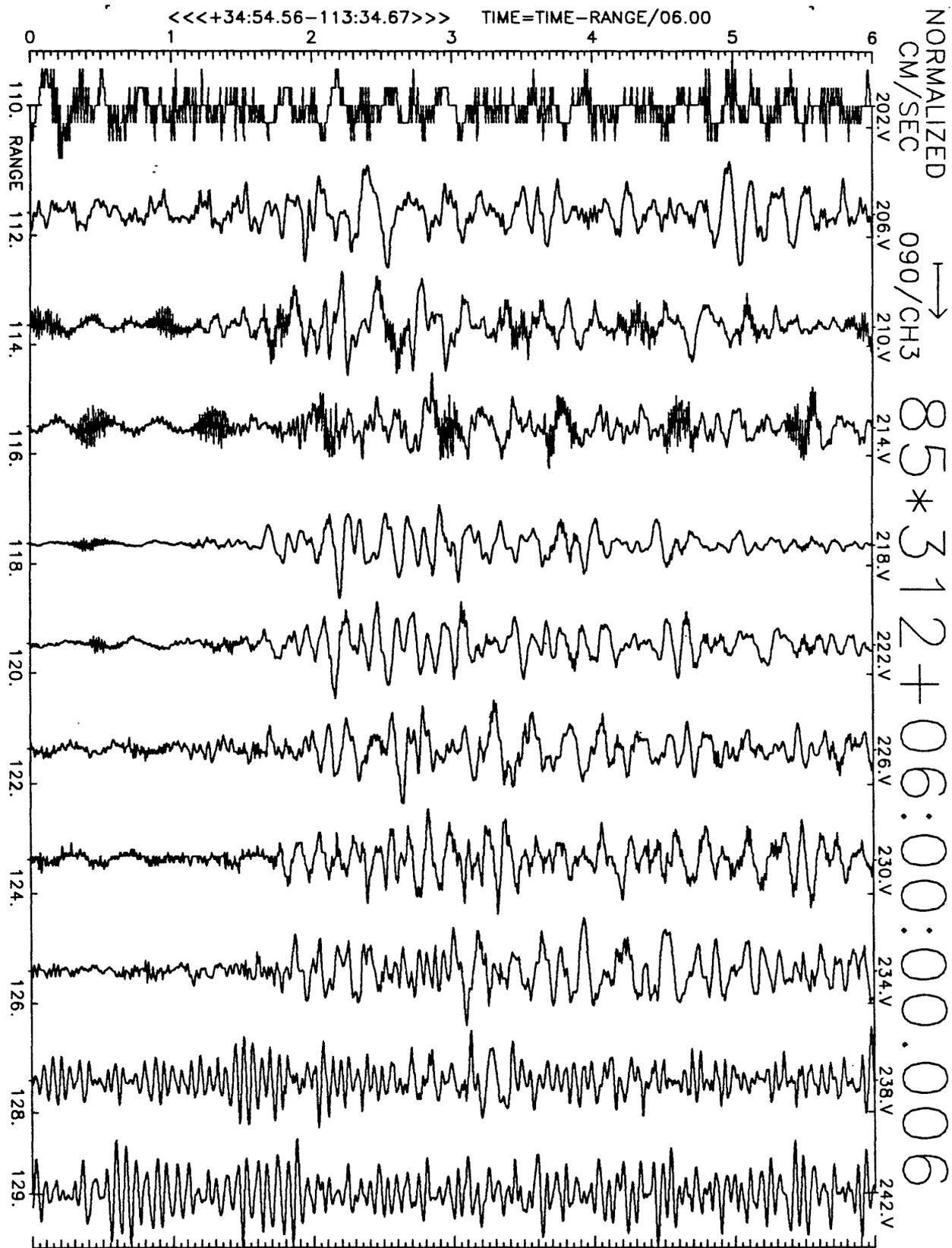
Figure A11(c), shot point 12: 6 second velocity record. Positive N110E motion is to right. Abscissa is distance to shot point. Top of trace is labeled with station number. Times are reduced by 6 km/sec. Shot time is indicated.
