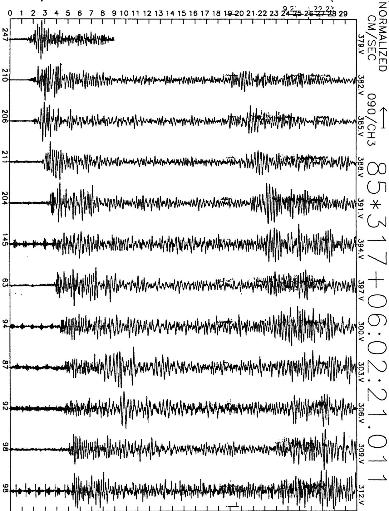
Figure A23(f), shot point 14: 30 second N115E velocity record. Abscissa is labeled with maximum counts in record (multiply by  $\frac{10}{2^{24}-2^8} \approx 6 \times 10^{-7}$  to get cm/sec). Times are unreduced beginning at time indicated.
