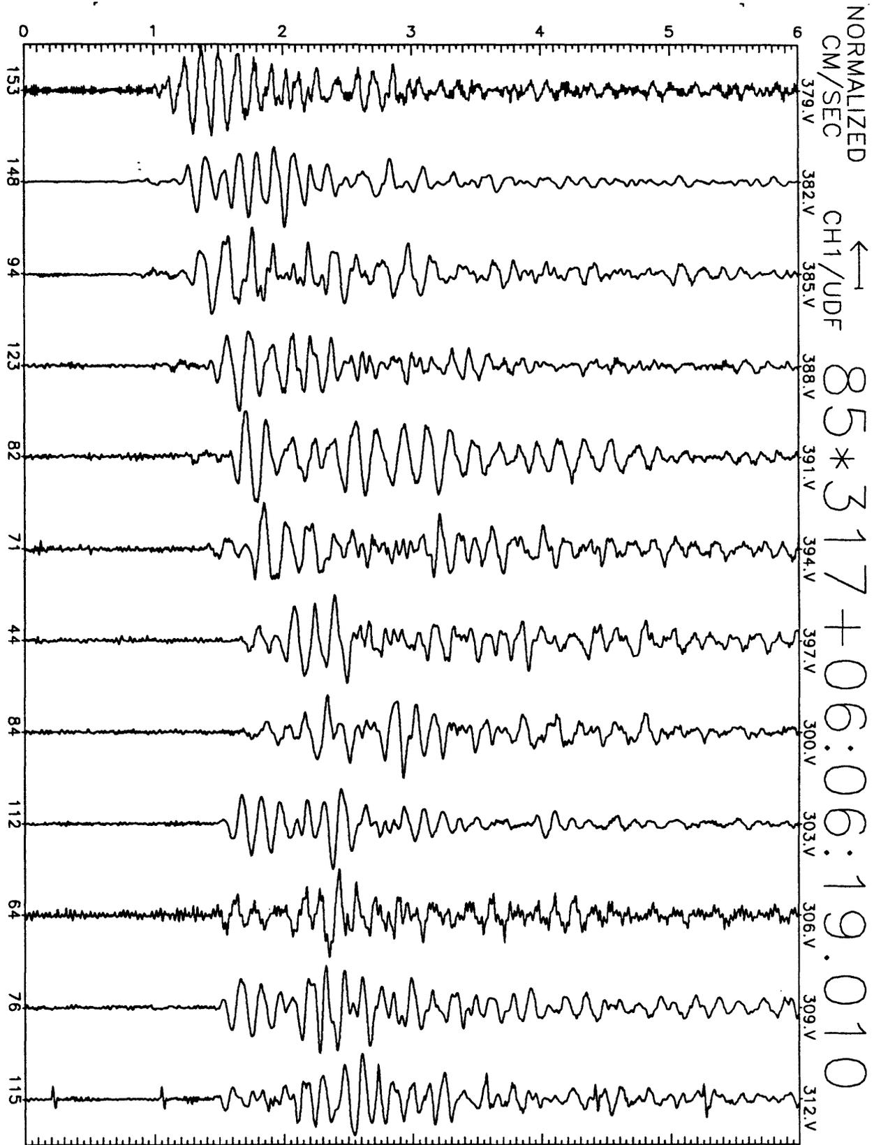
Figure A25(a), shot point 11 (fan shot): 6 second velocity record. Positive vertical motion is to left. Abscissa is labeled with maximum counts in record. Distances are  $\sim 117.5 \pm 1.5 \text{ km}$ . Times are unreduced beginning at shot time + 19 seconds.
