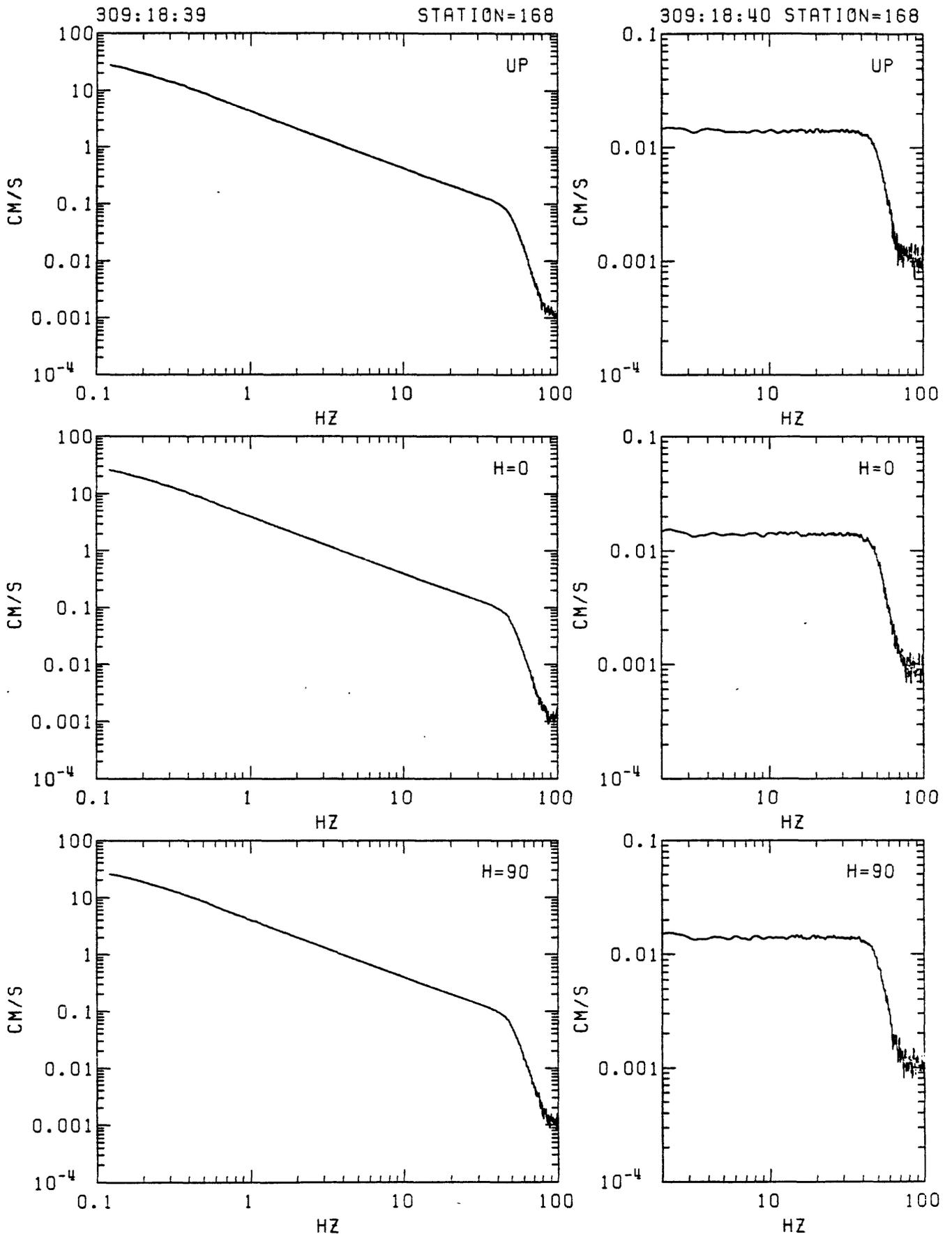
Figure D3. Station 168 in-situ 18db acceleration calibration spectra. Left: response to step in acceleration (reset FBA servo amplifier reference voltage from non-zero). Right: response to delta function in acceleration (voltage impulse applied to recorder input). From top: vertical, N33W and N57W.
