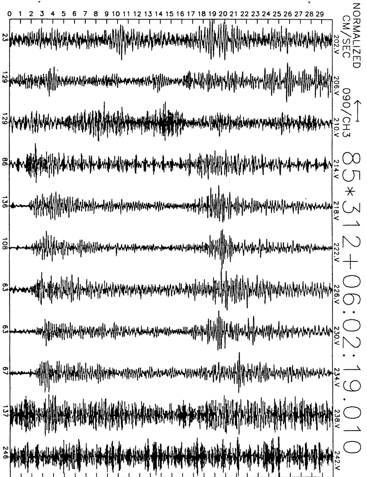
Figure A12(f), shot point 11: 30 second N110E velocity record. Abscissa is labeled with maximum counts in record (multiply by  $\frac{10}{2^{24}-2^8} \approx 6 \times 10^{-7}$  to get cm/sec). Times are unreduced beginning at time indicated.
