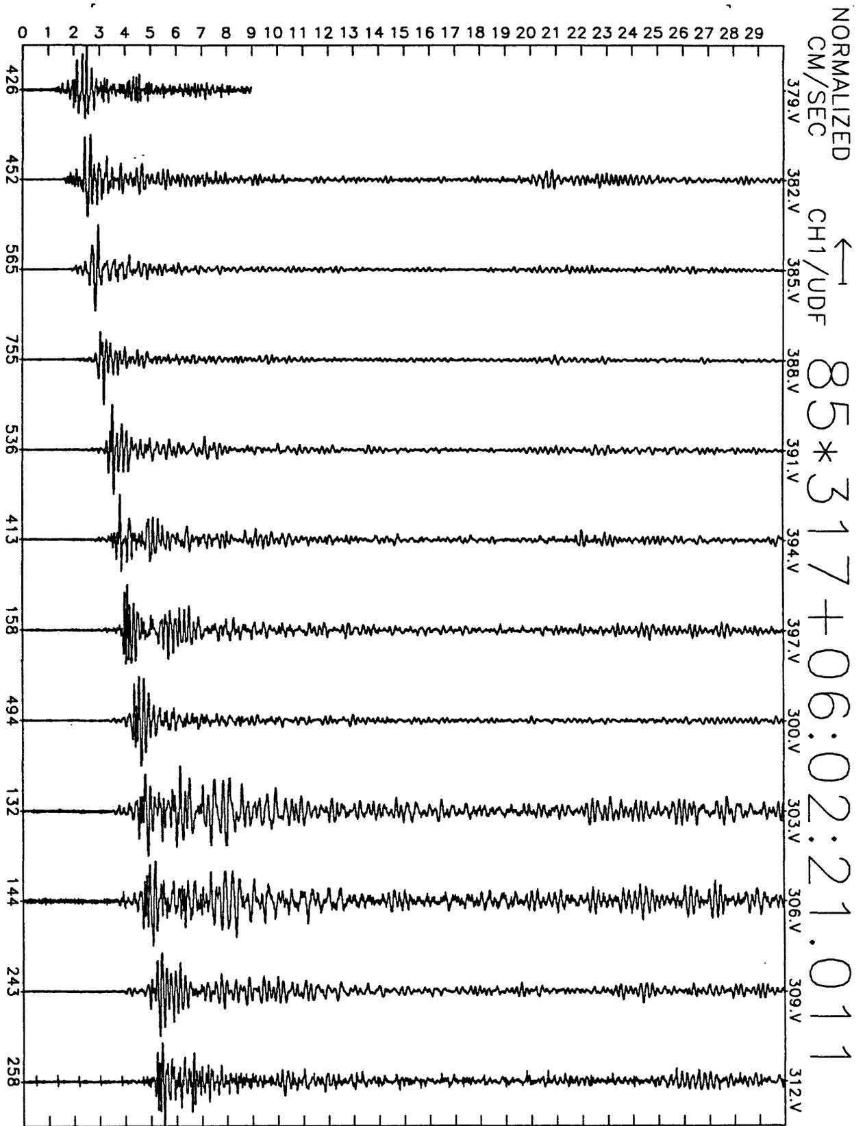
Figure A22(d), shot point 12: 30 second vertical velocity record. Abscissa is labeled with maximum counts in record (multiply by  $\frac{10}{2^{24}-2^8} \approx 6 \times 10^{-7}$  to get cm/sec). Times are unreduced beginning at time indicated.
