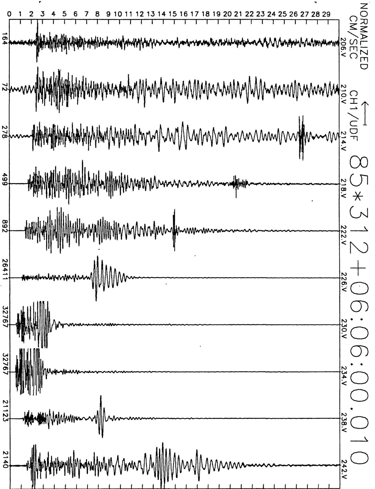
Figure A14(g), shot point 3: 30 second vertical velocity record. Abscissa is labeled with maximum counts in record (multiply by  $\frac{10}{2^{24}-2^8} \approx 6 \times 10^{-7}$  to get cm/sec). Times are unreduced beginning at time indicated.
