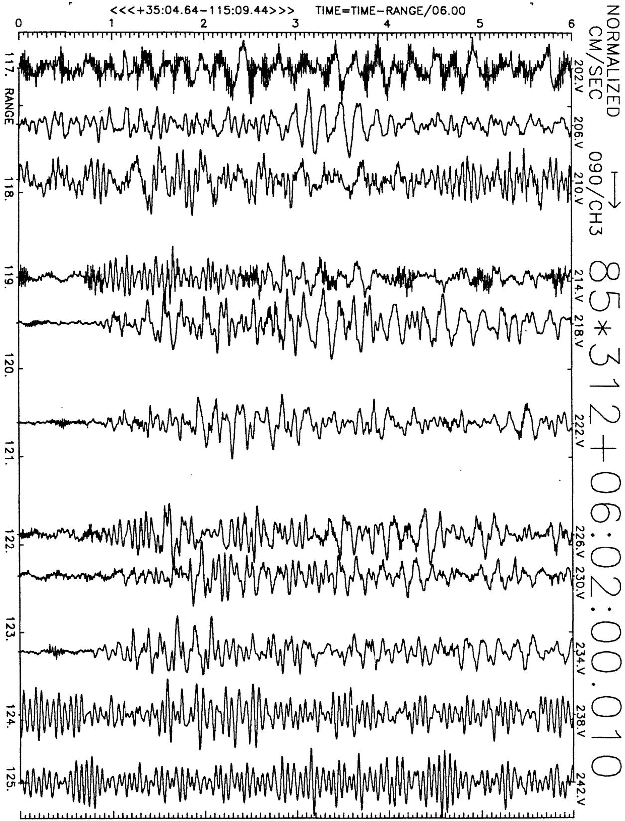
Figure A12(c), shot point 11: 6 second velocity record. Positive N110E motion is to right. Abscissa is distance to shot point. Top of trace is labeled with station number. Times are reduced by 6 km/sec. Shot time is indicated.
