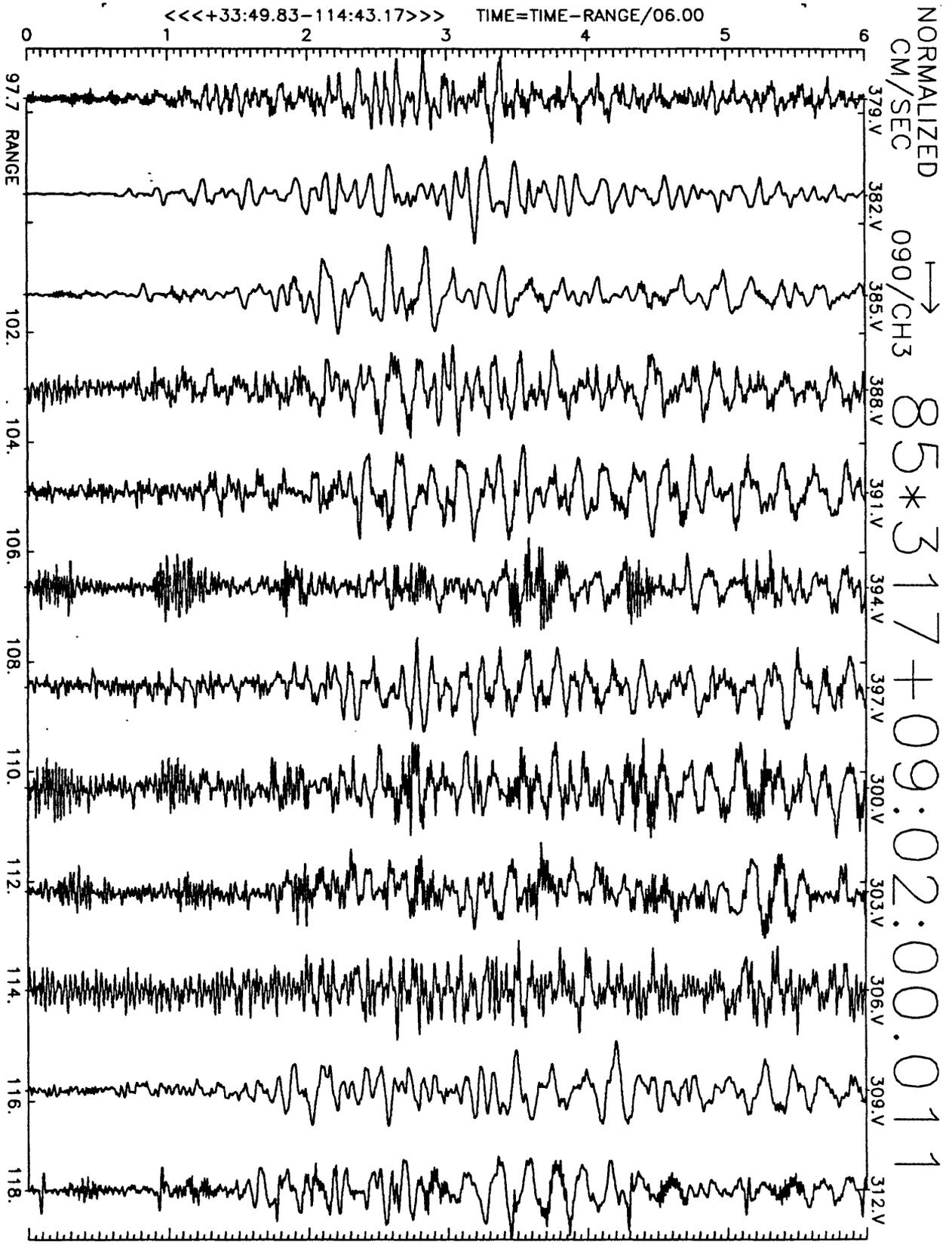
Figure A28(c), shot point 1: 6 second velocity record. Positive N115E motion is to right. Abscissa is distance to shot point. Top of trace is labeled with station number. Times are reduced by 6 km/sec. Shot time is indicated.
