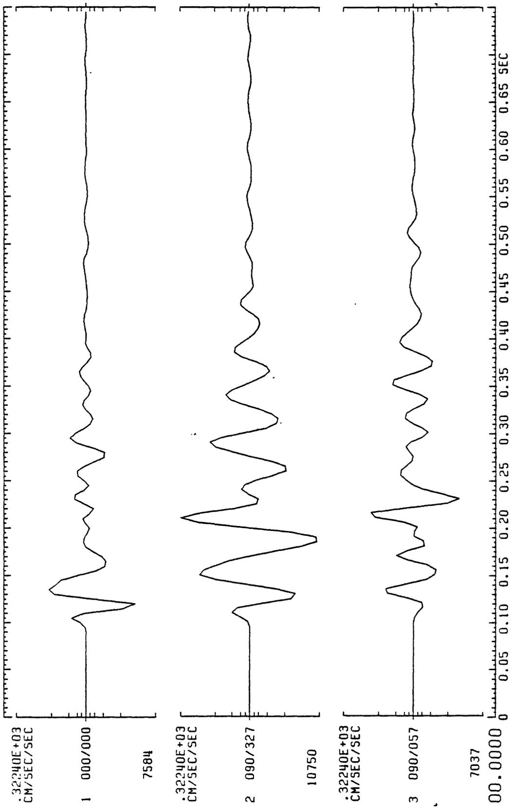
Figure B2(b), shot point 9': Three component accelerometer for station 166. Lower traces show horizontal motion. Azimuths are indicated immediately to the left of the traces. Start time is arbitrary.
