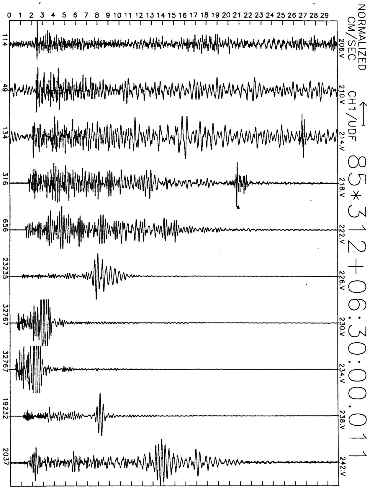
Figure A16(g), shot point 3': 30 second vertical velocity record. Abscissa is labeled with maximum counts in record (multiply by  $\frac{10}{2^{24}-2^8} \approx 6 \times 10^{-7}$  to get cm/sec). Times are unreduced beginning at time indicated.
