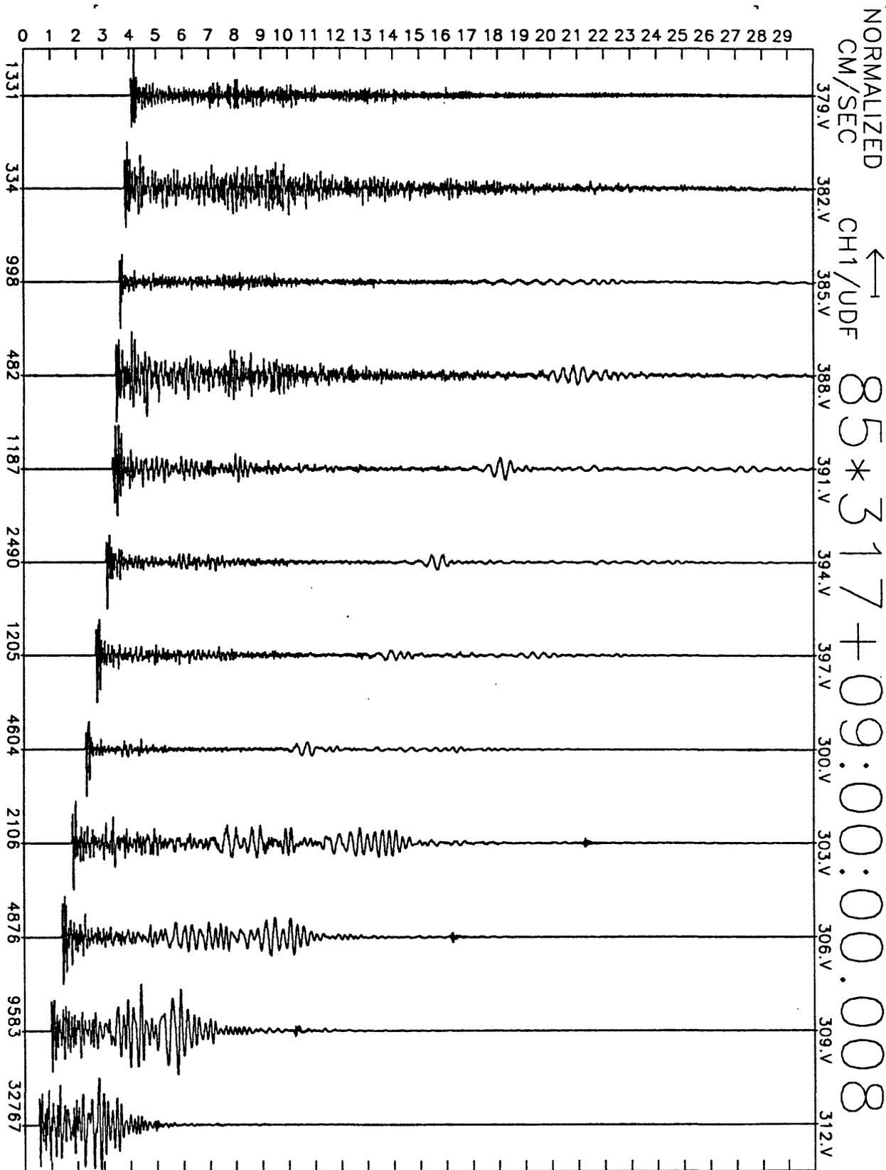
Figure A27(d), shot point 7: 30 second vertical velocity record. Abscissa is labeled with maximum counts in record (multiply by  $\frac{10}{2^{24}-2^8} \approx 6 \times 10^{-7}$  to get cm/sec). Times are unreduced beginning at time indicated.
