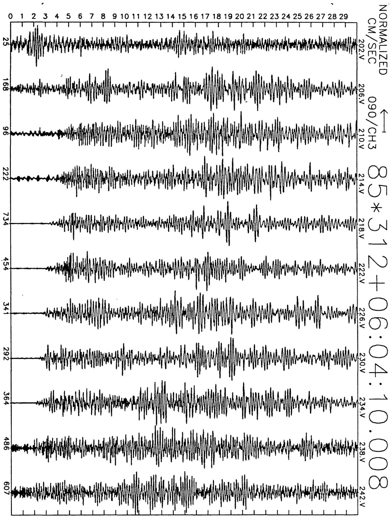
Figure A13(f), shot point 14: 30 second N110E velocity record. Abscissa is labeled with maximum counts in record (multiply by  $\frac{10}{2^{24}-2^0} \approx 6 \times 10^{-7}$  to get cm/sec). Times are unreduced beginning at time indicated.
