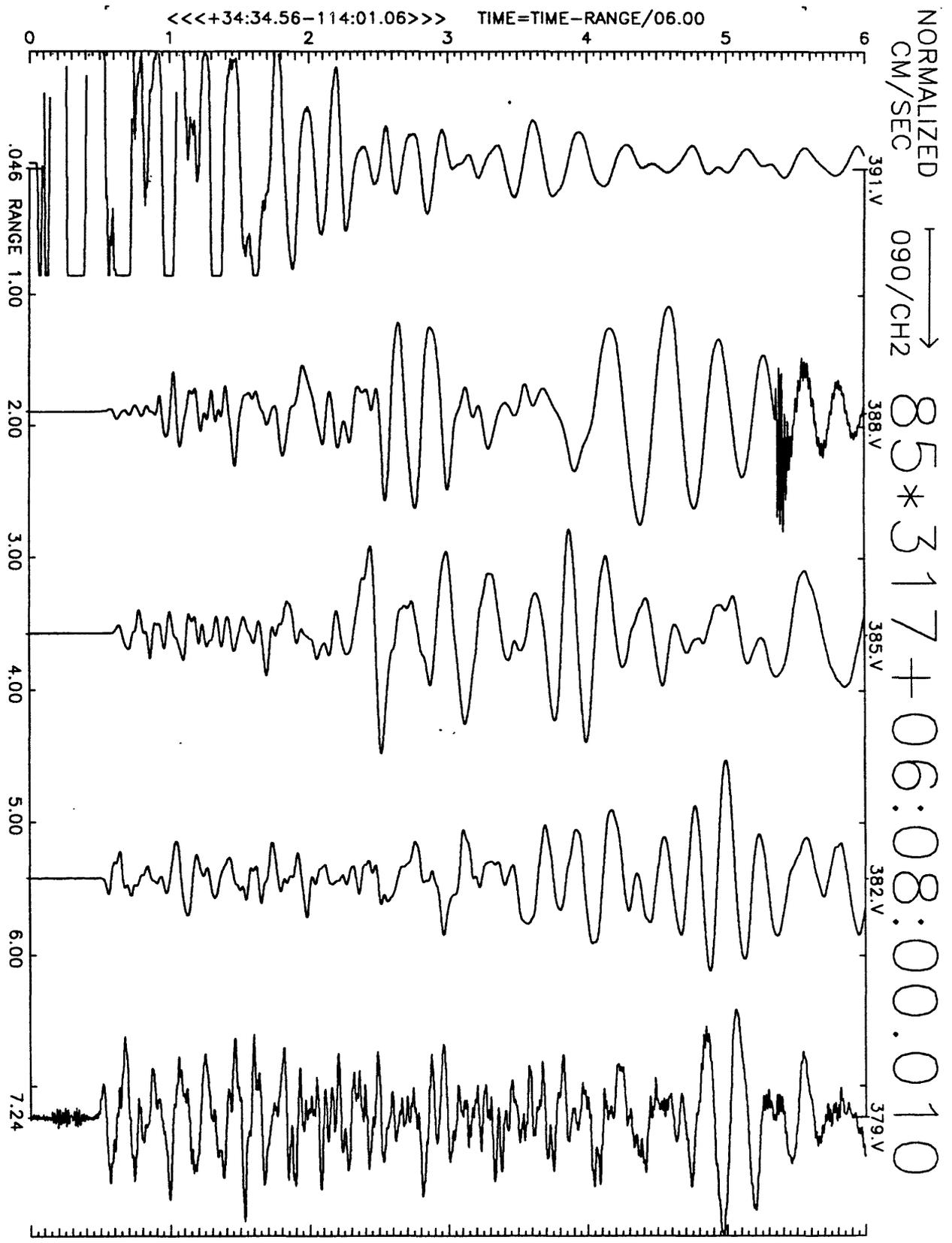
Figure A26(b), shot point 6X, SW stations: 6 second velocity record. Positive N25E motion is to right. Abscissa is distance to shot point. Top of trace is labeled with station number. Times are reduced by 6 km/sec. Shot time is indicated.
