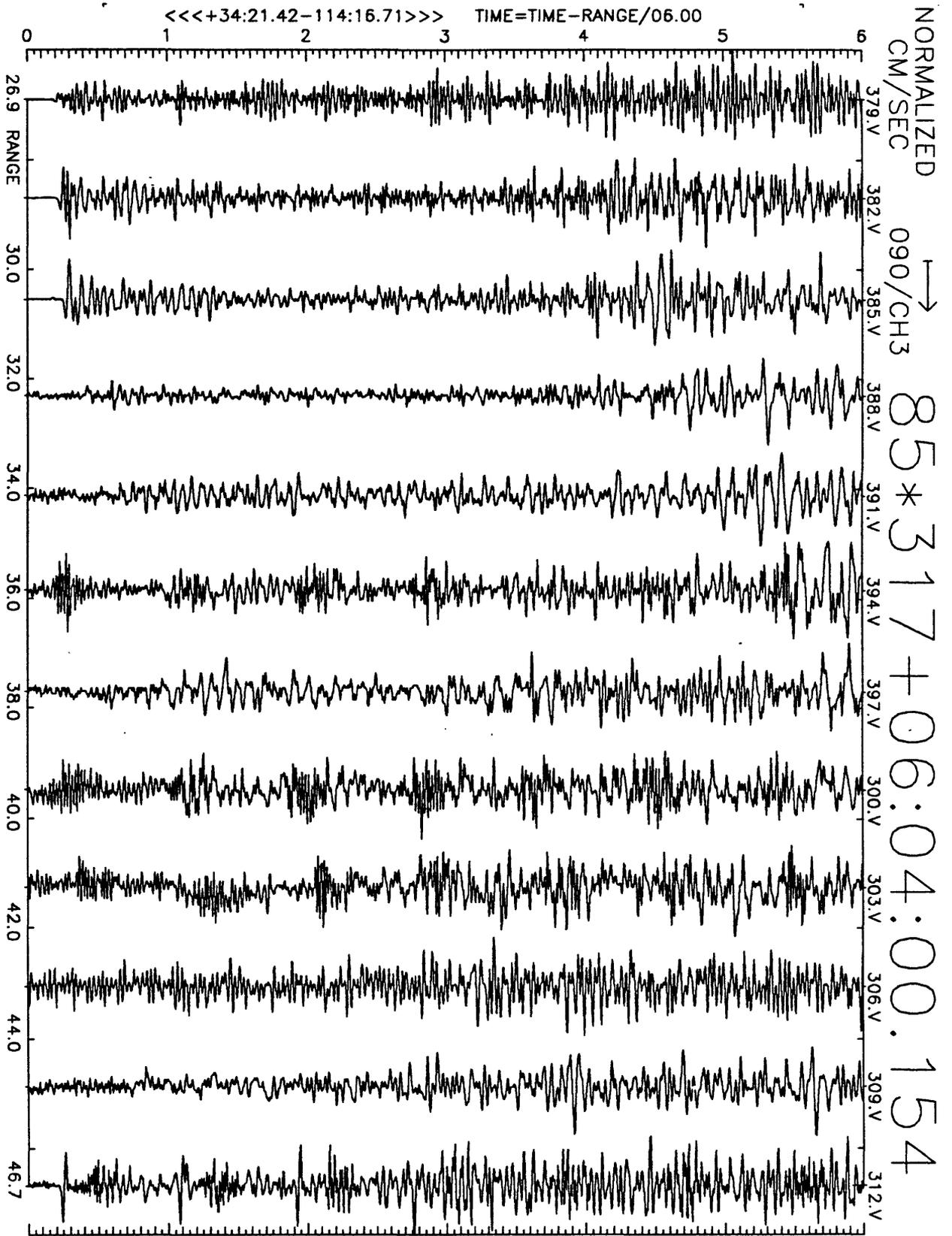
Figure A24(c), shot point 5: 6 second velocity record. Positive N115E motion is to right. Abscissa is distance to shot point. Top of trace is labeled with station number. Times are reduced by 6 km/sec. Shot time is indicated.
