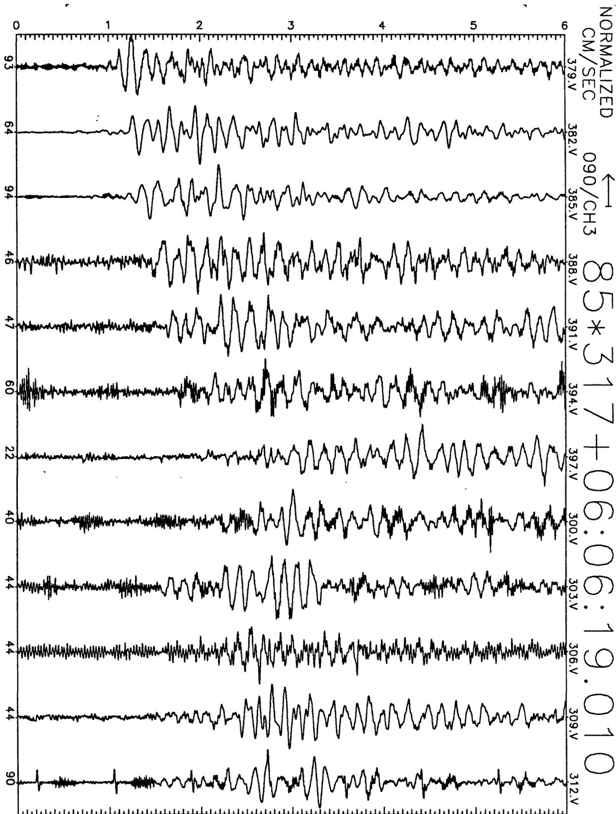
Figure A25(c), shot point 11 (fan shot): 6 second velocity record. Positive N115E-motion is to left. Abscissa is labeled with maximum counts in record. Distances are  $\sim 117.5 \pm 1.5 \text{ km}$ . Times are unreduced beginning at shot time + 19 seconds.
