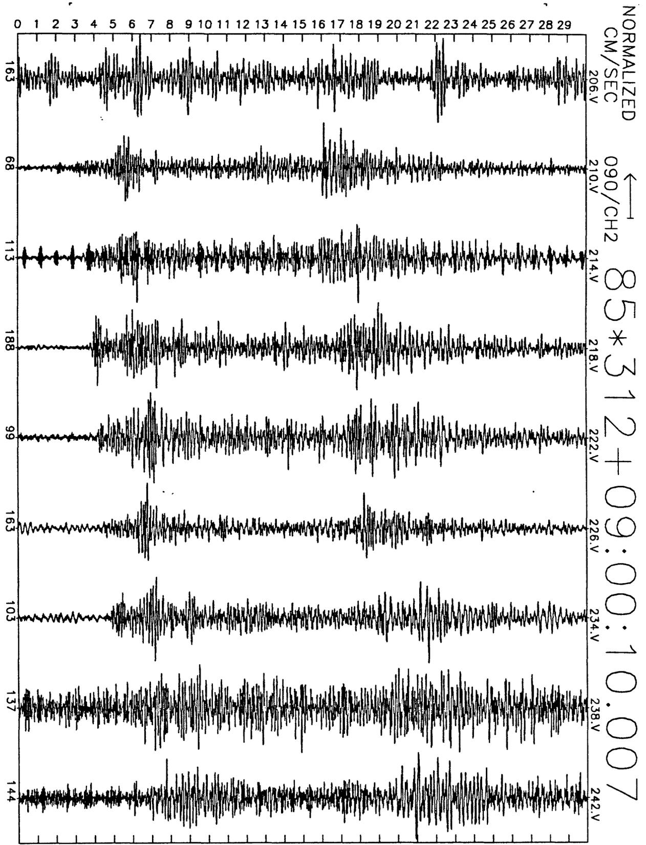
Figure A18(e), shot point 7: 30 second N20E velocity record. Abscissa is labeled with maximum counts in record (multiply by  $\frac{10}{2^{24}-2^8} \approx 6 \times 10^{-7}$  to get cm/sec). Times are unreduced beginning at time indicated.
