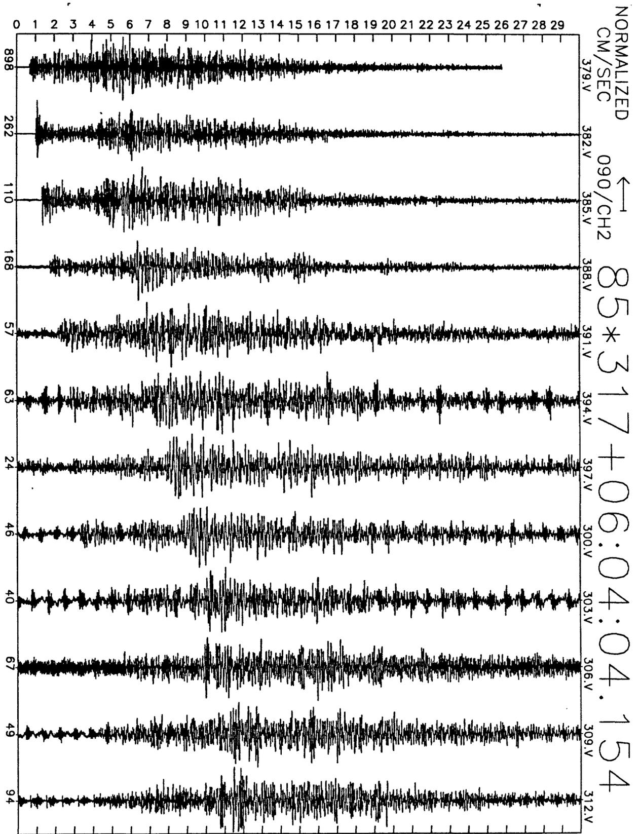
Figure A24(e), shot point 5: 30 second N25E velocity record. Abscissa is labeled with maximum counts in record (multiply by  $\frac{10}{2^{24}-2^8} \approx 6 \times 10^{-7}$  to get cm/sec). Times are unreduced beginning at time indicated.
