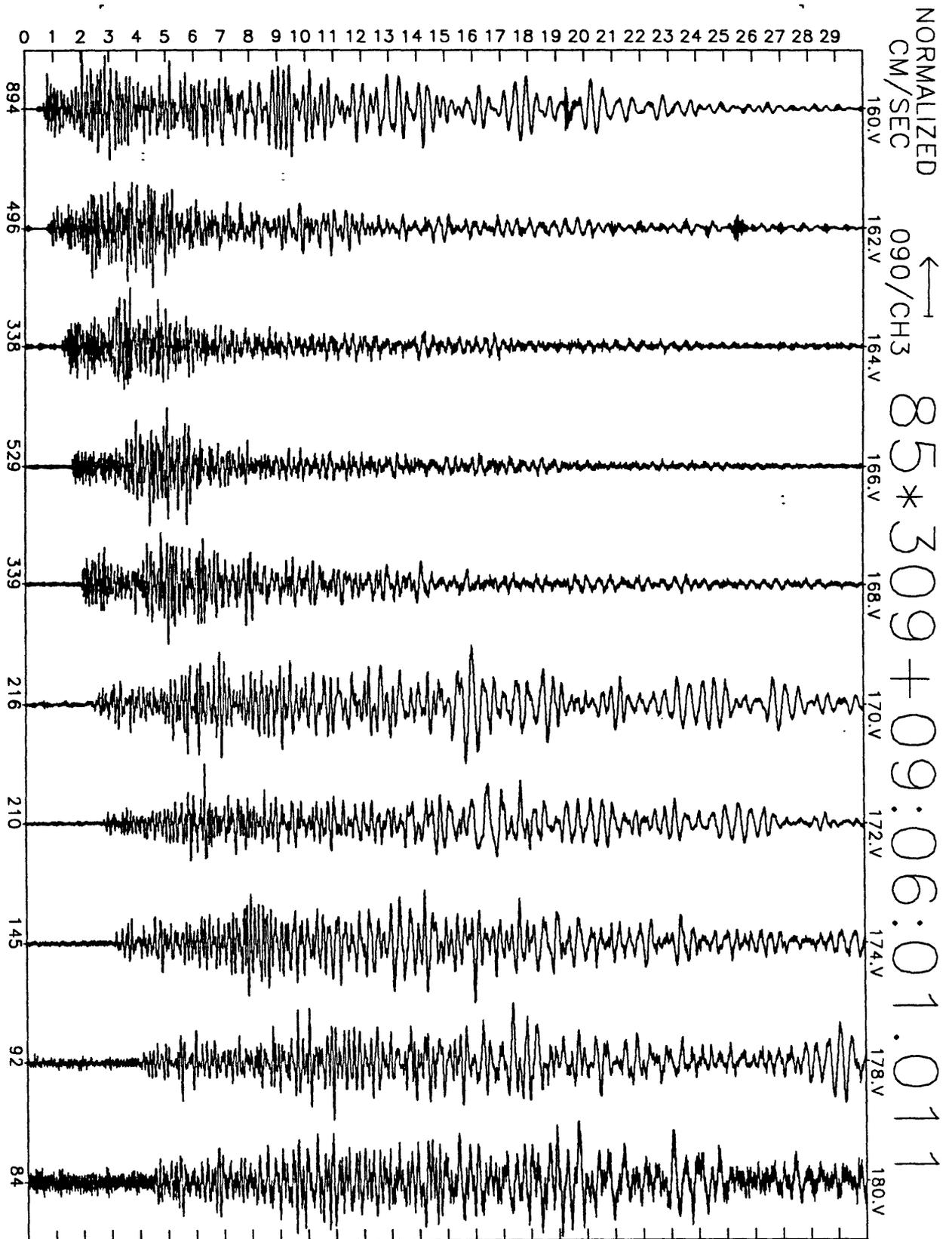
Figure A9(f), shot point 9X: 30 second N57E velocity record. Abscissa is labeled with maximum counts in record (multiply by  $\frac{10}{2^{24}-2^8} \approx 6 \times 10^{-7}$  to get cm/sec). Times are unreduced beginning at time indicated.
