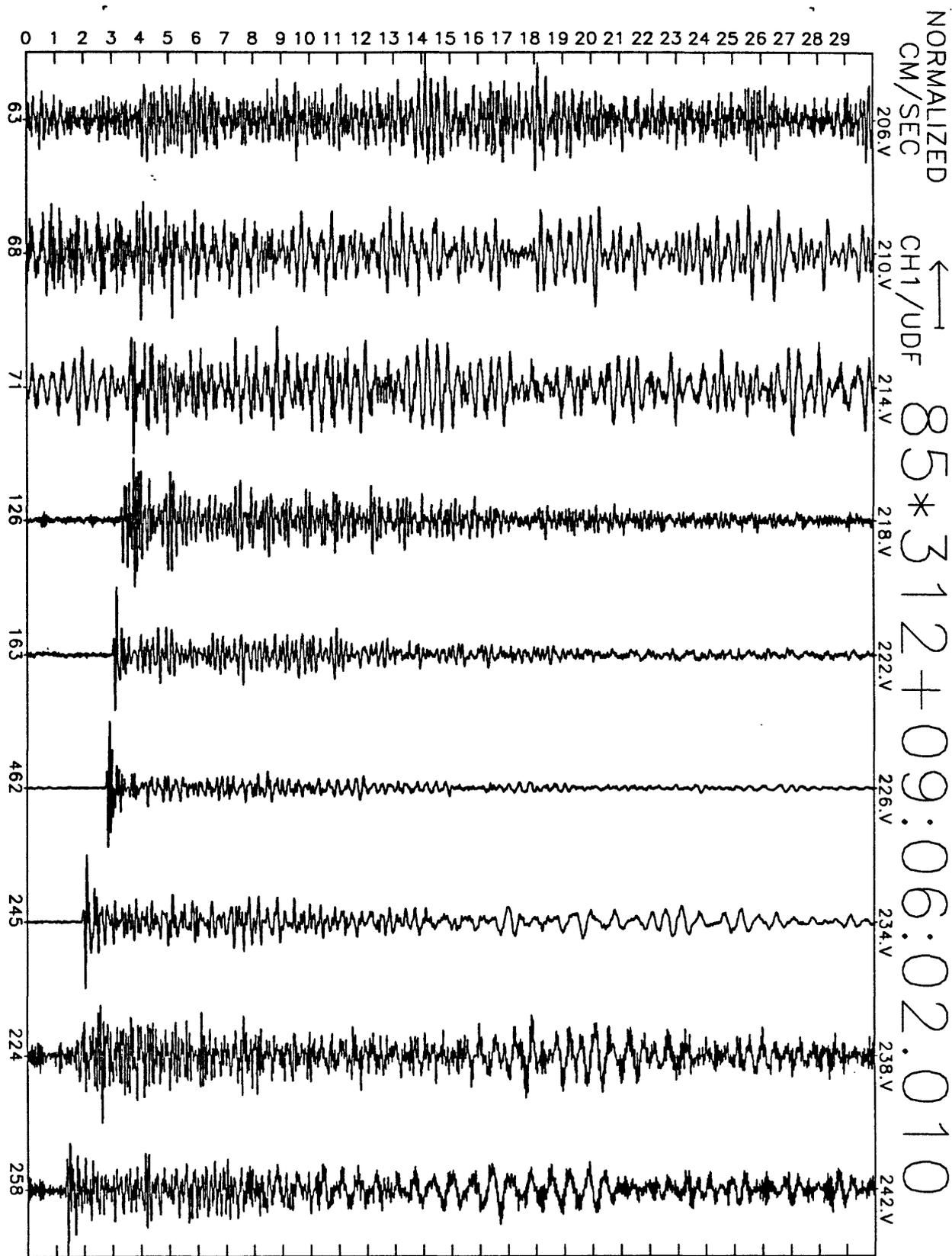
Figure A21(d), shot point 1X: 30 second vertical velocity record. Abscissa is labeled with maximum counts in record (multiply by  $\frac{10}{2^{24}-2^8} \approx 6 \times 10^{-7}$  to get cm/sec). Times are unreduced beginning at time indicated.
