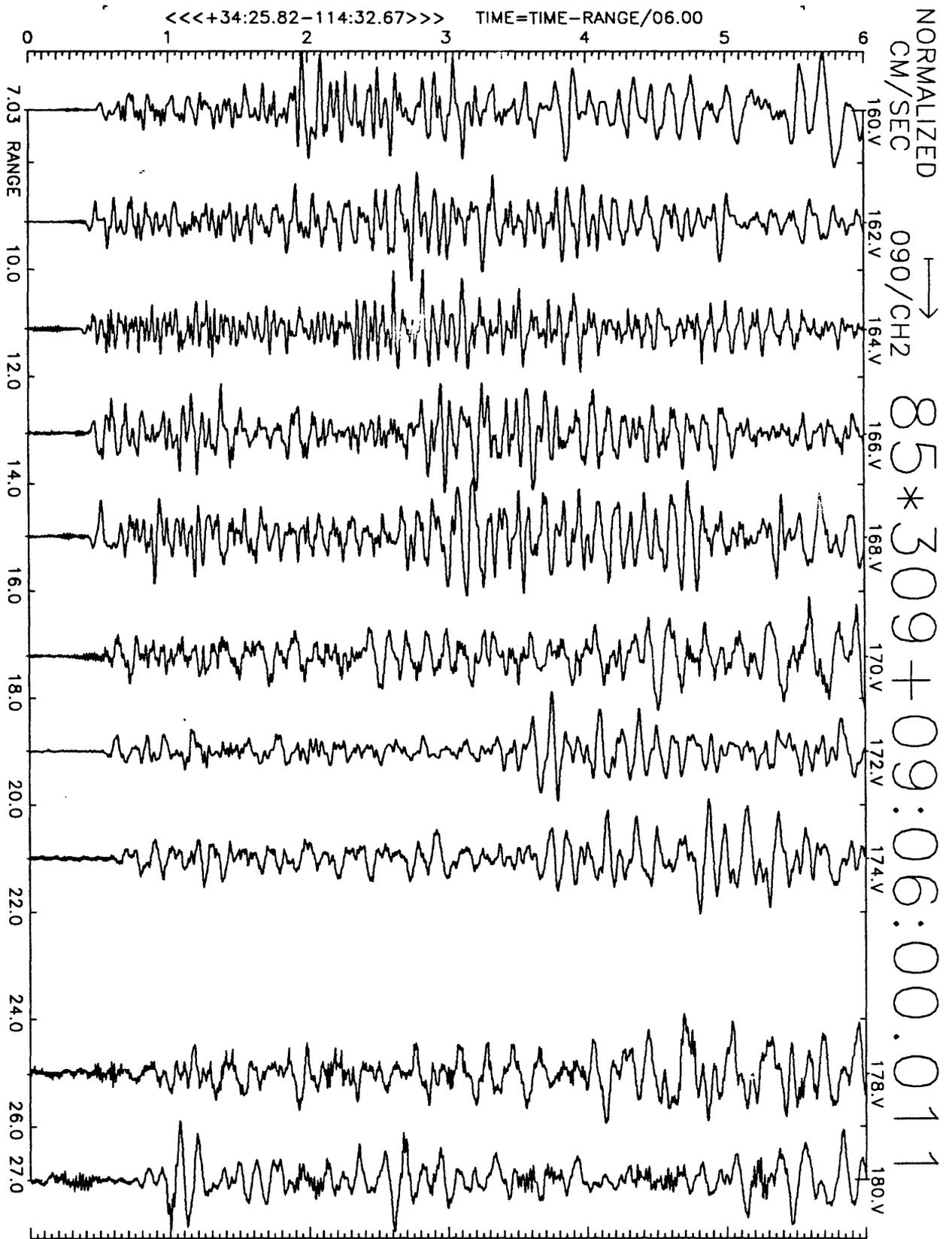
Figure A9(b), shot point 9X: 6 second velocity record. Positive N33W motion is to right. Abscissa is distance to shot point. Top of trace is labeled with station number. Times are reduced by 6 km/sec. Shot time is indicated.
