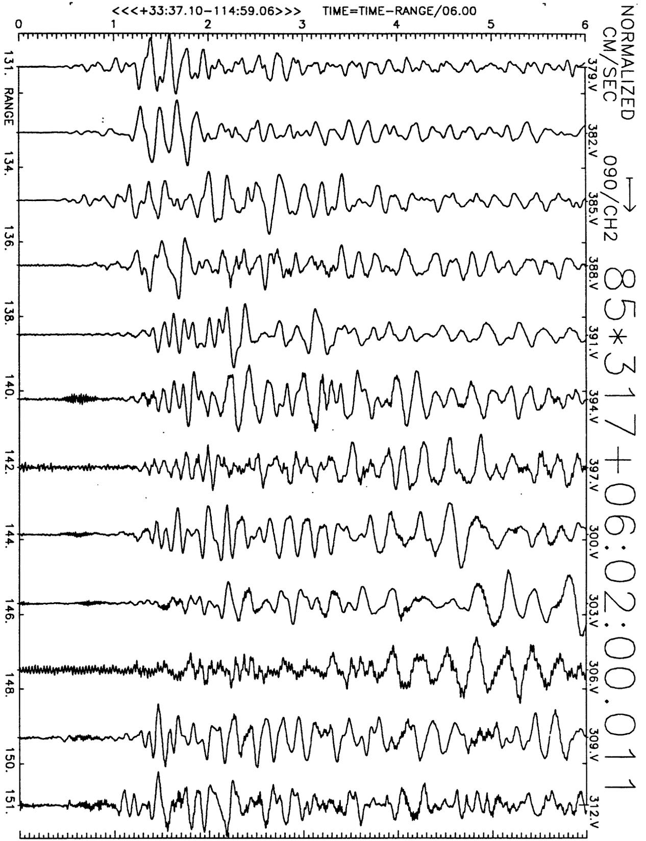
Figure A23(b), shot point 14: 6 second velocity record. Positive N25E motion is to right. Abscissa is distance to shot point. Top of trace is labeled with station number. Times are reduced by 6 km/sec. Shot time is indicated.
