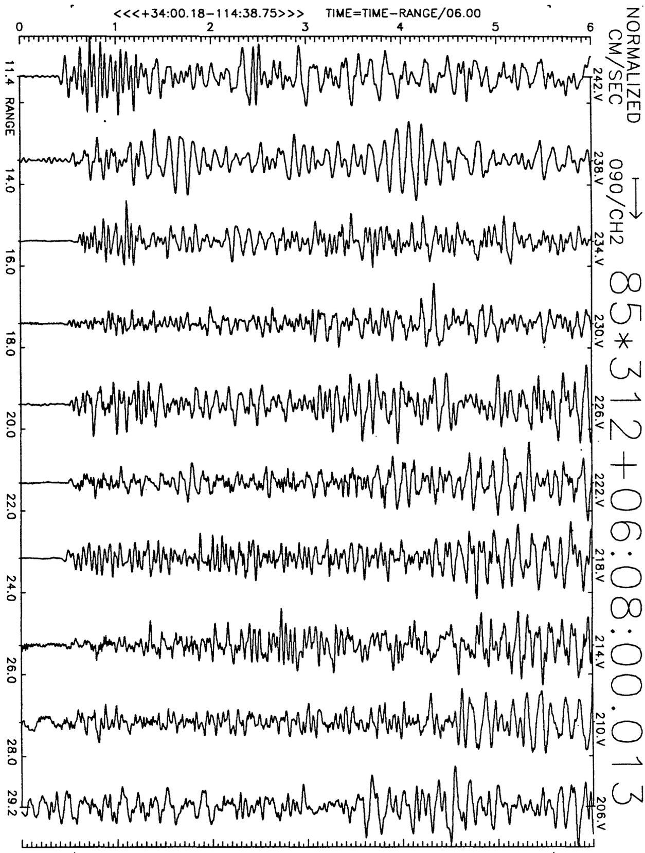
Figure A15(b), shot point 2: 6 second velocity record. Positive N20E motion is to right. Abscissa is distance to shot point. Top of trace is labeled with station number. Times are reduced by 6 km/sec. Shot time is indicated.
