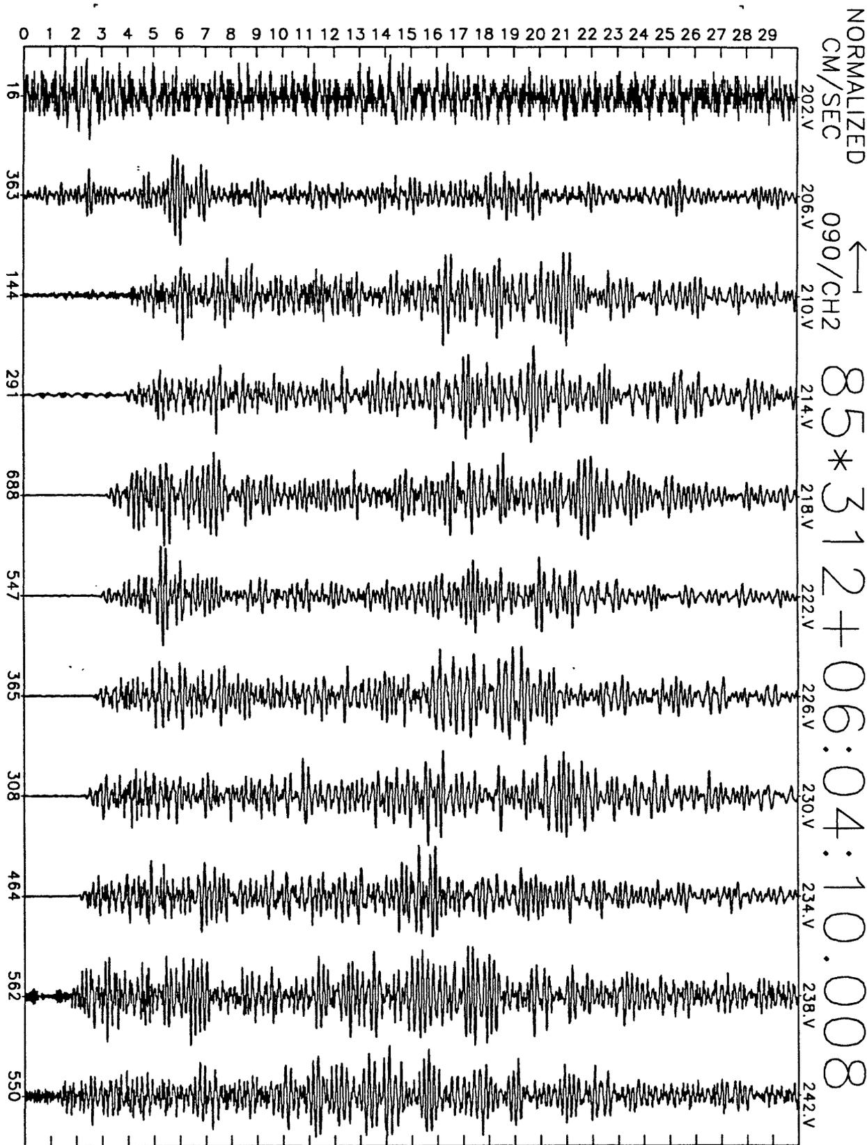
Figure A13(e), shot point 14: 30 second N20E velocity record. Abscissa is labeled with maximum counts in record (multiply by  $\frac{10}{2^{24}-2^8} \approx 6 \times 10^{-7}$  to get cm/sec). Times are unreduced beginning at time indicated.
