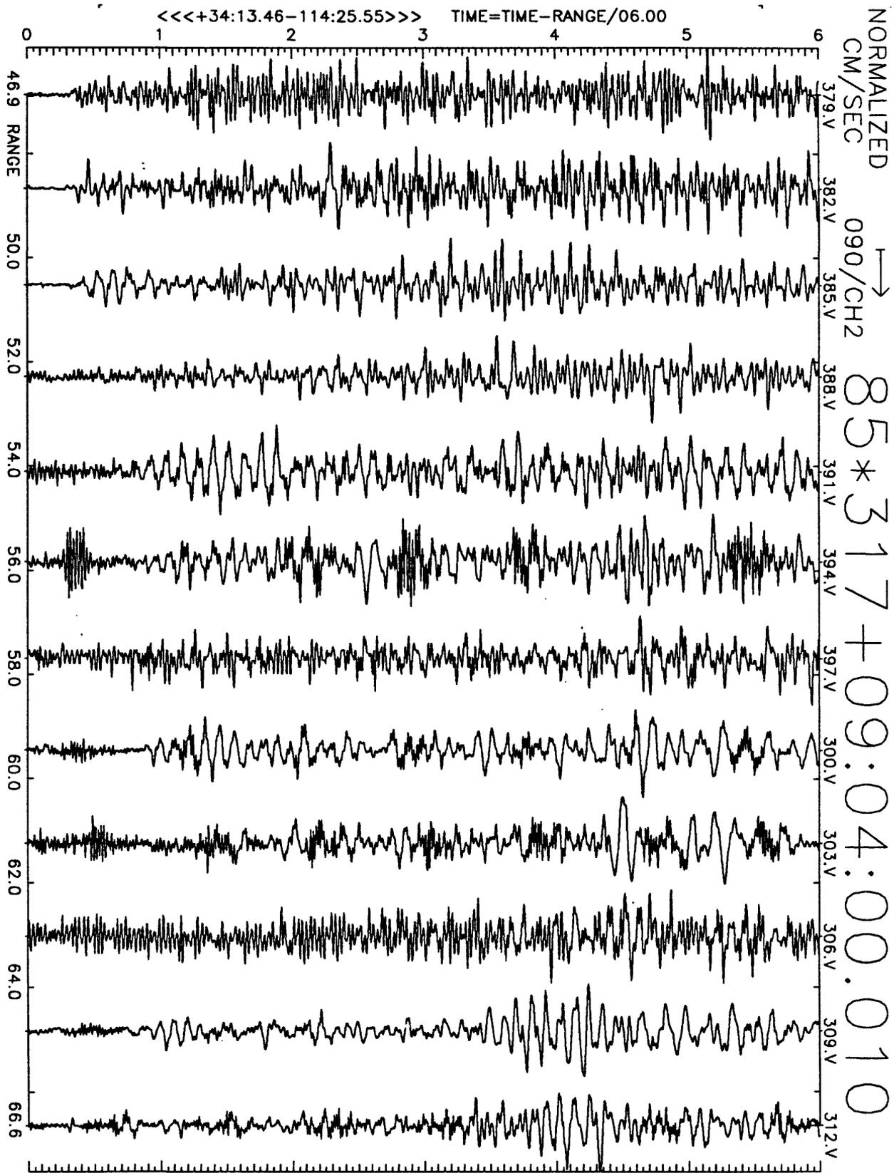
Figure A29(b), shot point 4B: 6 second velocity record. Positive N25E motion is to right. Abscissa is distance to shot point. Top of trace is labeled with station number. Times are reduced by 6 km/sec. Shot time is indicated.
