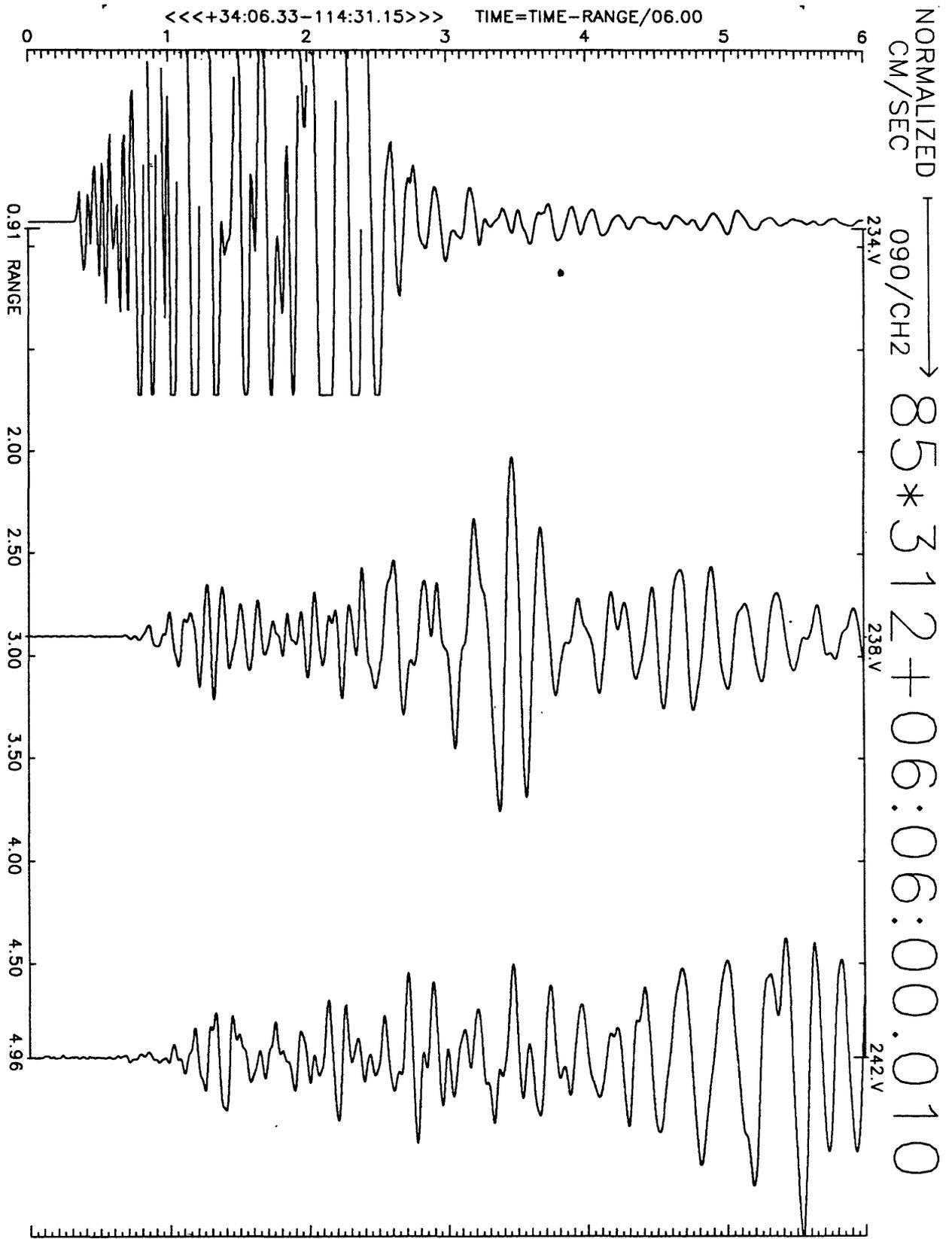
Figure A14(b), shot point 3, SW stations: 6 second velocity record. Positive N20E motion is to right. Abscissa is distance to shot point. Top of trace is labeled with station number. Times are reduced by 6 km/sec. Shot time is indicated.
