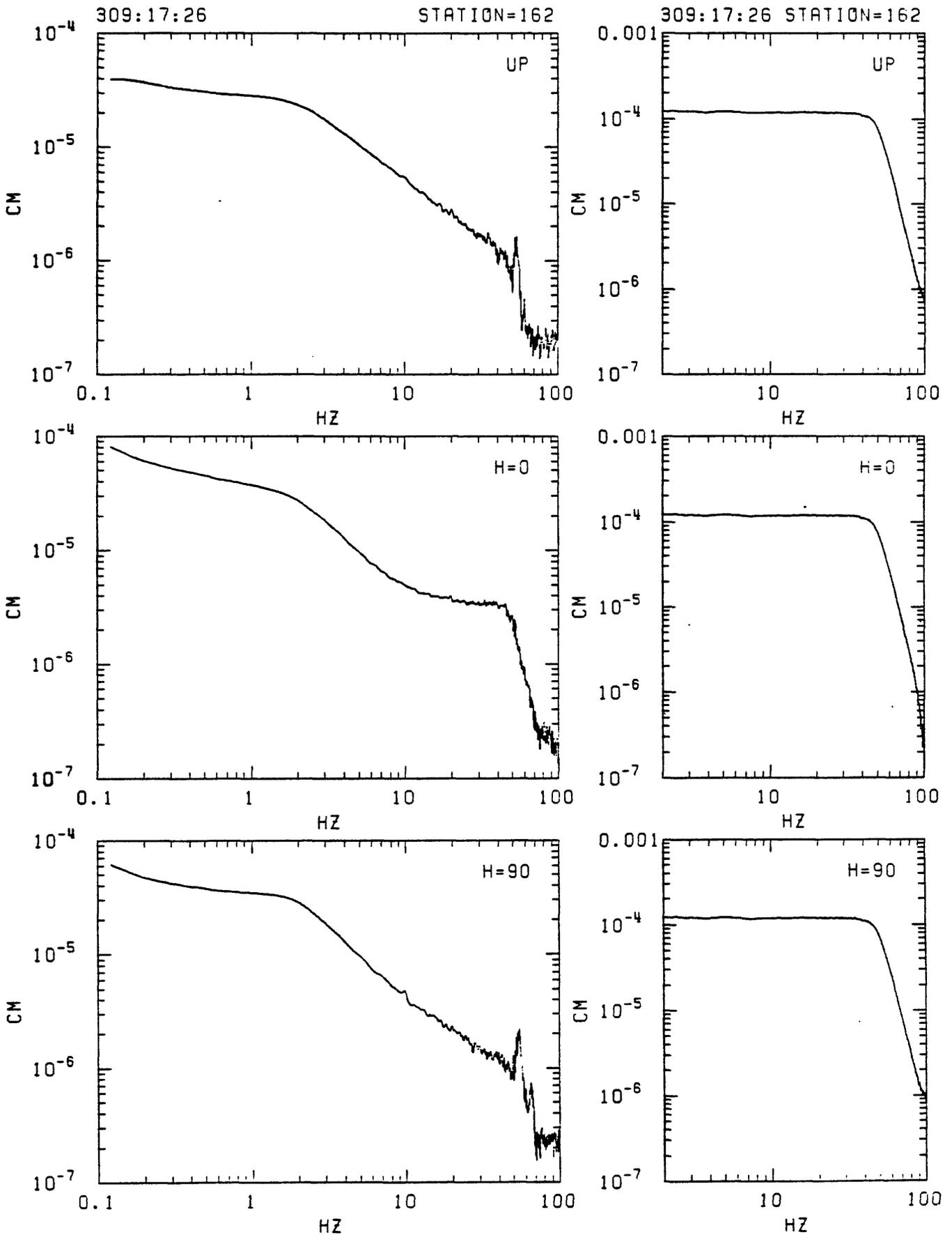
Figure C2. Station 162 in-situ velocity calibration spectra. Left: response to step in acceleration (seismometer mass released from rest at offset position). Right: response to delta function in velocity (voltage impulse applied to recorder input). From top: vertical, N33W and N57E.
