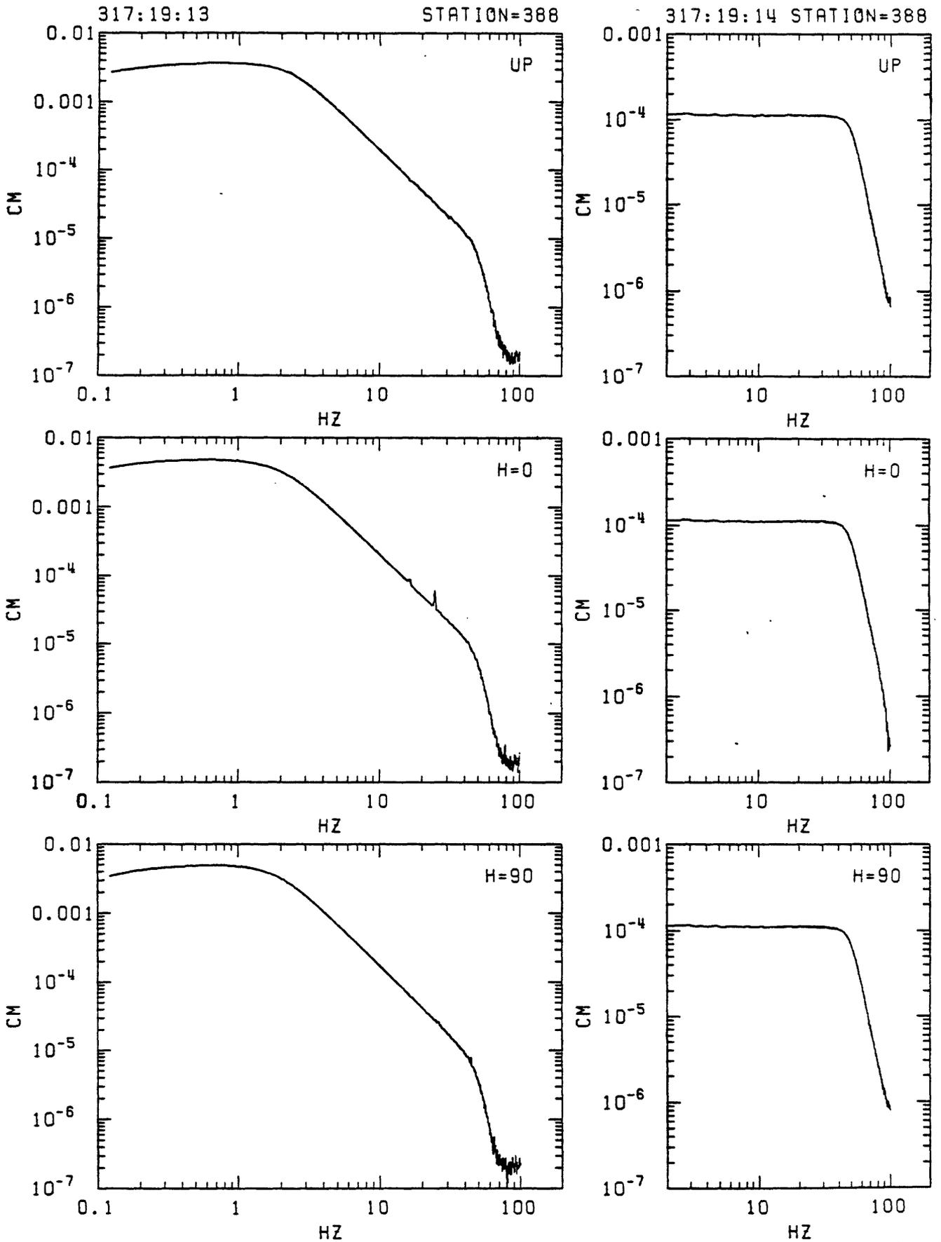
Figure C23. Station 388 in-situ velocity calibration spectra. Left: response to step in acceleration (seismometer mass released from rest at offset position). Right: response to delta function in velocity (voltage impulse applied to recorder input). From top: vertical, N25E and N115E.
