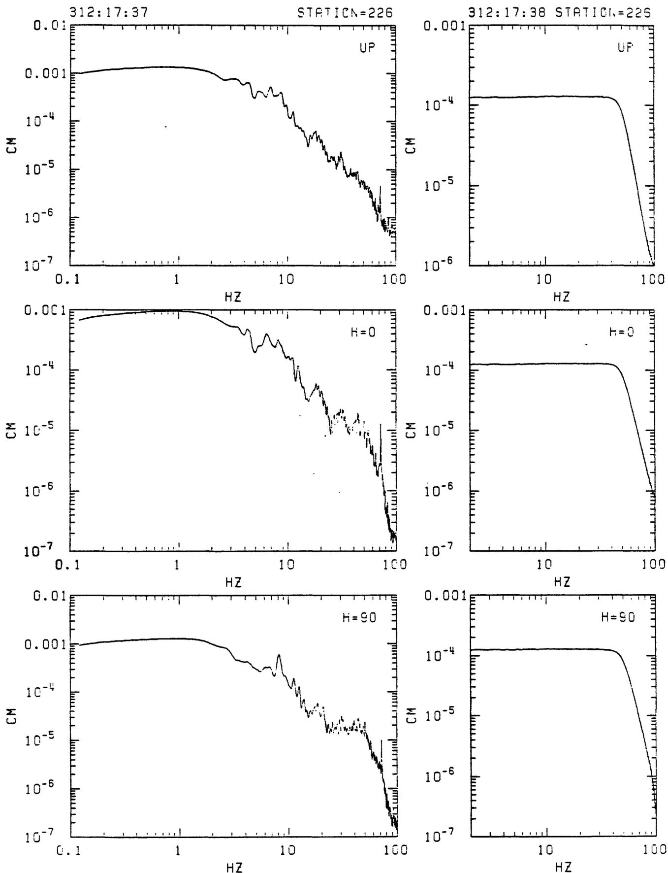
Figure C17. Station 226 in-situ velocity calibration spectra. Left: response to step in acceleration (seismometer mass released from rest at offset position). Right: response to delta function in velocity (voltage impulse applied to recorder input). From top: vertical, N20E and N110E.
