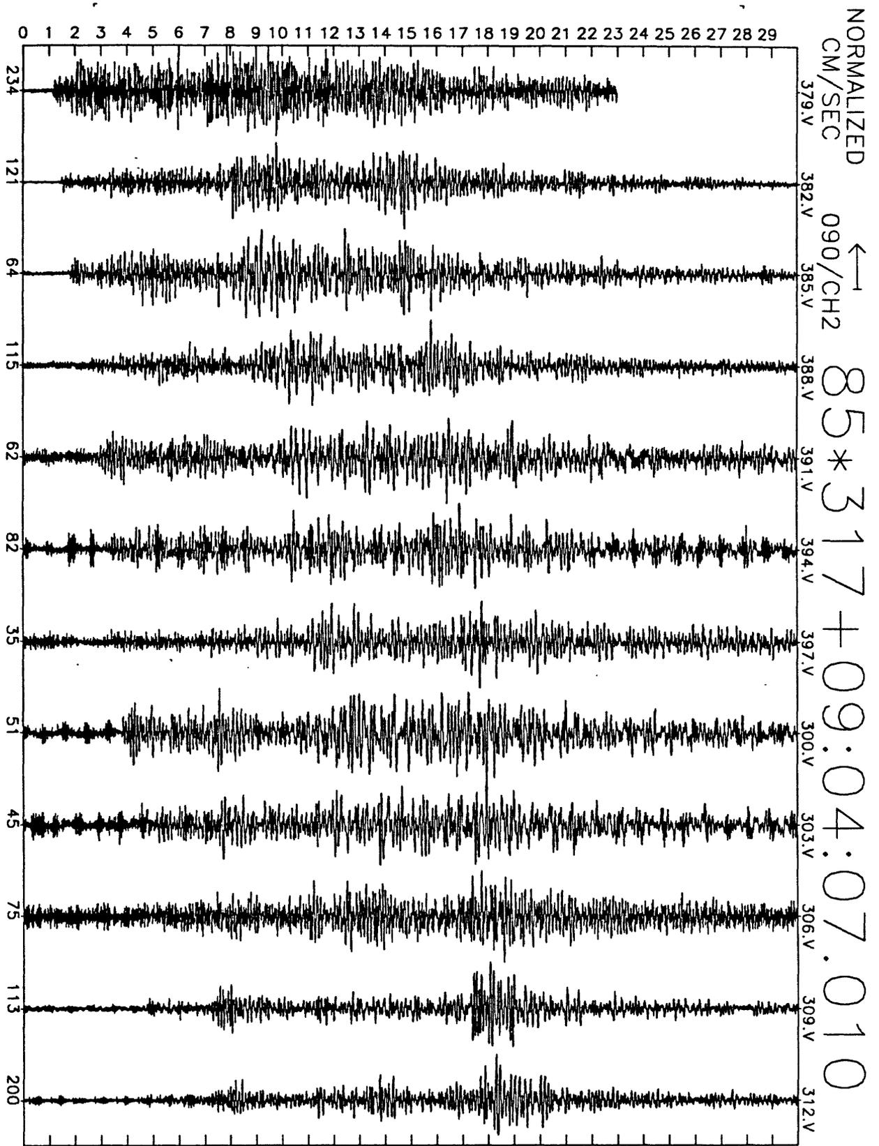
Figure A29(e), shot point 4B: 30 second N25E velocity record. Abscissa is labeled with maximum counts in record (multiply by  $\frac{10}{224-2^8} \approx 6 \times 10^{-7}$  to get cm/sec). Times are unreduced beginning at time indicated.
