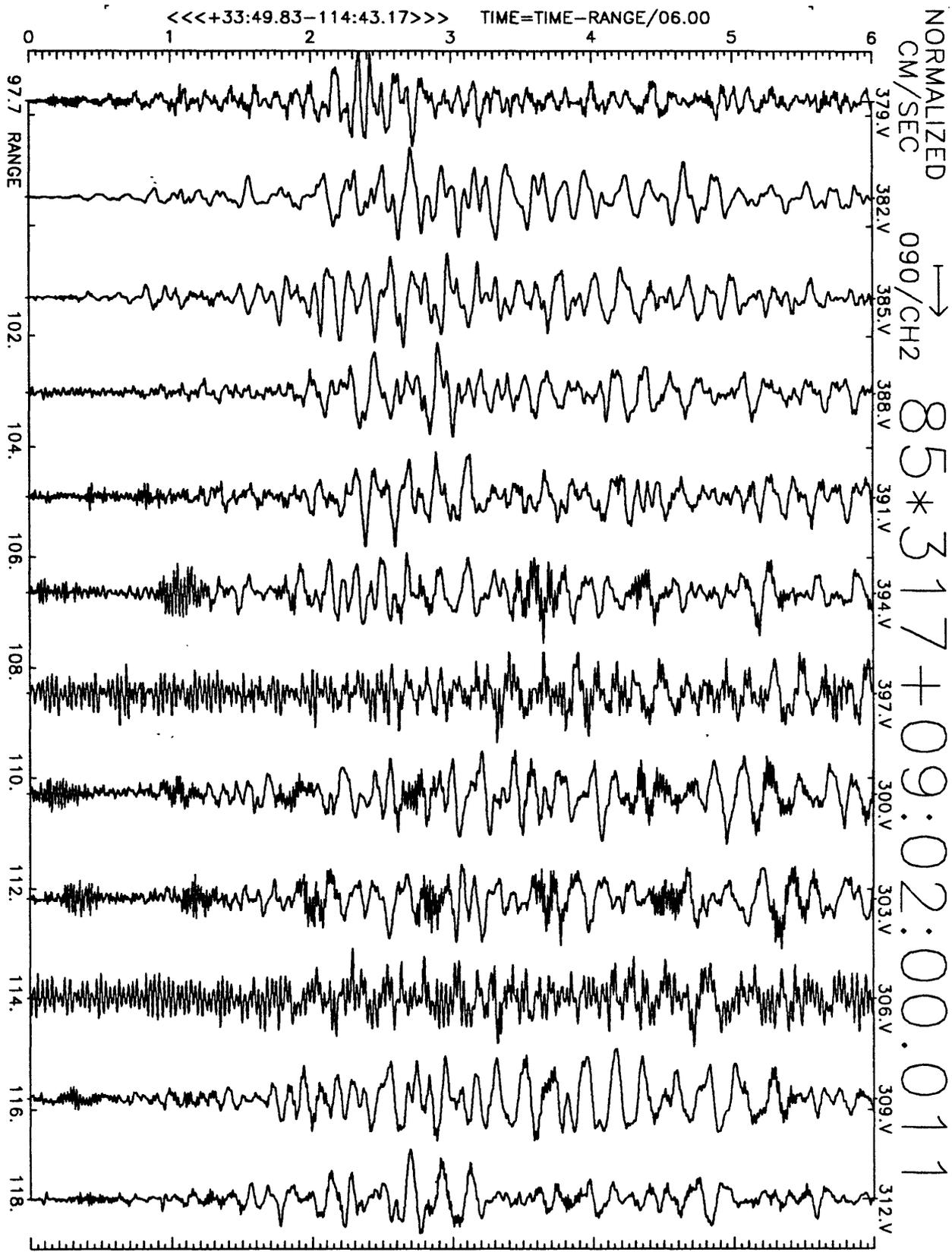
Figure A28(b), shot point 1: 6 second velocity record. Positive N25E motion is to right. Abscissa is distance to shot point. Top of trace is labeled with station number. Times are reduced by 6 km/sec. Shot time is indicated.
