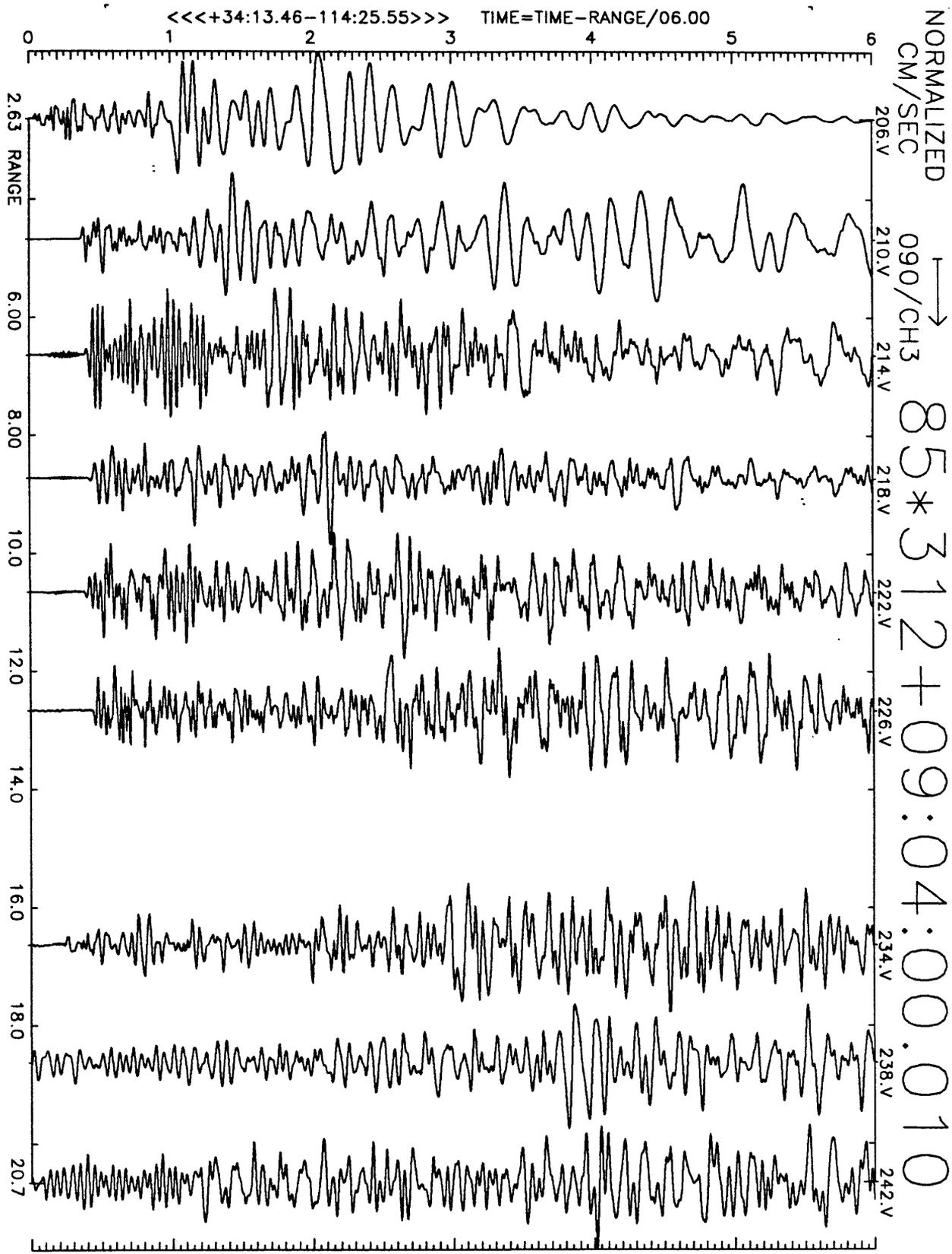
Figure A20(c), shot point 4B: 6 second velocity record. Positive N110E motion is to right. Abscissa is distance to shot point. Top of trace is labeled with station number. Times are reduced by 6 km/sec. Shot time is indicated.
