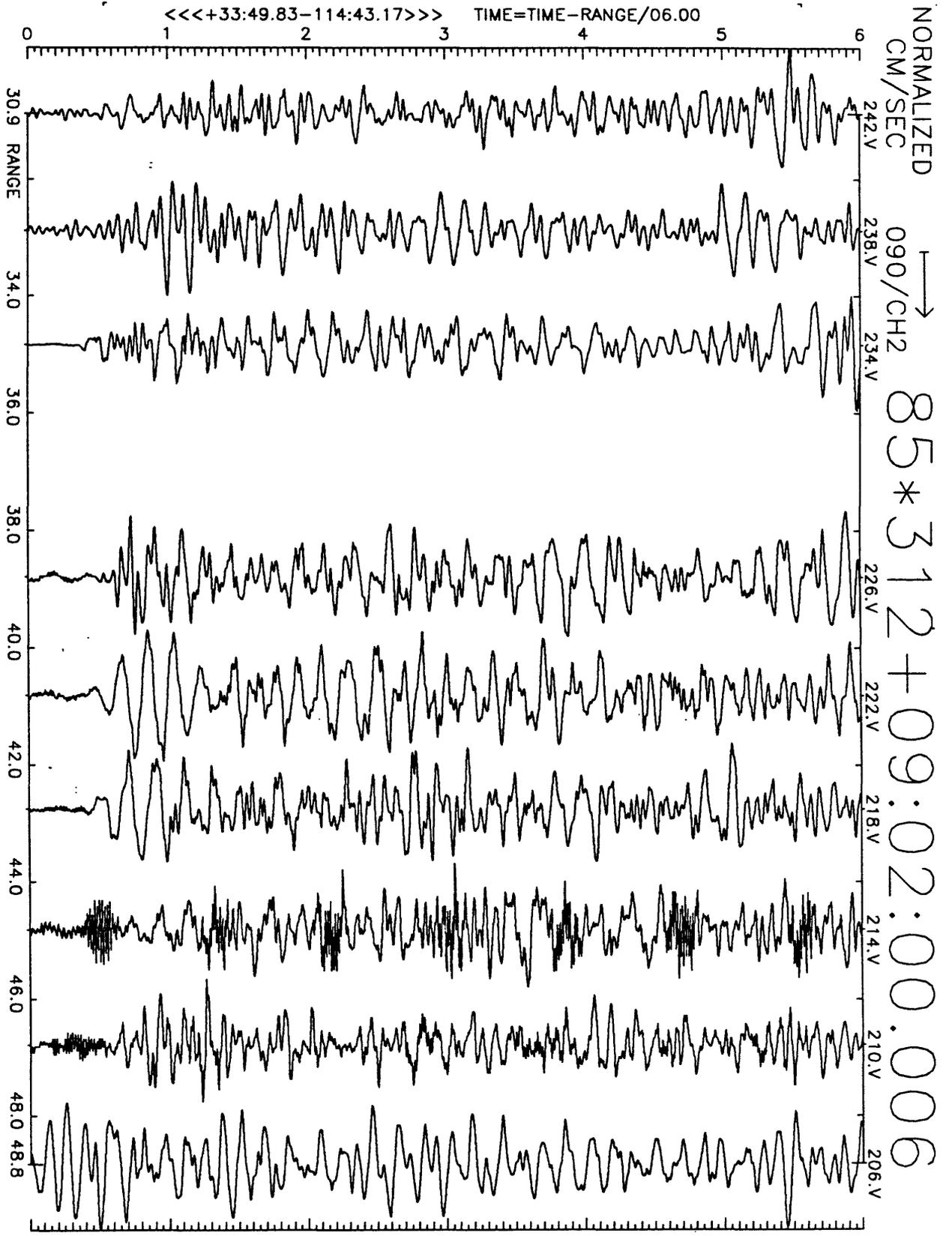
Figure A19(b), shot point 1: 6 second velocity record. Positive N20E motion is to right. Abscissa is distance to shot point. Top of trace is labeled with station number. Times are reduced by 6 km/sec. Shot time is indicated.
