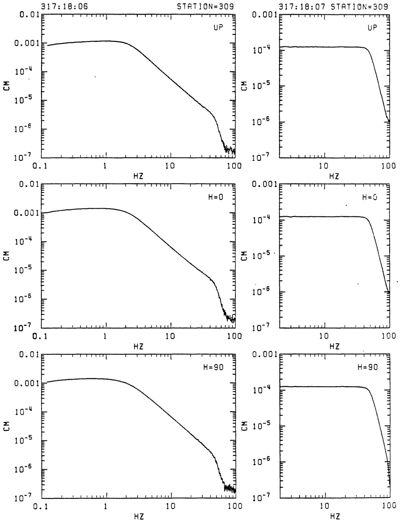
Figure C29. Station 309 in-situ velocity calibration spectra. Left: response to step in acceleration (seismometer mass released from rest at offset position). Right: response to delta function in velocity (voltage impulse applied to recorder input). From top: vertical, N25E and N115E.
