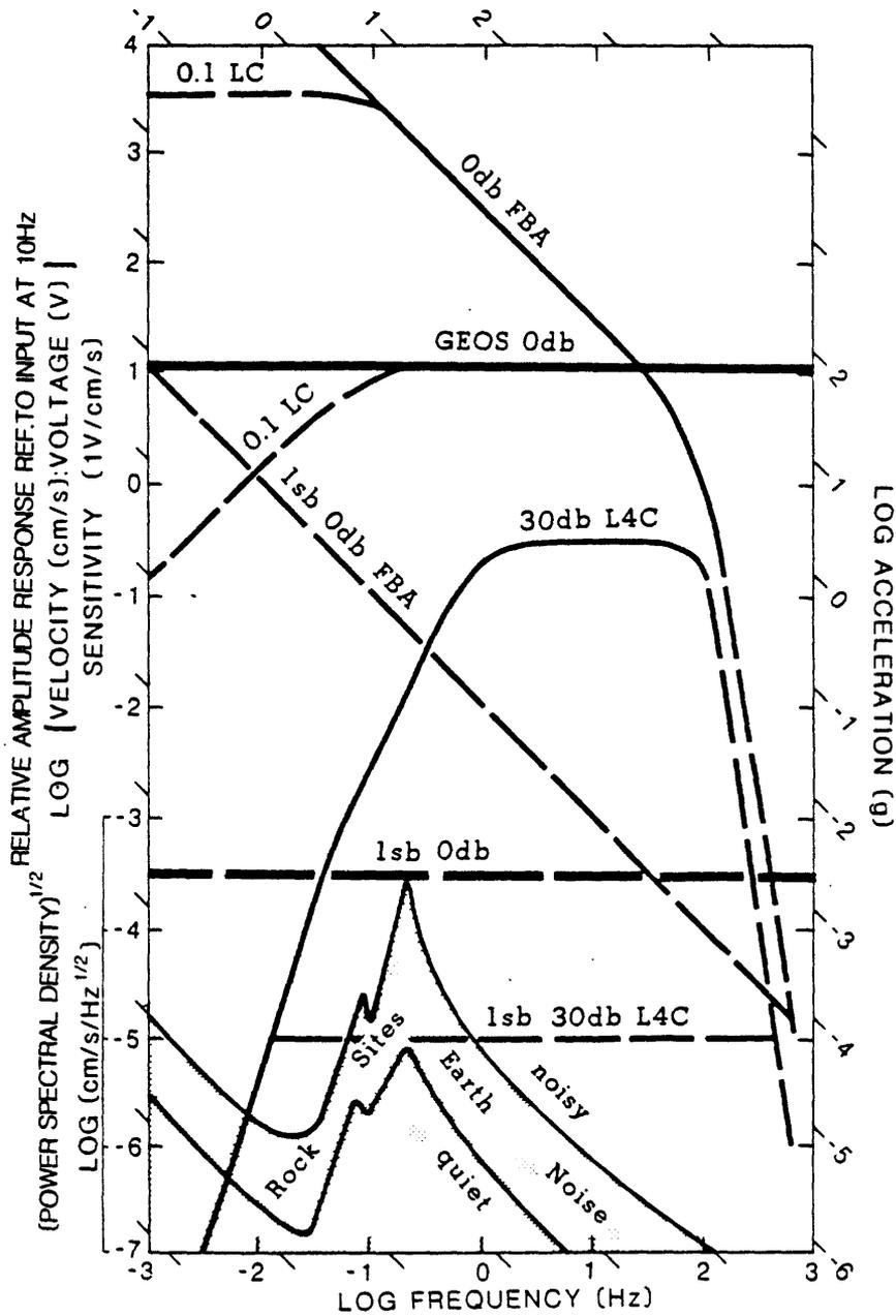
Figure 2. The unit-impulse response designed for the GEOS recorder, spectra for Earth noise (Aki and Richards, 1980), and complete system response with two types of sensors (force-balance accelerometer at 0 dB gain and L4-C velocity transducer at 30 dB gain). Two sets of sensors and linear dynamic range of 96 dB (16-bit) offers the capability to record without gain change 10 Hz signals on scale with amplitudes ranging from 20 angstroms in displacements to 2 g in acceleration.
