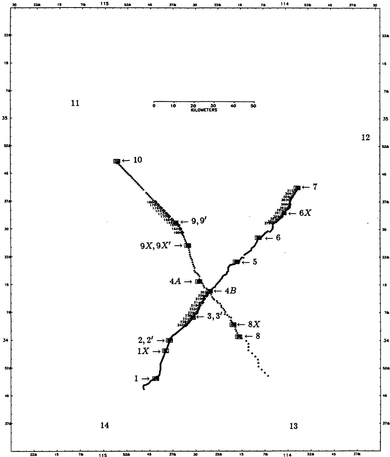
Figure 3: Map showing locations of three deployments of GEOS recorders (labeled by three digit station names) relative to cassette recorder deployments, and shots (labeled by shot point number).
