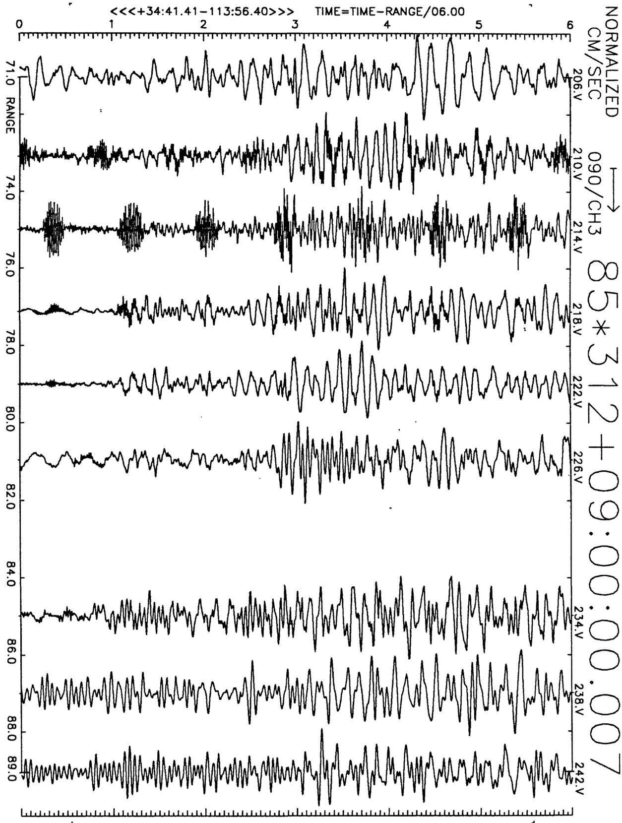
Figure A18(c), shot point 7: 6 second velocity record. Positive N110E motion is to right. Abscissa is distance to shot point. Top of trace is labeled with station number. Times are reduced by 6 km/sec. Shot time is indicated.
