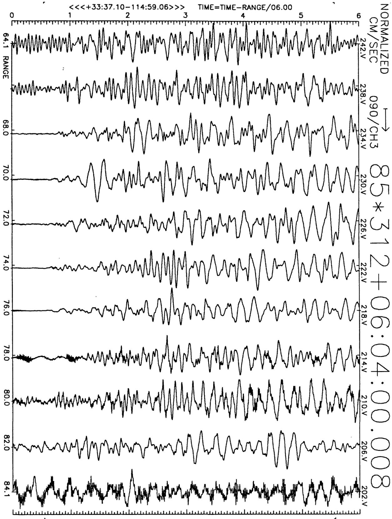
Figure A13(c), shot point 14: 6 second velocity record. Positive N110E motion is to right. Abscissa is distance to shot point. Top of trace is labeled with station number. Times are reduced by 6 km/sec. Shot time is indicated.
