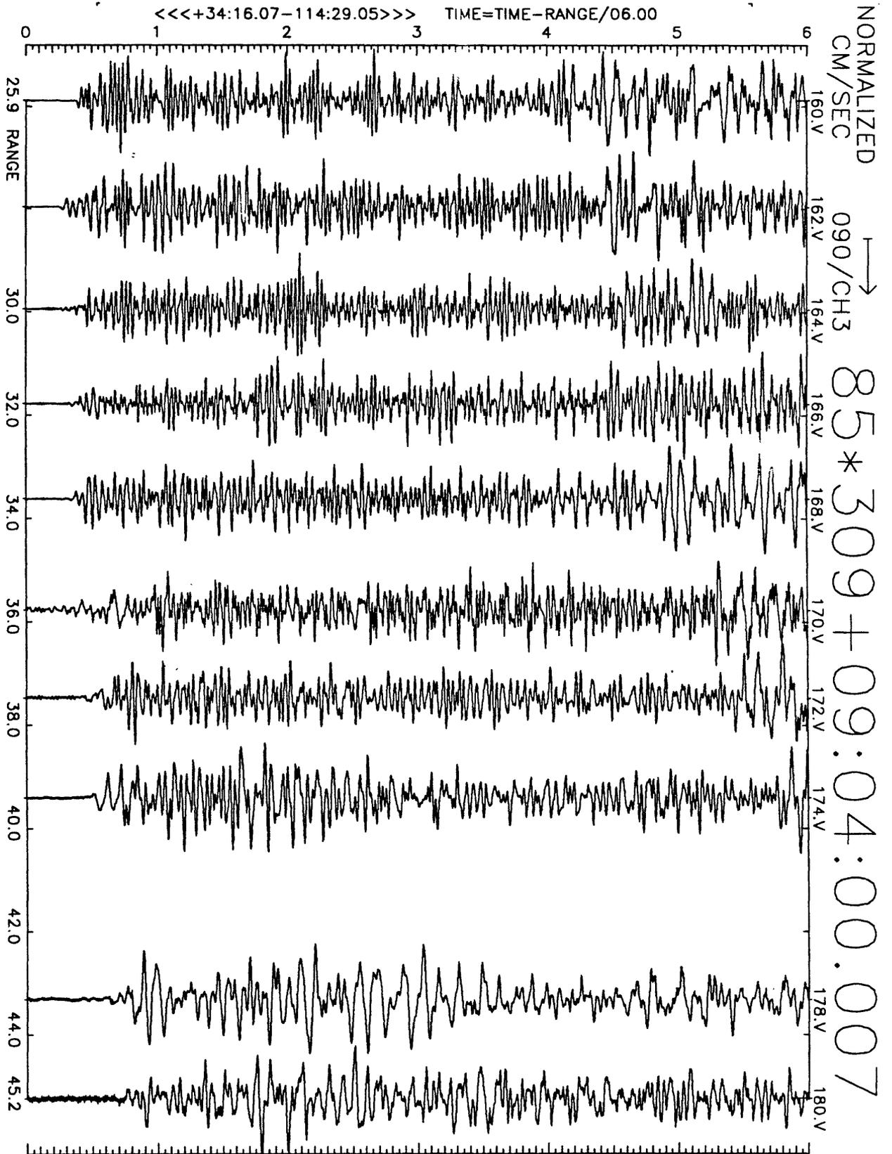
Figure A8(c), shot point 4A: 6 second velocity record. Positive N57E motion is to right. Abscissa is distance to shot point. Top of trace is labeled with station number. Times are reduced by 6 km/sec. Shot time is indicated.
