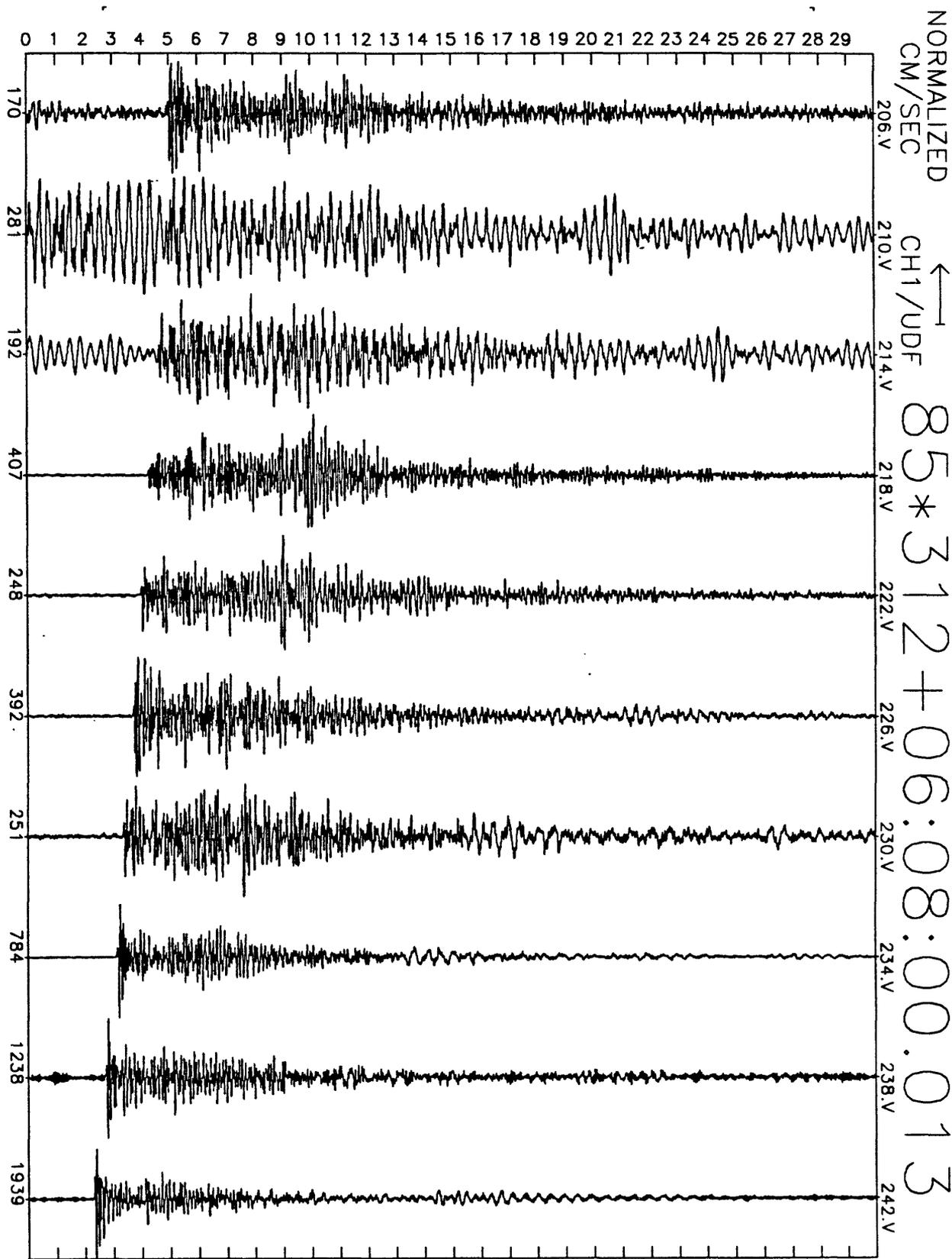
Figure A15(d), shot point 2: 30 second vertical velocity record. Abscissa is labeled with maximum counts in record (multiply by  $\frac{10}{2^{24}-2^8} \approx 6 \times 10^{-7}$  to get cm/sec). Times are unreduced beginning at time indicated.
