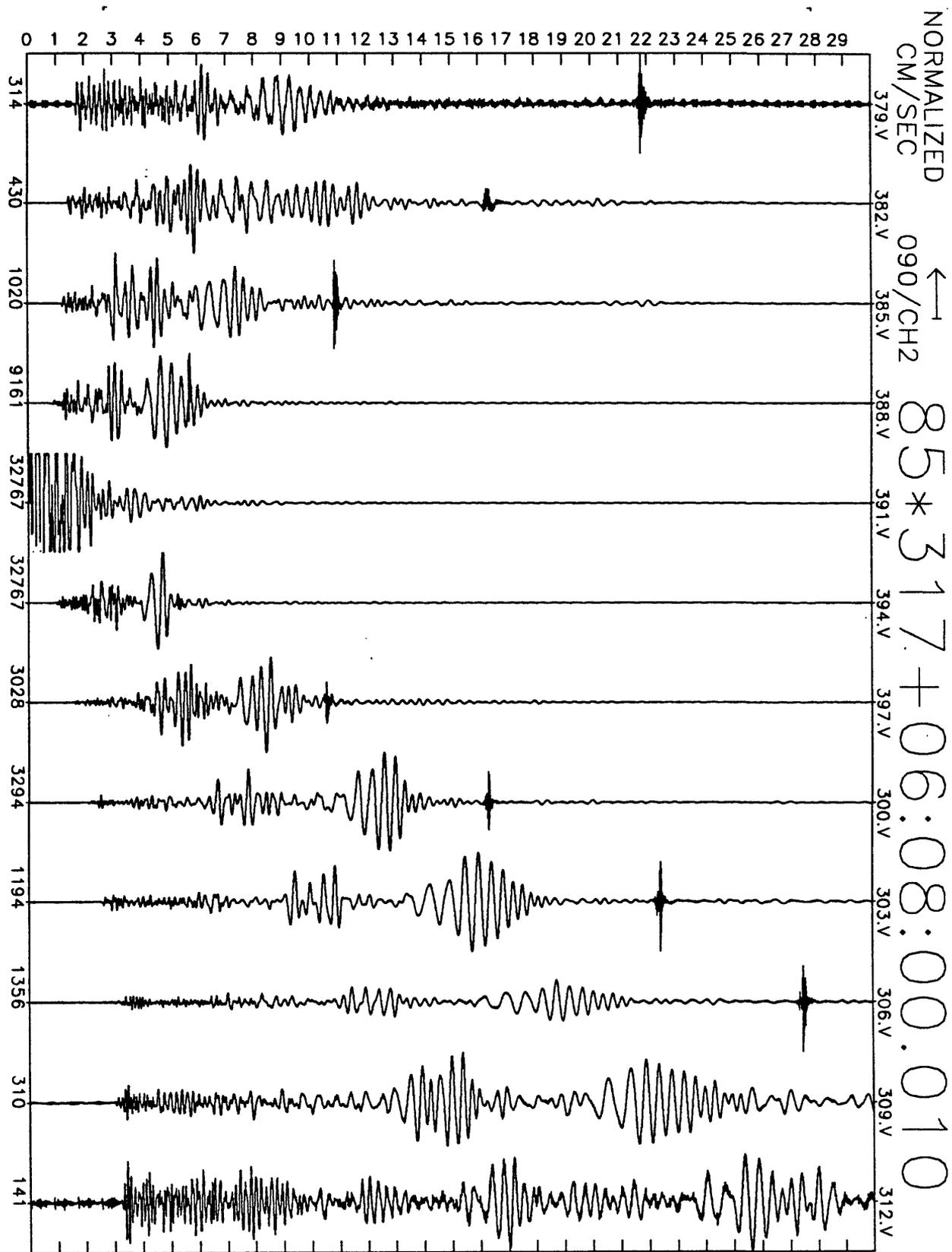
Figure A26(h), shot point 6X: 30 second N25E velocity record. Abscissa is labeled with maximum counts in record (multiply by  $\frac{10}{2^{24}-2^8} \approx 6 \times 10^{-7}$  to get cm/sec). Times are unreduced beginning at time indicated.
