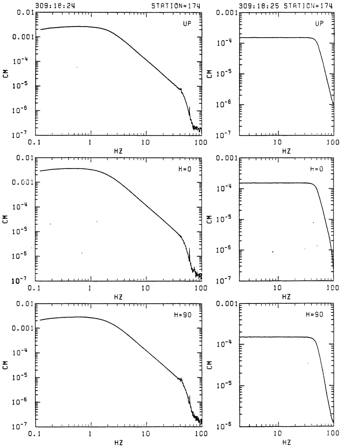
Figure C8. Station 174 in-situ velocity calibration spectra. Left: response to step in acceleration (seismometer mass released from rest at offset position). Right: response to delta function in velocity (voltage impulse applied to recorder input). From top: vertical, N33W and N57E.
