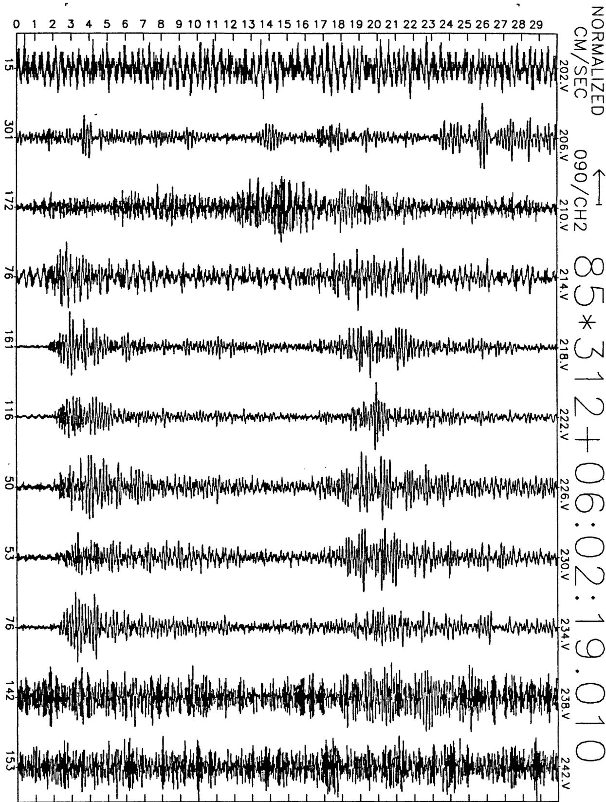
Figure A12(e), shot point 11: 30 second N20E velocity record. Abscissa is labeled with maximum counts in record (multiply by  $\frac{10}{2^{24}-2^8} \approx 6 \times 10^{-7}$  to get cm/sec). Times are unreduced beginning at time indicated.
