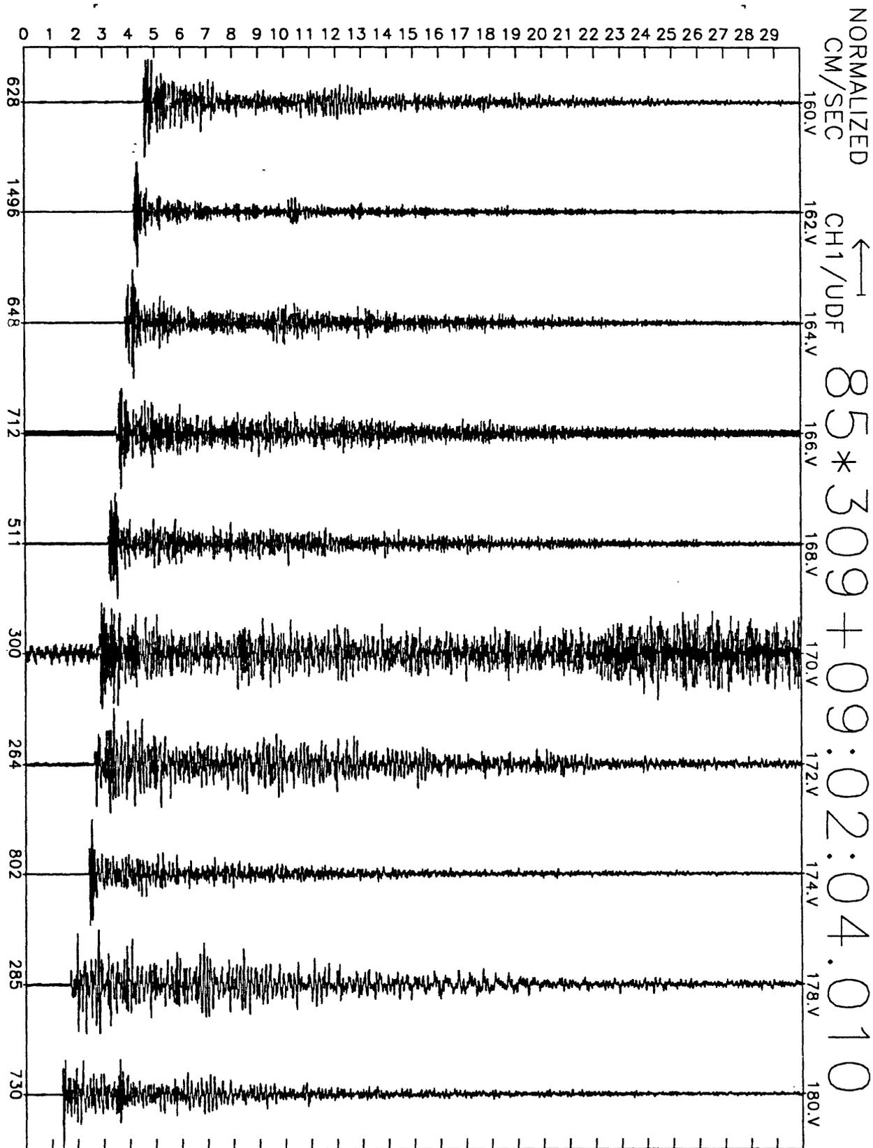
Figure A7(d), shot point 10: 30 second vertical velocity record. Abscissa is labeled with maximum counts in record (multiply by  $\frac{10}{2^{24}-2^8} \approx 6 \times 10^{-7}$  to get cm/sec). Times are unreduced beginning at time indicated.
