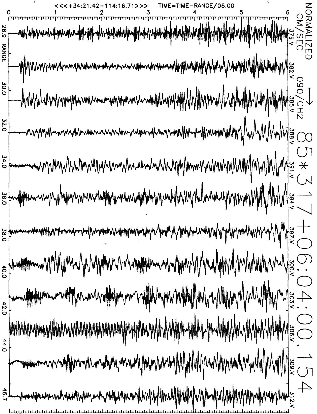
Figure A24(b), shot point 5: 6 second velocity record. Positive N25E motion is to right. Abscissa is distance to shot point. Top of trace is labeled with station number. Times are reduced by 6 km/sec. Shot time is indicated.
