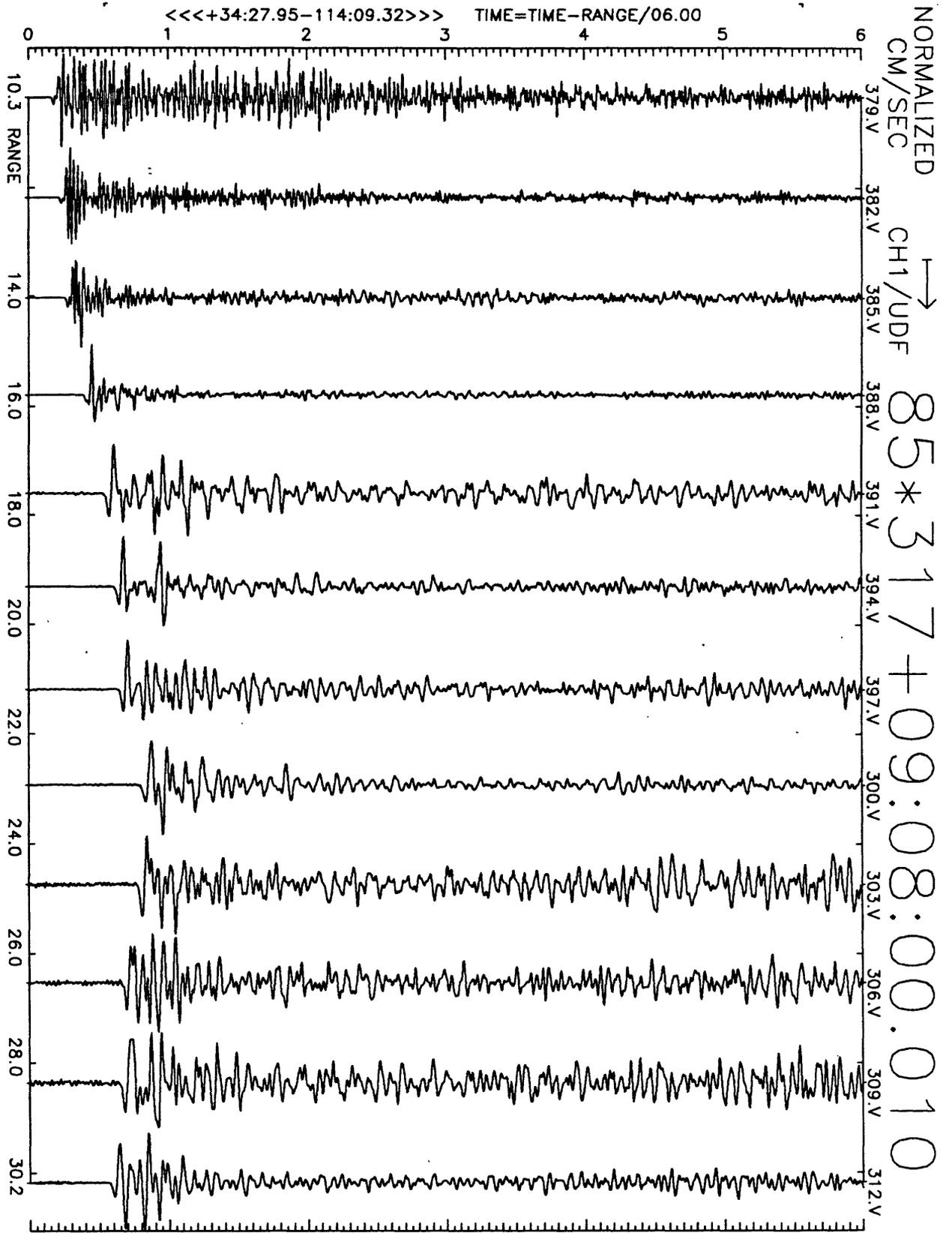
Figure A30(a), shot point 6: 6 second velocity record. Positive vertical motion is to right. Abscissa is distance to shot point. Top of trace is labeled with station number. Times are reduced by 6 km/sec. Shot time is indicated.
