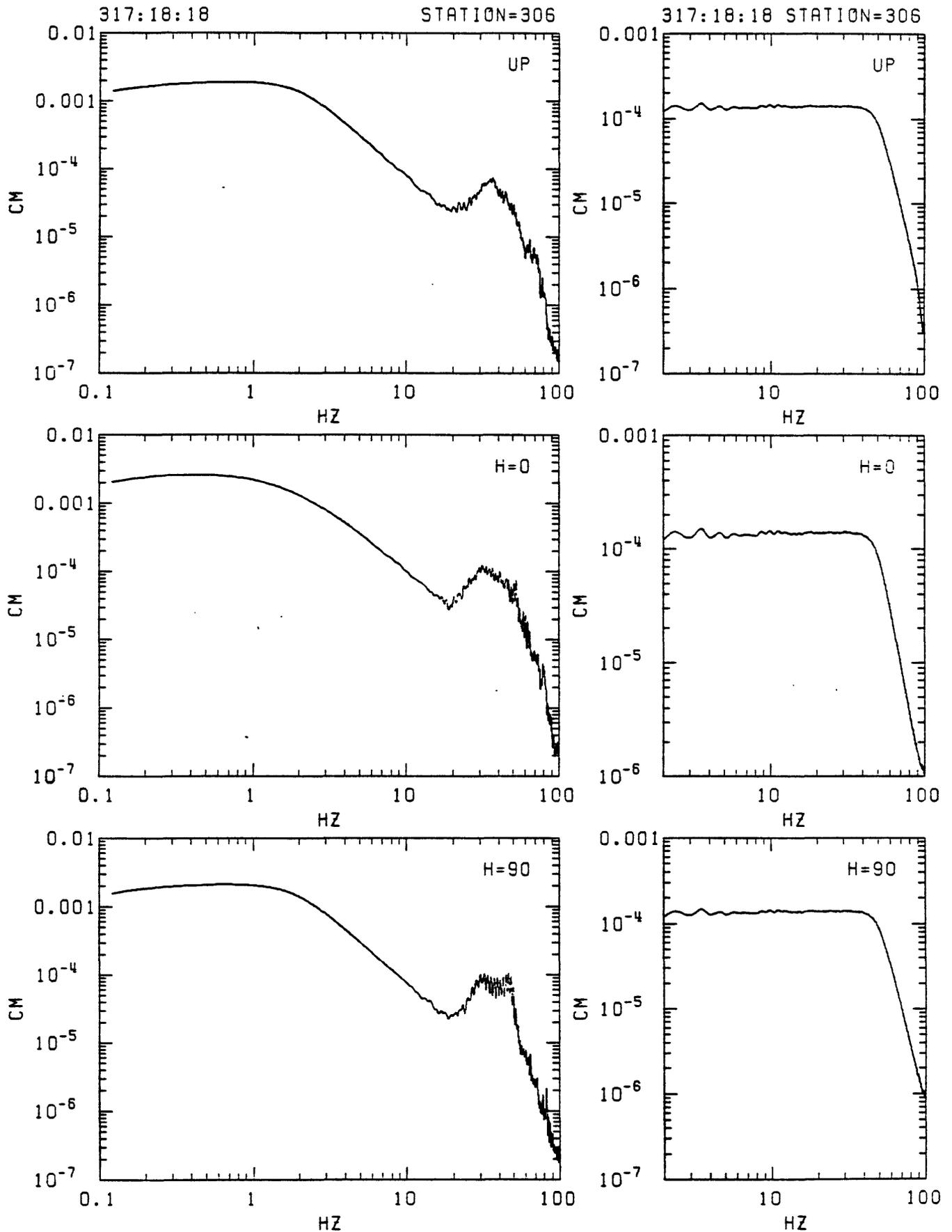
Figure C28. Station 306 in-situ velocity calibration spectra. Left: response to step in acceleration (seismometer mass released from rest at offset position). Right: response to delta function in velocity (voltage impulse applied to recorder input). From top: vertical, N25E and N115E.
