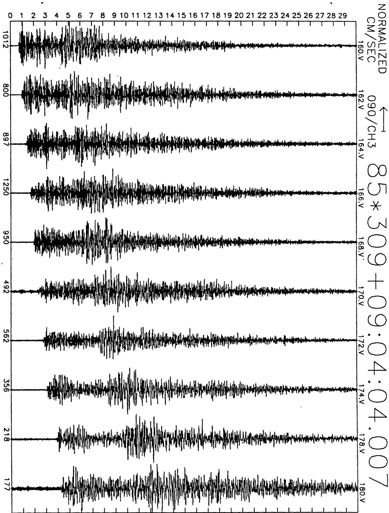
Figure A8(f), shot point 4A: 30 second N57E velocity record. Abscissa is labeled with maximum counts in record (multiply by  $\frac{10}{2^{24}-2^8} \approx 6 \times 10^{-7}$  to get cm/sec). Times are unreduced beginning at time indicated.
