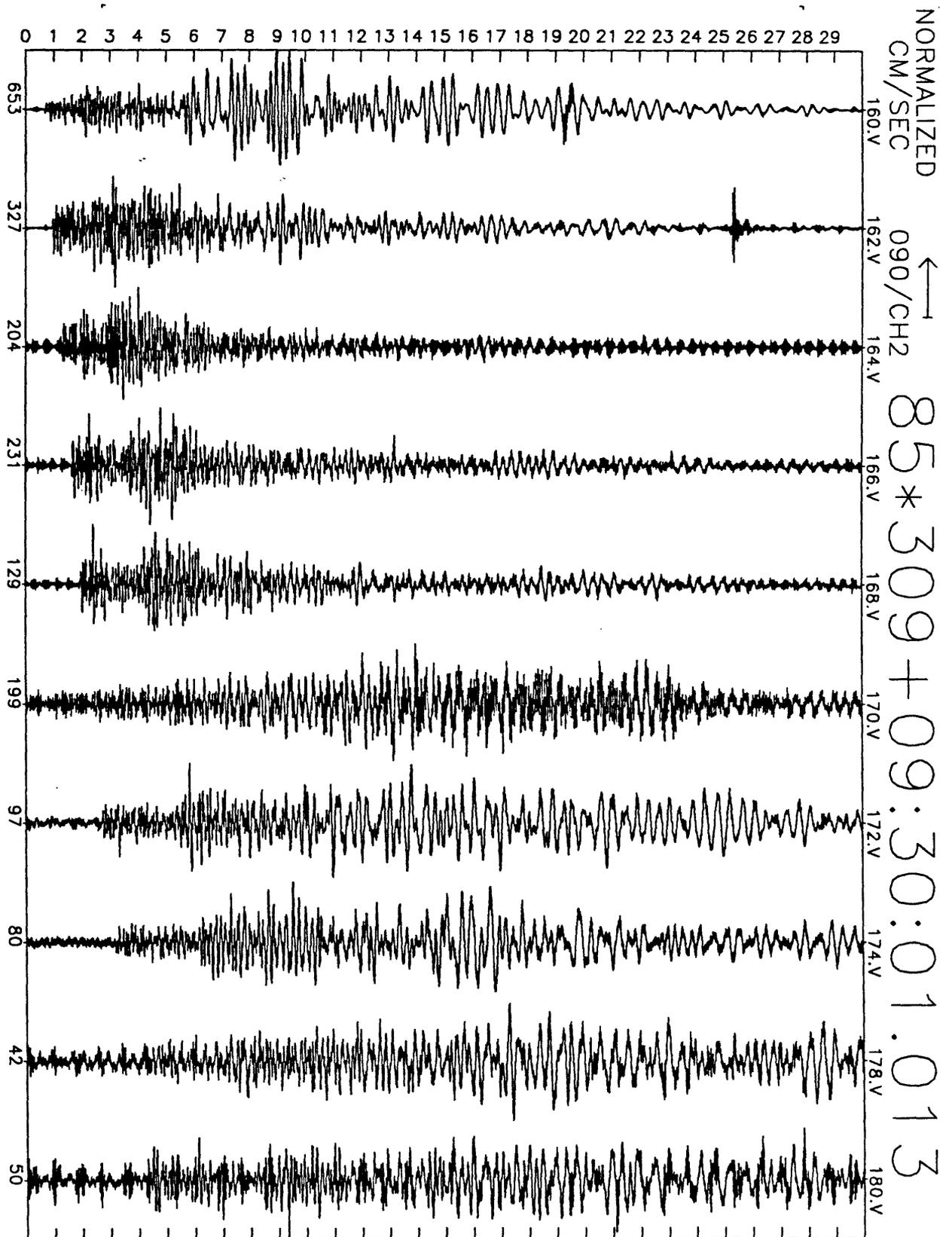
Figure A10(e), shot point 9X': 30 second N33W velocity record. Abscissa is labeled with maximum counts in record (multiply by  $\frac{10}{2^{24}-2^8} \approx 6 \times 10^{-7}$  to get cm/sec). Times are unreduced beginning at time indicated.
