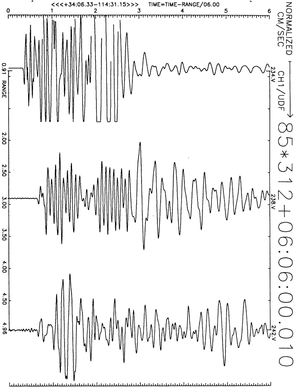
Figure A14(a), shot point 3, SW stations: 6 second velocity record. Positive vertical motion is to right. Abscissa is distance to shot point. Top of trace is labeled with station number. Times are reduced by 6 km/sec. Shot time is indicated.
