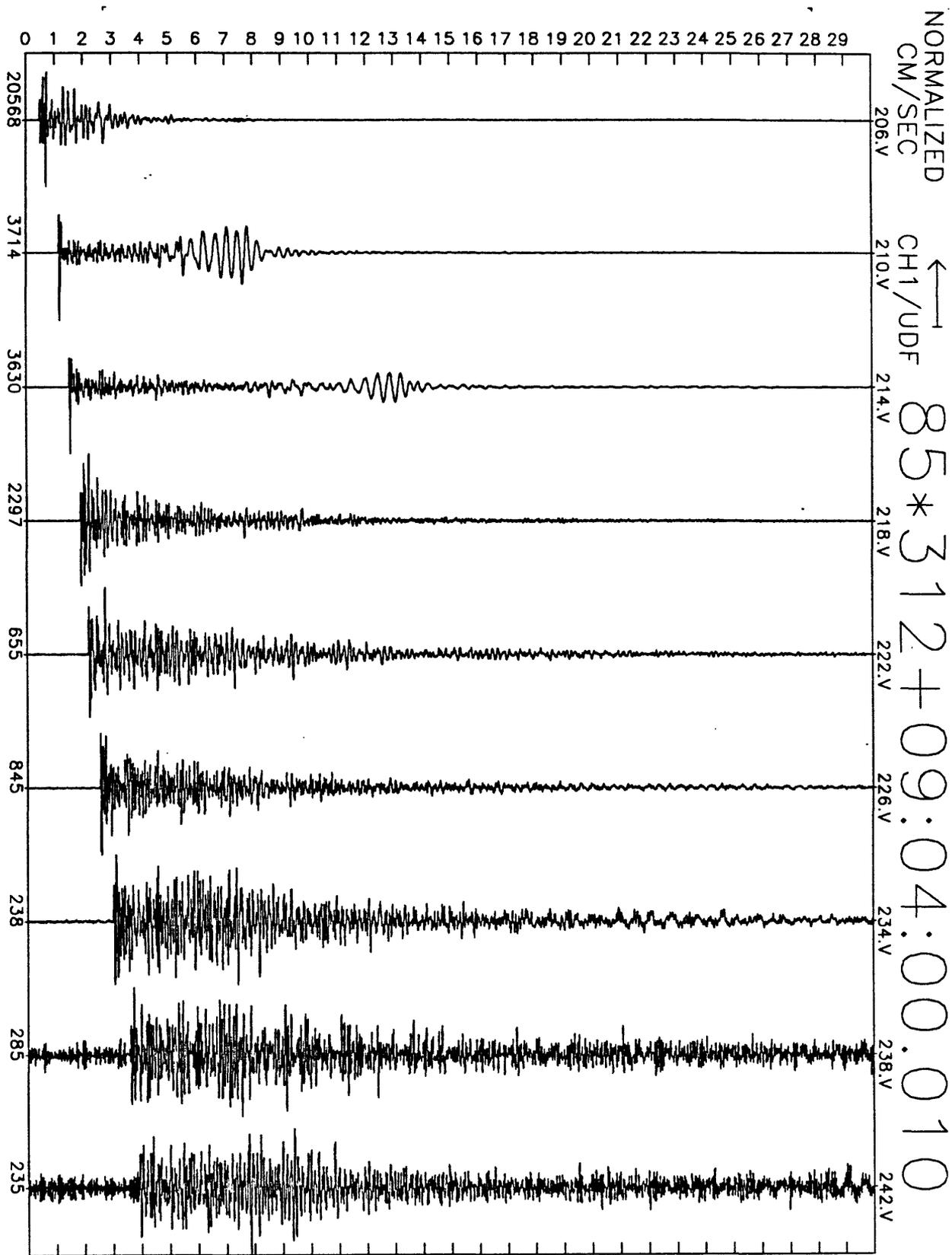
Figure A20(d), shot point 4B: 30 second vertical velocity record. Abscissa is labeled with maximum counts in record (multiply by  $\frac{10}{2^{24}-2^8} \approx 6 \times 10^{-7}$  to get cm/sec). Times are unreduced beginning at time indicated.
