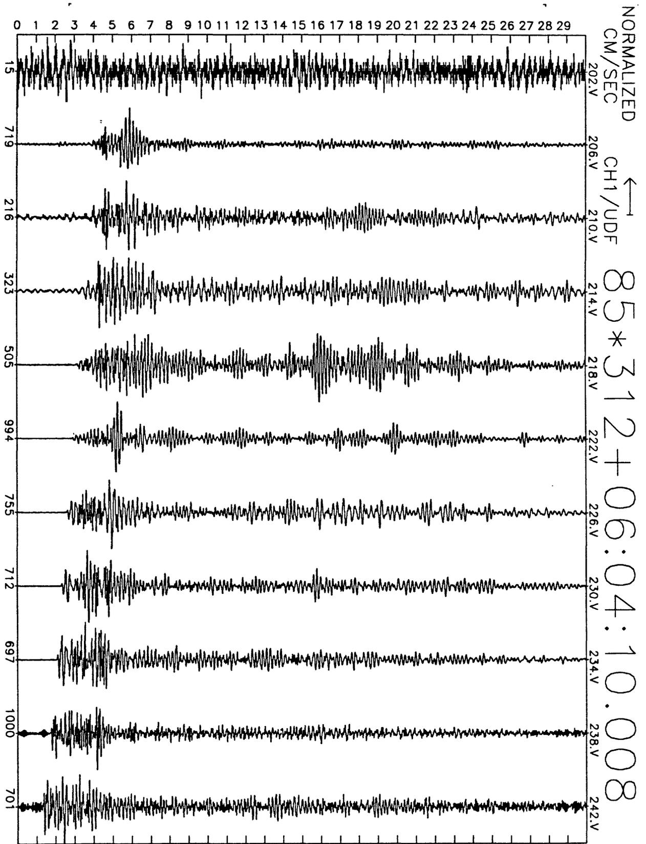
Figure A13(d), shot point 14: 30 second vertical velocity record. Abscissa is labeled with maximum counts in record (multiply by  $\frac{10}{2^{24}-2^8} \approx 6 \times 10^{-7}$  to get cm/sec). Times are unreduced beginning at time indicated.
