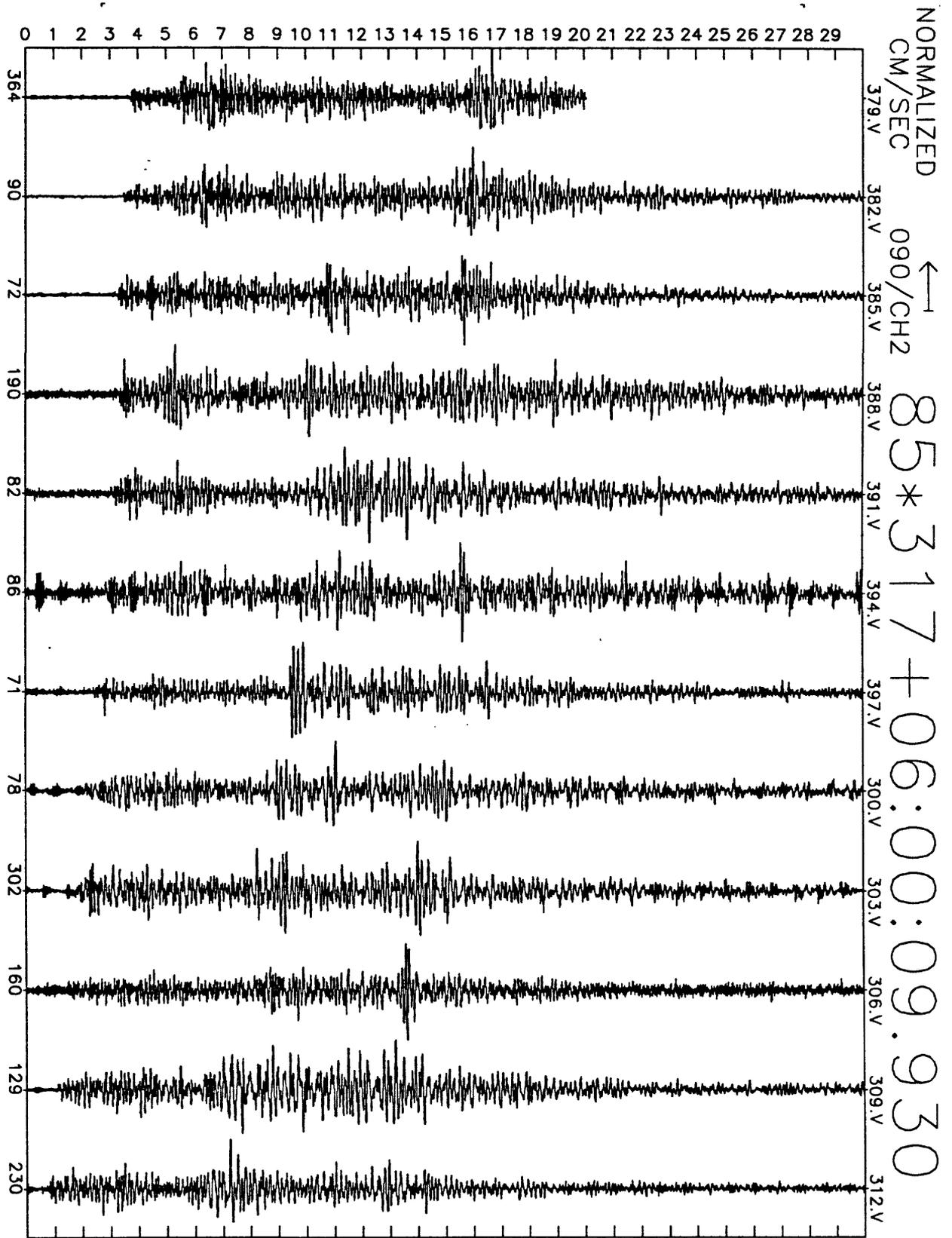
Figure A22(f), shot point 12: 30 second N115E velocity record. Abscissa is labeled with maximum counts in record (multiply by  $\frac{10}{2^{24}-2^8} \approx 6 \times 10^{-7}$  to get cm/sec). Times are unreduced beginning at time indicated.
