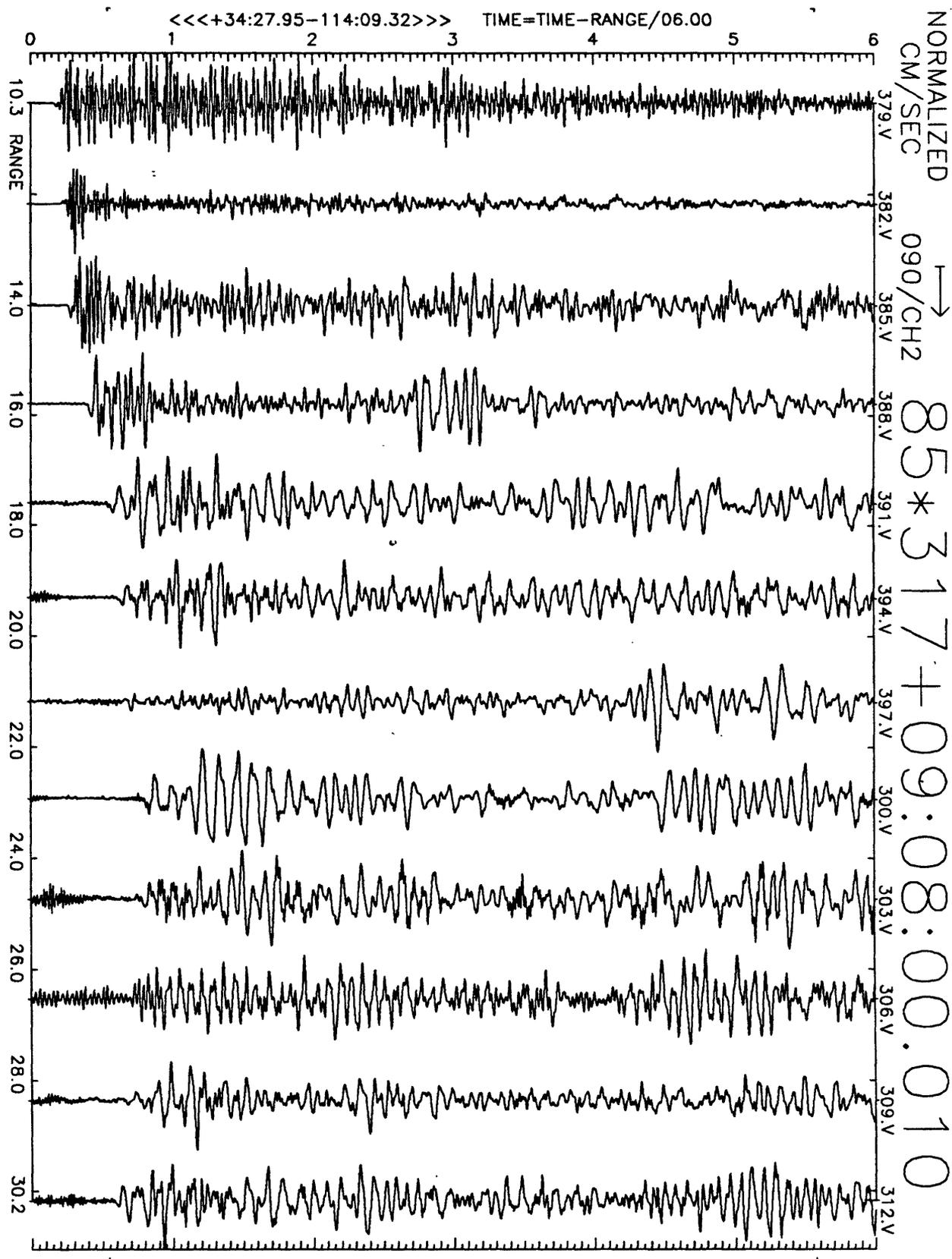
Figure A30(b), shot point 6: 6 second velocity record. Positive N25E motion is to right. Abscissa is distance to shot point. Top of trace is labeled with station number. Times are reduced by 6 km/sec. Shot time is indicated.
