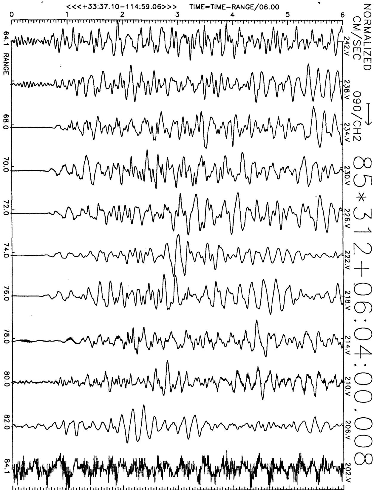
Figure A13(b), shot point 14: 6 second velocity record. Positive N20E motion is to right. Abscissa is distance to shot point. Top of trace is labeled with station number. Times are reduced by 6 km/sec. Shot time is indicated.
