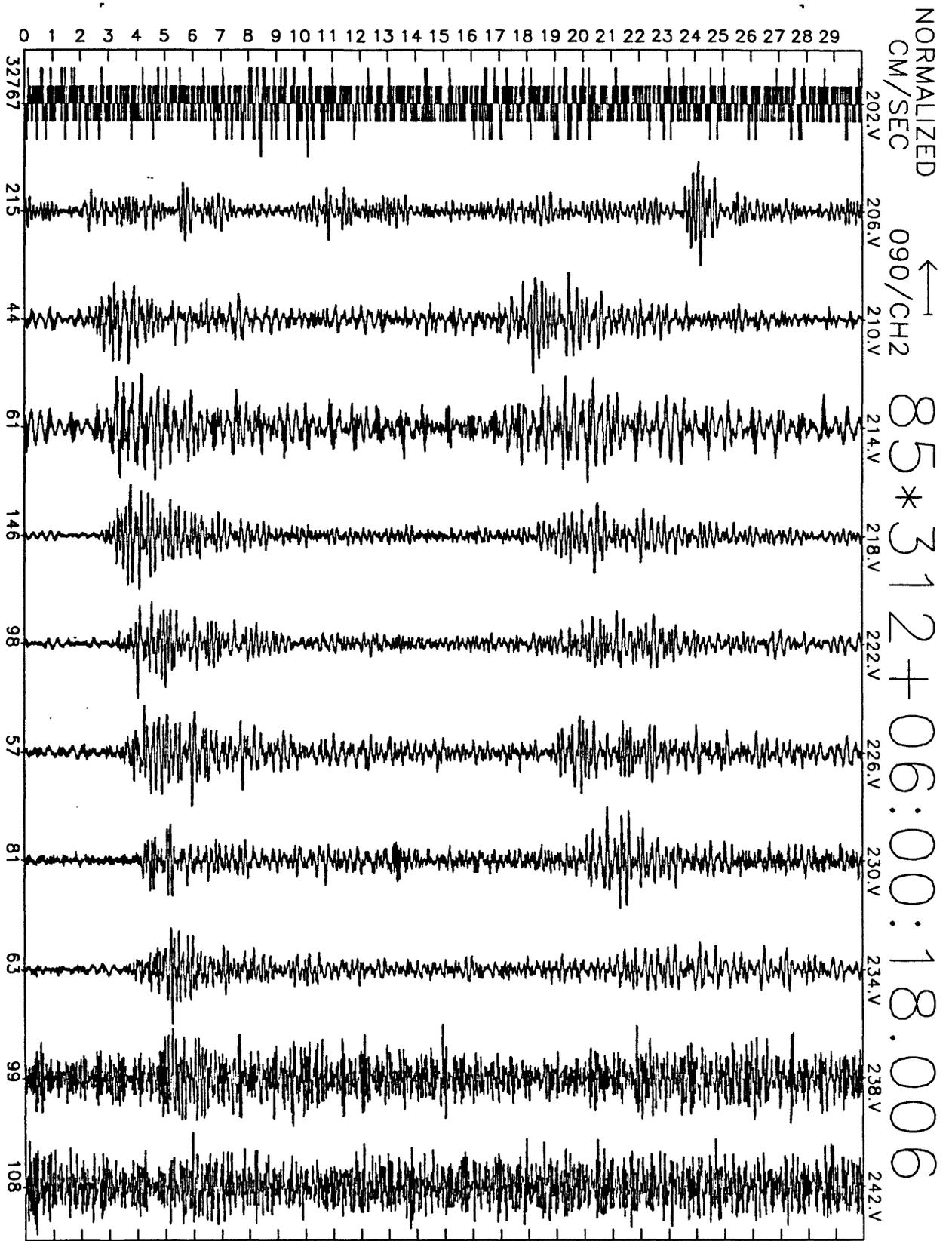
Figure A11(e), shot point 12: 30 second N20E velocity record. Abscissa is labeled with maximum counts in record (multiply by  $\frac{10}{2^{24}-2^8} \approx 6 \times 10^{-7}$  to get cm/sec). Times are unreduced beginning at time indicated.
