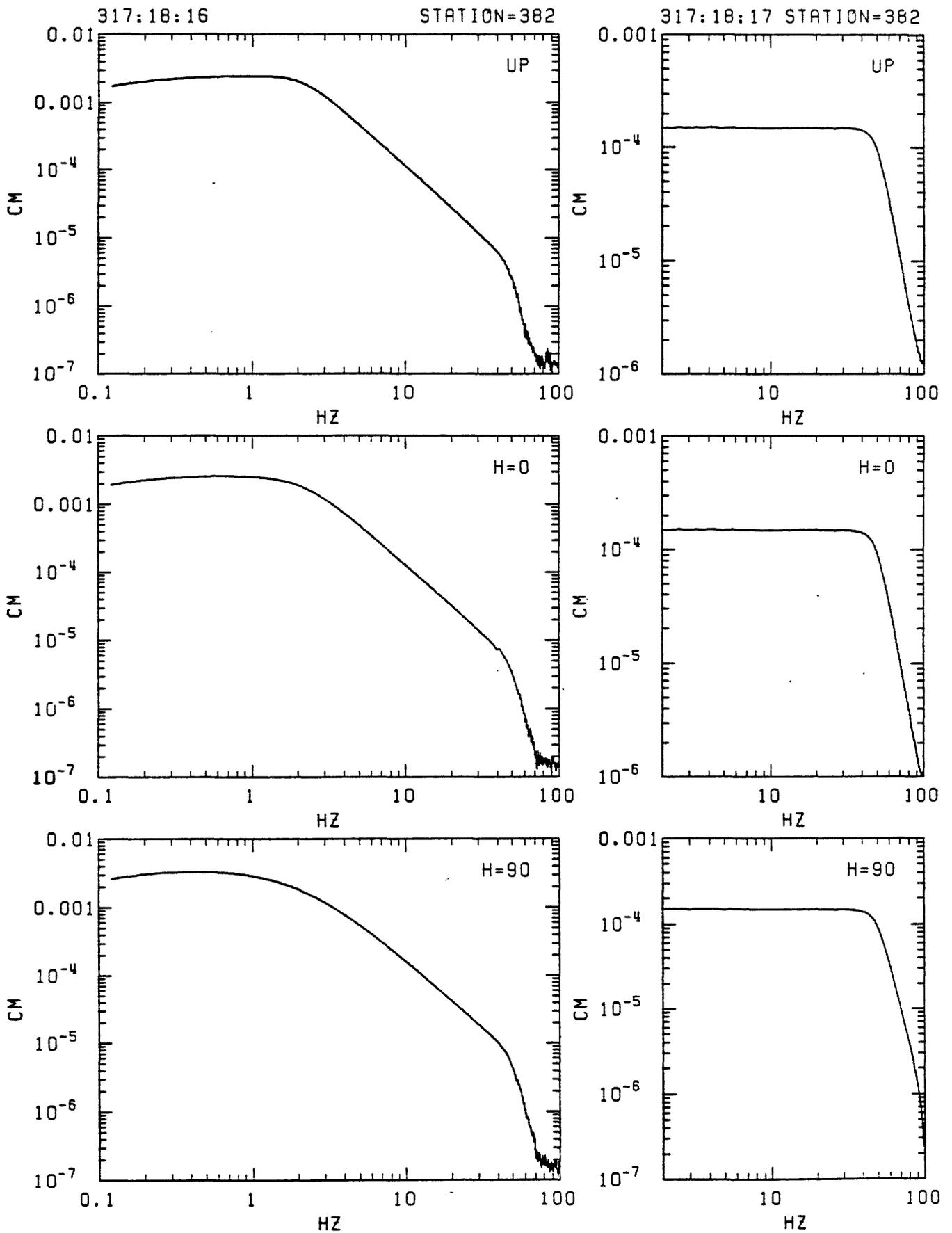
Figure C21. Station 382 in-situ velocity calibration spectra. Left: response to step in acceleration (seismometer mass released from rest at offset position). Right: response to delta function in velocity (voltage impulse applied to recorder input). From top: vertical, N25E and N115E.
