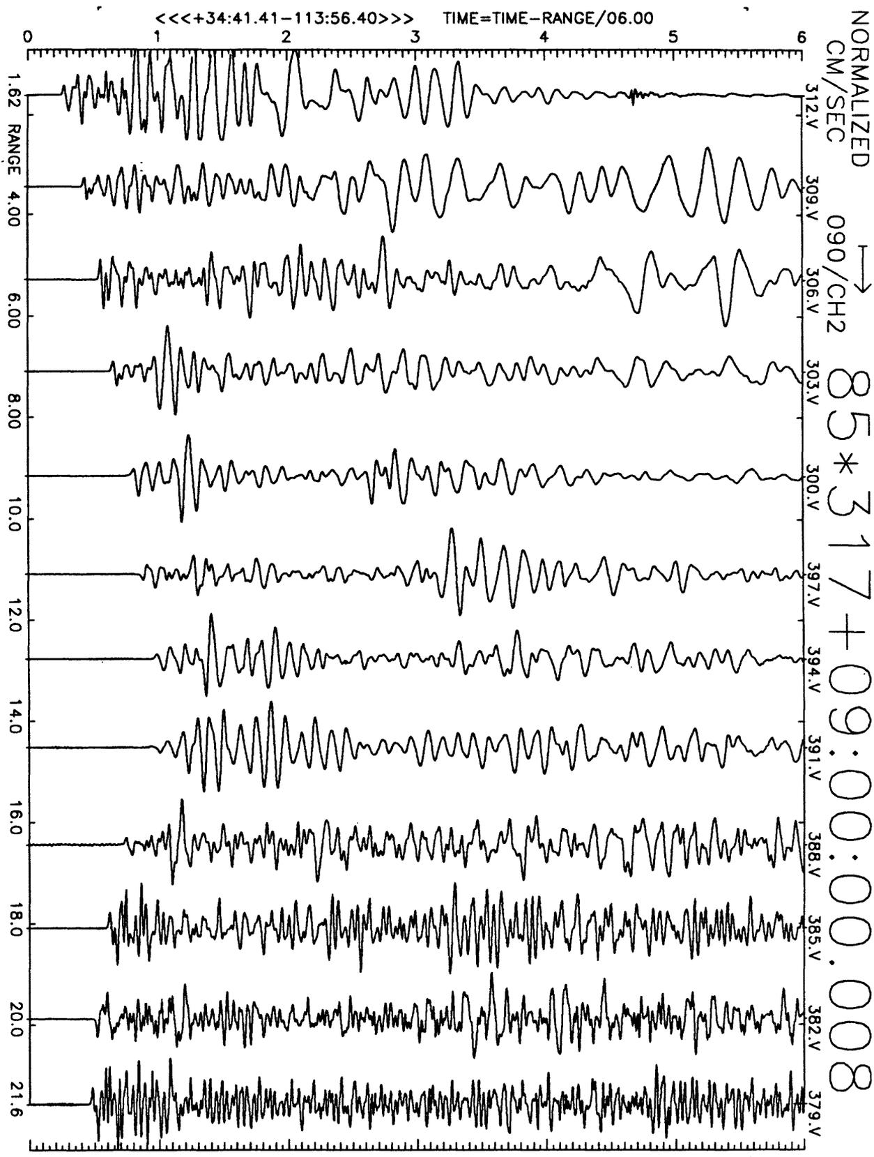
Figure A27(b), shot point 7: 6 second velocity record. Positive N25E motion is to right. Abscissa is distance to shot point. Top of trace is labeled with station number. Times are reduced by 6 km/sec. Shot time is indicated.
