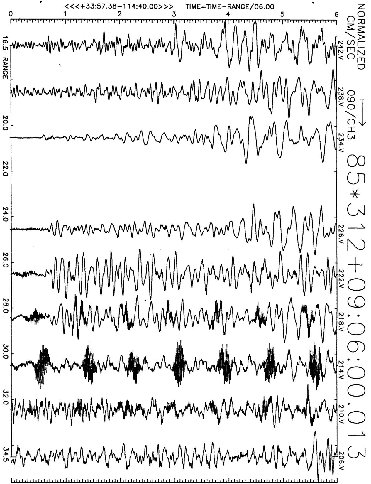
Figure A21(c), shot point 1X: 6 second velocity record. Positive N110E motion is to right. Abscissa is distance to shot point. Top of trace is labeled with station number. Times are reduced by 6 km/sec. Shot time is indicated.
