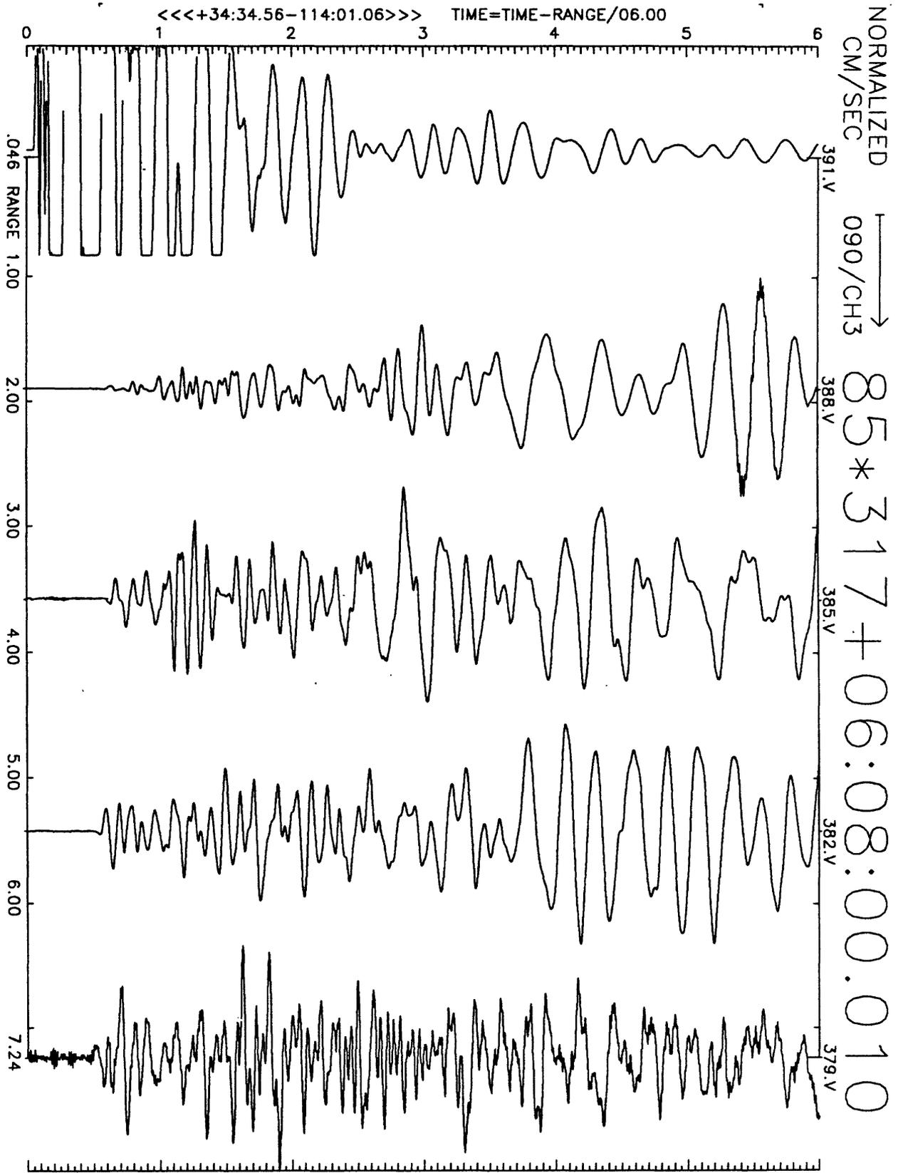
Figure A26(c), shot point 6X, SW stations: 6 second velocity record. Positive N115E motion is to right. Abscissa is distance to shot point. Top of trace is labeled with station number. Times are reduced by 6 km/sec. Shot time is indicated.
