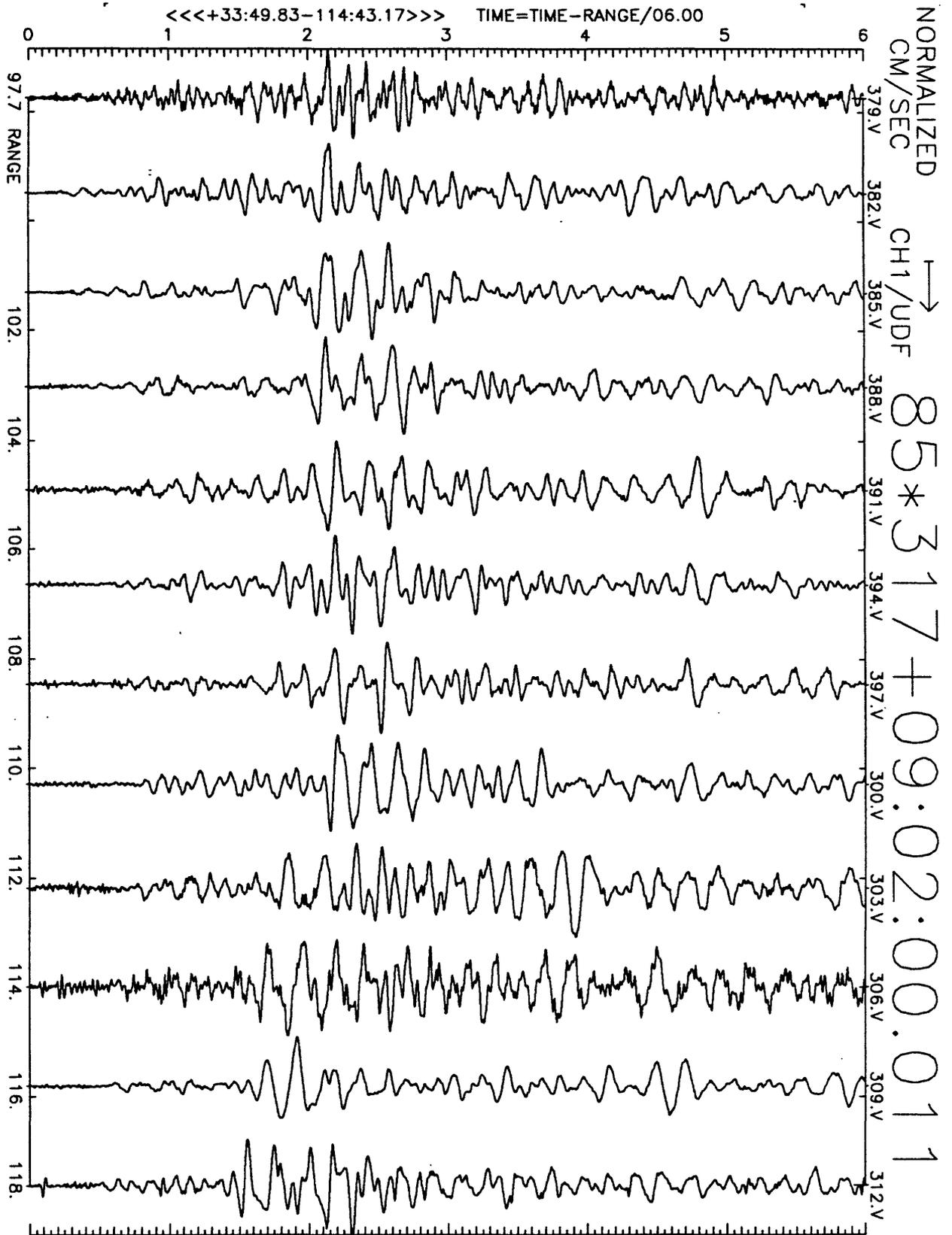
Figure A28(a), shot point 1: 6 second velocity record. Positive vertical motion is to right. Abscissa is distance to shot point. Top of trace is labeled with station number. Times are reduced by 6 km/sec. Shot time is indicated.
