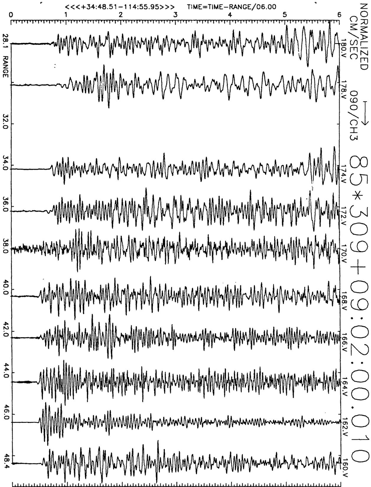
Figure A7(c), shot point 10: 6 second velocity record. Positive N57E motion is to right. Abscissa is distance to shot point. Top of trace is labeled with station number. Times are reduced by 6 km/sec. Shot time is indicated.
