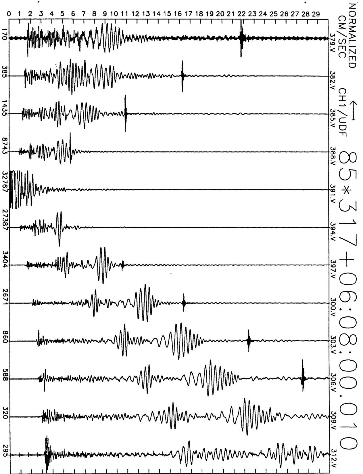
Figure A26(g), shot point 6X: 30 second vertical velocity record. Abscissa is labeled with maximum counts in record (multiply by  $\frac{10}{2^{24}-2^8} \approx 6 \times 10^{-7}$  to get cm/sec). Times are unreduced beginning at time indicated.
