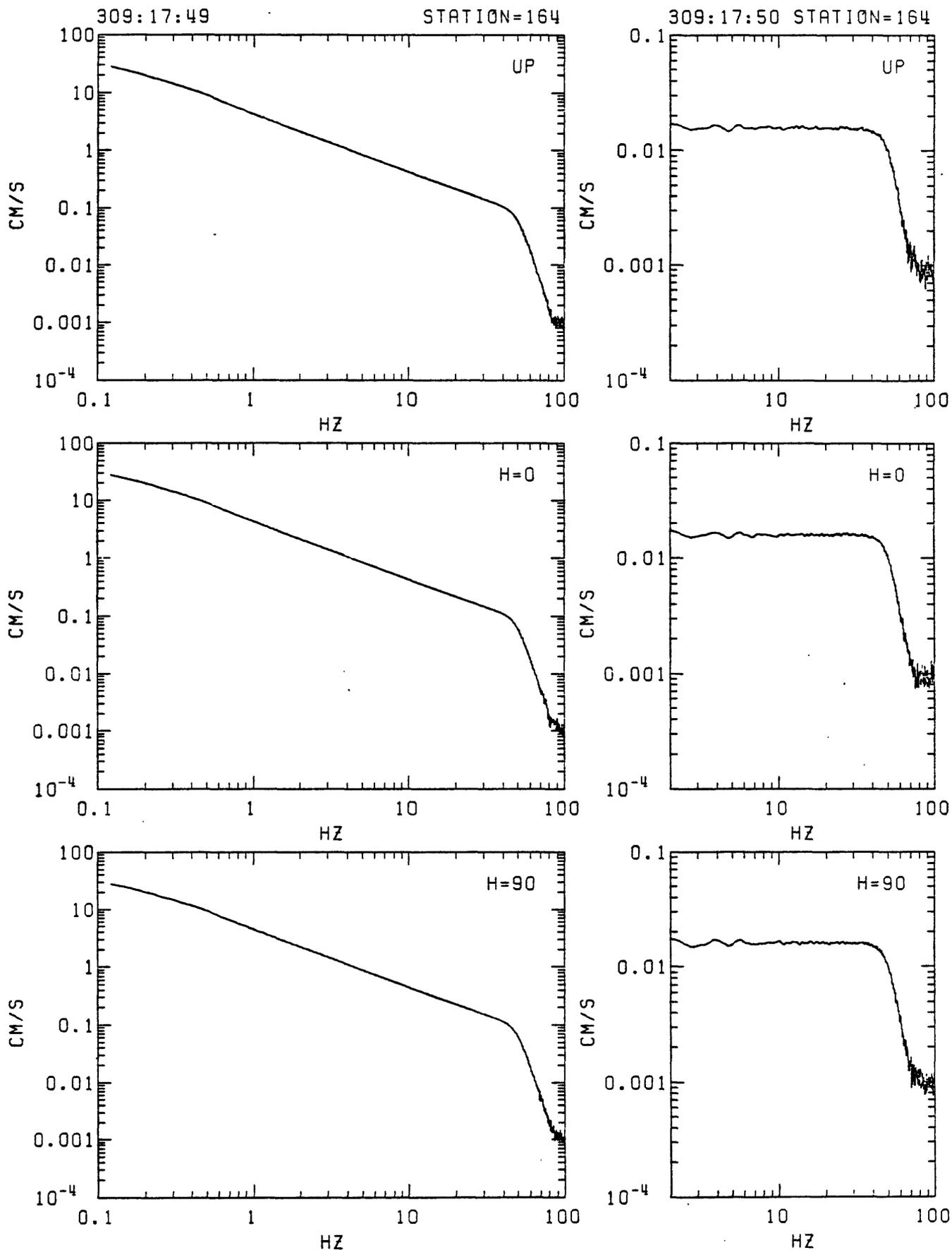
Figure D1. Station 164 in-situ 18db acceleration calibration spectra. Left: response to step in acceleration (reset FBA servo amplifier reference voltage from non-zero). Right: response to delta function in acceleration (voltage impulse applied to recorder input). From top: vertical, N33W and N57E.
