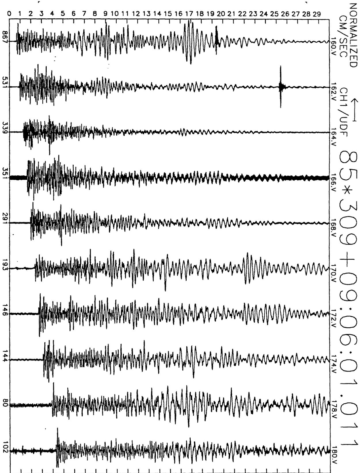
Figure A9(d), shot point 9X: 30 second vertical velocity record. Abscissa is labeled with maximum counts in record (multiply by  $\frac{10}{2^{24}-2^8} \approx 6 \times 10^{-7}$  to get cm/sec). Times are unreduced beginning at time indicated.
