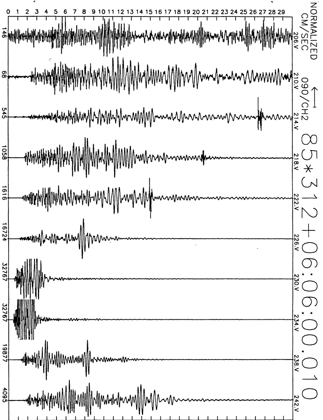
Figure A14(h), shot point 3: 30 second N20E velocity record. Abscissa is labeled with maximum counts in record (multiply by  $\frac{10}{2^{24}-2^8} \approx 6 \times 10^{-7}$  to get cm/sec). Times are unreduced beginning at time indicated.
