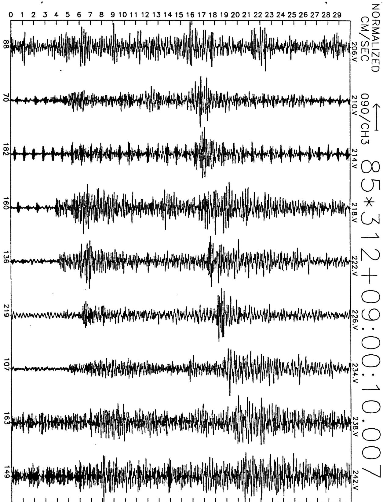
Figure A18(f), shot point 7: 30 second N110E velocity record. Abscissa is labeled with maximum counts in record (multiply by  $\frac{10}{2^{24}-2^8} \approx 6 \times 10^{-7}$  to get cm/sec). Times are unreduced beginning at time indicated.
