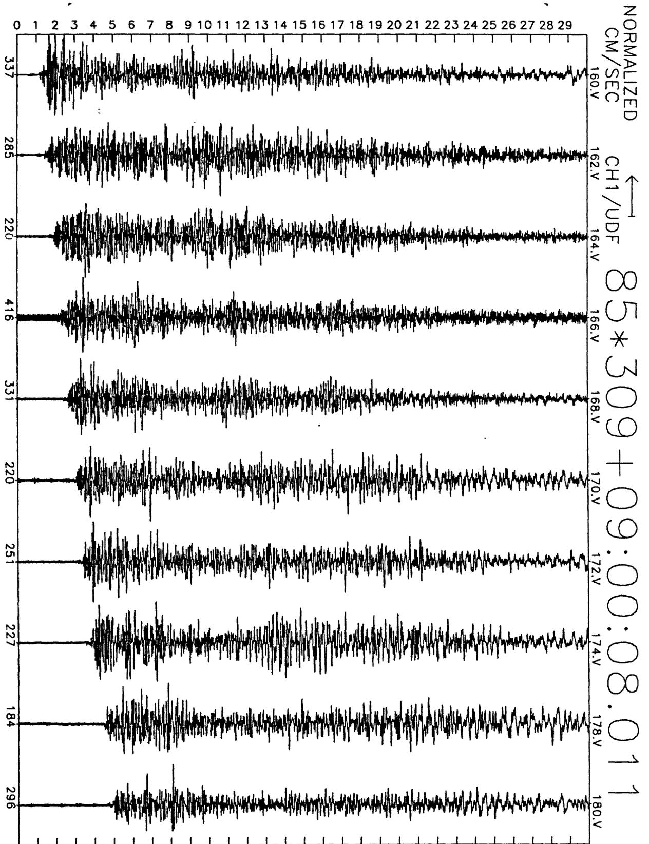
Figure A6(d), shot point 8X: 30 second vertical velocity record. Abscissa is labeled with maximum counts in record (multiply by  $\frac{10}{2^{24}-2^8} \approx 6 \times 10^{-7}$  to get cm/sec). Times are unreduced beginning at time indicated.
