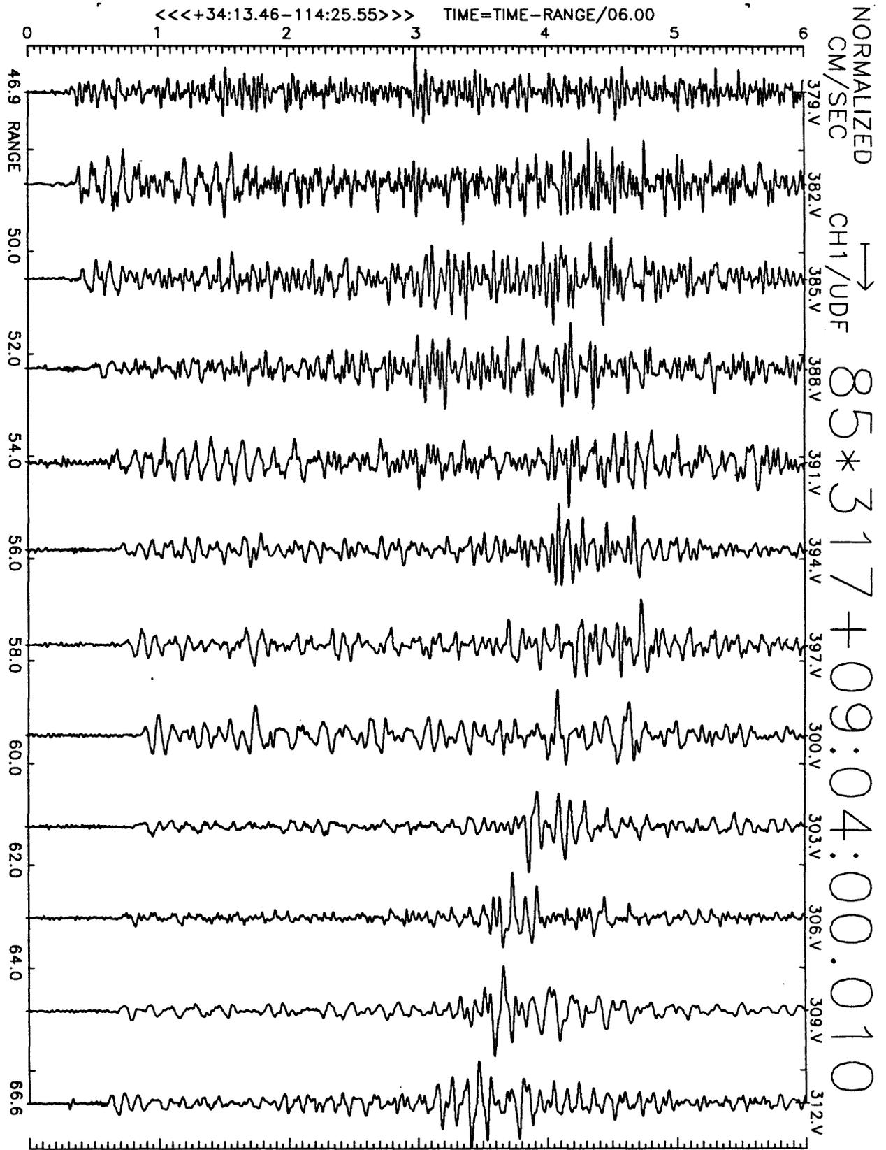
Figure A29(a), shot point 4B: 6 second velocity record. Positive vertical motion is to right. Abscissa is distance to shot point. Top of trace is labeled with station number. Times are reduced by 6 km/sec. Shot time is indicated.
