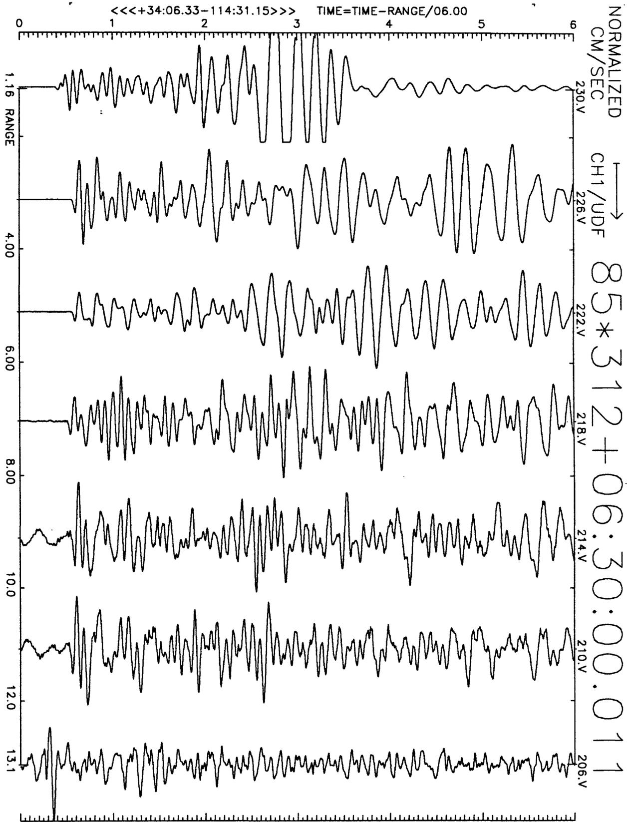
Figure A16(d), shot point 3', NE stations: 6 second velocity record. Positive vertical motion is to right. Abscissa is distance to shot point. Top of trace is labeled with station number. Times are reduced by 6 km/sec. Shot time is indicated.
