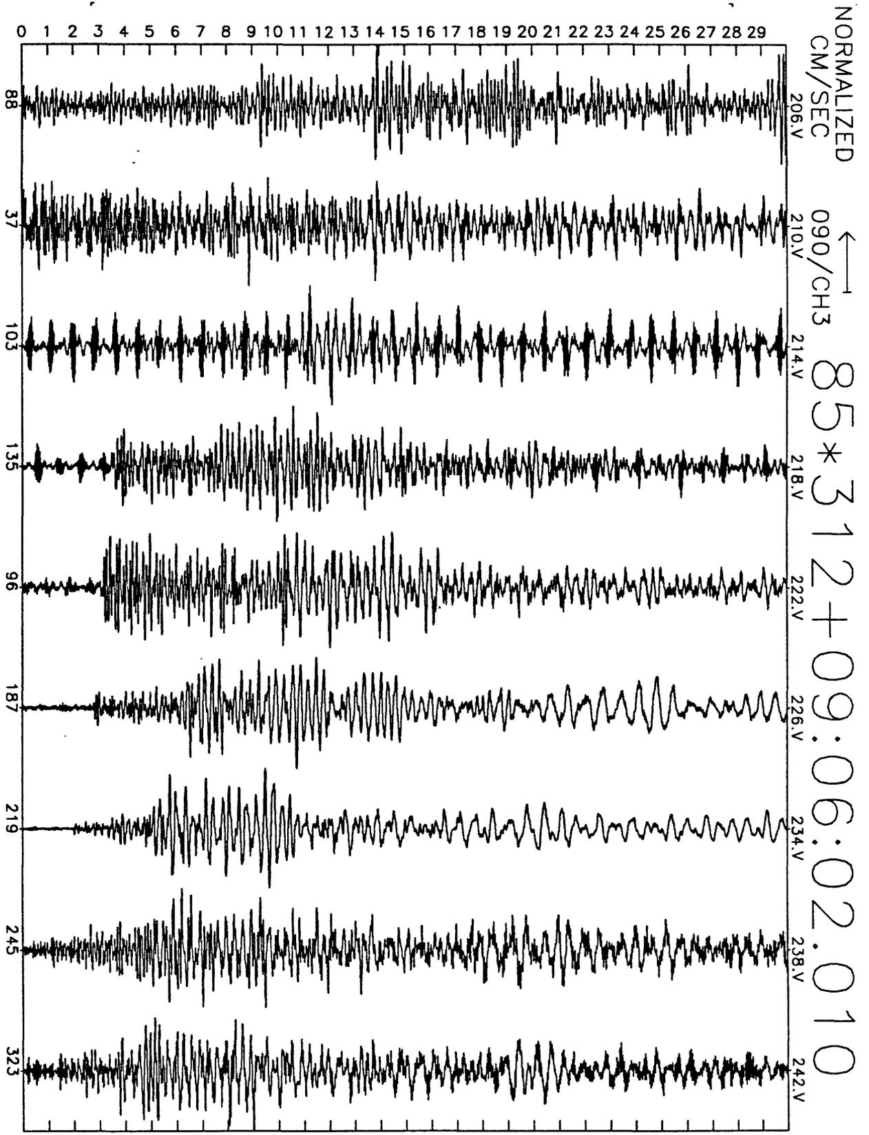
Figure A21(f), shot point 1X: 30 second N110E velocity record. Abscissa is labeled with maximum counts in record (multiply by  $\frac{10}{2^{24}-2^8} \approx 6 \times 10^{-7}$  to get cm/sec). Times are unreduced beginning at time indicated.
