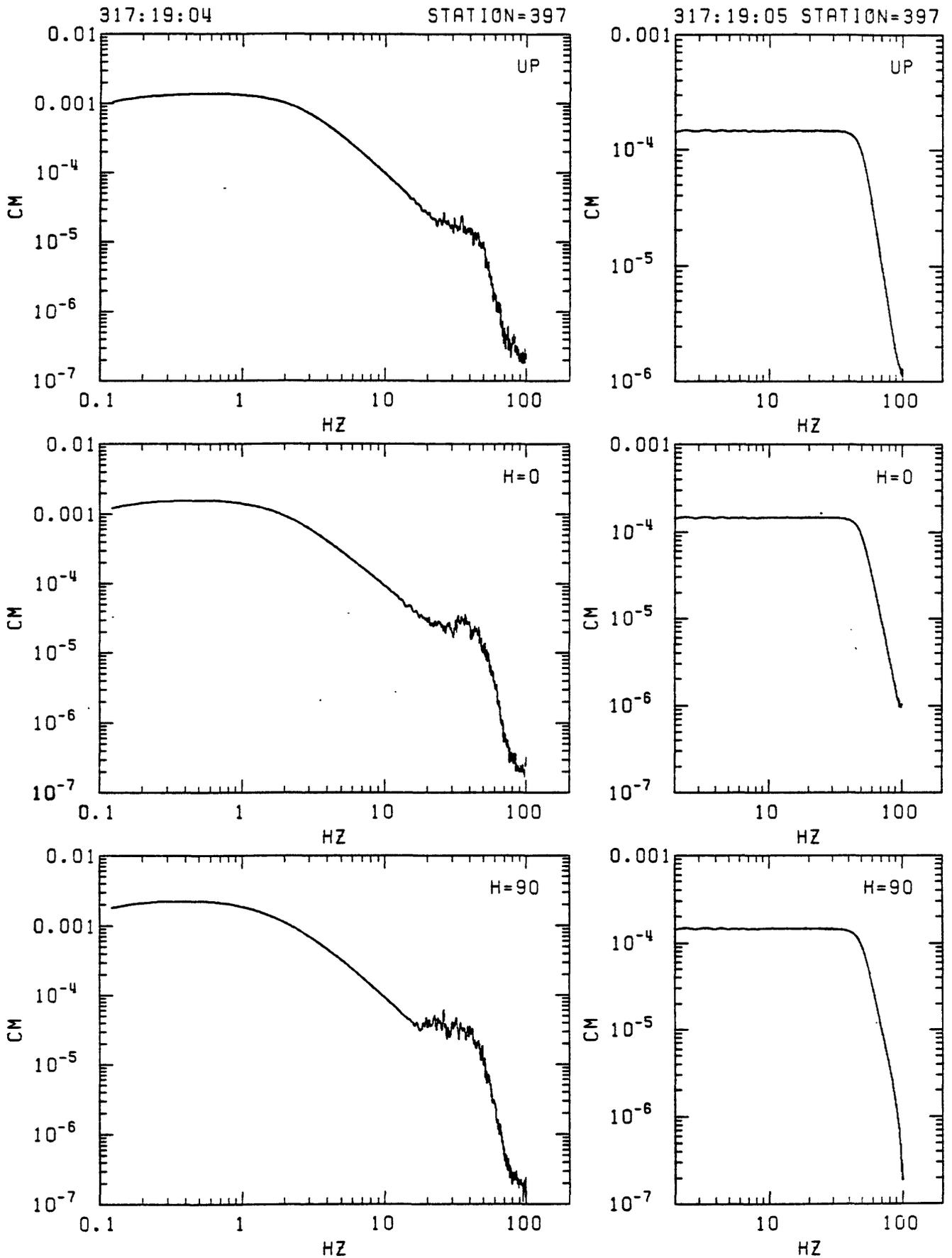
Figure C26. Station 397 in-situ velocity calibration spectra. Left: response to step in acceleration (seismometer mass released from rest at offset position). Right: response to delta function in velocity (voltage impulse applied to recorder input). From top: vertical, N25E and N115E.
