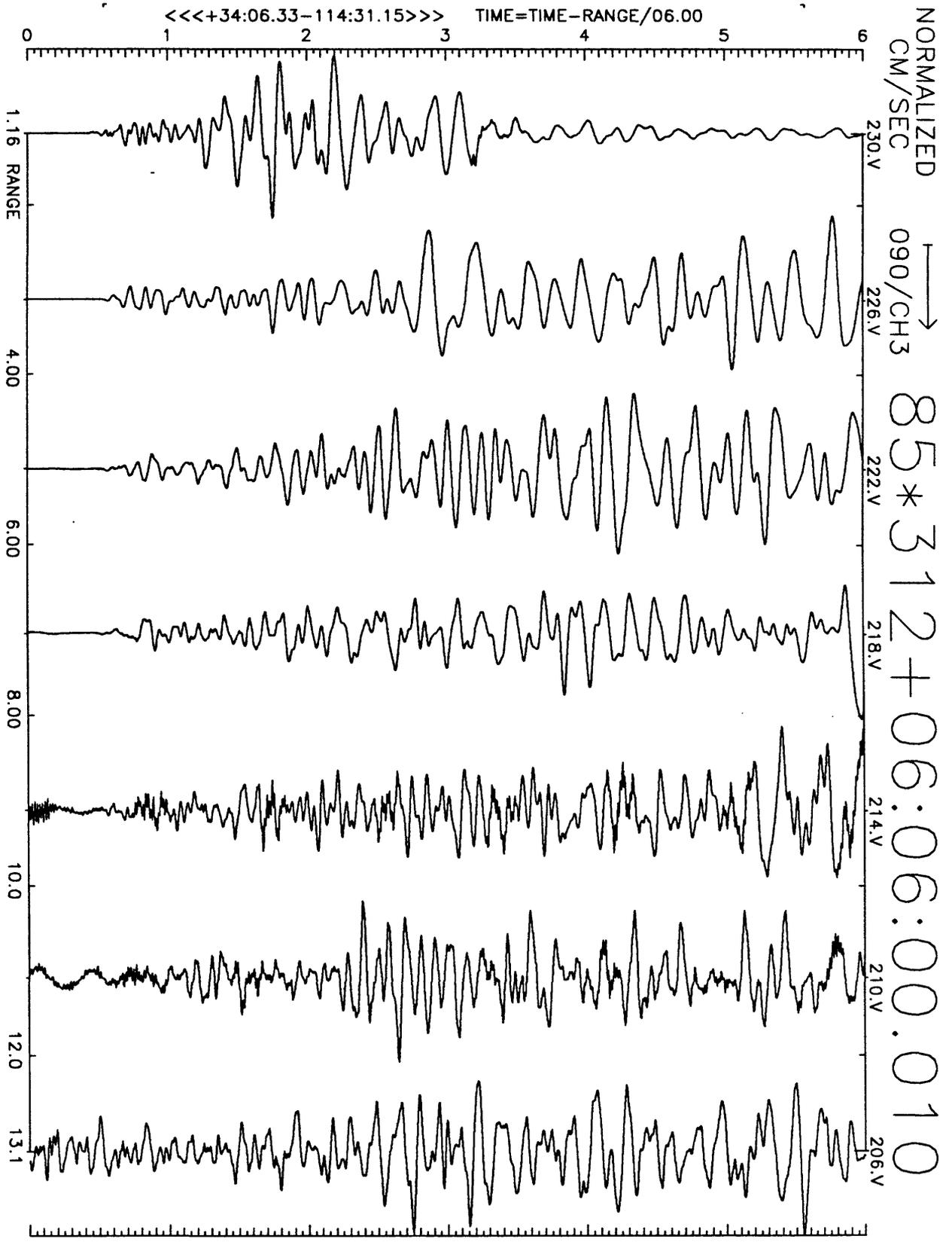
Figure A14(f), shot point 3, NE stations: 6 second velocity record. Positive N110E motion is to right. Abscissa is distance to shot point. Top of trace is labeled with station number. Times are reduced by 6 km/sec. Shot time is indicated.
