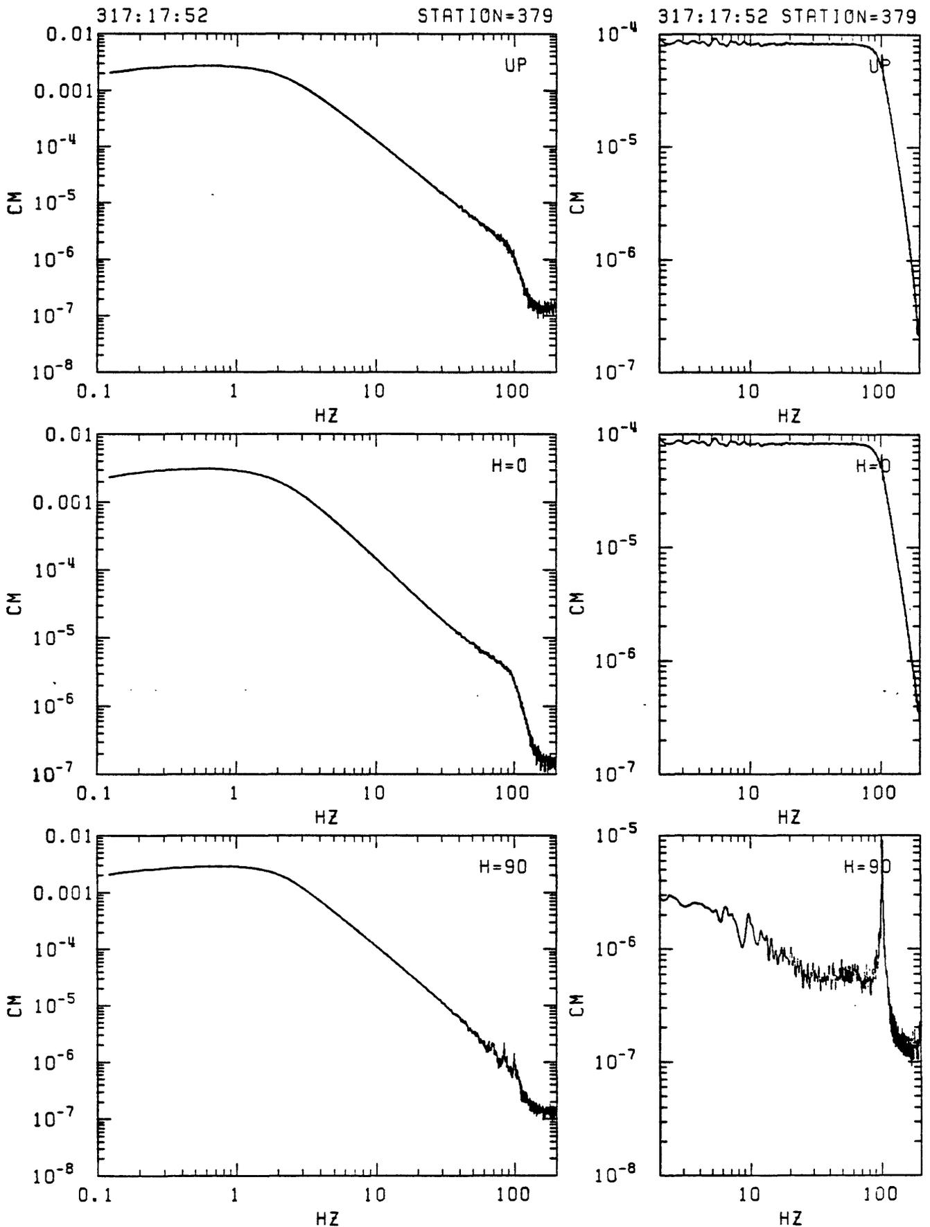
Figure C20. Station 379 in-situ velocity calibration spectra. Left: response to step in acceleration (seismometer mass released from rest at offset position). Right: response to delta function in velocity (voltage impulse applied to recorder input). From top: vertical, N25E and N115E.
