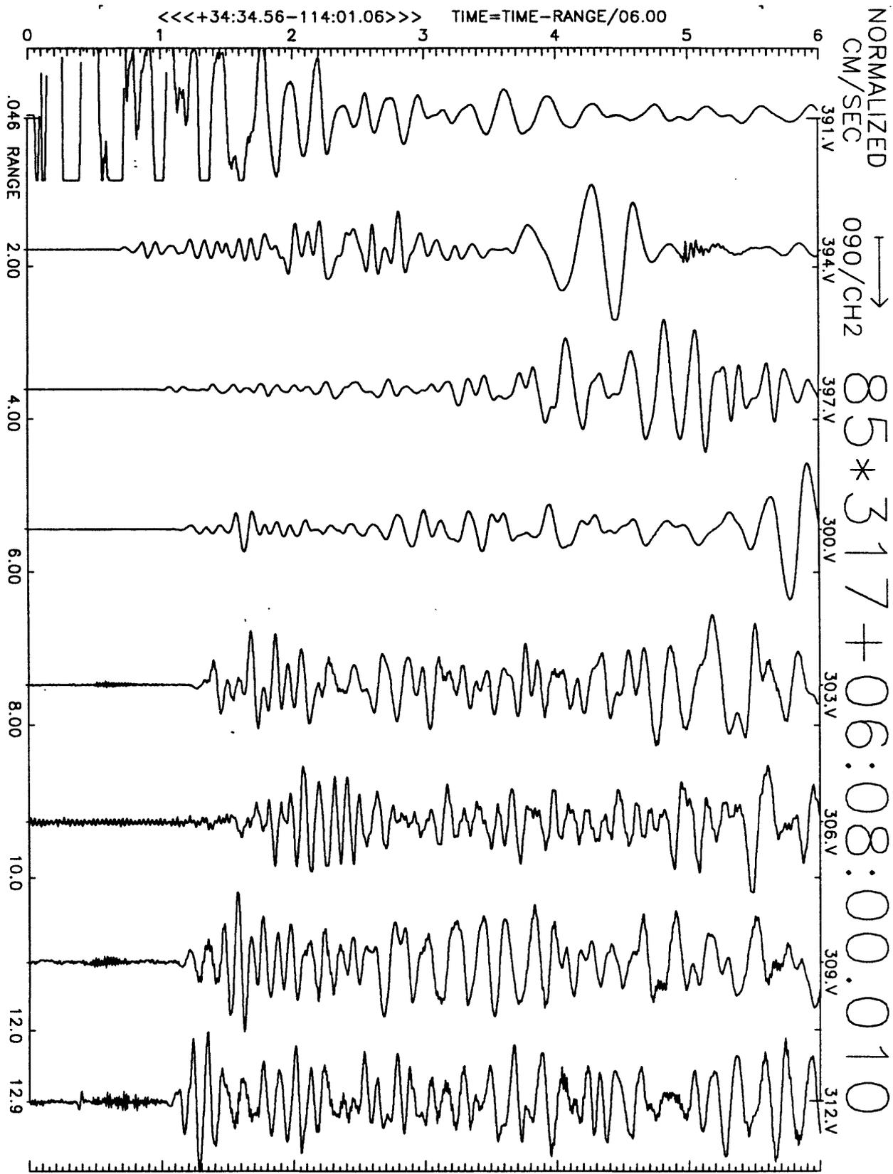
Figure A26(e), shot point 6X, NE stations: 6 second velocity record. Positive N25E motion is to right. Abscissa is distance to shot point. Top of trace is labeled with station number. Times are reduced by 6 km/sec. Shot time is indicated.
