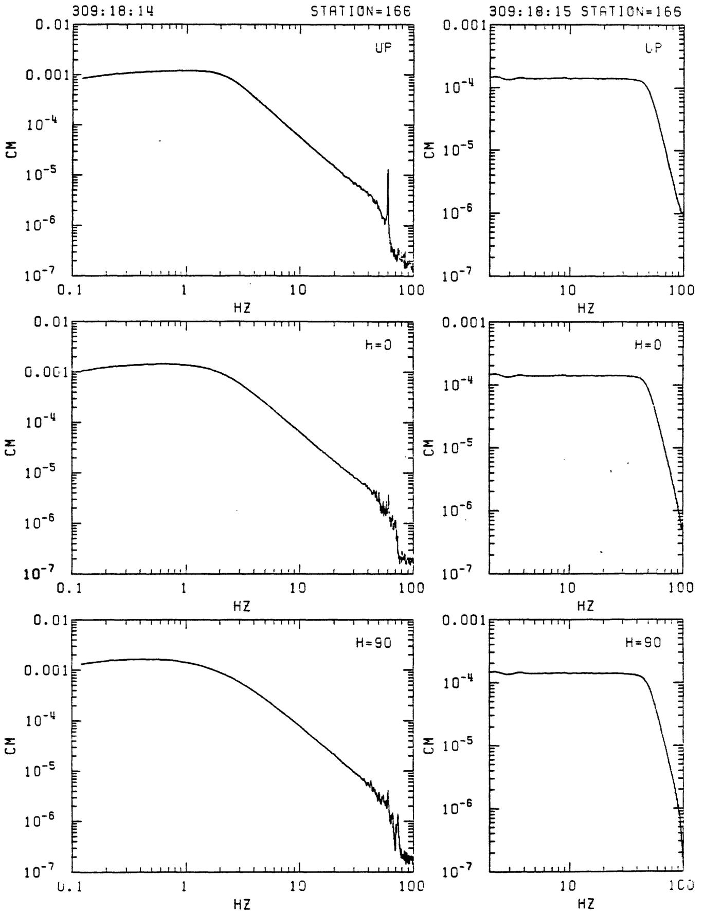
Figure C4. Station 166 in-situ velocity calibration spectra. Left: response to step in acceleration (seismometer mass released from rest at offset position). Right: response to delta function in velocity (voltage impulse applied to recorder input). From top: vertical, N33W and N57E.
