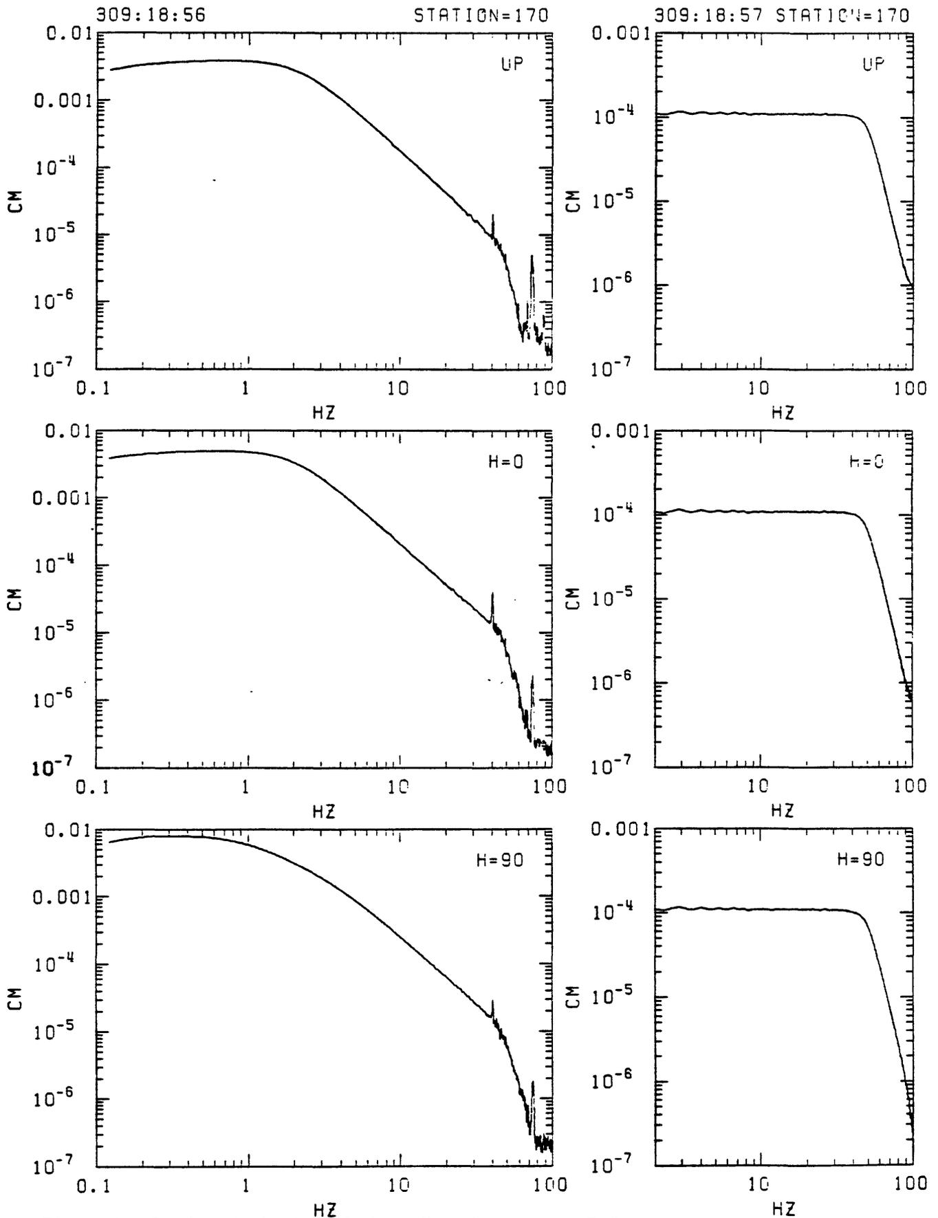
Figure C6. Station 170 in-situ velocity calibration spectra. Left: response to step in acceleration (seismometer mass released from rest at offset position). Right: response to delta function in velocity (voltage impulse applied to recorder input). From top: vertical, N33W and N57E.
