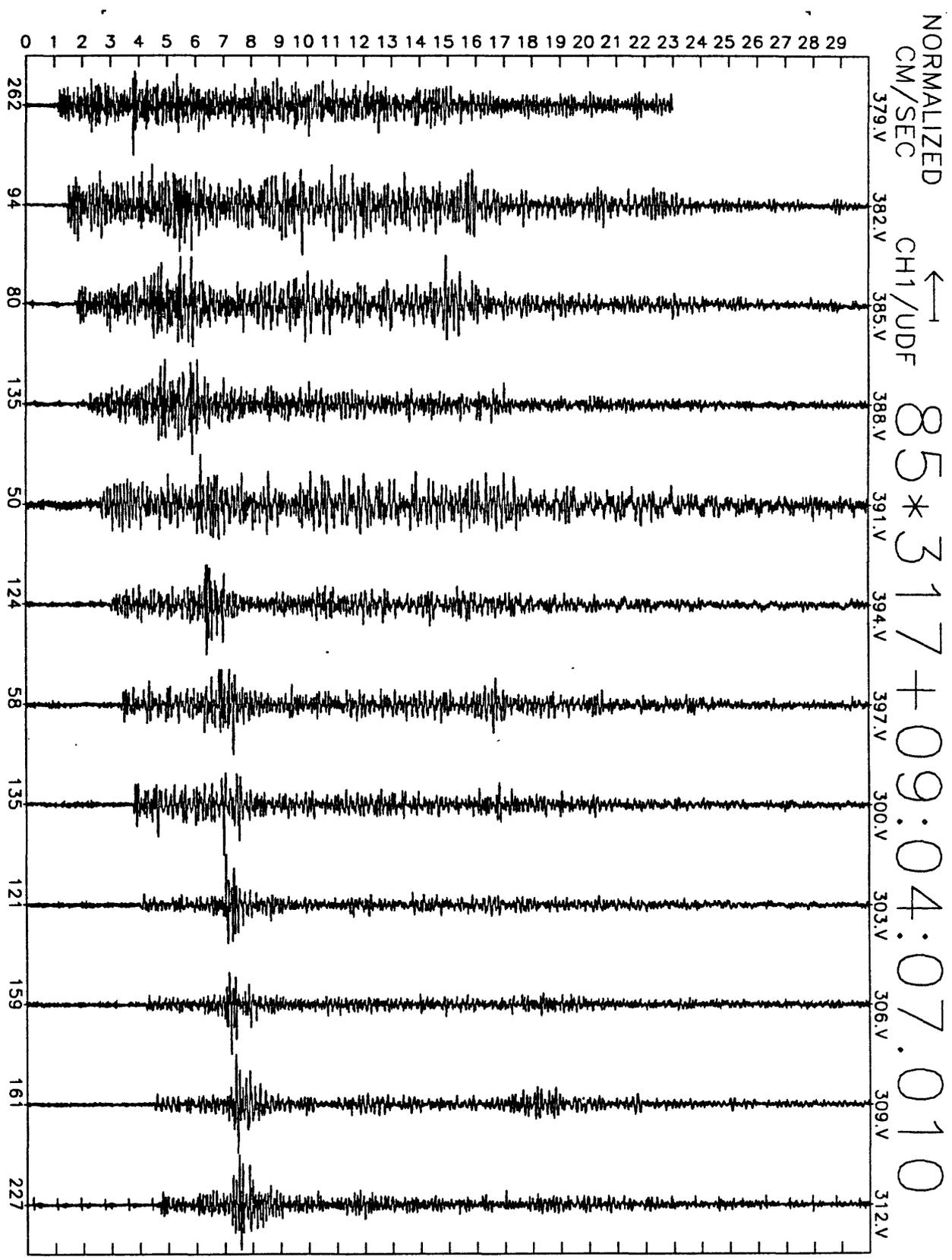
Figure A29(d), shot point 4B: 30 second vertical velocity record. Abscissa is labeled with maximum counts in record (multiply by  $\frac{10}{2^{24}-2^8} \approx 6 \times 10^{-7}$  to get cm/sec). Times are unreduced beginning at time indicated.
