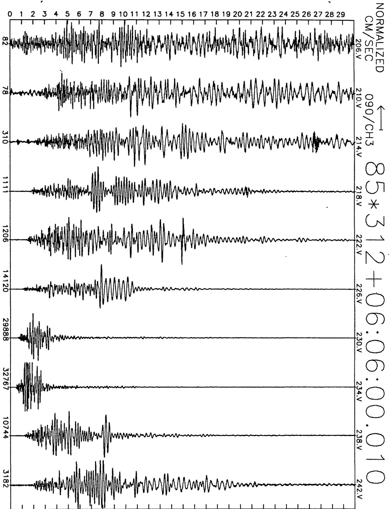
Figure A14(i), shot point 3: 30 second N110E velocity record. Abscissa is labeled with maximum counts in record (multiply by  $\frac{10}{274-26} \approx 6 \times 10^{-7}$  to get cm/sec). Times are unreduced beginning at time indicated.
