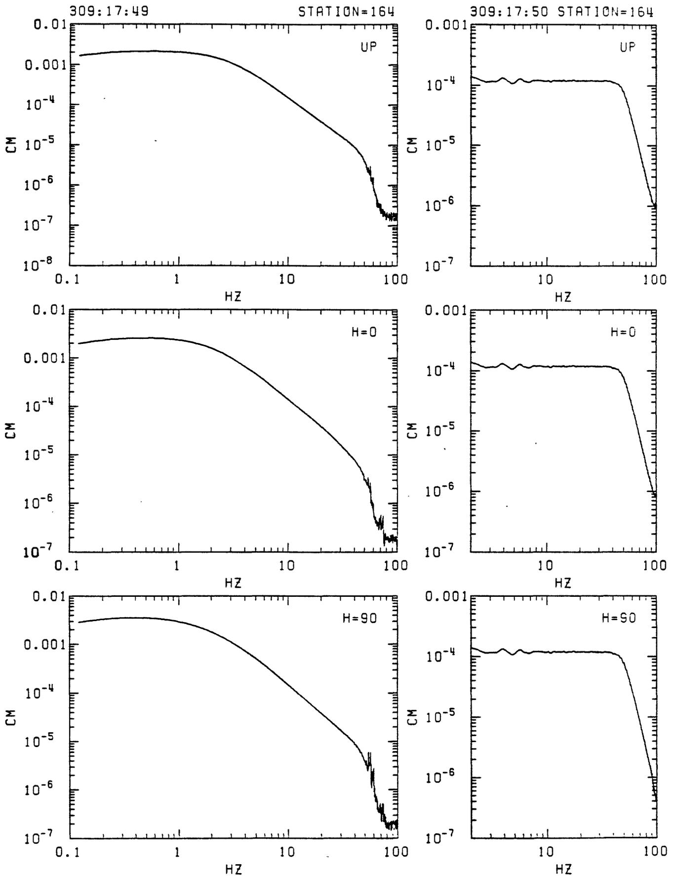
Figure C3. Station 164 in-situ velocity calibration spectra. Left: response to step in acceleration (seismometer mass released from rest at offset position). Right: response to delta function in velocity (voltage impulse applied to recorder input). From top: vertical, N33W and N57E.
