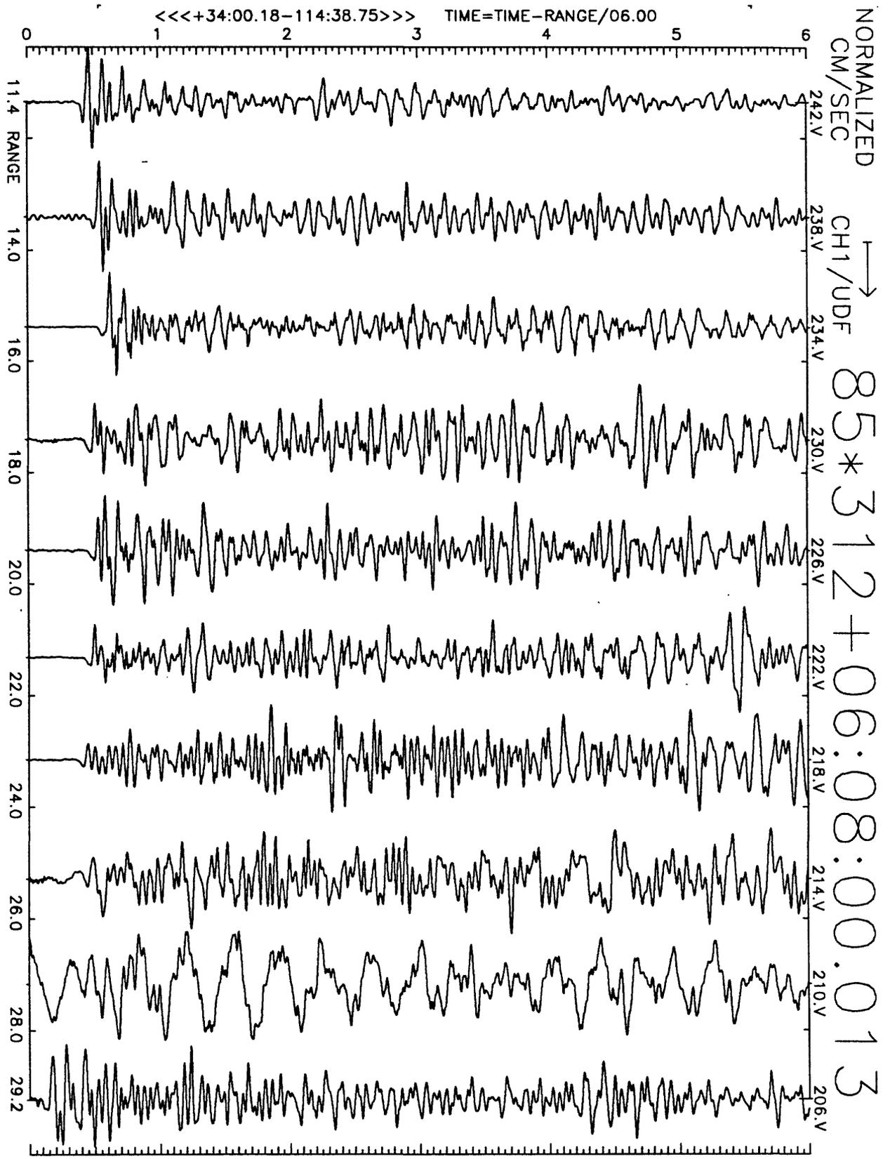
Figure A15(a), shot point 2: 6 second velocity record. Positive vertical motion is to right. Abscissa is distance to shot point. Top of trace is labeled with station number. Times are reduced by 6 km/sec. Shot time is indicated.
