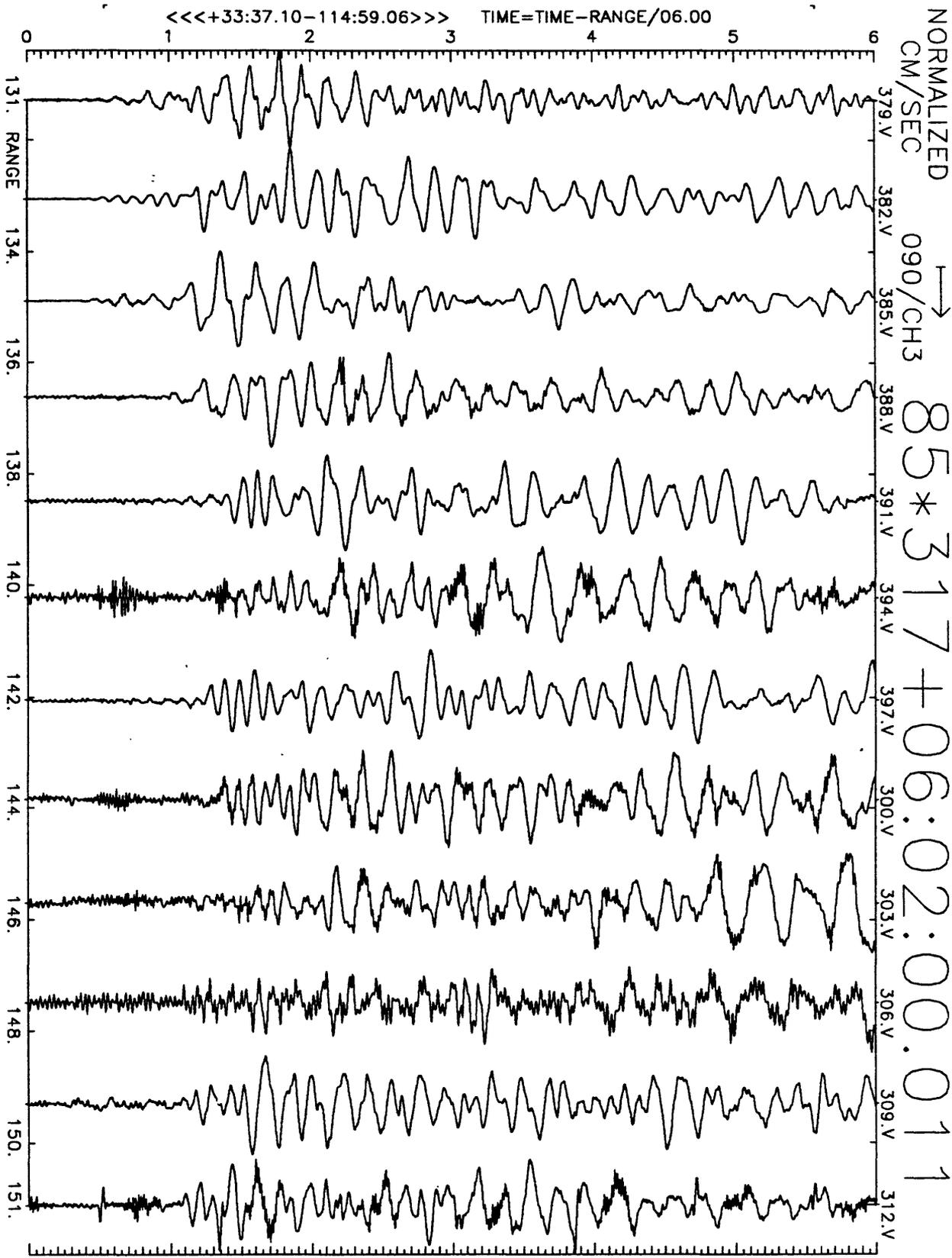
Figure A23(c), shot point 14: 6 second velocity record. Positive N115E motion is to right. Abscissa is distance to shot point. Top of trace is labeled with station number. Times are reduced by 6 km/sec. Shot time is indicated.
