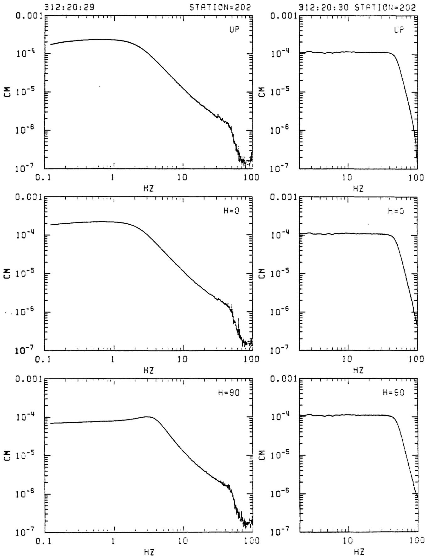
Figure C11. Station 202 in-situ velocity calibration spectra. Left: response to step in acceleration (seismometer mass released from rest at offset position). Right: response to delta function in velocity (voltage impulse applied to recorder input). From top: vertical, N20E and N110E.
