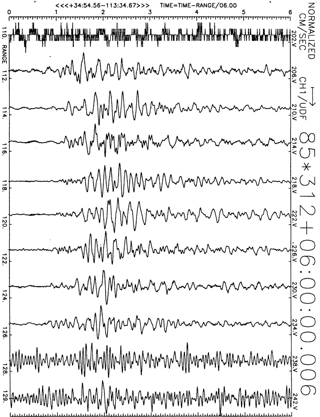
Figure A11(a), shot point 12: 6 second velocity record. Positive vertical motion is to right. Abscissa is distance to shot point. Top of trace is labeled with station number. Times are reduced by 6 km/sec. Shot time is indicated.
