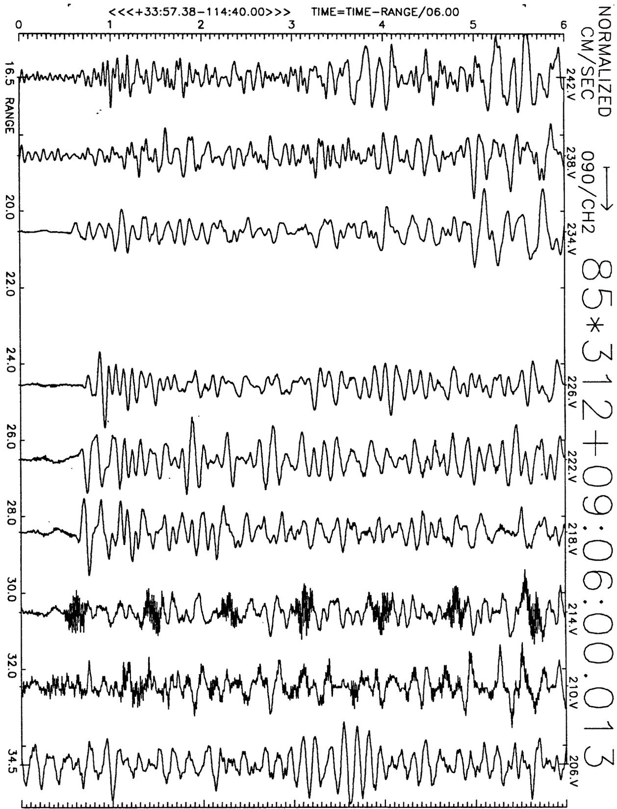
Figure A21(b), shot point 1X: 6 second velocity record. Positive N20E motion is to right. Abscissa is distance to shot point. Top of trace is labeled with station number. Times are reduced by 6 km/sec. Shot time is indicated.
