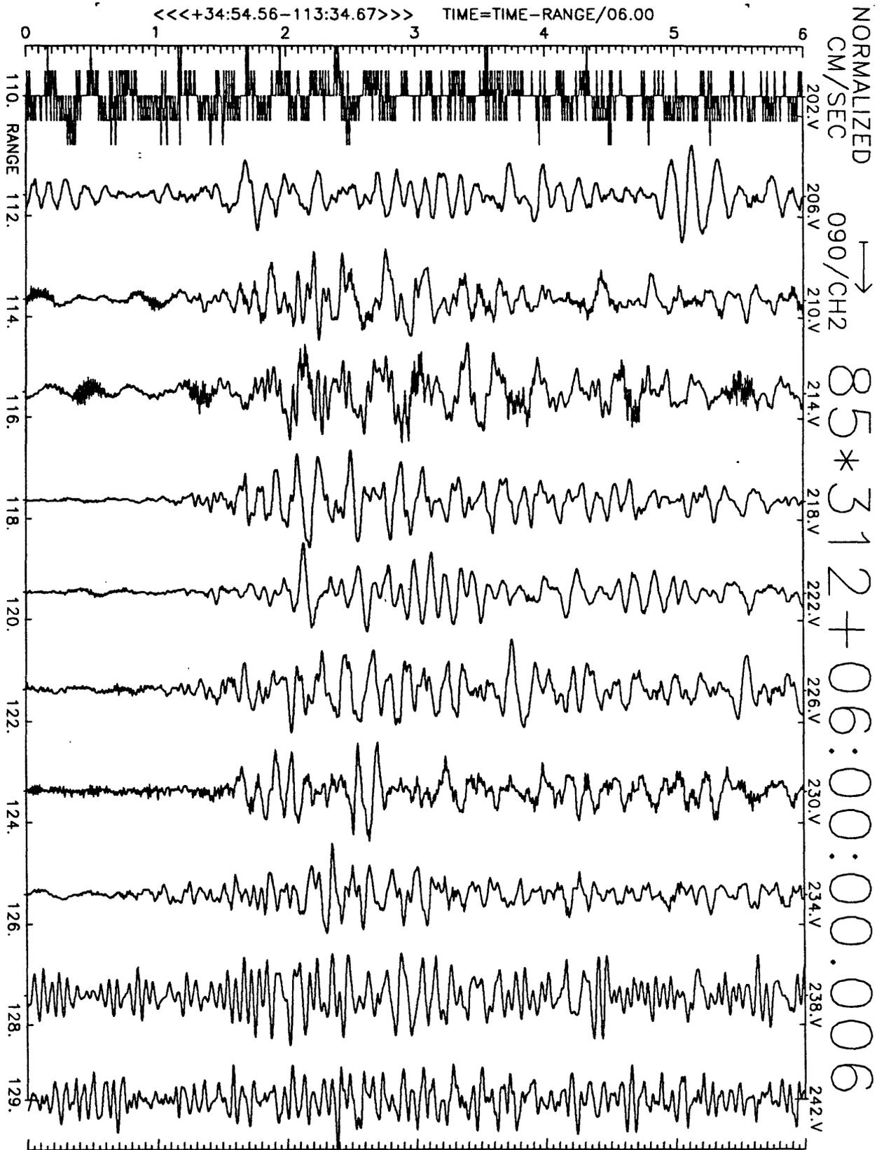
Figure A11(b), shot point 12: 6 second velocity record. Positive N20E motion is to right. Abscissa is distance to shot point. Top of trace is labeled with station number. Times are reduced by 6 km/sec. Shot time is indicated.
