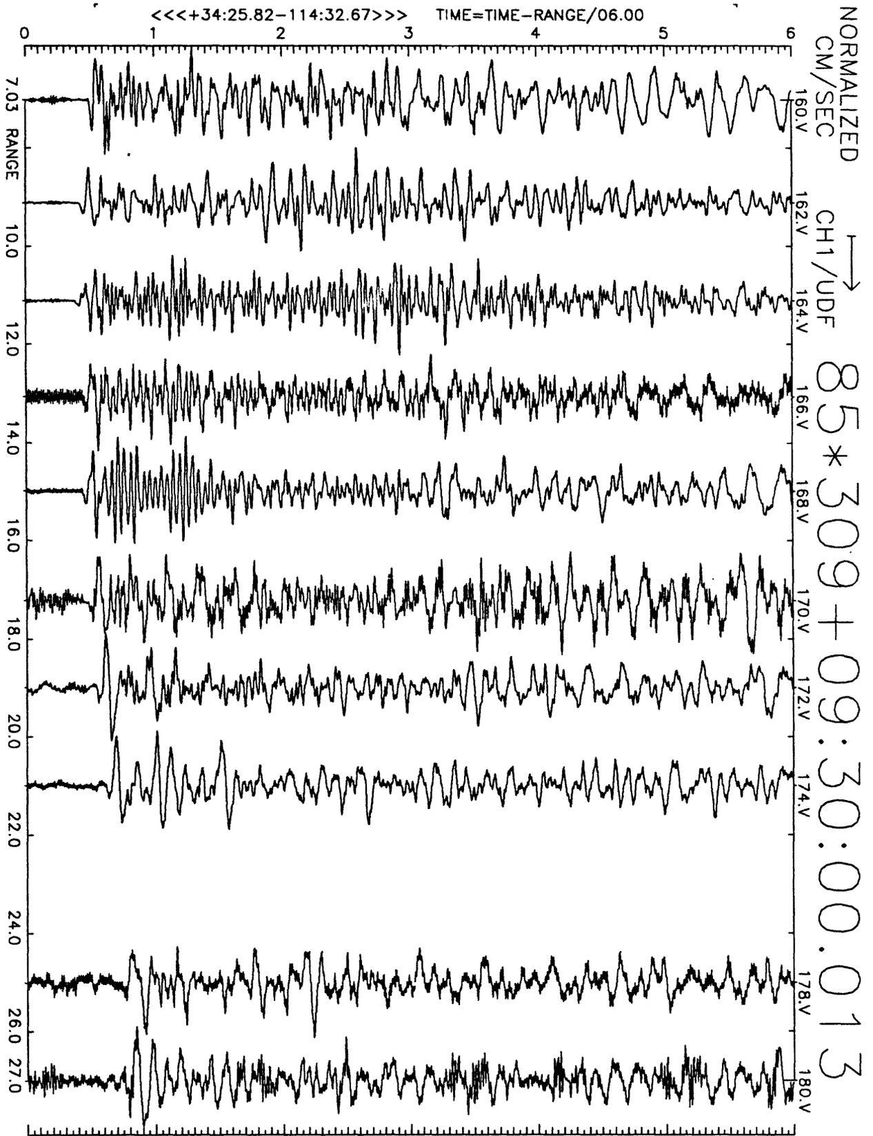
Figure A10(a), shot point 9X': 6 second velocity record. Positive vertical motion is to right. Abscissa is distance to shot point. Top of trace is labeled with station number. Times are reduced by 6 km/sec. Shot time is indicated.
