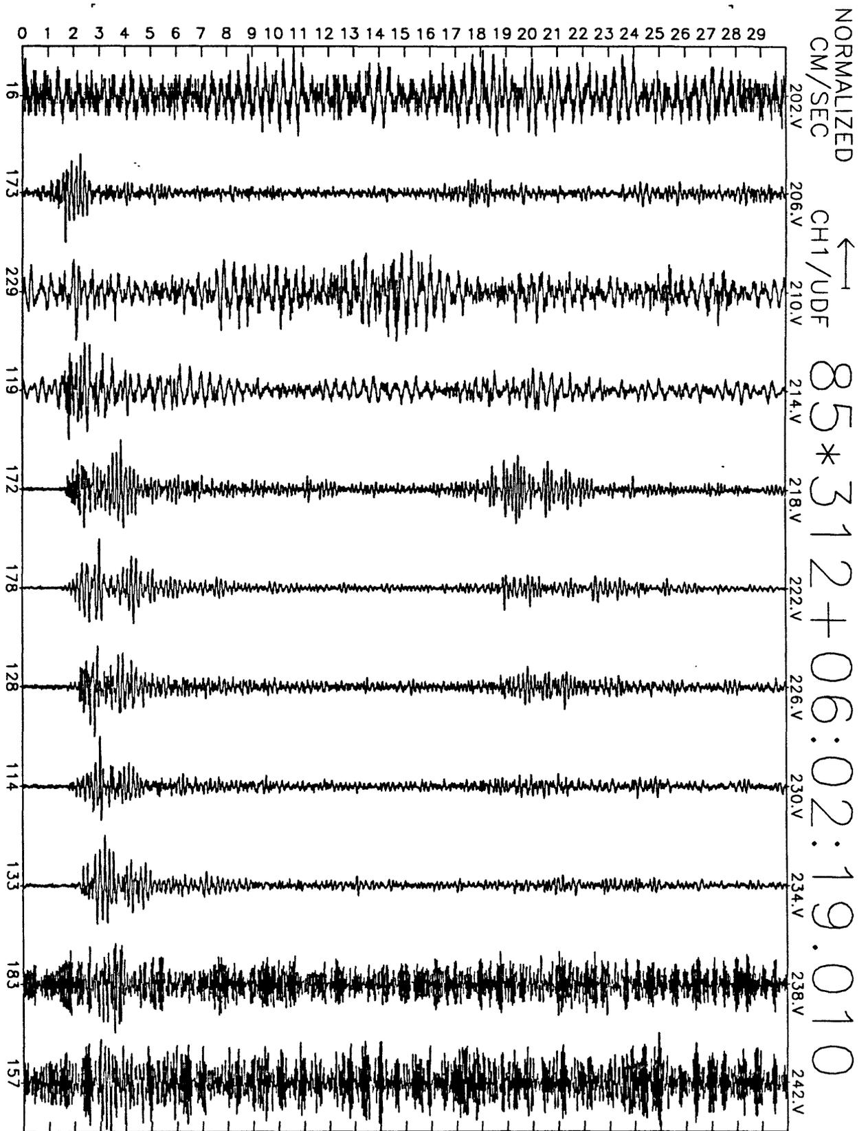
Figure A12(d), shot point 11: 30 second vertical velocity record. Abscissa is labeled with maximum counts in record (multiply by  $\frac{10}{2^{24}-2^8} \approx 6 \times 10^{-7}$  to get cm/sec). Times are unreduced beginning at time indicated.
