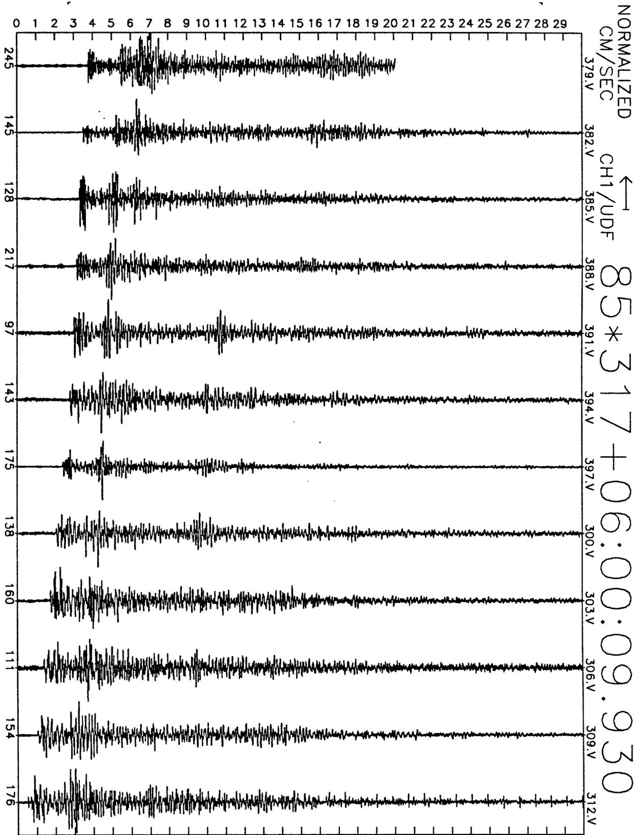
Figure A22(e), shot point 12: 30 second N25E velocity record. Abscissa is labeled with maximum counts in record (multiply by  $\frac{10}{2^{24}-2^8} \approx 6 \times 10^{-7}$  to get cm/sec). Times are unreduced beginning at time indicated.
