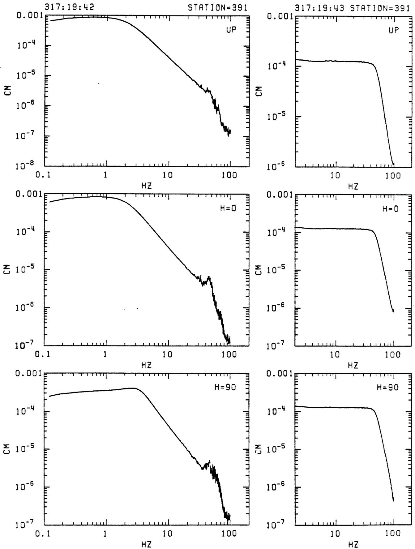
Figure C24. Station 391 in-situ velocity calibration spectra. Left: response to step in acceleration (seismometer mass released from rest at offset position). Right: response to delta function in velocity (voltage impulse applied to recorder input). From top: vertical, N25E and N115E.
