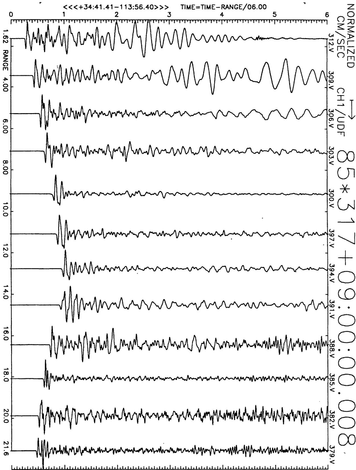
Figure A27(a), shot point 7: 6 second velocity record. Positive vertical motion is to right. Abscissa is distance to shot point. Top of trace is labeled with station number. Times are reduced by 6 km/sec. Shot time is indicated.
