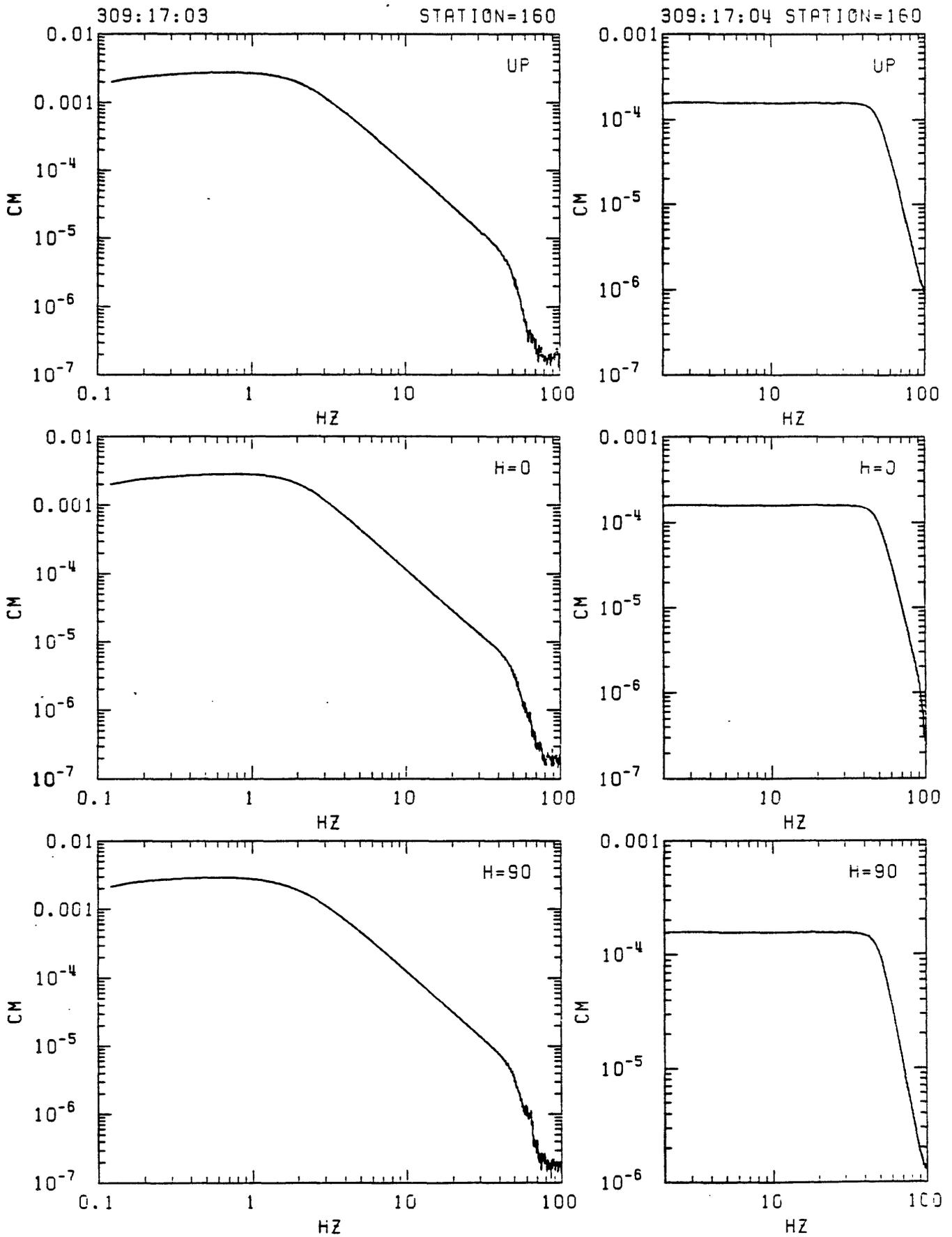
Figure C1. Station 160 in-situ velocity calibration spectra. Left: response to step in acceleration (seismometer mass released from rest at offset position). Right: response to delta function in velocity (voltage impulse applied to recorder input). From top: vertical, N33W and N57E.
