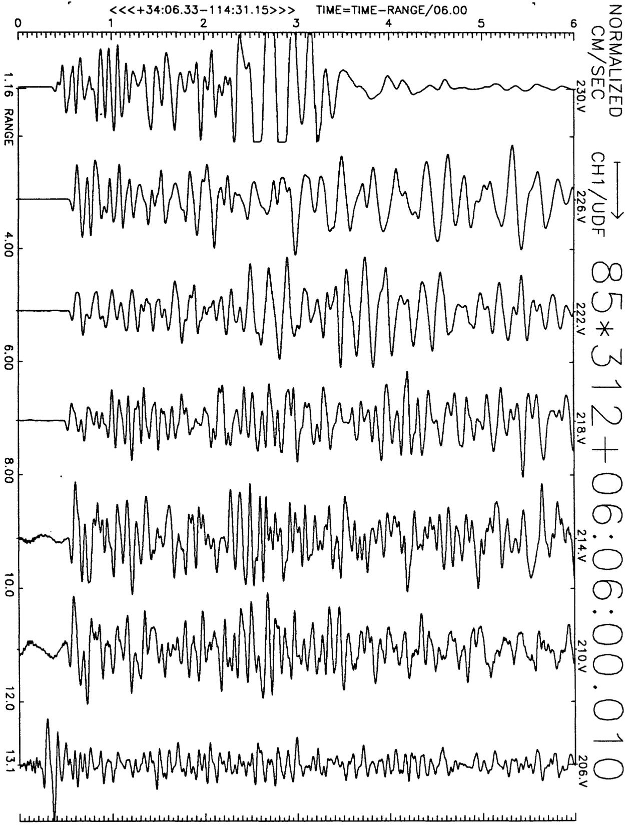
Figure A14(d), shot point 3, NE stations: 6 second velocity record. Positive vertical motion is to right. Abscissa is distance to shot point. Top of trace is labeled with station number. Times are reduced by 6 km/sec. Shot time is indicated.
