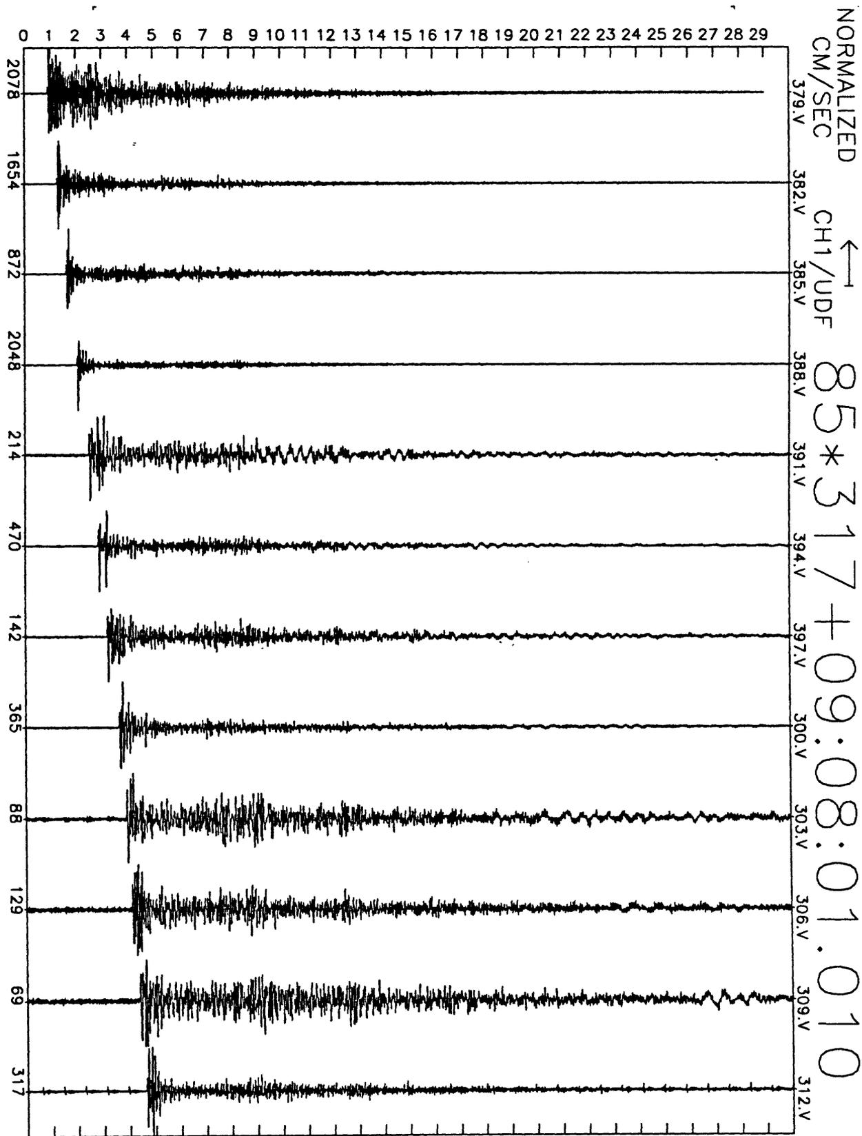
Figure A30(d), shot point 6: 30 second vertical velocity record. Abscissa is labeled with maximum counts in record (multiply by  $\frac{10}{2^{24}-2^8} \approx 6 \times 10^{-7}$  to get cm/sec). Times are unreduced beginning at time indicated.
