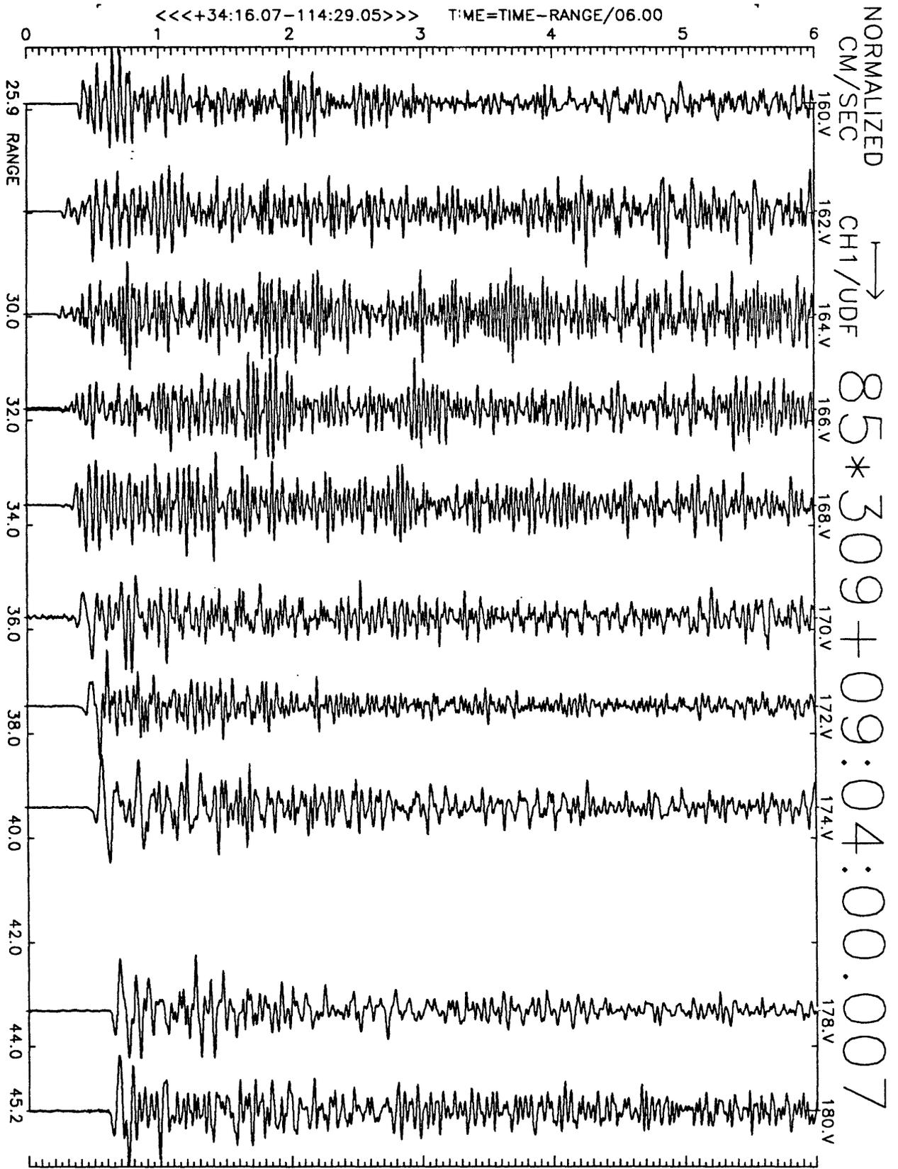
Figure A8(a), shot point 4A: 6 second velocity record. Positive vertical motion is to right. Abscissa is distance to shot point. Top of trace is labeled with station number. Times are reduced by 6 km/sec. Shot time is indicated.
