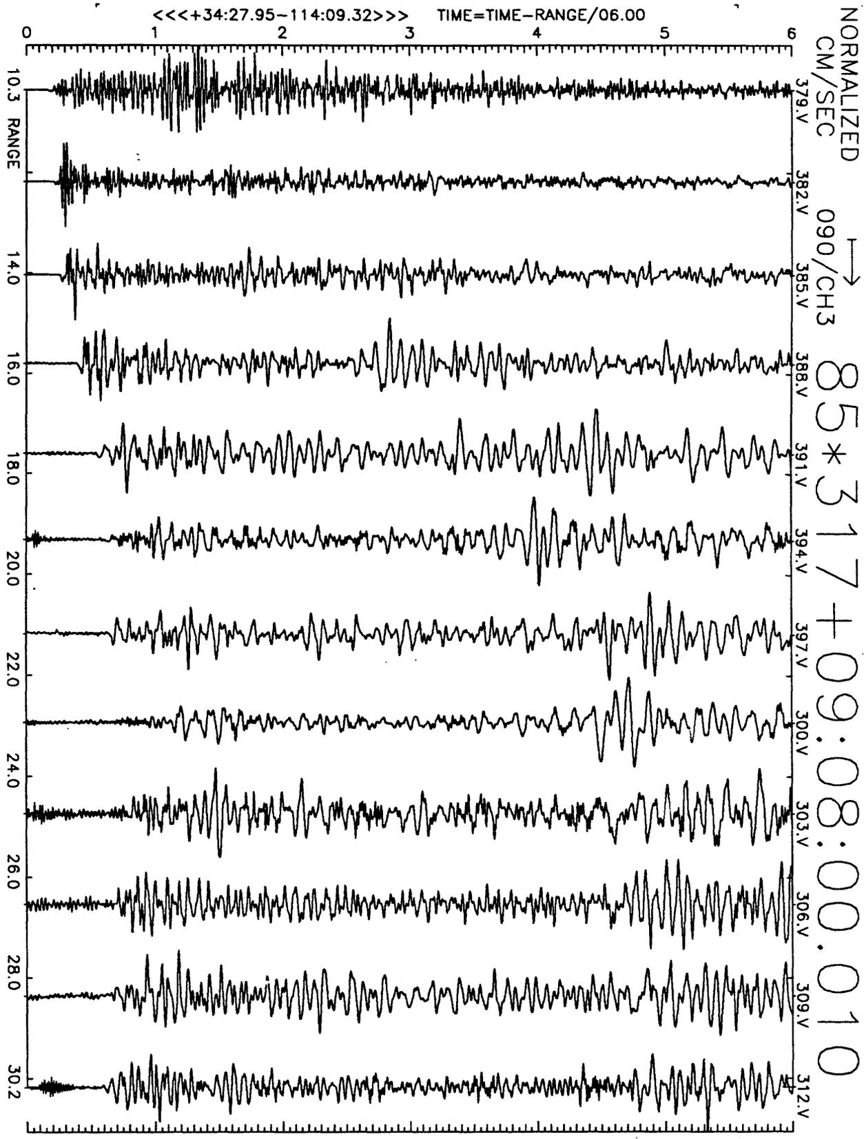
Figure A30(c), shot point 6: 6 second velocity record. Positive N115E motion is to right. Abscissa is distance to shot point. Top of trace is labeled with station number. Times are reduced by 6 km/sec. Shot time is indicated.
