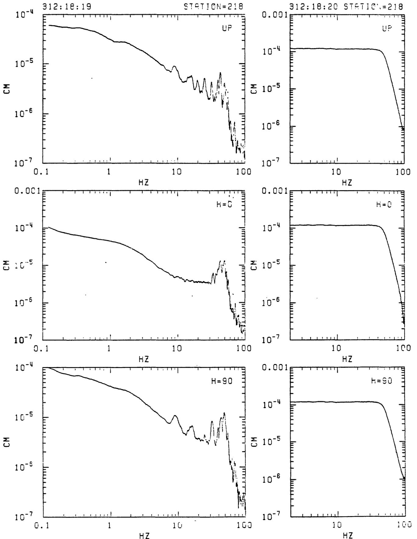
Figure C15. Station 218 in-situ velocity calibration spectra. Left: response to step in acceleration (seismometer mass released from rest at offset position). Right: response to delta function in velocity (voltage impulse applied to recorder input). From top: vertical, N20E and N110E.
