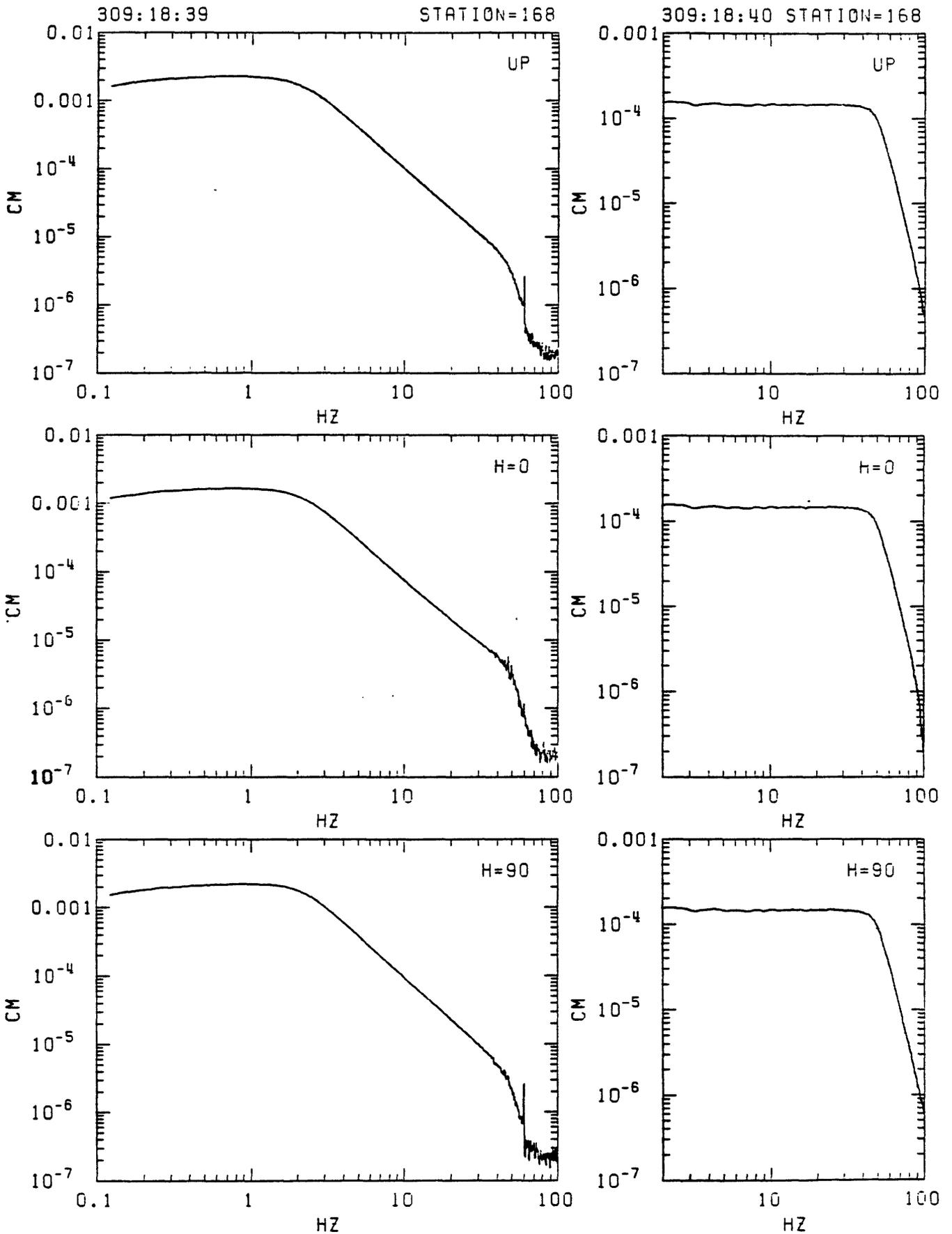
Figure C5. Station 168 in-situ velocity calibration spectra. Left: response to step in acceleration (seismometer mass released from rest at offset position). Right: response to delta function in velocity (voltage impulse applied to recorder input). From top: vertical, N33W and N57E.
