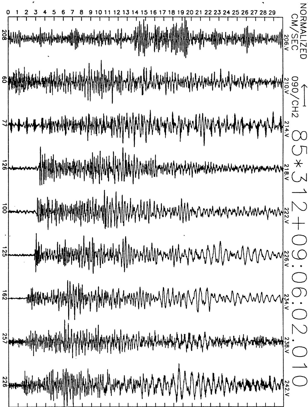
Figure A21(e), shot point 1X: 30 second N20E velocity record. Abscissa is labeled with maximum counts in record (multiply by  $\frac{10}{2^{24}-2^6} \approx 6 \times 10^{-7}$  to get cm/sec). Times are unreduced beginning at time indicated.
