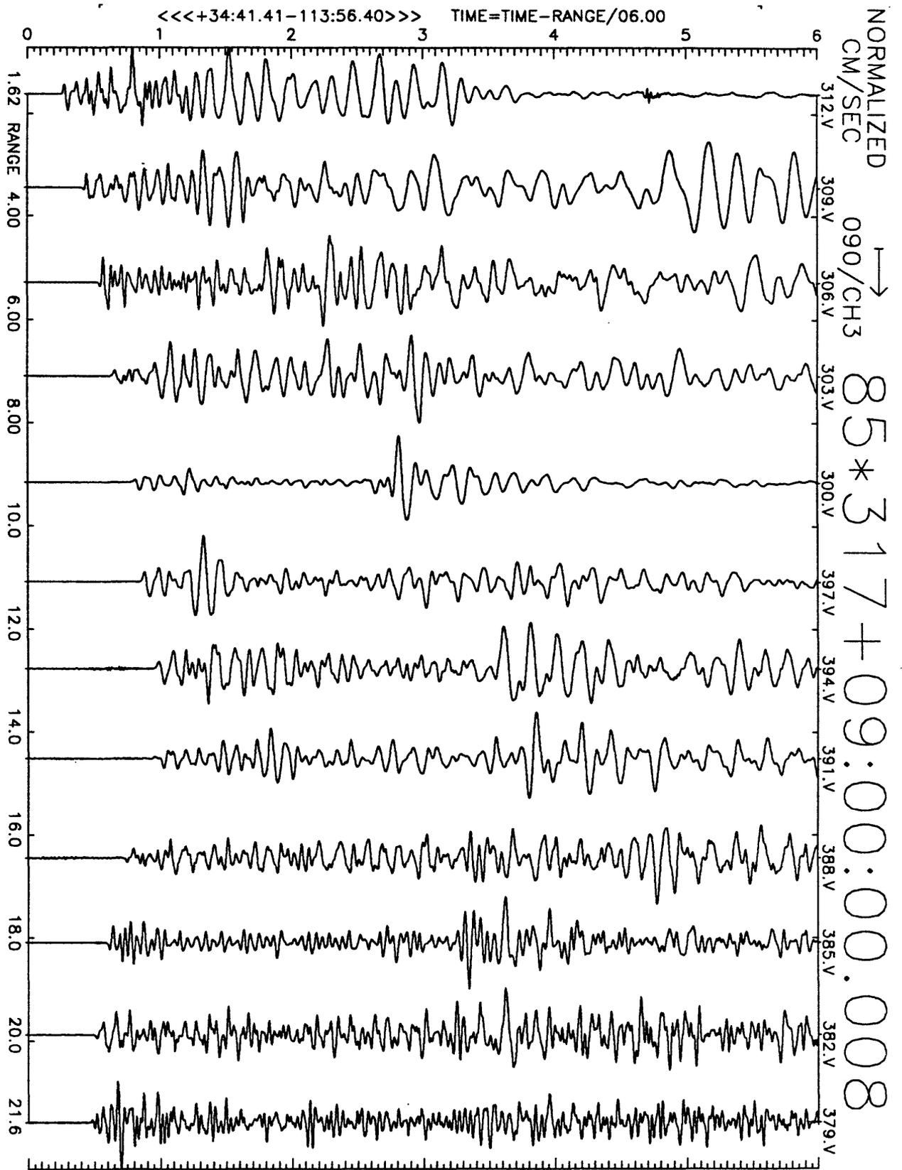
Figure A27(c), shot point 7: 6 second velocity record. Positive N115E motion is to right. Abscissa is distance to shot point. Top of trace is labeled with station number. Times are reduced by 6 km/sec. Shot time is indicated.
