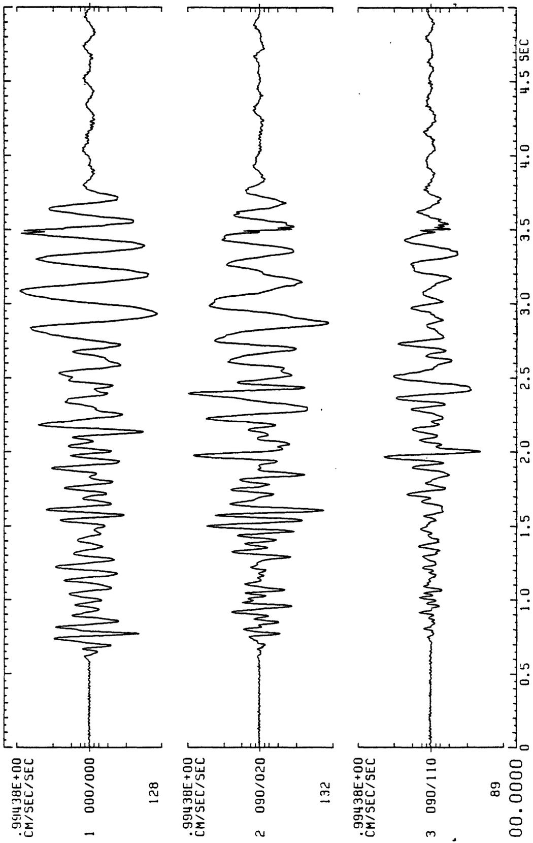
Figure B4(a), shot point 3': Three component accelerogram for station 230. Lower traces show horizontal motion. Azimuths are indicated immediately to the left of the traces. Start time is arbitrary.
