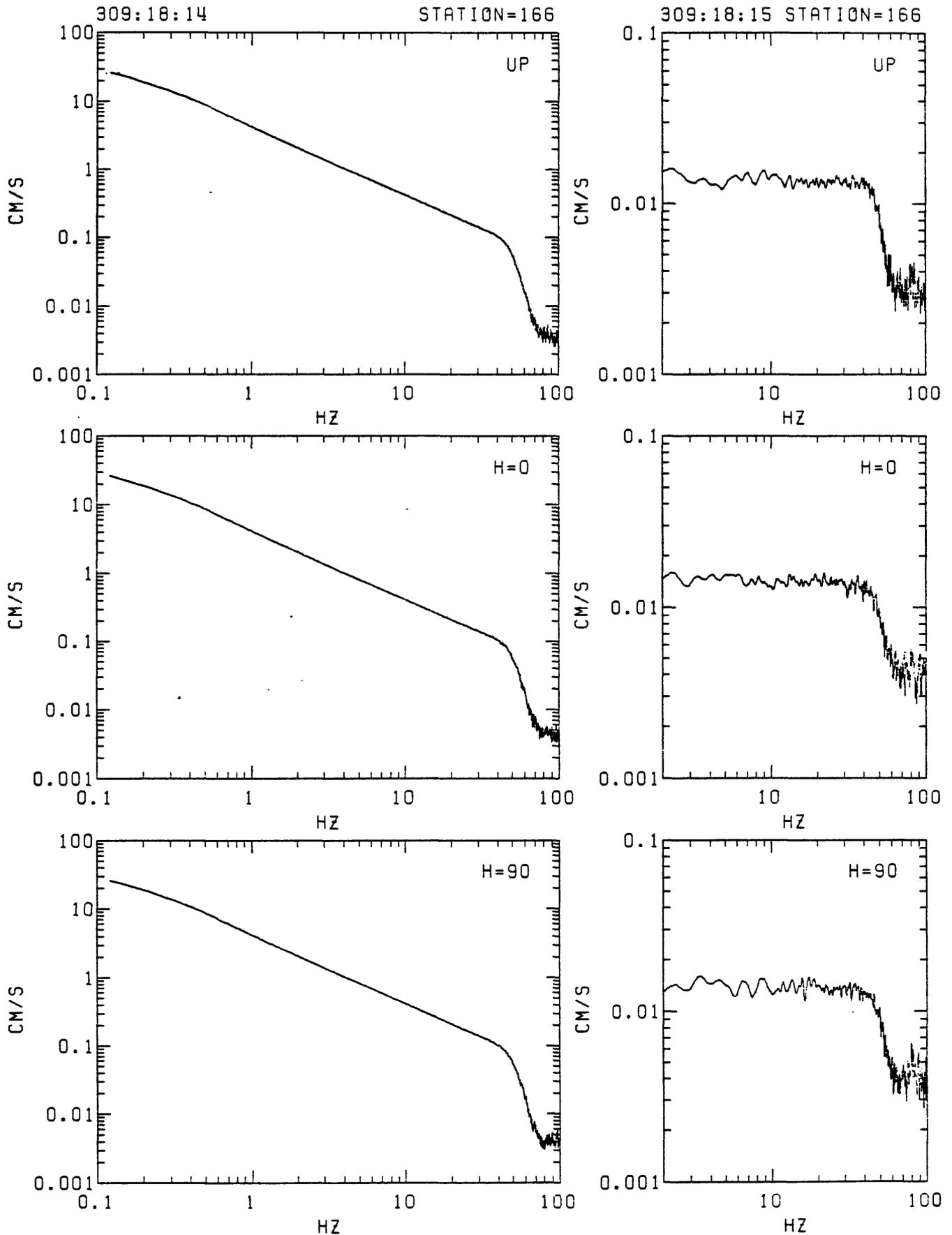
Figure D2. Station 166 in-situ 6db acceleration calibration spectra. Left: response to step in acceleration (reset FBA servo amplifier reference voltage from non-zero). Right: response to delta function in acceleration (voltage impulse applied to recorder input). From top: vertical, N33W and N57W.
