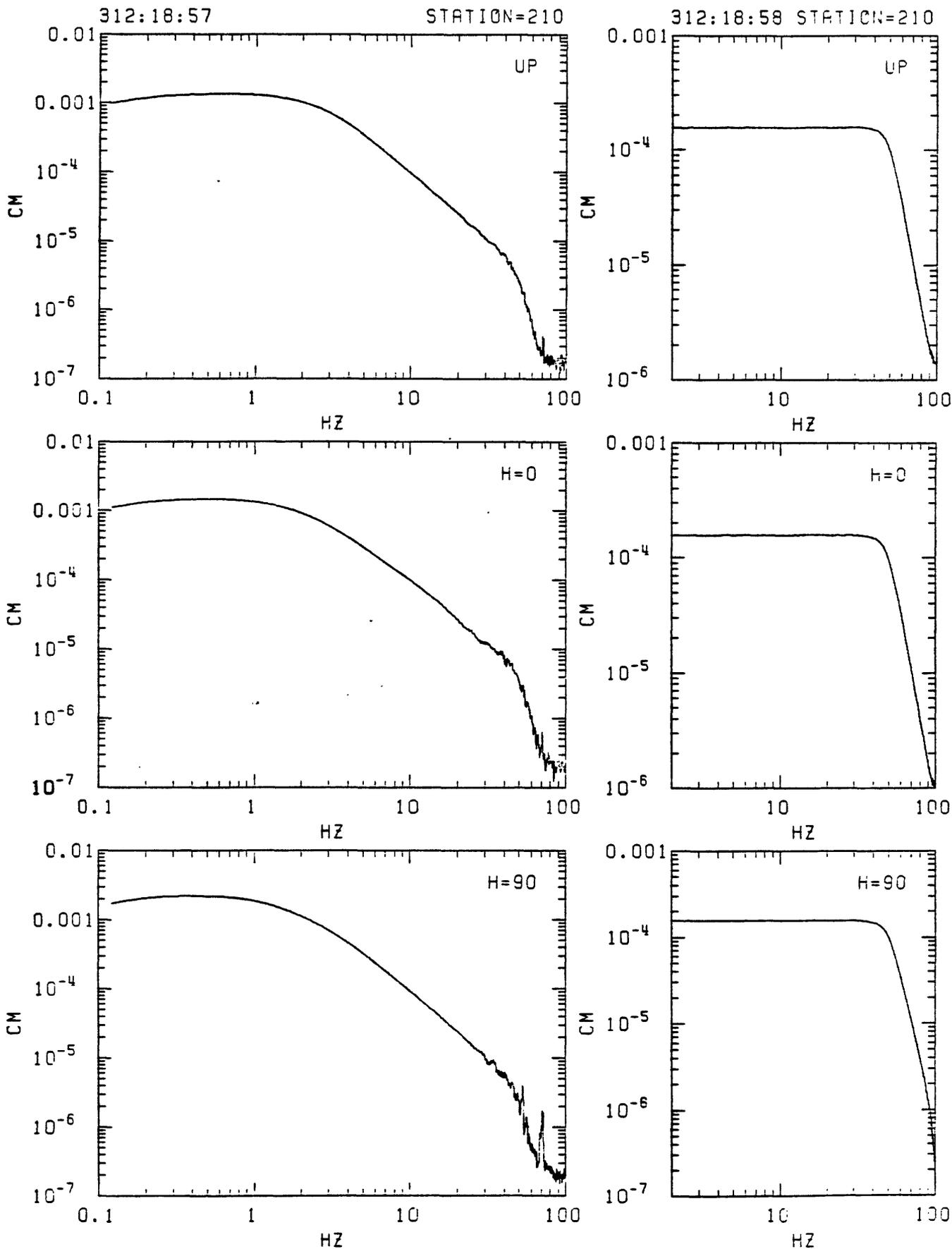
Figure C13. Station 210 in-situ velocity calibration spectra. Left: response to step in acceleration (seismometer mass released from rest at offset position). Right: response to delta function in velocity (voltage impulse applied to recorder input). From top: vertical, N20E and N110E.
