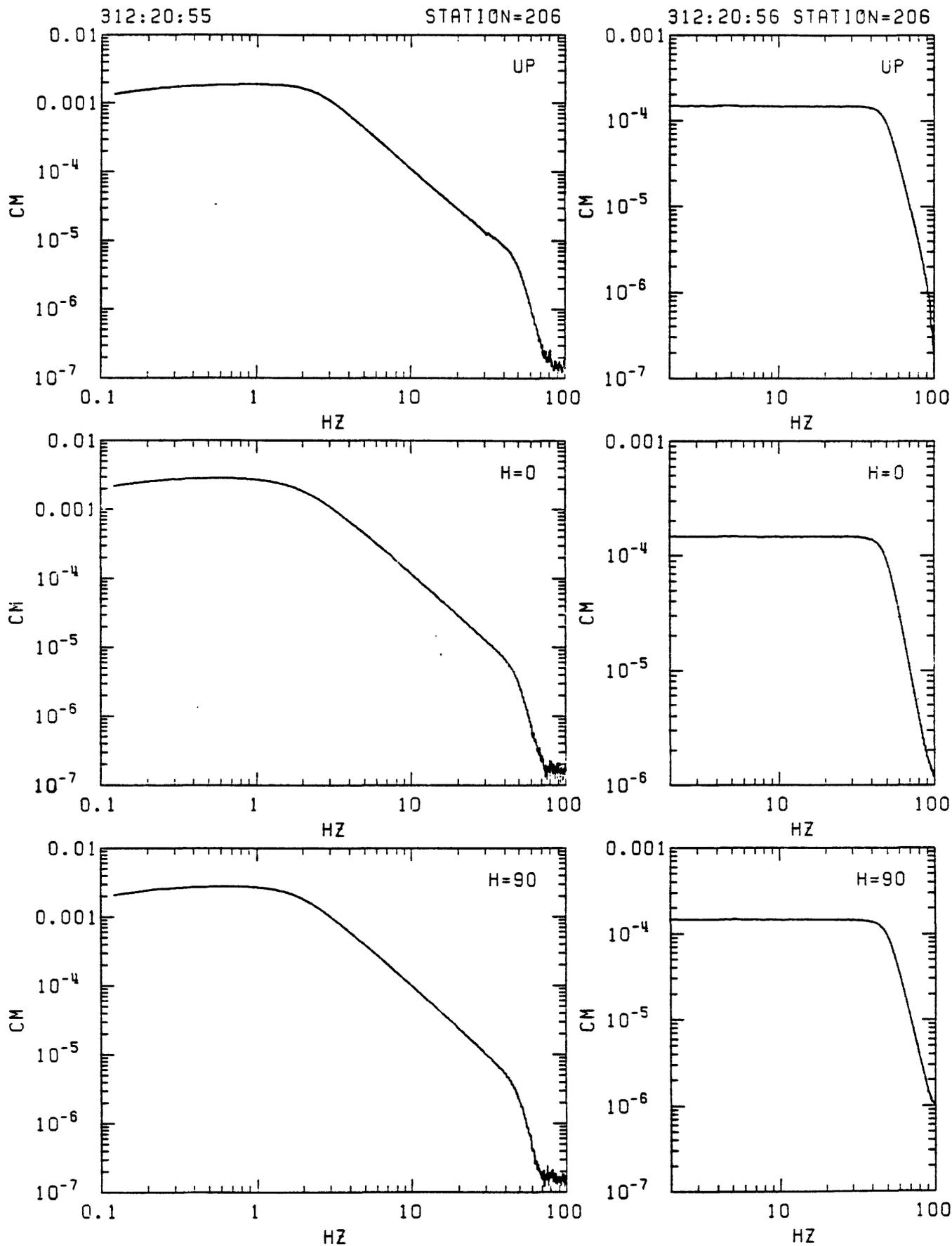
Figure C12. Station 206 in-situ velocity calibration spectra. Left: response to step in acceleration (seismometer mass released from rest at offset position). Right: response to delta function in velocity (voltage impulse applied to recorder input). From top: vertical, N20E and N110E.
