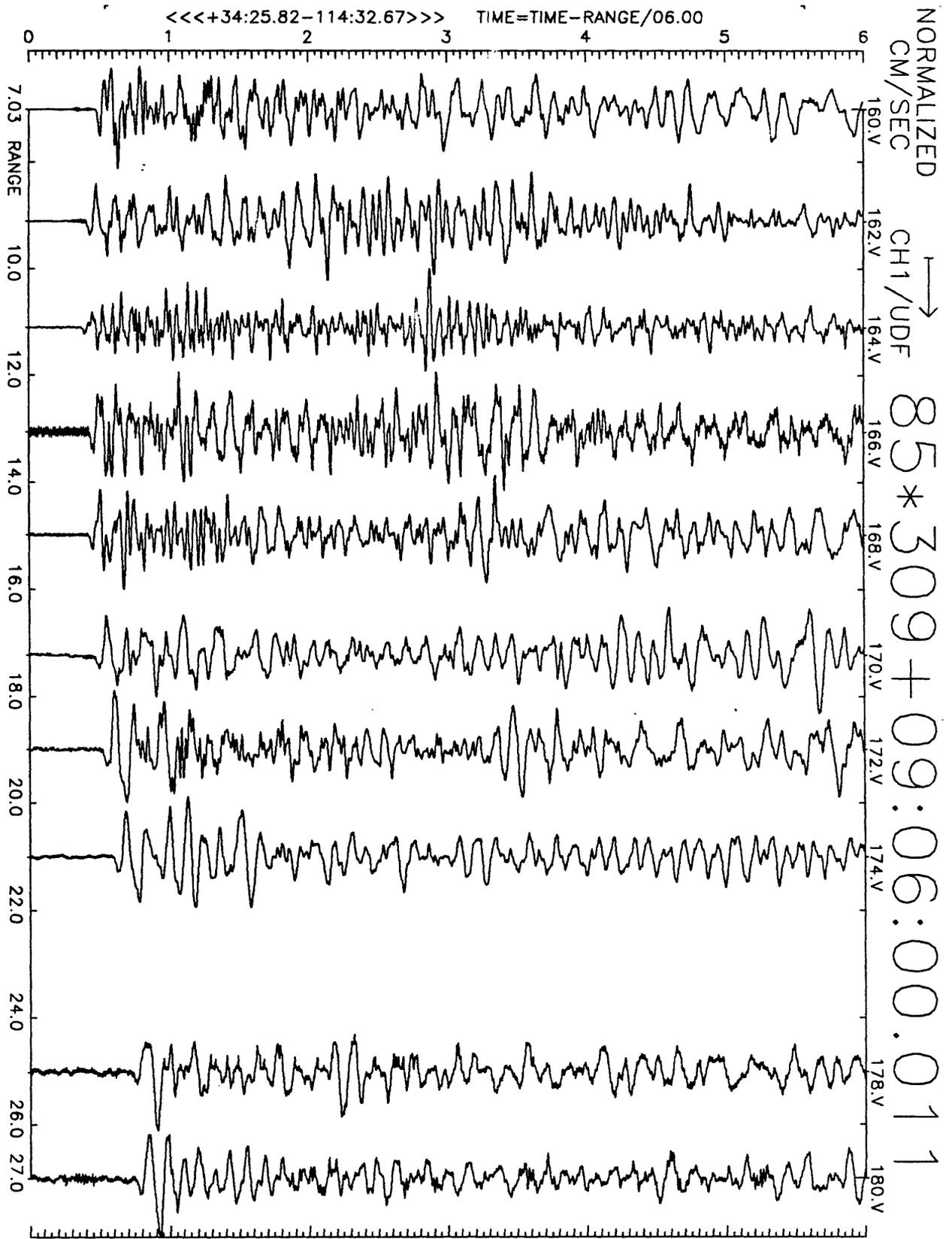
Figure A9(a), shot point 9X: 6 second velocity record. Positive vertical motion is to right. Abscissa is distance to shot point. Top of trace is labeled with station number. Times are reduced by 6 km/sec. Shot time is indicated.
