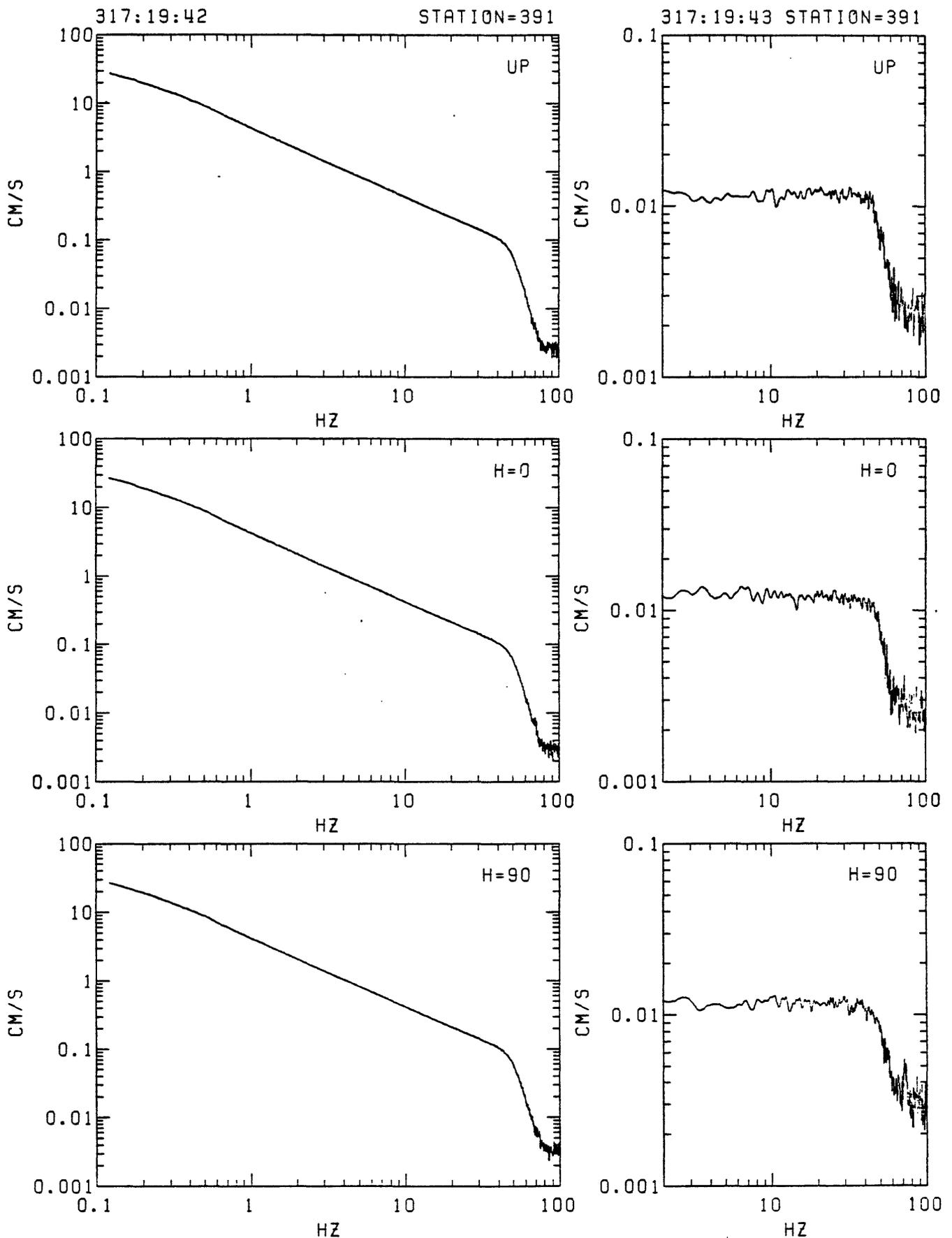
Figure D6. Station 391 in-situ 6db acceleration calibration spectra. Left: response to step in acceleration (reset FBA servo amplifier reference voltage from non-zero). Right: response to delta function in acceleration (voltage impulse applied to recorder input). From top: vertical, N25E and N115E.
