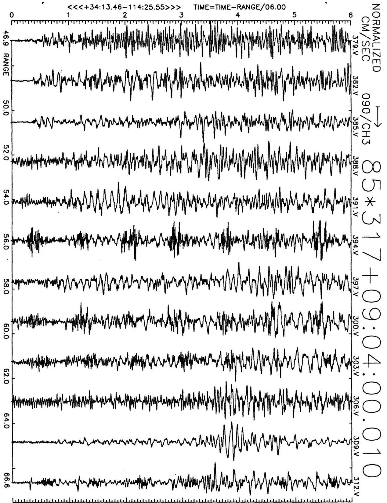
Figure A29(c), shot point 4B: 6 second velocity record. Positive N115E motion is to right. Abscissa is distance to shot point. Top of trace is labeled with station number. Times are reduced by 6 km/sec. Shot time is indicated.
