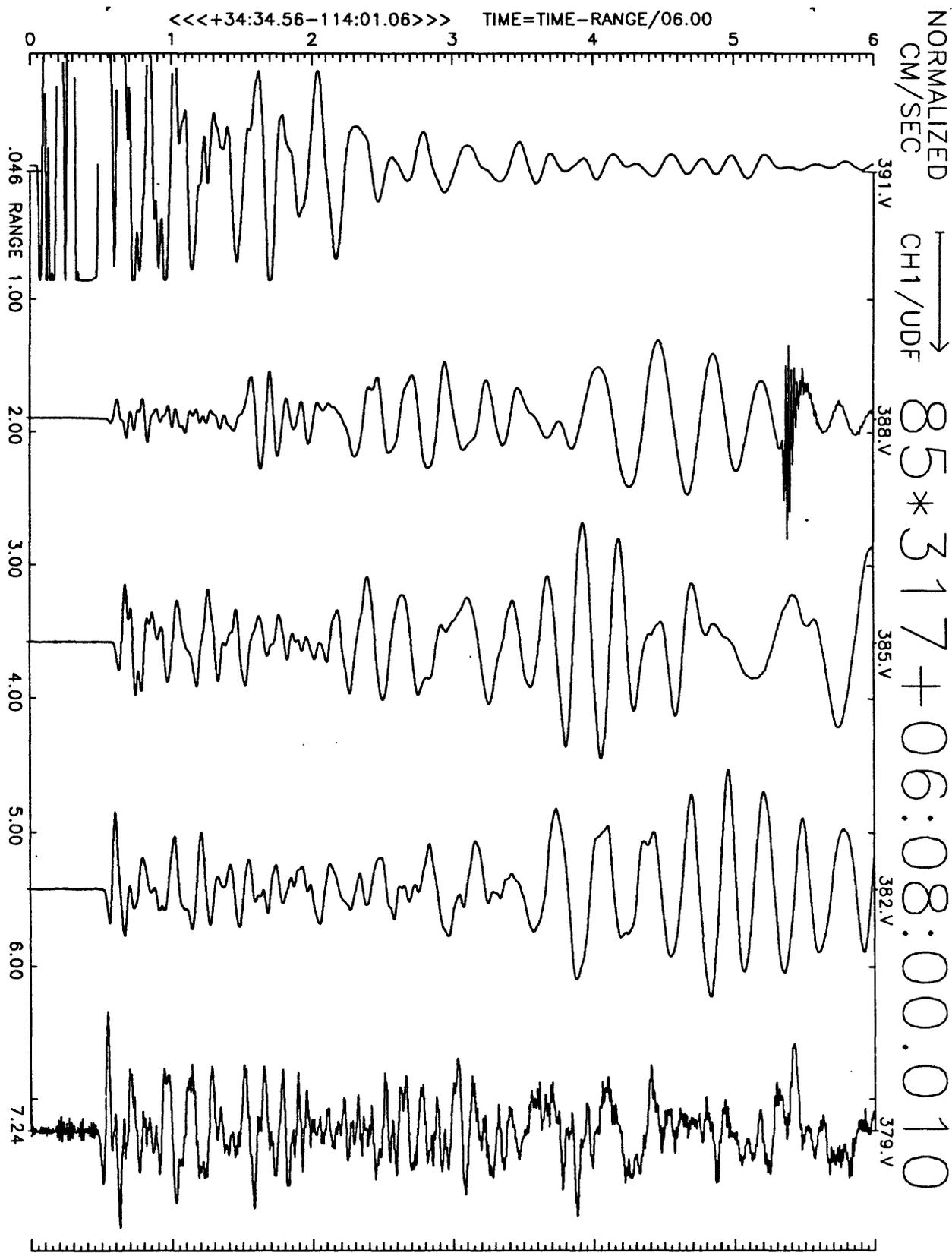
Figure A26(a), shot point 6X, SW stations: 6 second velocity record. Positive vertical motion is to right. Abscissa is distance to shot point. Top of trace is labeled with station number. Times are reduced by 6 km/sec. Shot time is indicated.
