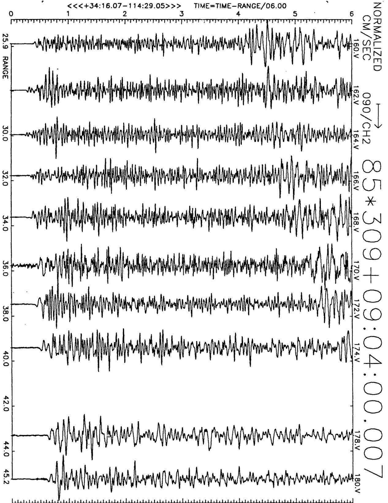
Figure A8(b), shot point 4A: 6 second velocity record. Positive N33W motion is to right. Abscissa is distance to shot point. Top of trace is labeled with station number. Times are reduced by 6 km/sec. Shot time is indicated.
