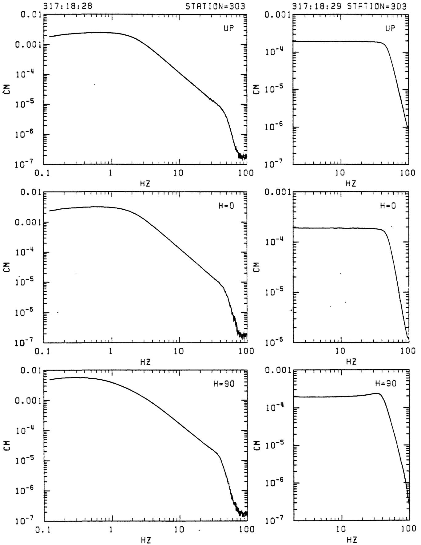
Figure C27. Station 303 in-situ velocity calibration spectra. Left: response to step in acceleration (seismometer mass released from rest at offset position). Right: response to delta function in velocity (voltage impulse applied to recorder input). From top: vertical, N25E and N115E.
