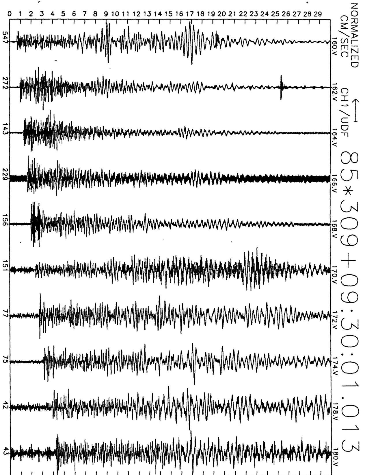
Figure A10(d), shot point 9X': 30 second vertical velocity record. Abscissa is labeled with maximum counts in record (multiply by  $\frac{10}{2^{24}-2^8} \approx 6 \times 10^{-7}$  to get cm/sec). Times are unreduced beginning at time indicated.
