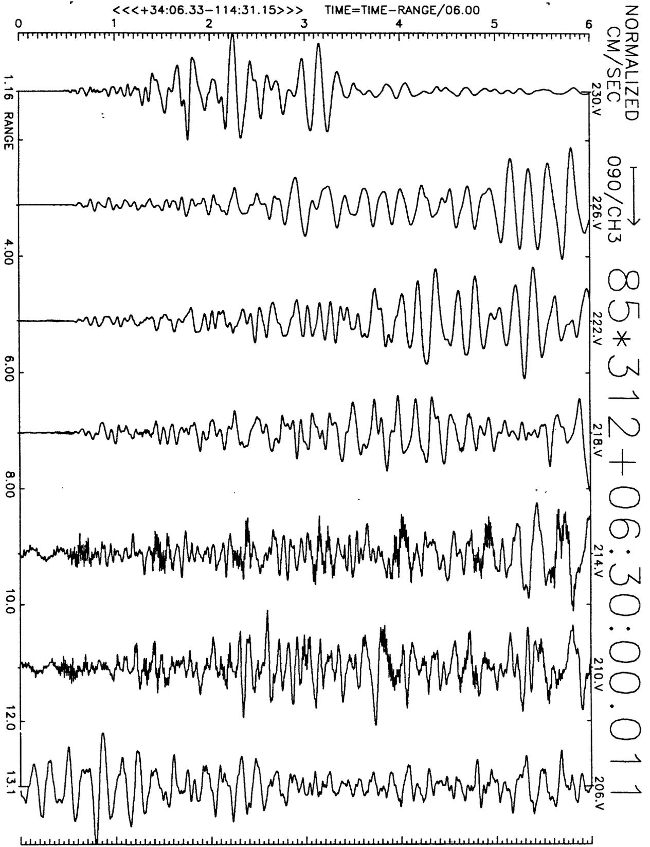
Figure A16(f), shot point 3', NE stations: 6 second velocity record. Positive N110E motion is to right. Abscissa is distance to shot point. Top of trace is labeled with station number. Times are reduced by 6 km/sec. Shot time is indicated.
