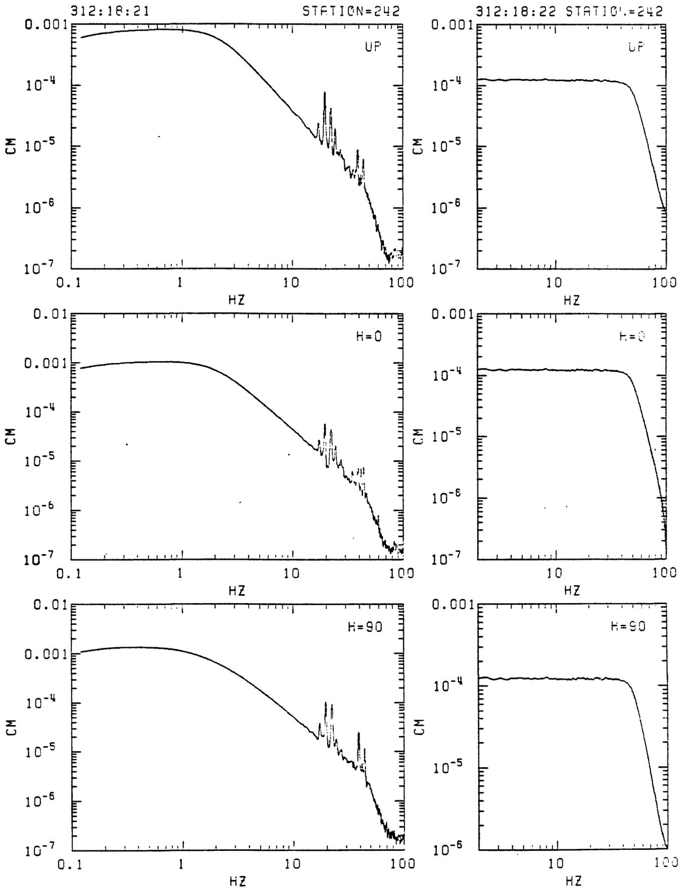
Figure C19. Station 242 in-situ velocity calibration spectra. Left: response to step in acceleration (seismometer mass released from rest at offset position). Right: response to delta function in velocity (voltage impulse applied to recorder input). From top: vertical, N20E and N110E.
