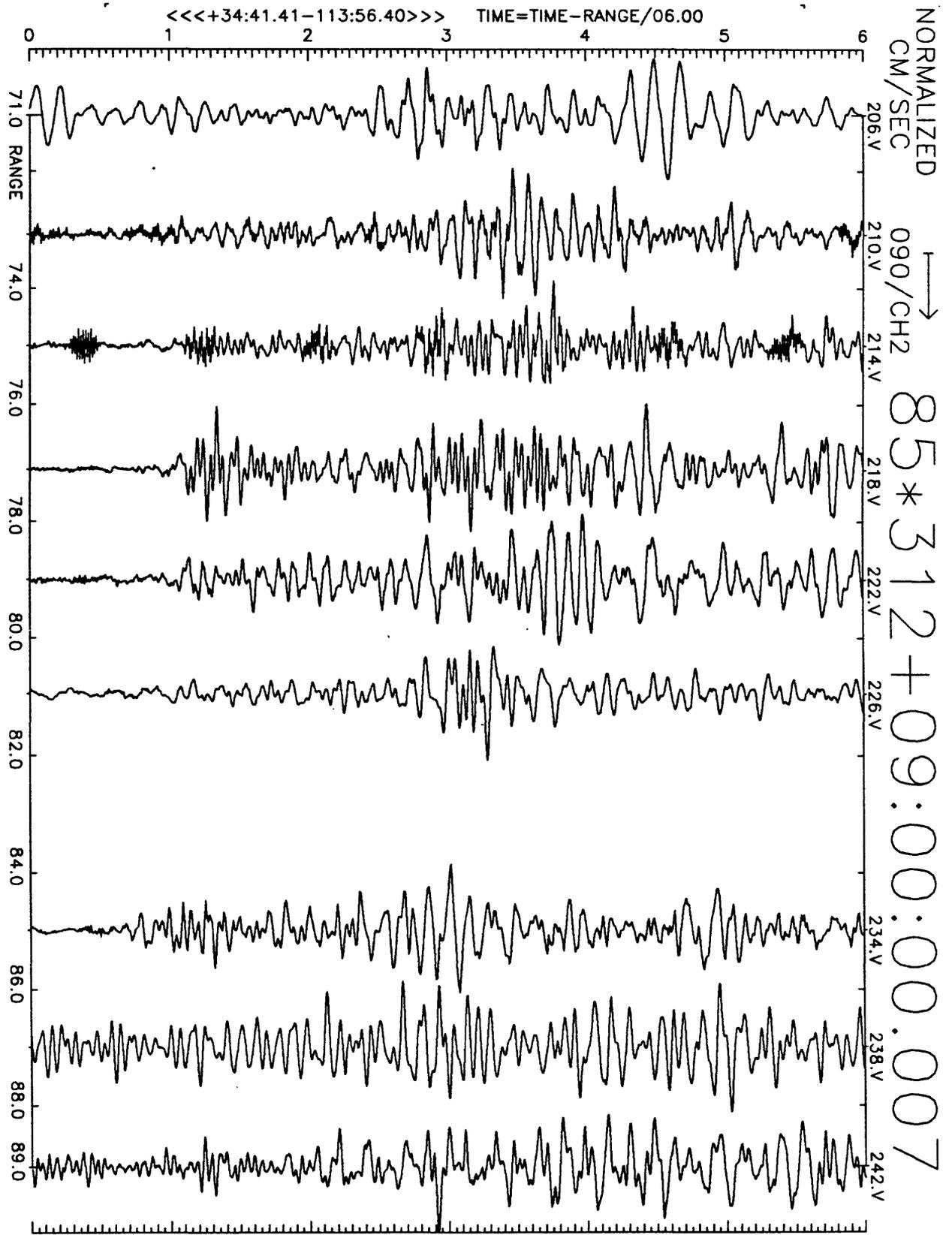
Figure A18(b), shot point 7: 6 second velocity record. Positive N20E motion is to right. Abscissa is distance to shot point. Top of trace is labeled with station number. Times are reduced by 6 km/sec. Shot time is indicated.
