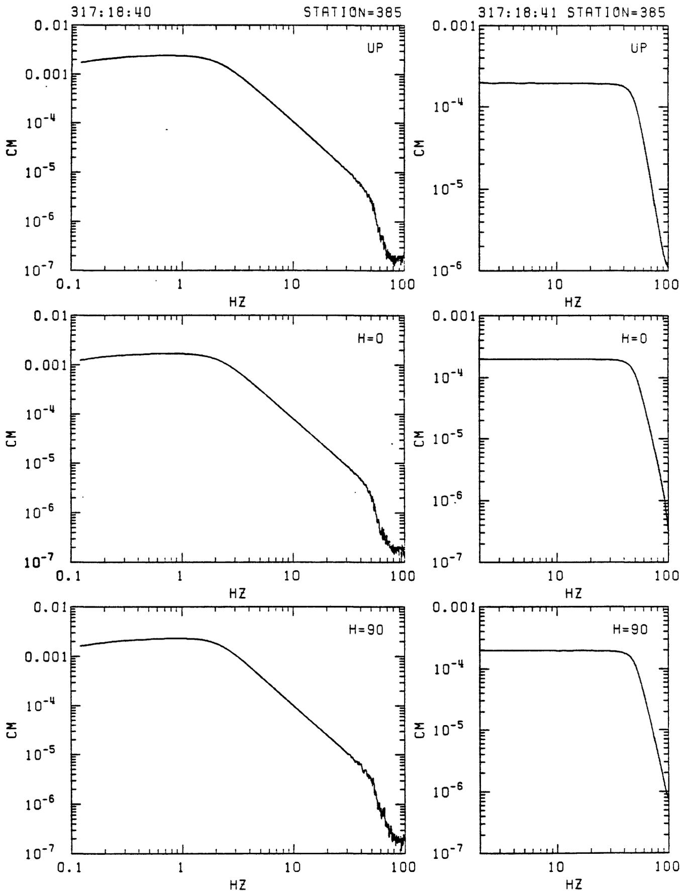
Figure C22. Station 385 in-situ velocity calibration spectra. Left: response to step in acceleration (seismometer mass released from rest at offset position). Right: response to delta function in velocity (voltage impulse applied to recorder input). From top: vertical, N25E and N115E.
