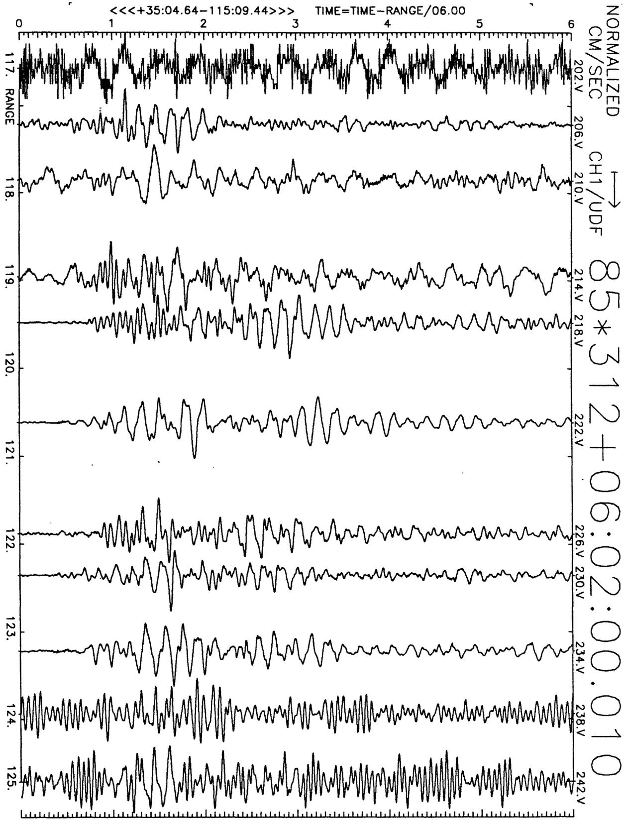
Figure A12(a), shot point 11: 6 second velocity record. Positive vertical motion is to right. Abscissa is distance to shot point. Top of trace is labeled with station number. Times are reduced by 6 km/sec. Shot time is indicated.
