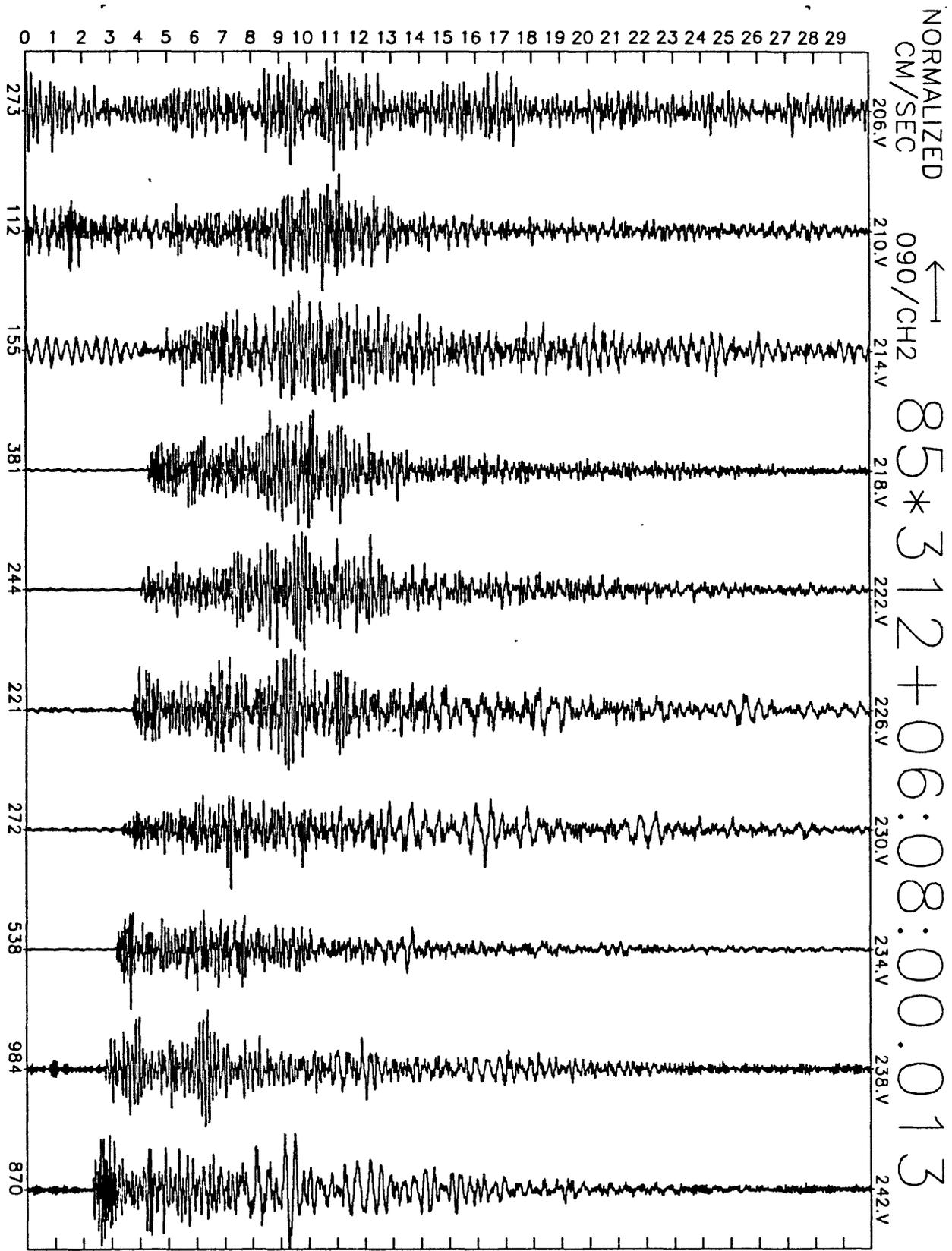
Figure A15(e), shot point 2: 30 second N20E velocity record. Abscissa is labeled with maximum counts in record (multiply by  $\frac{10}{2^{24}-2^8} \approx 6 \times 10^{-7}$  to get cm/sec). Times are unreduced beginning at time indicated.
