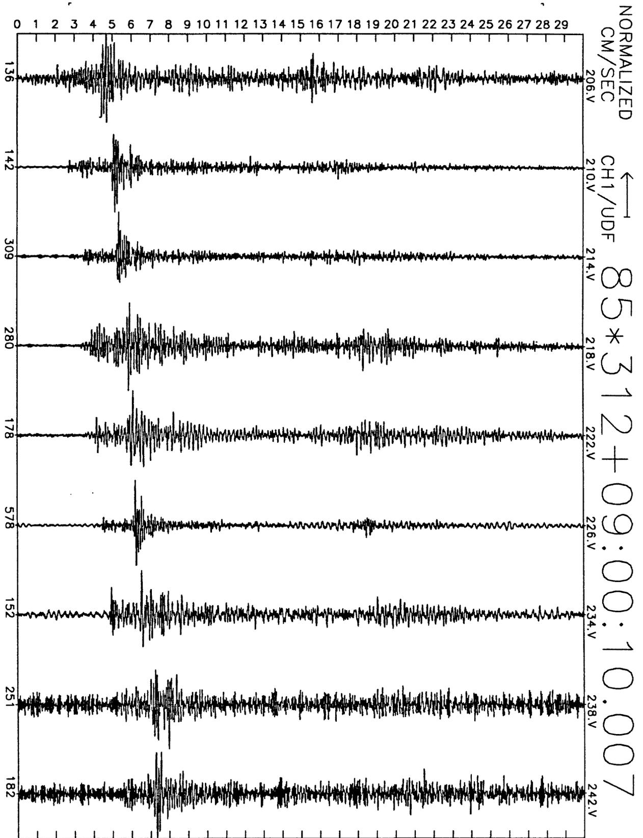
Figure A18(d), shot point 7: 30 second vertical velocity record. Abscissa is labeled with maximum counts in record (multiply by  $\frac{10}{2^{24}-2^8} \approx 6 \times 10^{-7}$  to get cm/sec). Times are unreduced beginning at time indicated.
