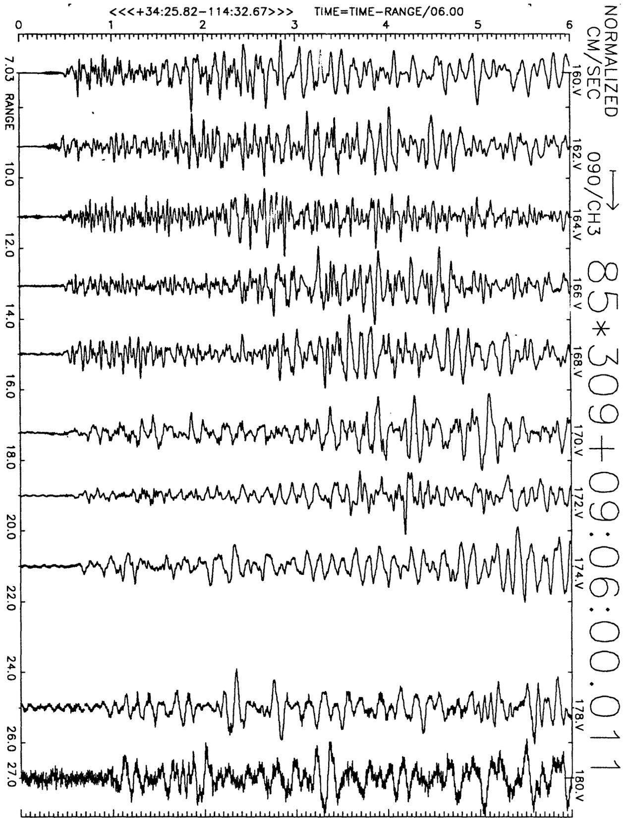
Figure A9(c), shot point 9X: 6 second velocity record. Positive N57E motion is to right. Abscissa is distance to shot point. Top of trace is labeled with station number. Times are reduced by 6 km/sec. Shot time is indicated.
