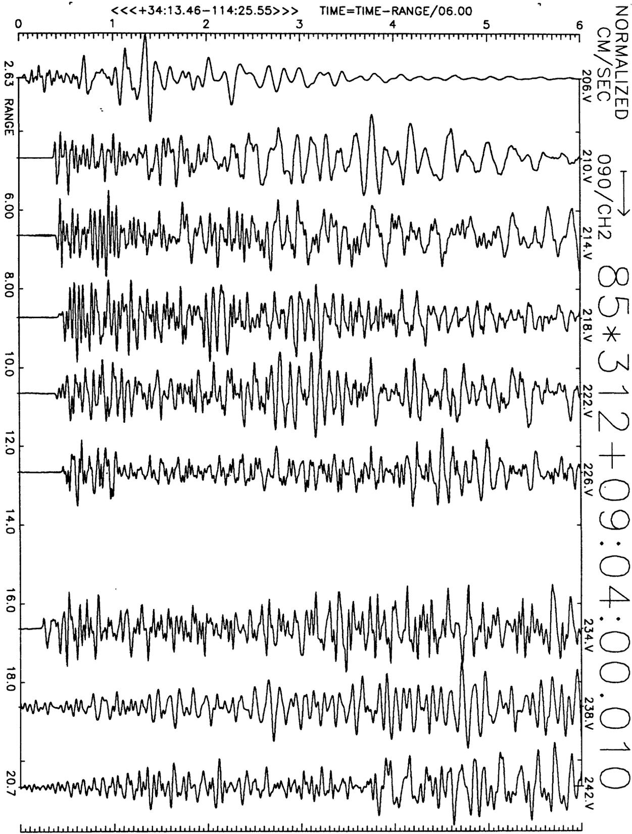
Figure A20(b), shot point 4B: 6 second velocity record. Positive N20E motion is to right. Abscissa is distance to shot point. Top of trace is labeled with station number. Times are reduced by 6 km/sec. Shot time is indicated.
