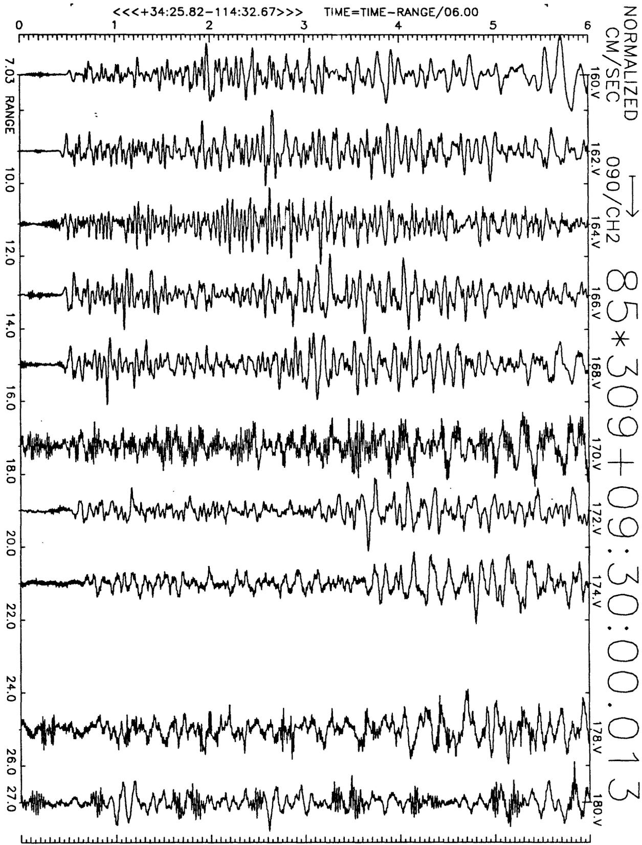
Figure A10(b), shot point 9X': 6 second velocity record. Positive N33W motion is to right. Abscissa is distance to shot point. Top of trace is labeled with station number. Times are reduced by 6 km/sec. Shot time is indicated.
