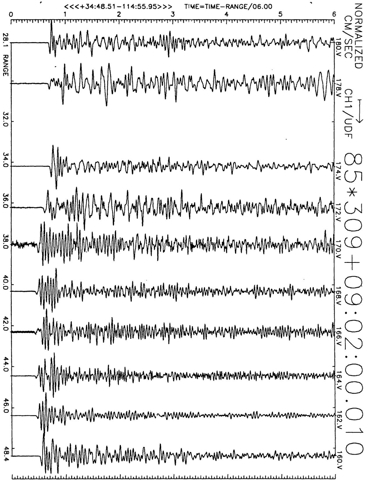
Figure A7(a), shot point 10: 6 second velocity record. Positive vertical motion is to right. Abscissa is distance to shot point. Top of trace is labeled with station number. Times are reduced by 6 km/sec. Shot time is indicated.
