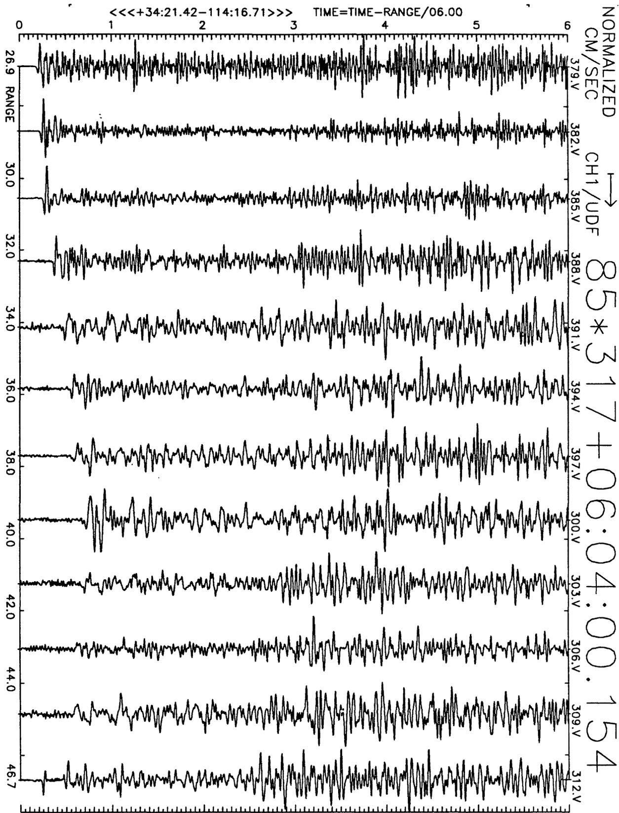
Figure A24(a), shot point 5: 6 second velocity record. Positive vertical motion is to right. Abscissa is distance to shot point. Top of trace is labeled with station number. Times are reduced by 6 km/sec. Shot time is indicated.
