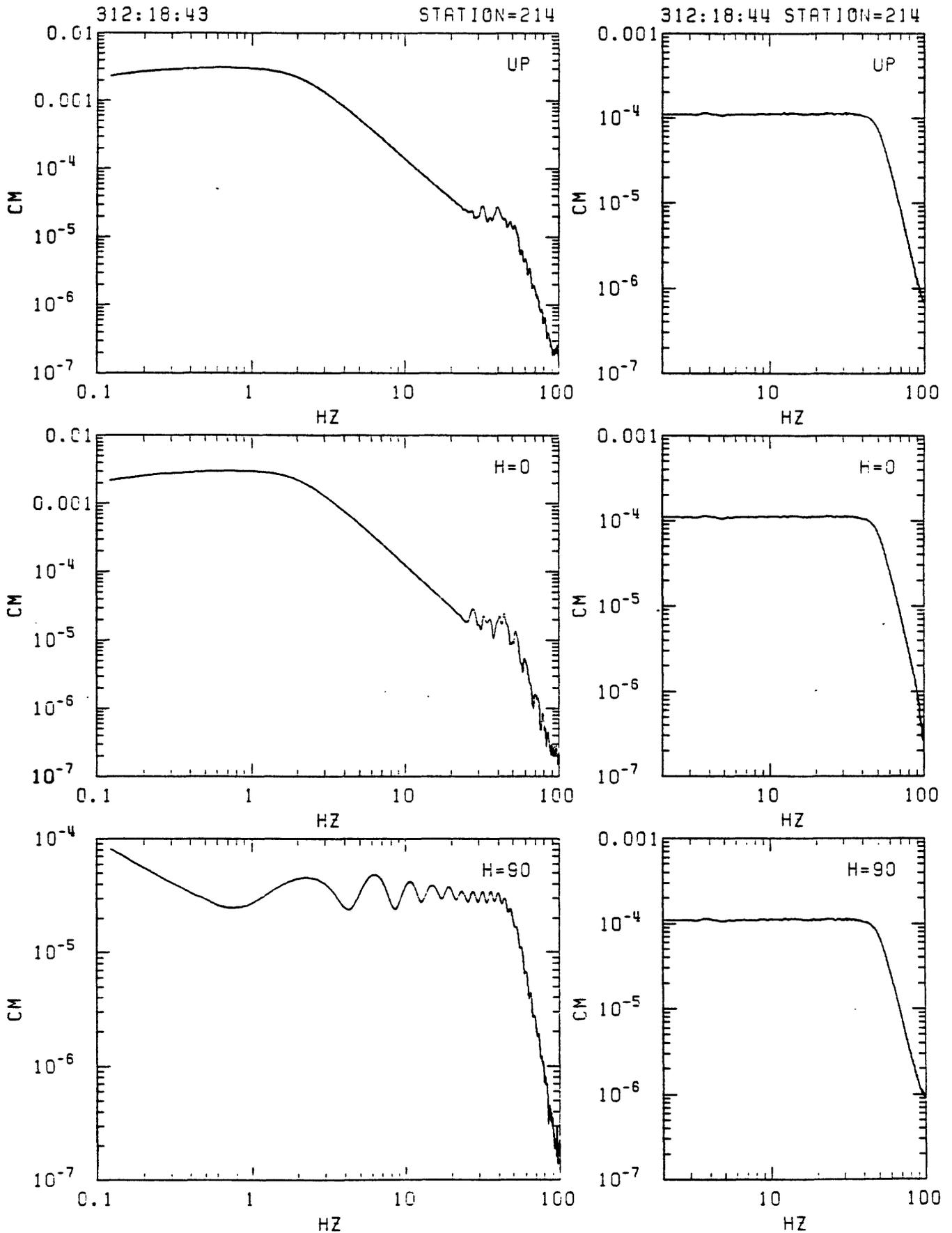
Figure C14. Station 214 in-situ velocity calibration spectra. Left: response to step in acceleration (seismometer mass released from rest at offset position). Right: response to delta function in velocity (voltage impulse applied to recorder input). From top: vertical, N20E and N110E.
