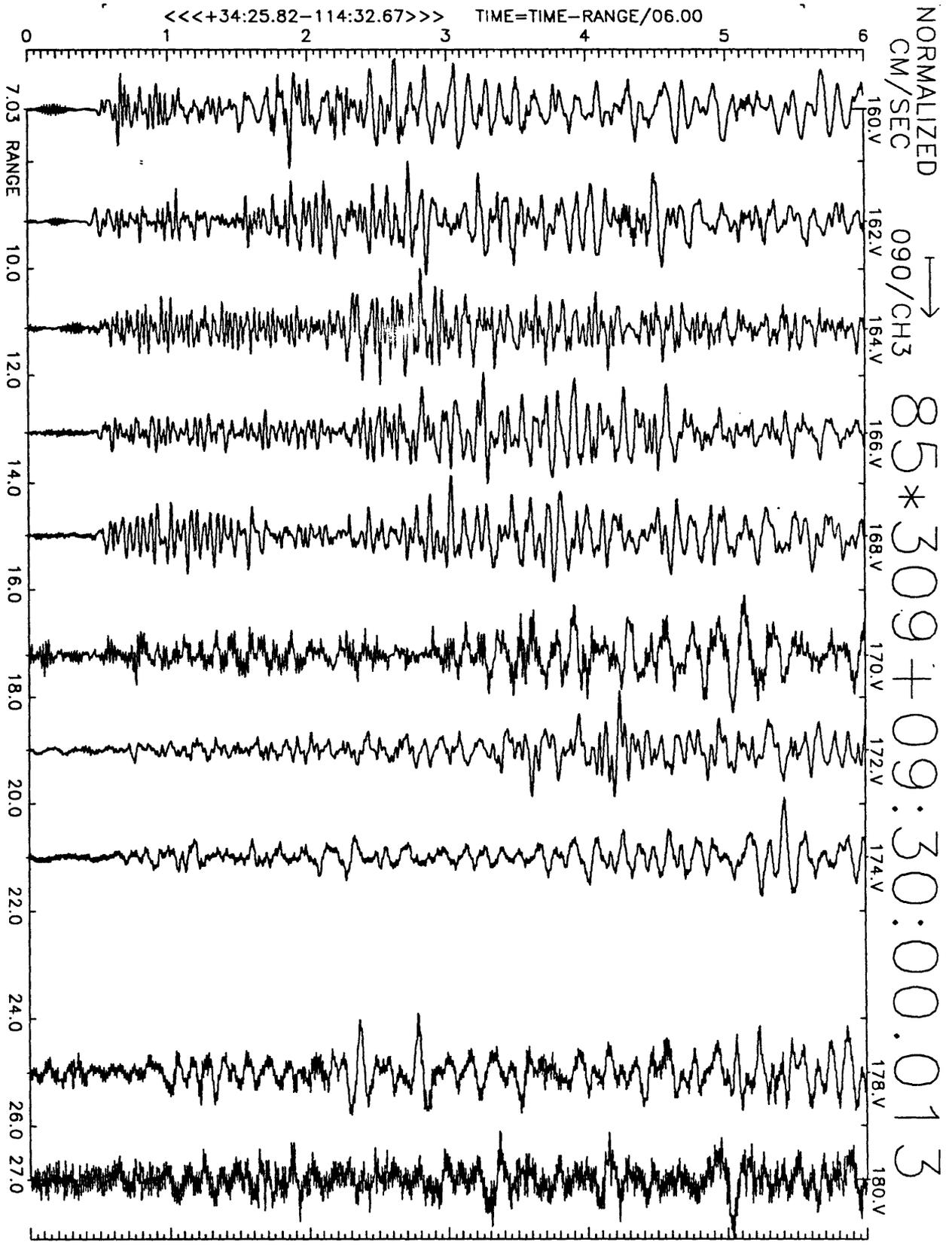
Figure A10(c), shot point 9X': 6 second velocity record. Positive N57E motion is to right. Abscissa is distance to shot point. Top of trace is labeled with station number. Times are reduced by 6 km/sec. Shot time is indicated.
