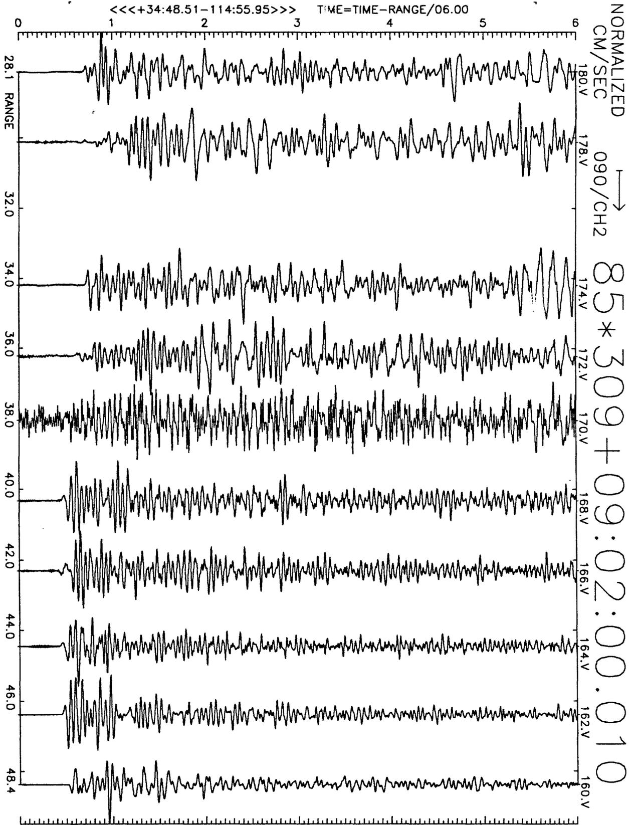
Figure A7(b), shot point 10: 6 second velocity record. Positive N33W motion is to right. Abscissa is distance to shot point. Top of trace is labeled with station number. Times are reduced by 6 km/sec. Shot time is indicated.
