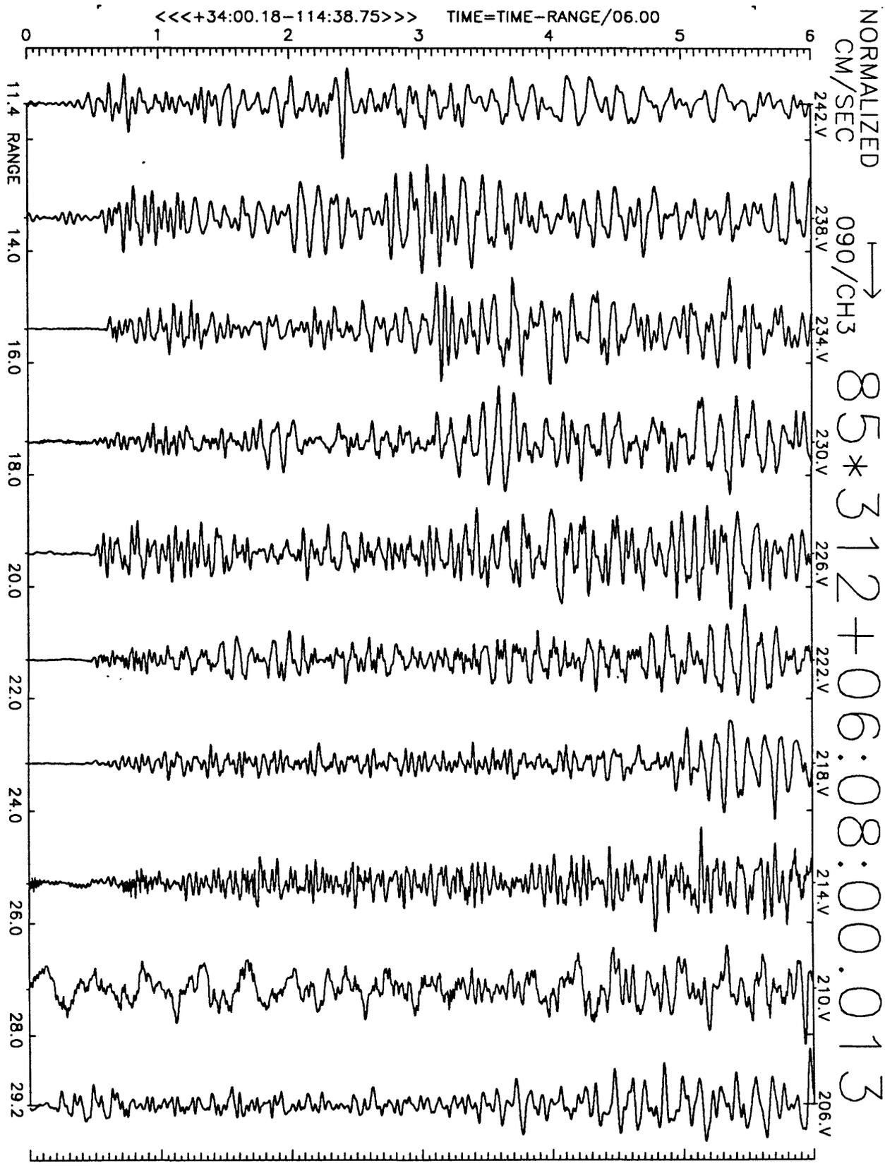
Figure A15(c), shot point 2: 6 second velocity record. Positive N110E motion is to right. Abscissa is distance to shot point. Top of trace is labeled with station number. Times are reduced by 6 km/sec. Shot time is indicated.
