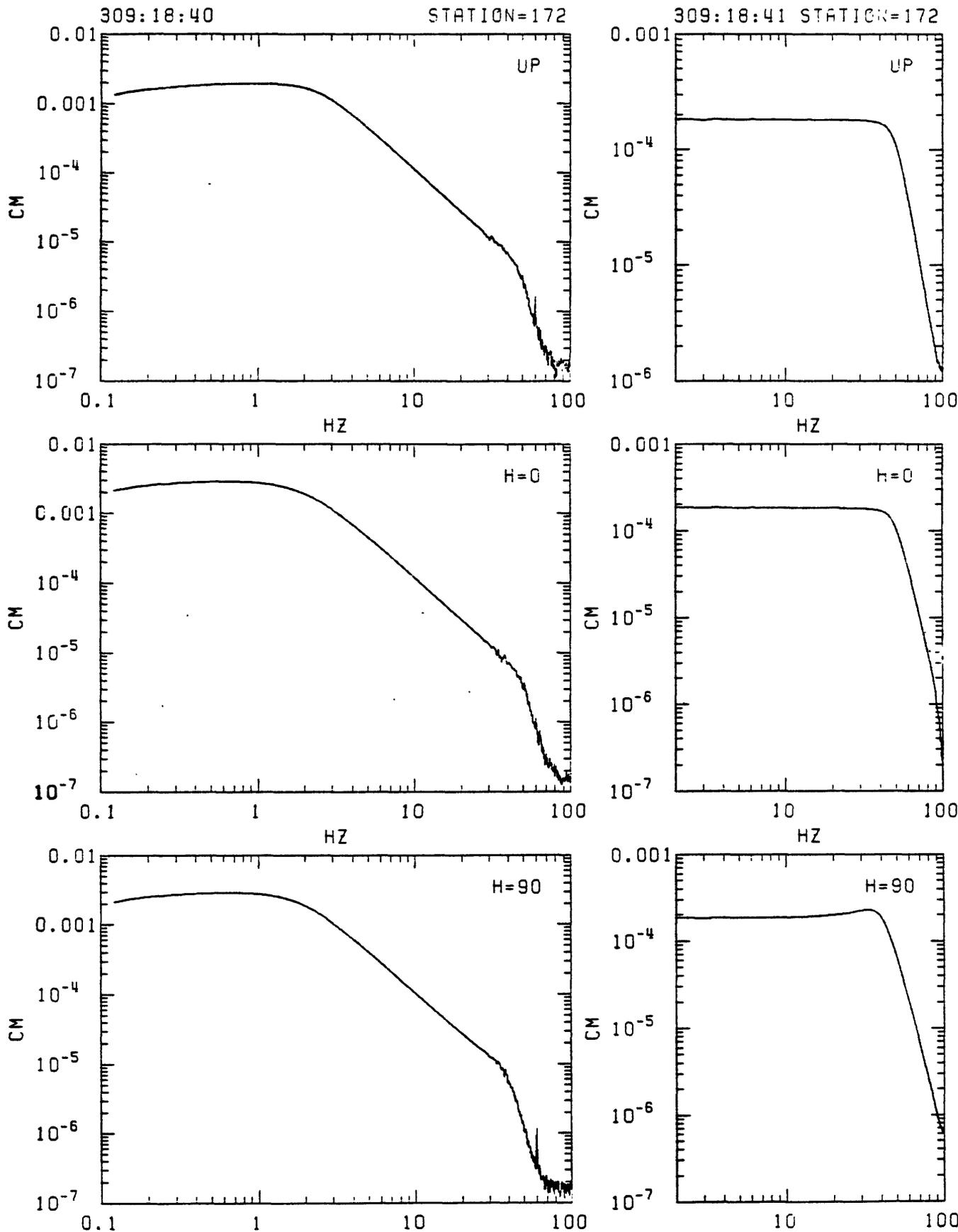
Figure C7. Station 172 in-situ velocity calibration spectra. Left: response to step in acceleration (seismometer mass released from rest at offset position). Right: response to delta function in velocity (voltage impulse applied to recorder input). From top: vertical, N33W and N57E.
