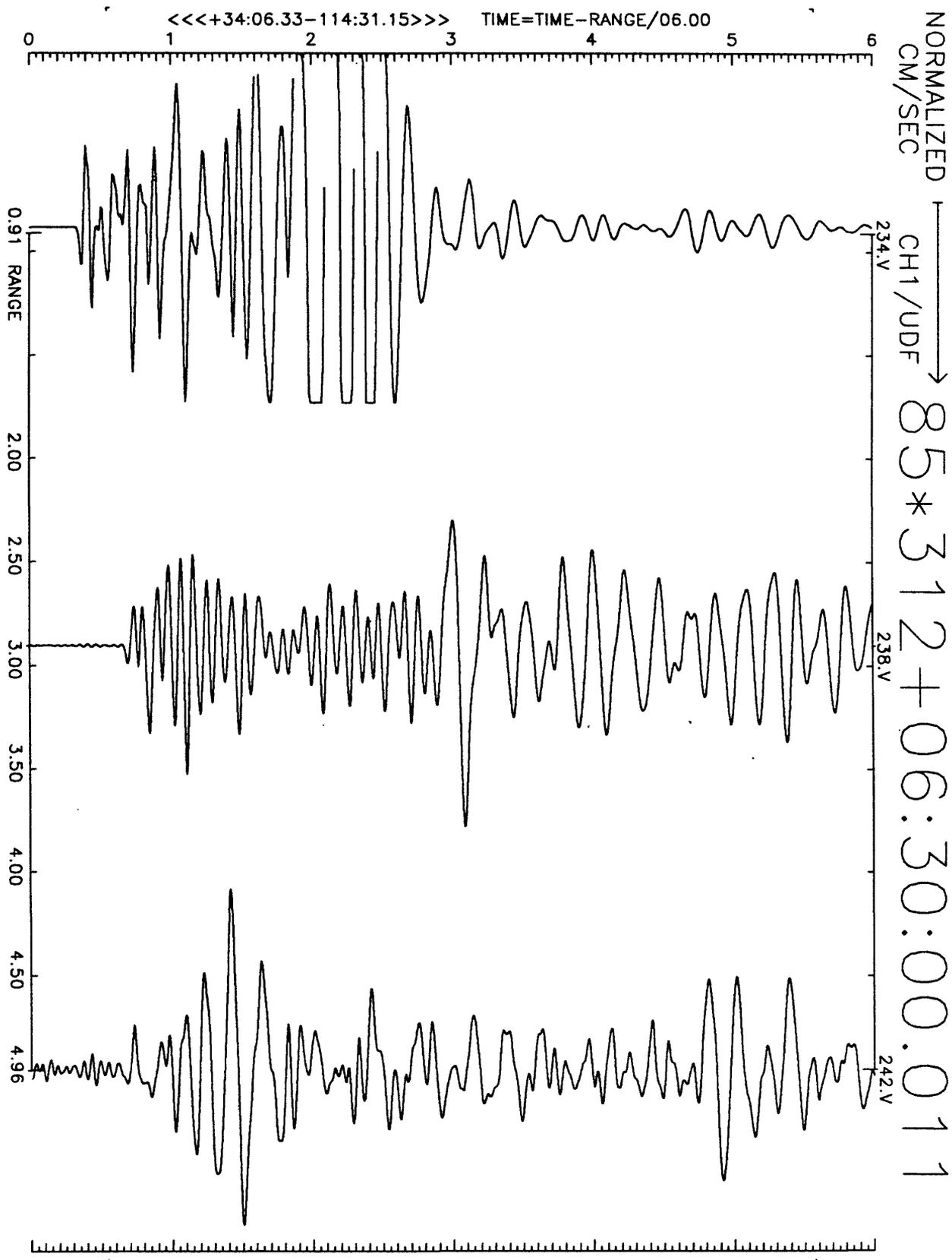
Figure A16(a), shot point 3', SW stations: 6 second velocity record. Positive vertical motion is to right. Abscissa is distance to shot point. Top of trace is labeled with station number. Times are reduced by 6 km/sec. Shot time is indicated.
