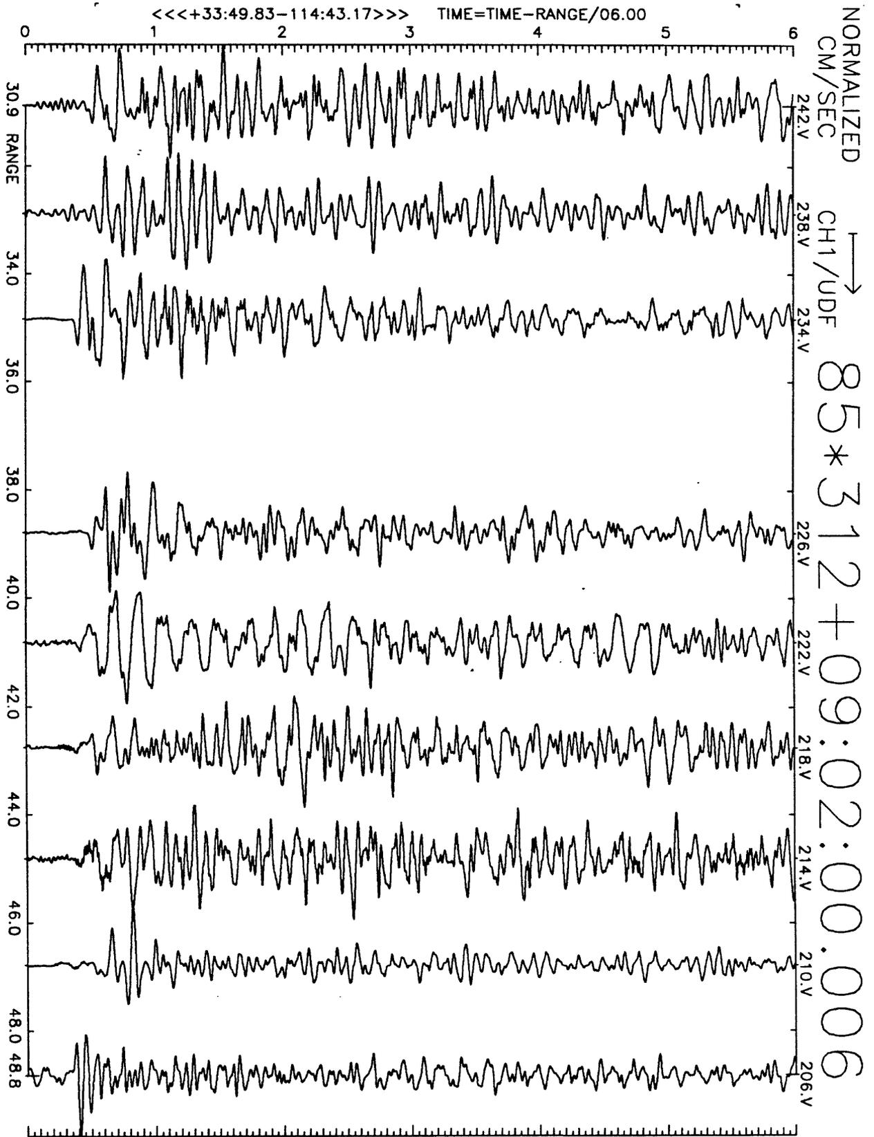
Figure A19(a), shot point 1: 6 second velocity record. Positive vertical motion is to right. Abscissa is distance to shot point. Top of trace is labeled with station number. Times are reduced by 6 km/sec. Shot time is indicated.
