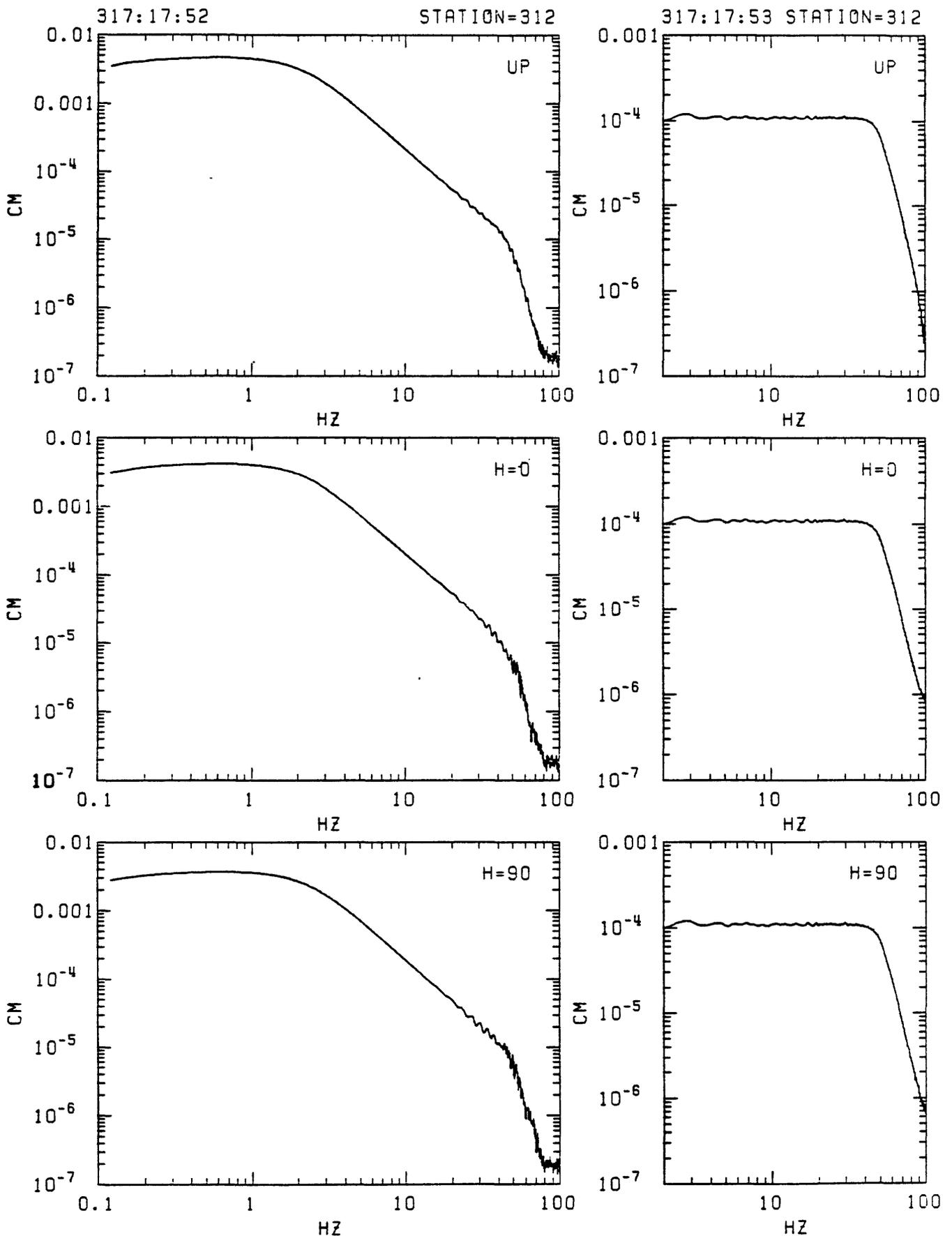
Figure C30. Station 312 in-situ velocity calibration spectra. Left: response to step in acceleration (seismometer mass released from rest at offset position). Right: response to delta function in velocity (voltage impulse applied to recorder input). From top: vertical, N25E and N115E.
