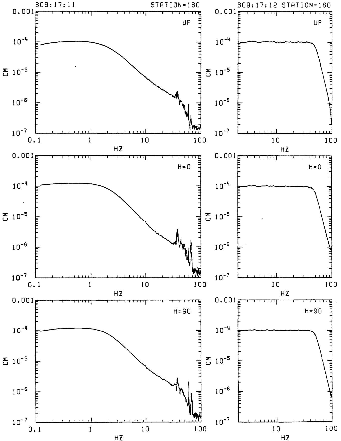
Figure C10. Station 180 in-situ velocity calibration spectra. Left: response to step in acceleration (seismometer mass released from rest at offset position). Right: response to delta function in velocity (voltage impulse applied to recorder input). From top: vertical, N33W and N57E.
