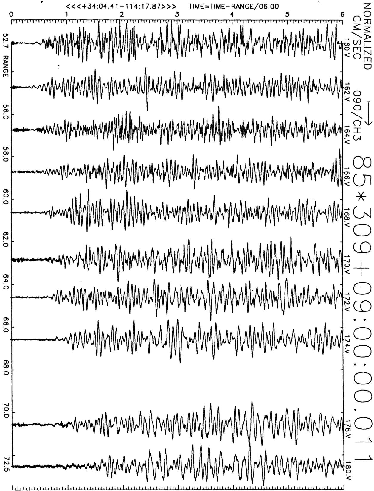
Figure A6(c), shot point 8X: 6 second velocity record. Positive N57E motion is to right. Abscissa is distance to shot point. Top of trace is labeled with station number. Times are reduced by 6 km/sec. Shot time is indicated.
