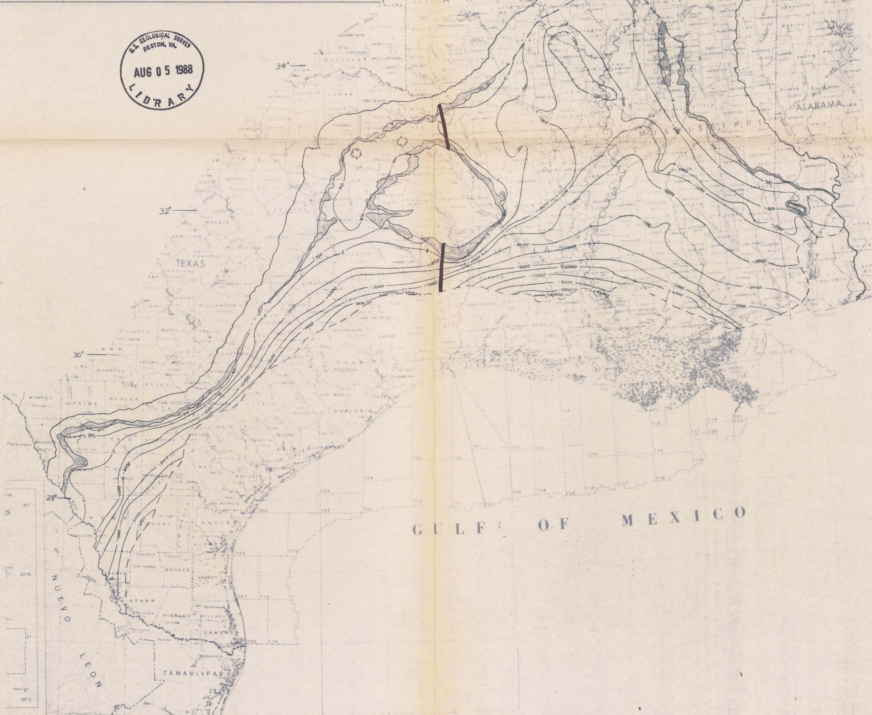
Figure 29.-- Altitude and configuration of top of the lower Claiborne confining unit, Mississippi embayment and Texas coastal uplands aquifer systems, south-central United States.
