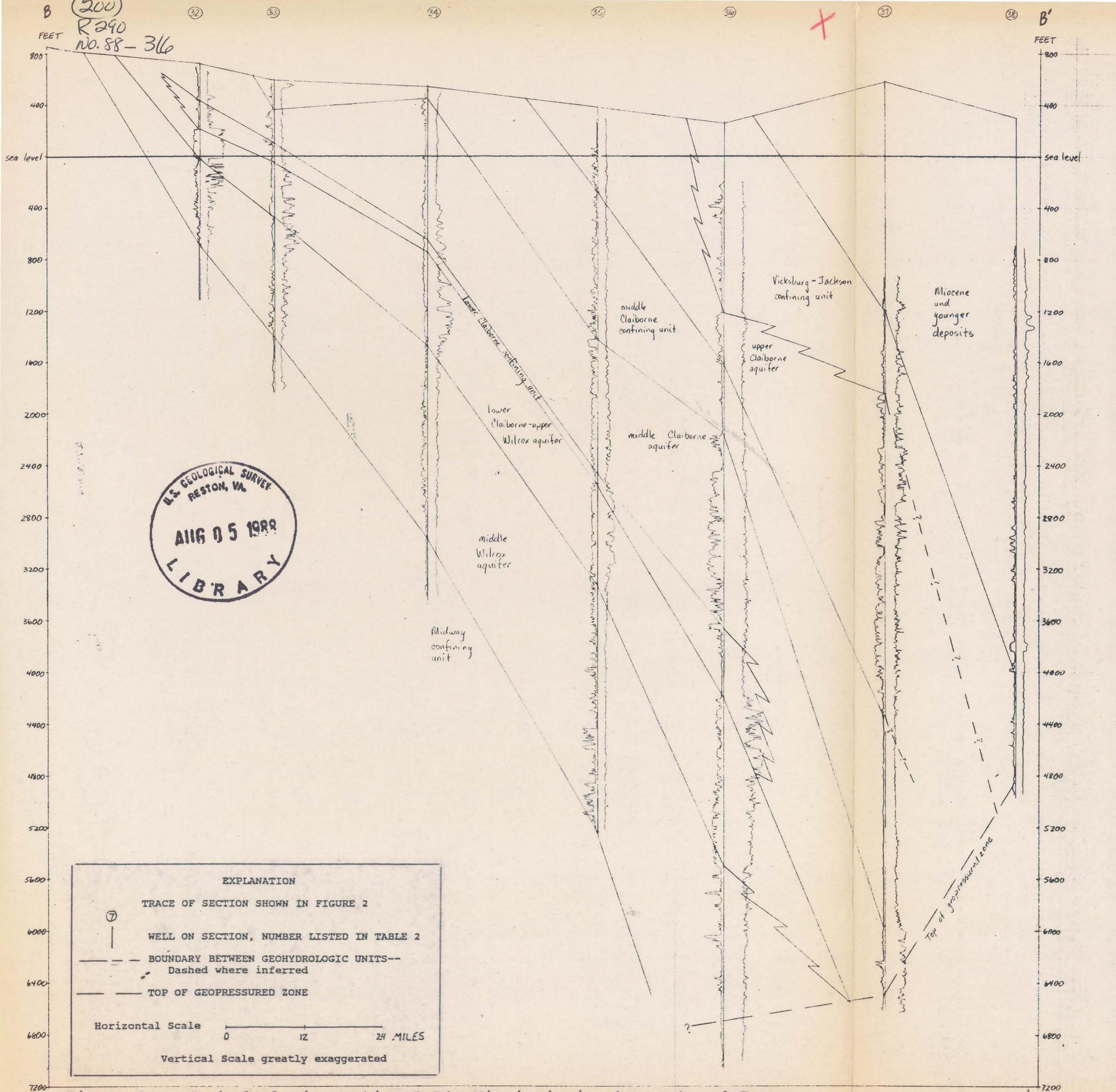
Figure 8.-- Geohydrologic section B-B', Mississippi embayment and Texas coastal uplands aquifer systems, south-central United States.
