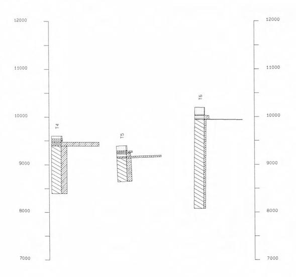
Figure 3. Example of cross section with numeric variables plotted as a bar graph attached to the lithologic log. GSLITH plot file SECT1.PLT, numeric variable file HIST.VAR.
