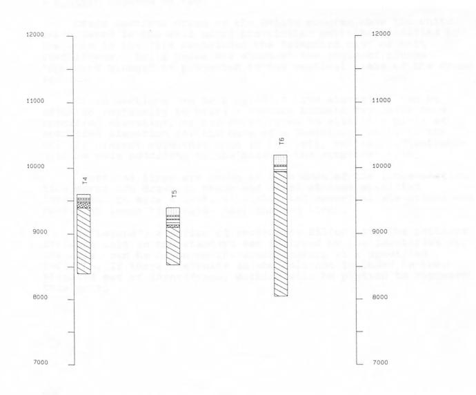
Figure 7. Section of type 3, compare with Fig. 2, especially the apparent change in length of hole T5 due to 60 plunge of hole. Distance and spacing specified in an ASCII file. GSLITH plot file SECT3.PLT, ASCII data file, SECT1.ASC
