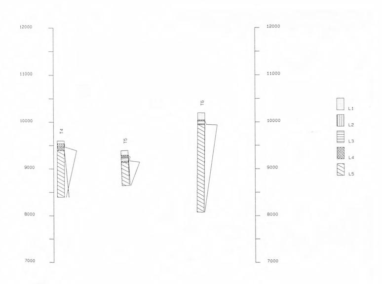
Figure 4. Cross section with numeric variables plotted as a trace on the right side of the lithologic log. GSLITH plot file SECT2.Plt, numeric variable file TRACE.VAR, legend plotted.
