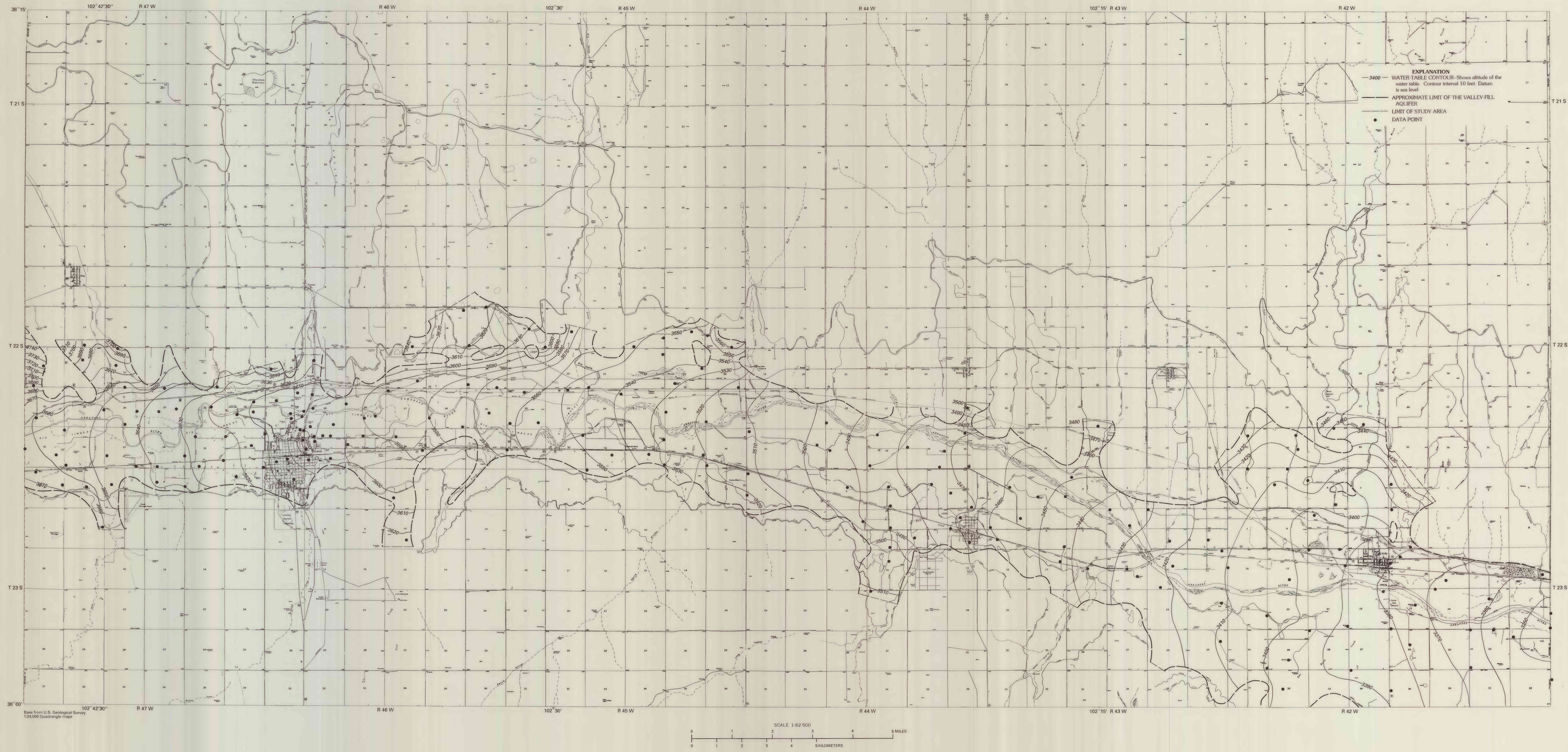
MAP SHOWING ALTITUDE AND CONFIGURATION OF THE WATER TABLE IN THE VALLEY-FILL AQUIFER, SPRING 1966
