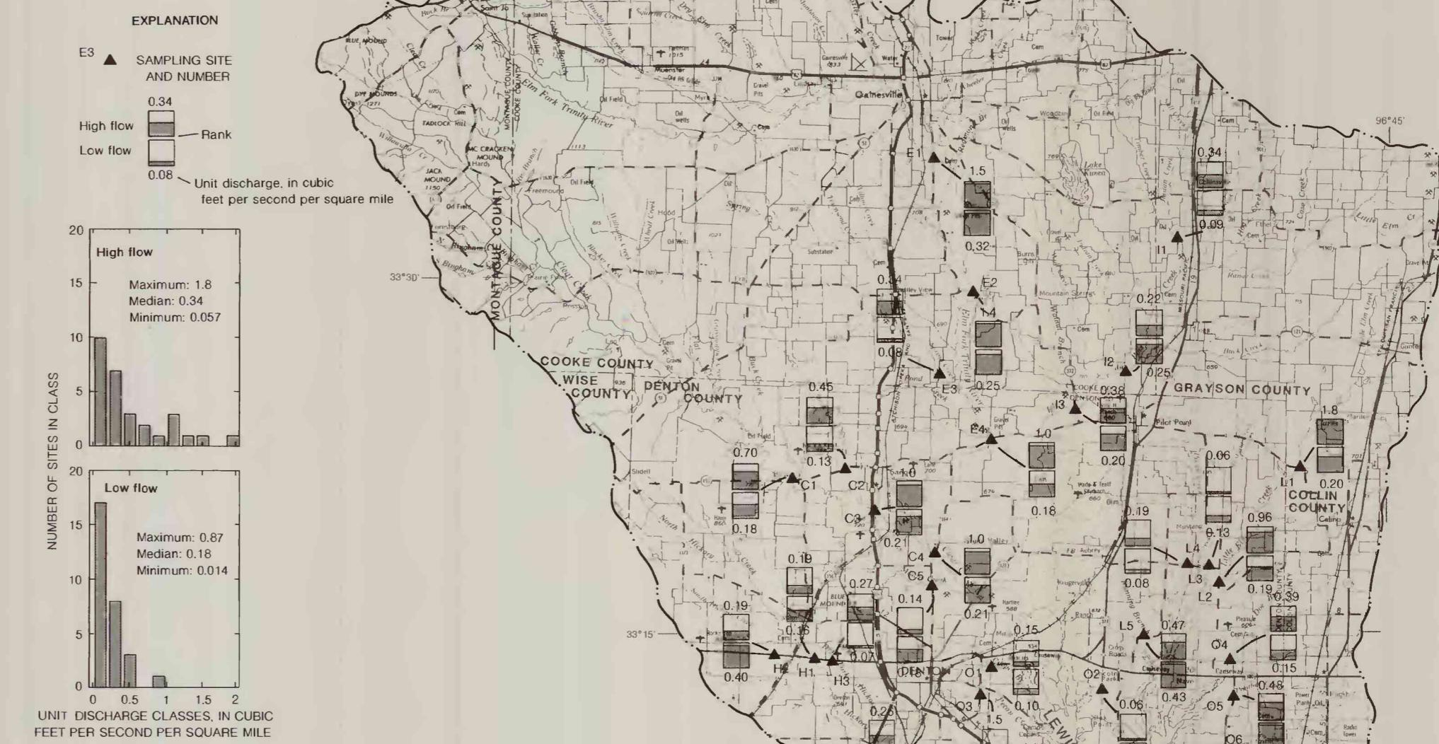
Figure 4.--Unit-discharge rankings, unit discharges and frequency histograms for low- and high-flow synoptic surveys.
