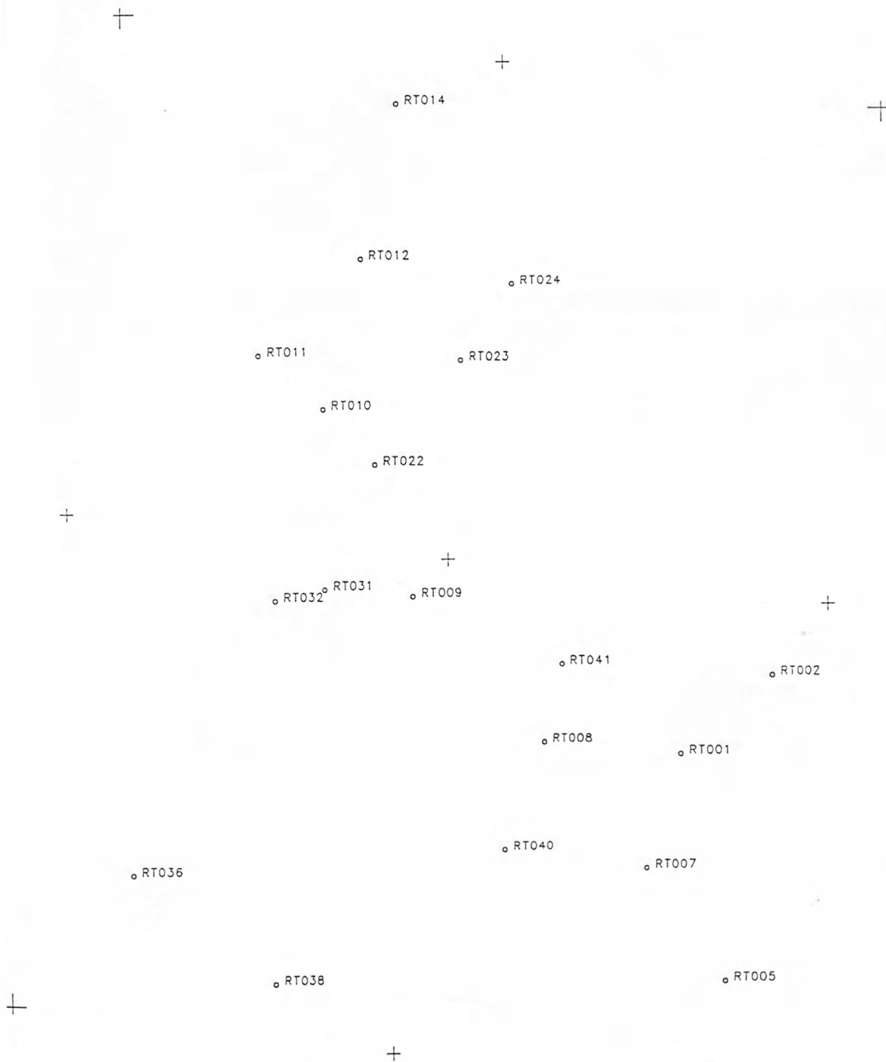
Fig. 4 _ Example of GSPOST plot. Plot file LL.PLT, projection file LL.PRJ, data file LL.PRN, Font #0; corners and internal geodetic ticks at 0,7,30 plotted. This kind of plot file, and data file makes an excellent star for on-screen editing.
