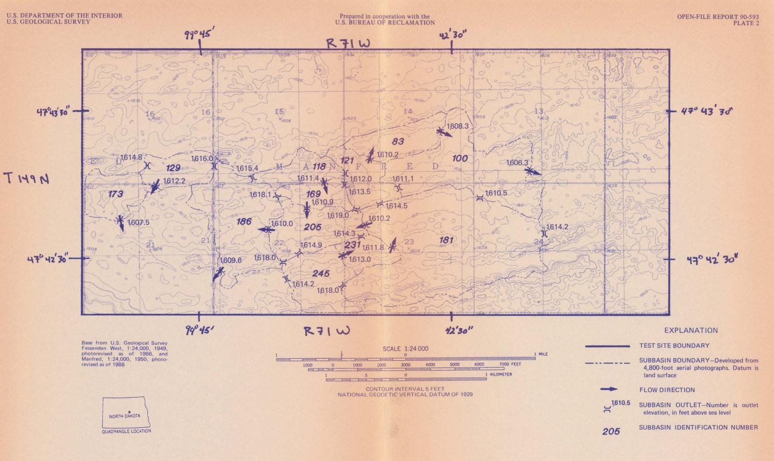
Plate 2.—Map showing drainage-area boundaries and outlet elevations of subbasins in test site 3 computed using a digital elevation model developed from 4,800-foot aerial photographs.
