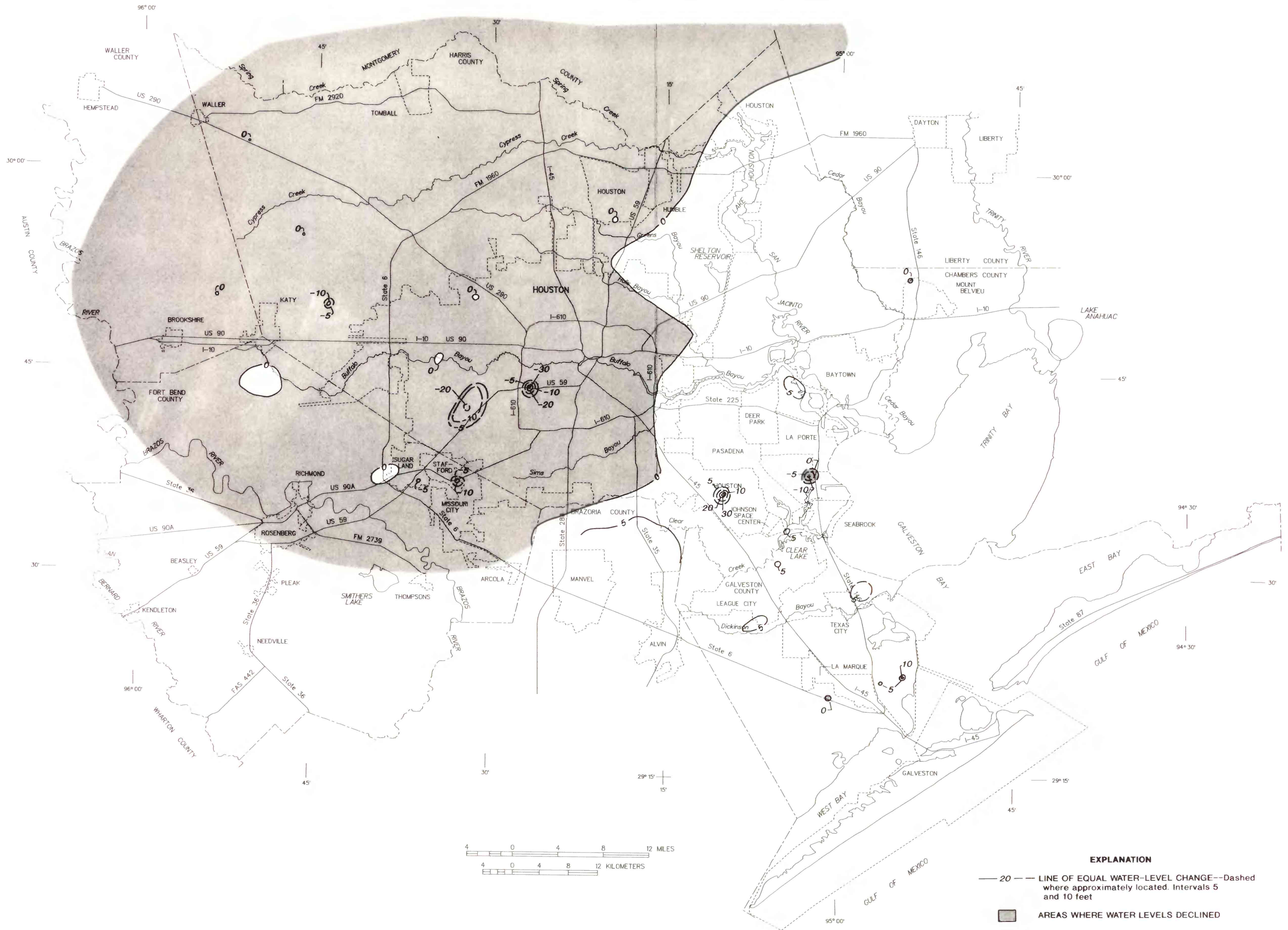
Figure 2.--Map showing approximate change in water levels in wells completed in the Chicot aquifer, 1990-91.
