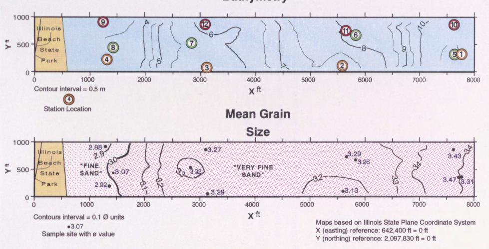
Fig. 5: Sediment mean grain size (ø-units) and sediment classification of diver core samples. Note similarities in texture of samples collected at the same water depth. Note also the difference between geologic and engineering (Unified) classification systems.
