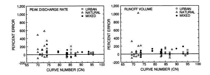
Figure 25. Comparison of the percent error between observed and estimated peak discharge rates and runoff volumes with the average watershed curve number using the NRCS TR-20 model.
