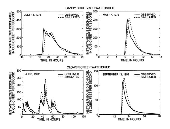
**Figure 26.** Typical observed hydrographs for storms occurring in the Gandy Boulevard and Clower Creek watersheds and corresponding hydrographs simulated using the NRCS TR-20 model.
