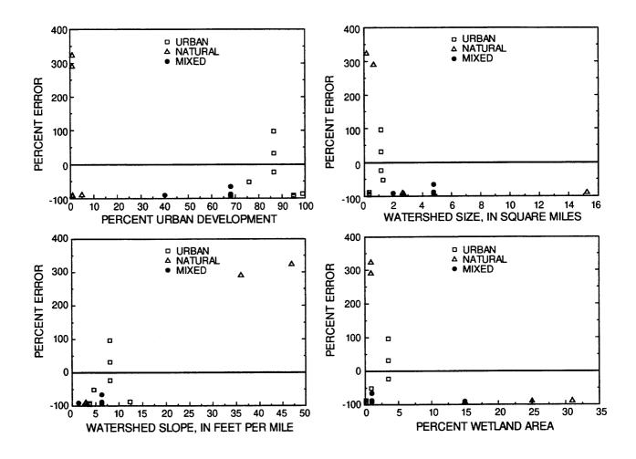
Figure 23. Comparison of the percent error between observed and estimated runoff volumes with watershed development, size, slope, and wetland area using the U.S. Geological Survey regional regression equations.
