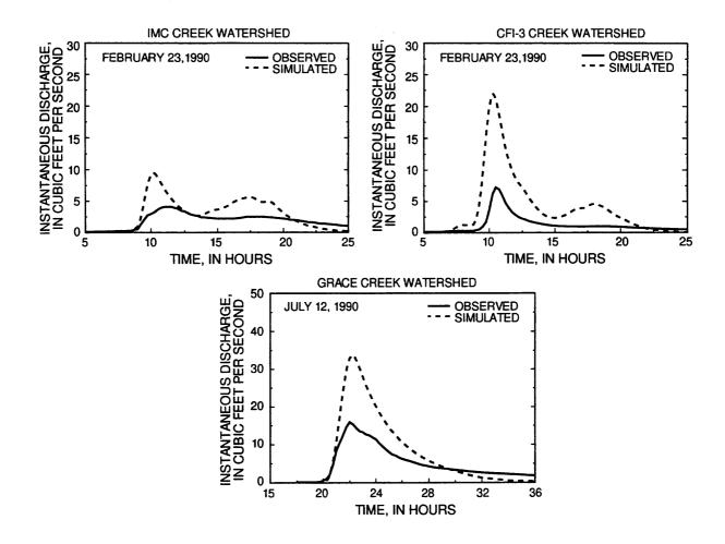
Figure 30. Typical observed hydrographs for storms occurring in the IMC, CFI-3, and Grace Creek watersheds and corresponding hydrographs simulated using the NRCS TR-20 model.
