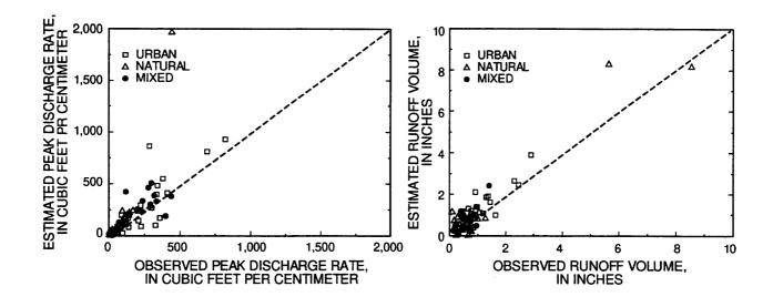
Figure 24. Comparison of the observed and estimated peak discharge rates and runoff volumes calculated using the NRCS TR-20 model.
