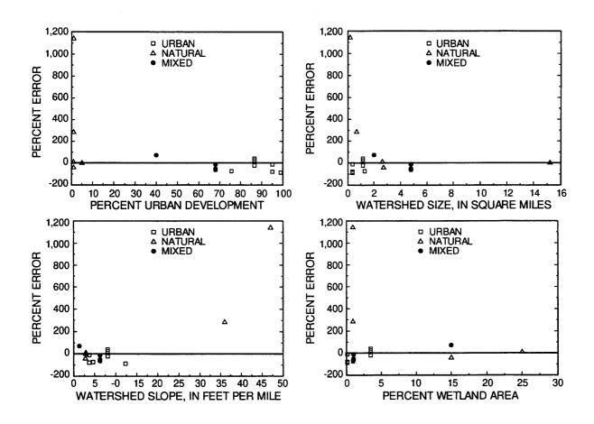
gure 22. Comparison of the percent error between observed and estimated peak discharge rates with watershed velopment, size, slope, and wetland area using the U.S. Geological Survey regional regression equations.
