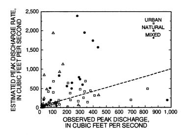
Figure 19. Comparison of observed and estimated peak discharge rates using the rational method.
