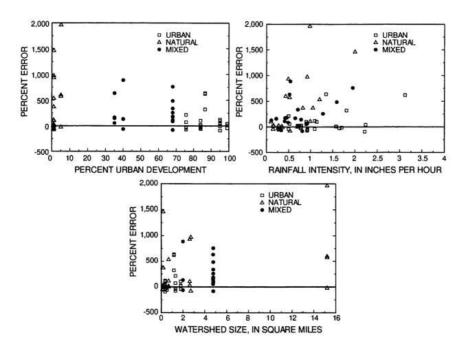
**igure 20.** Comparison of the percent error between observed and estimated peak discharge rates with watershed evelopment, rainfall intensity, and watershed size using the rational method.
