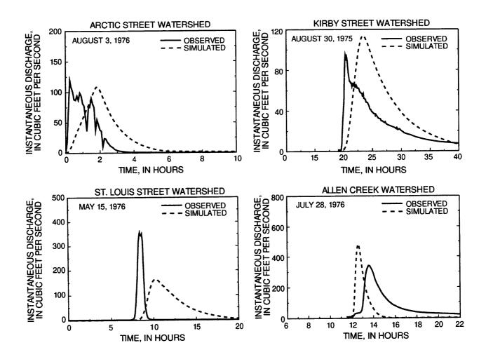
**Figure 27**. Typical observed hydrographs for storms occurring in the Arctic Street, Kirby Street, St. Louis Street, and Allen Creek watersheds, and corresponding hydrographs simulated using the NRCS TR-20 model.
