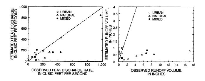
**Figure 21.** Comparison of observed and estimated peak discharge rates and runoff volumes using the U.S. Geological Survey regional regression equations.
