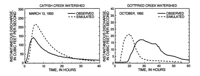
Figure 29. Typical observed hydrographs for storms occurring in the Catfish Creek and Gottfried Creek watersheds and corresponding hydrographs simulated using the NRCS TR-20 model.
