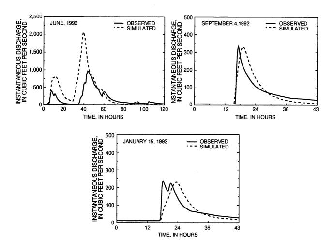
**Figure 28.** Typical observed hydrographs for storms occurring in the Walker Creek watershed and corresponding hydrographs simulated using the NRCS TR-20 model.
