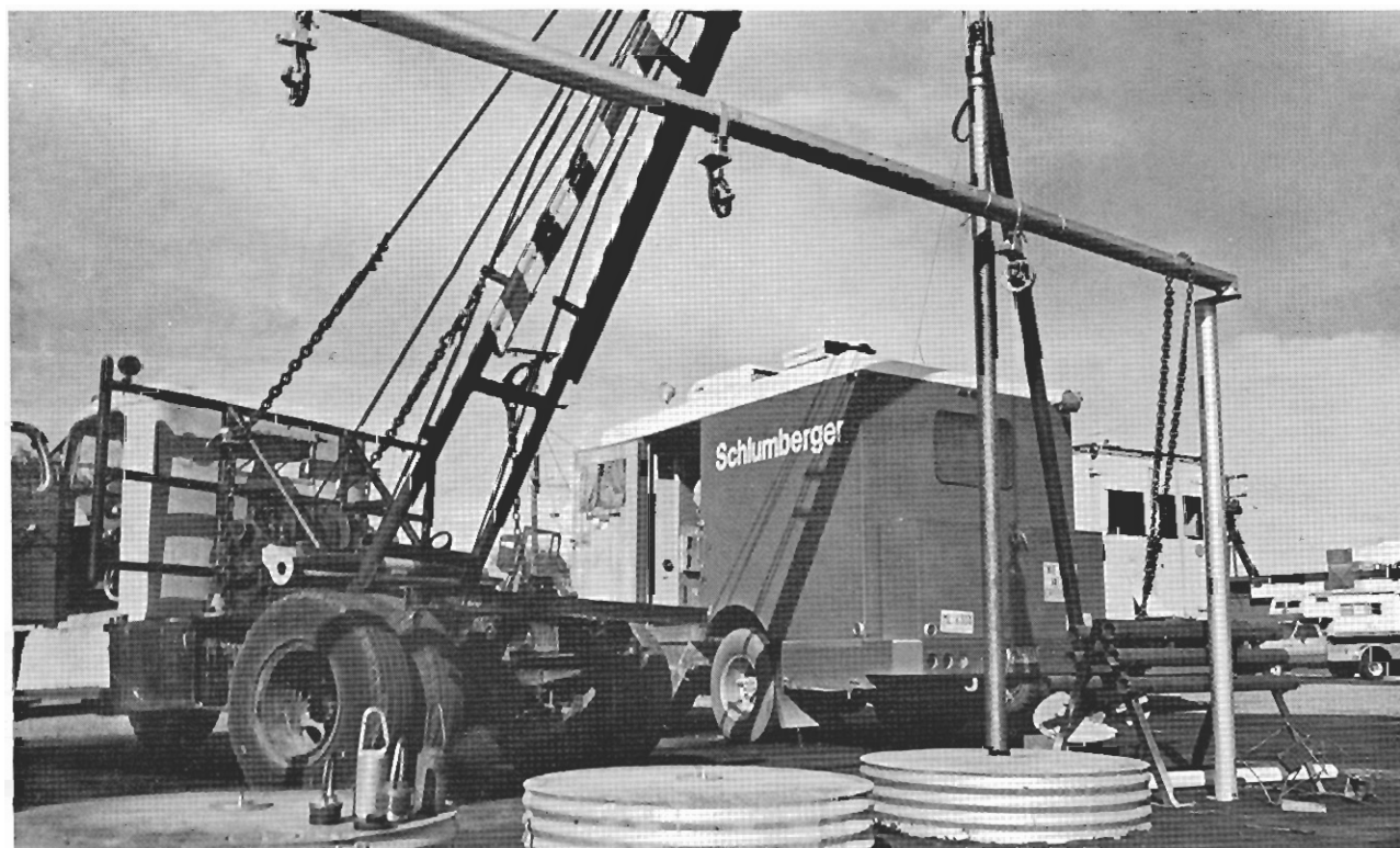
By using an auxiliary boom truck, an industry logging vehicle was able to use the Grand Junction KUT models to calibrate a petroleum spectral logging probe.
