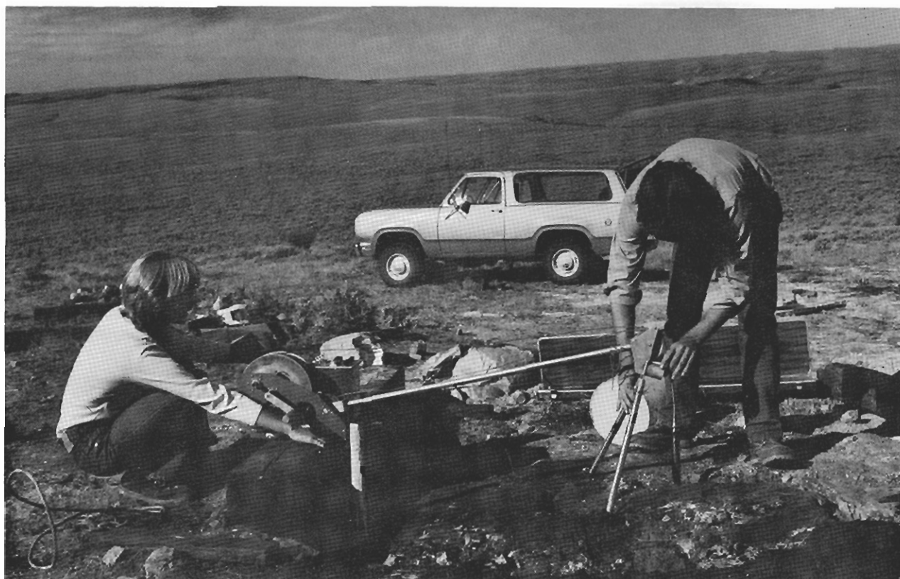
A portable down hole gross gamma-ray probe is used in one of the southeast Wyoming boreholes.
