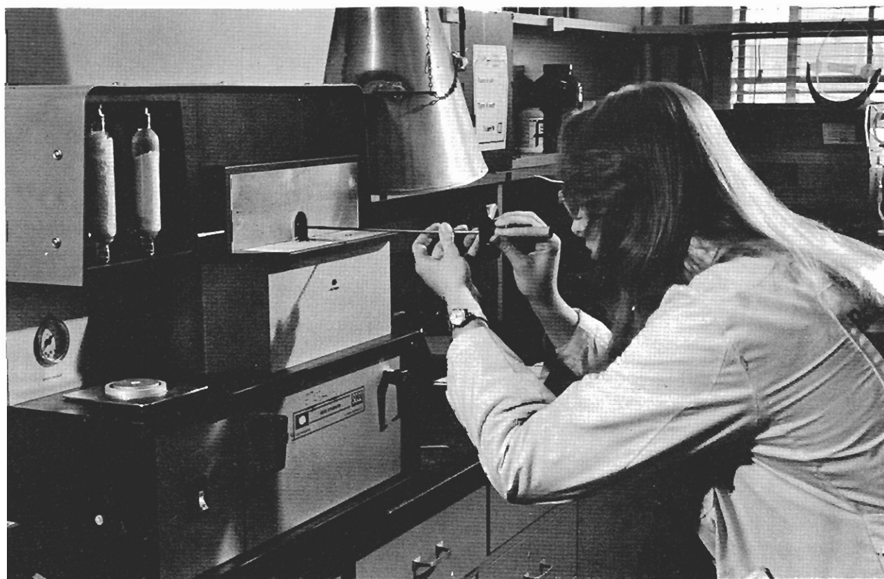
Chemist inserting boat in LECO sulphur analyzer at the Grand Junction laboratory.
