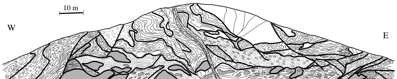
Figure 5. Sketch of exposed geology from the Beowawe turnoff road cut. Solid lines in sketch represent form lines of undifferentiated bedding ( S_0 ). Dashed, dash-dot lines either bedding or foliation ( S_1 ); Patterned or plain areas represent phacoids of competent rocks in sheared rock or clast-in-matrix rock (lensoid pattern). Rock types include laminated pelitic chert, massive chert, silty and calcareous sandstone, and massive dolomitic, fine-grained sandstone. See fig. 4 for location in area of Bob's Flat. See Peters (1996, 1997a) for detailed geologic legend and rock types.
