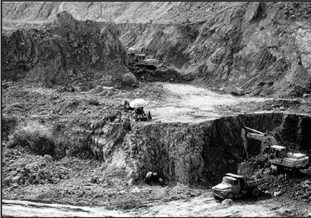
Figure 3. Photograph of mechanized mining in the Hengxian gold deposit, Guangxi district (Looking to southwest). Blasting is commonly done at the toe of the bench, which collapses the brow. Mucking and tramming is by 20 tonne dump truck.
