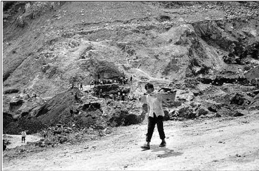
Figure 2. Photograph of manual mining in the Zimudang gold deposit, Guizhou province (Looking to southwest). Digging face in middle ground is the main shear zone.
