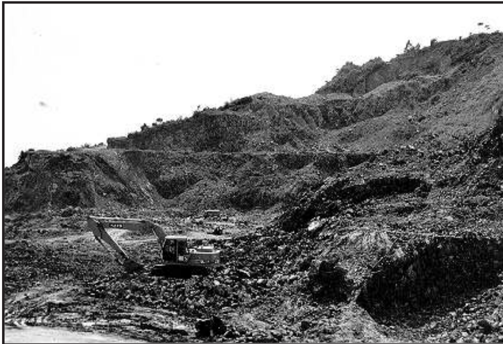
Figure 3. Photograph of mechanized mining in the Hengxian gold deposit, Guangxi district (Looking to southwest). Blasting is commonly done at the toe of the bench, which collapses the brow. Mucking and tramming is by 20 tonne dump truck.
