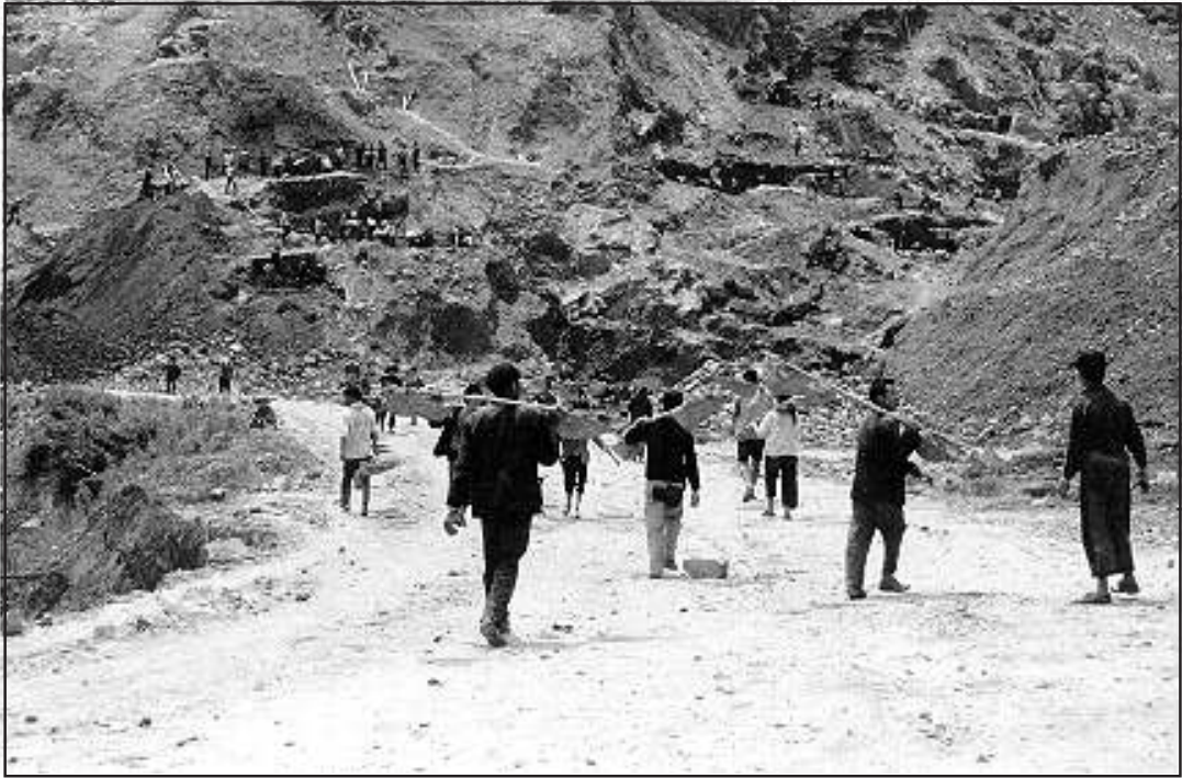
Figure 1. Photograph of manual mining in the Zimudang gold deposit, Guizhou province (Looking to southwest). Each miner trams about 25 kg of rock in double baskets. Total production is close to 300 tpd.
