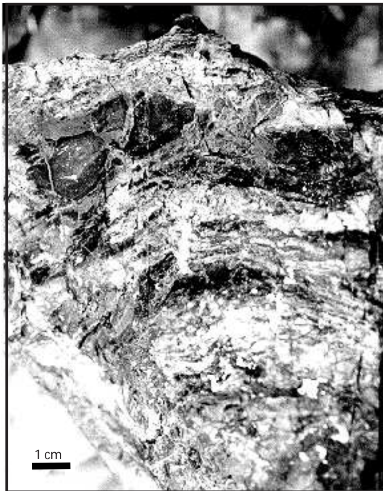
Figure 44. Photograph of mineralized jasperoid breccia in the Gaolong gold deposit, Guangxi District.
