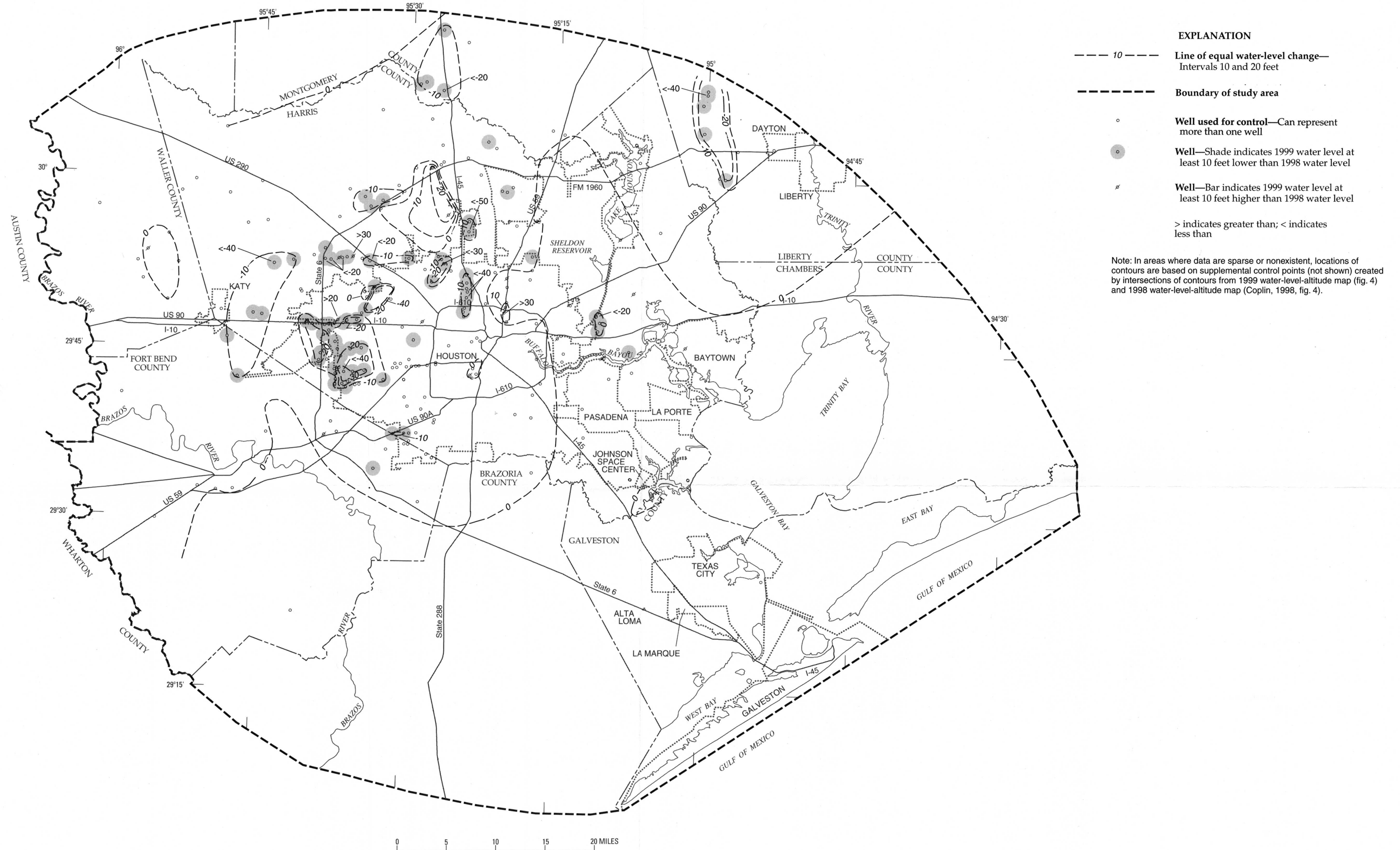
Figure 6. Map showing approximate water-level changes in the Evangeline aquifer, Houston-Galveston region, Texas, 1998-99.
