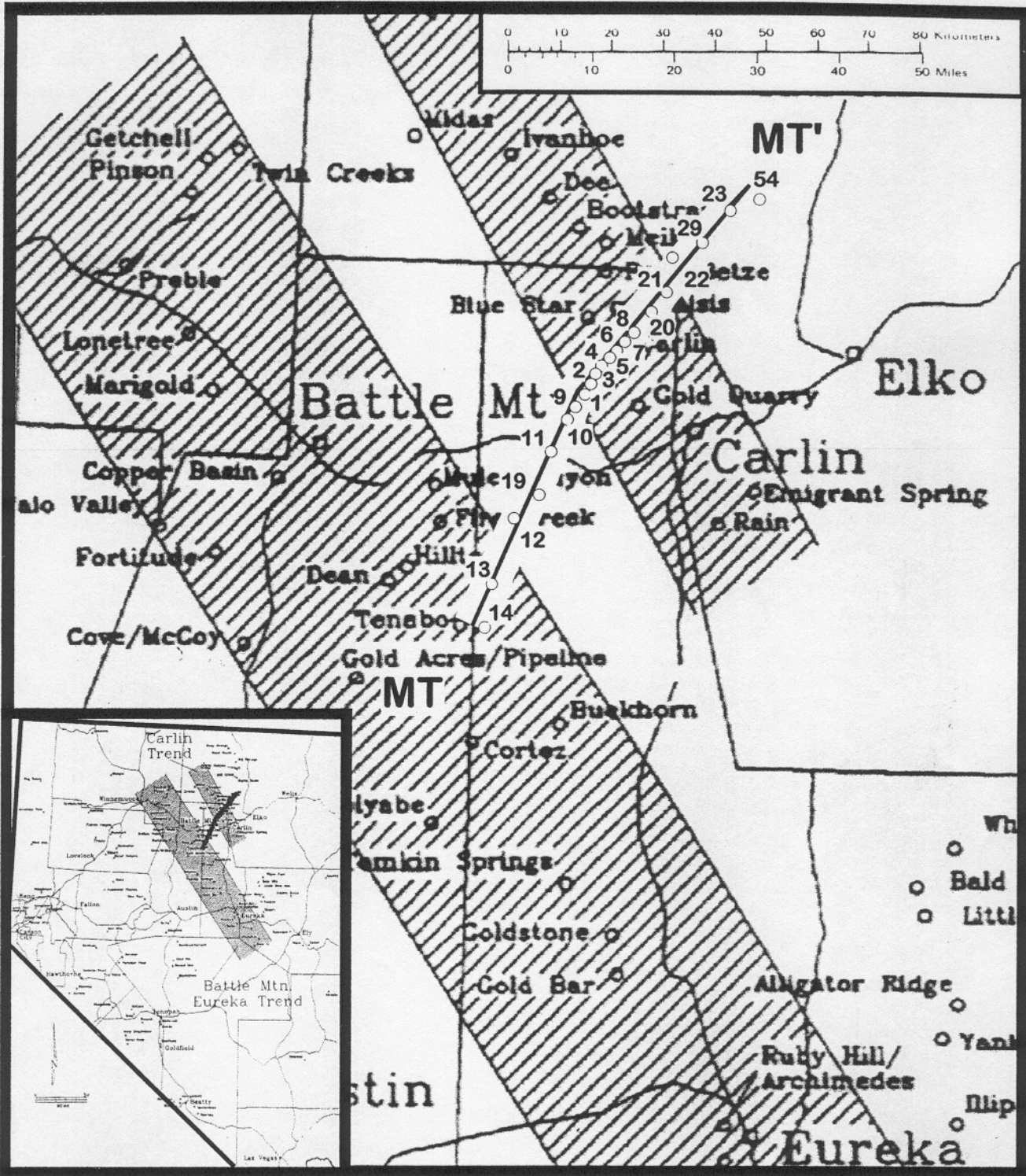
Figure 1. Index map. Magnetotelluric transect (MT-MT') acquired in 1996 across the Carlin trend in northeastern Nevada. Shaded zones are two northwest-trending mineralized belts in northeastern Nevada, the well-known Carlin trend and the less well defined Battle Mountain-Eureka trend. Base map adapted from Doebrich and others (1995).
