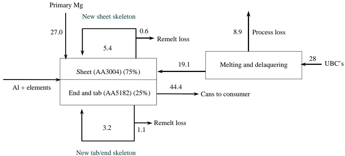
Figure 4. Simplified used beverage can processing, in thousand metric tons contained magnesium. UBC's, used beverage cans. (Adapted from Bowman, 1983.)
