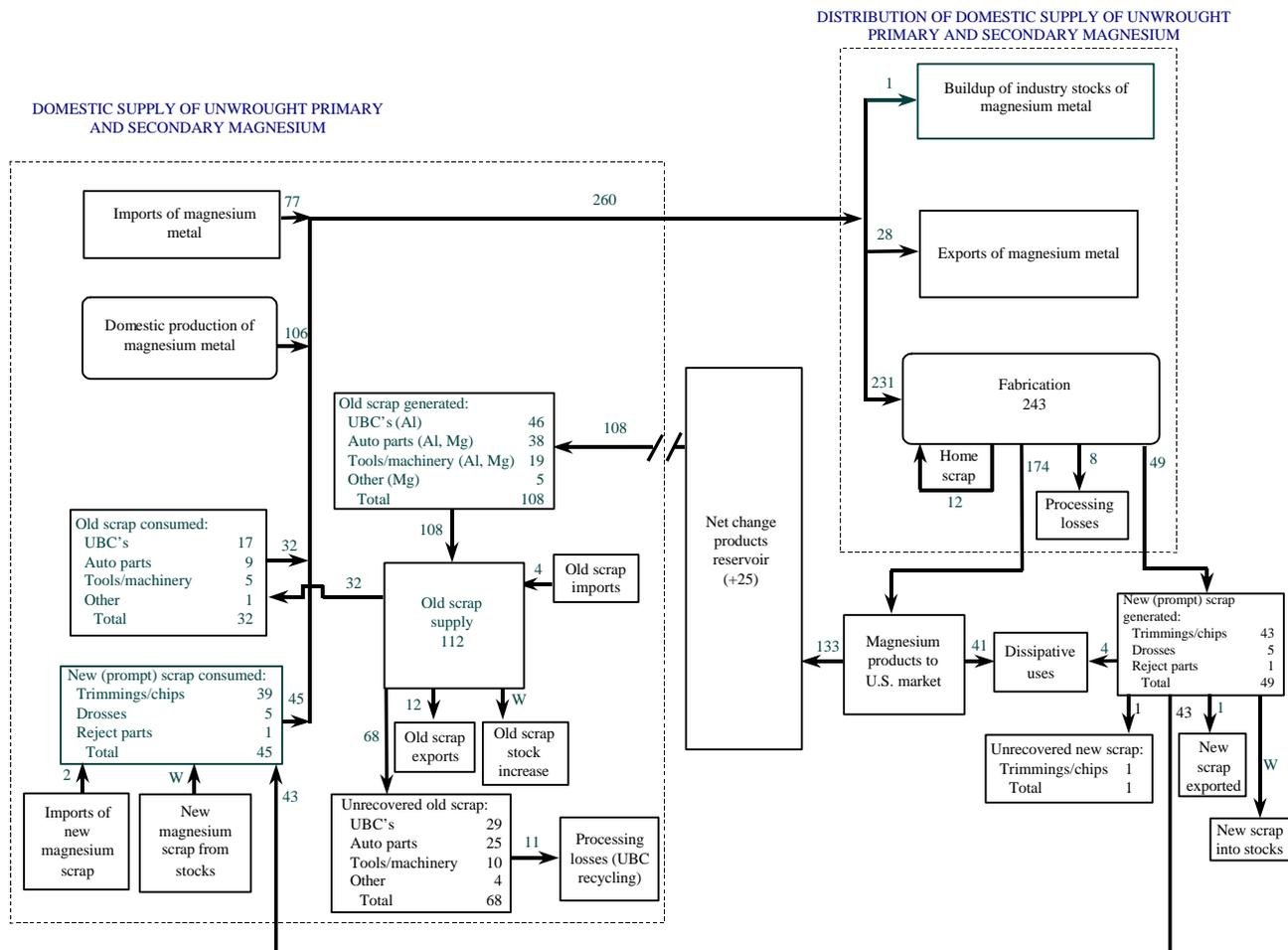
Figure 1. Magnesium recycling flow, 1998, in thousand metric tons contained magnesium. W, withheld to avoid disclosing company proprietary data; UBC's, used beverage cans.
