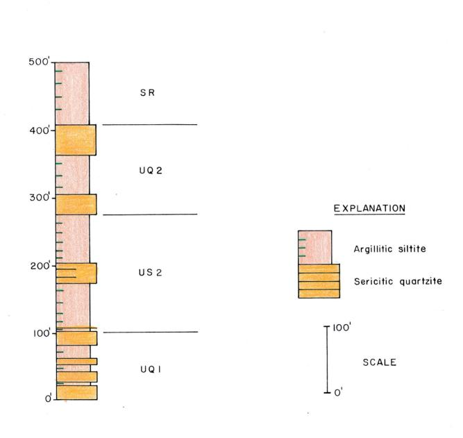
Plate 5 - Stratigraphy of Coeur 3400 E, as revealed by mapping. Distance along the rib has been converted trigonometrically to stratigraphic thickness.
