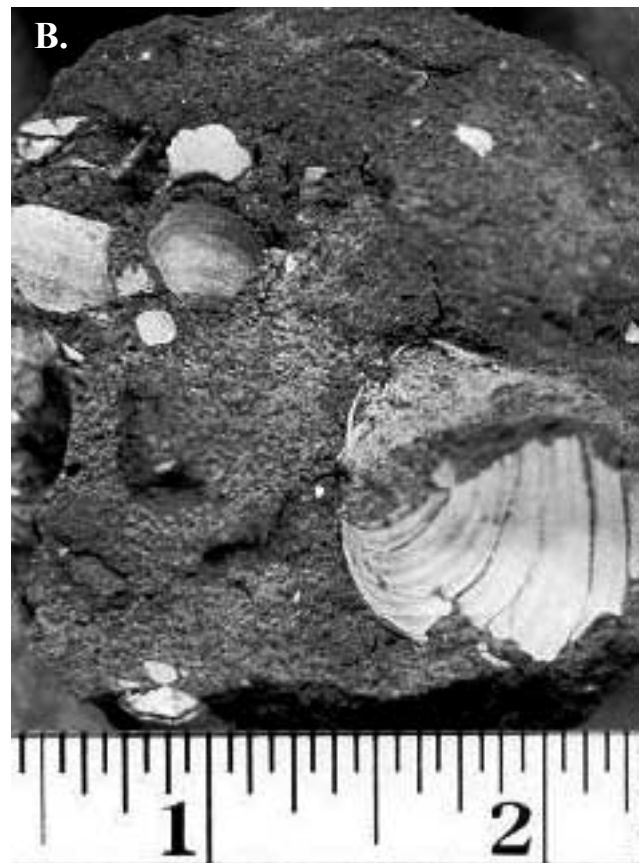
b. Cross-sectional view of core segment showing mollusk valves in the massive-sand lithofacies. Sample from a depth of 31.3 ft.
