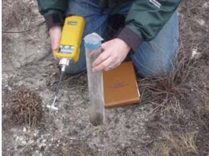
Figure 9- Individual is pulling the 61 cm tube from the auger hole. The PID is in his right hand. The small, white disk below the black tube on the PID is the water trap, a device designed to prevent water from entering the ionization chamber in the instrument. The probe tip is below the trap. The probe tip is inserted in the hole in the duct tape and the soil gas sample is drawn from the auger hole by the pump in the PID.
