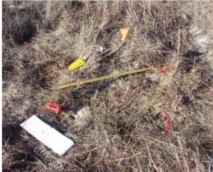
Figure 10- Site AH8. Initial hole is marked by the orange flag (the flag is visible but not the metal wire inserted into the ground; the hole is beneath the meter stick). Adjacent locations, AH8B, AH8C, and AH8D, are marked by 10-penny nails tied with red flagging. The opening for one of these holes is visible, just to the right of the red flagging on the left side of the photo. The PID (yellow) and an open field notebook are visible.
