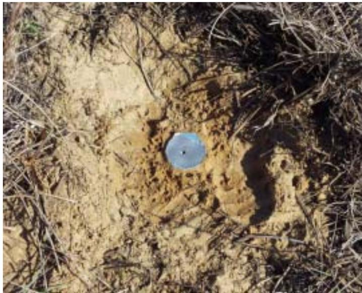
Figure 8- Site AH 16. Top of inserted tube with blue rigid plastic cap and duct tape. Note hand impressions from pushing soil down around the top of the tube to seal the soil. Also note the weak iron oxyhydroxide staining in soil surface layer.
