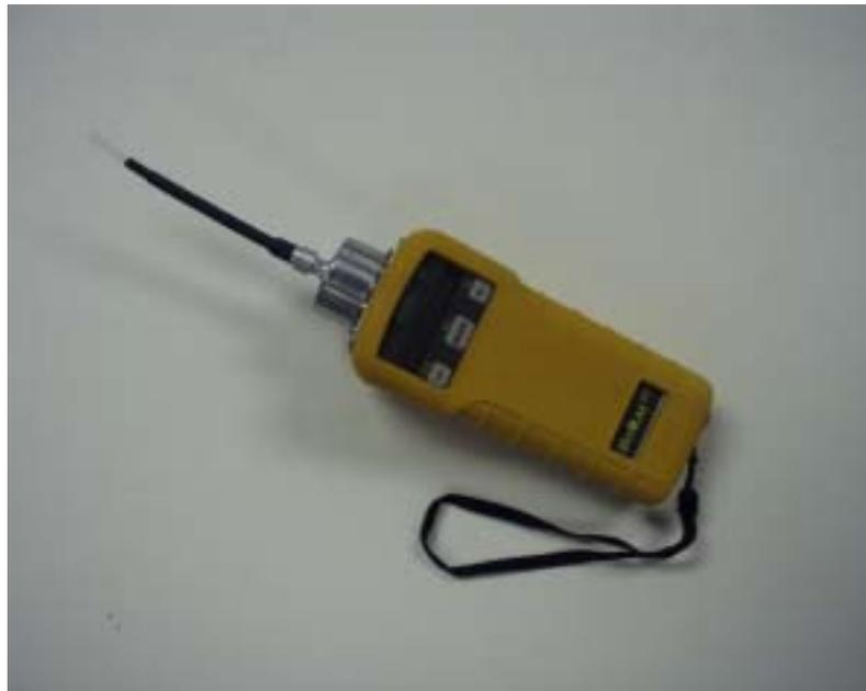
Figure 1- Photoionization detector (RAE Systems, appendix 1) used to determine the concentration of volatile organic compounds in air (either in soil gas in an auger hole or being given off by a soil sample to the headspace of a plastic sample bag).
