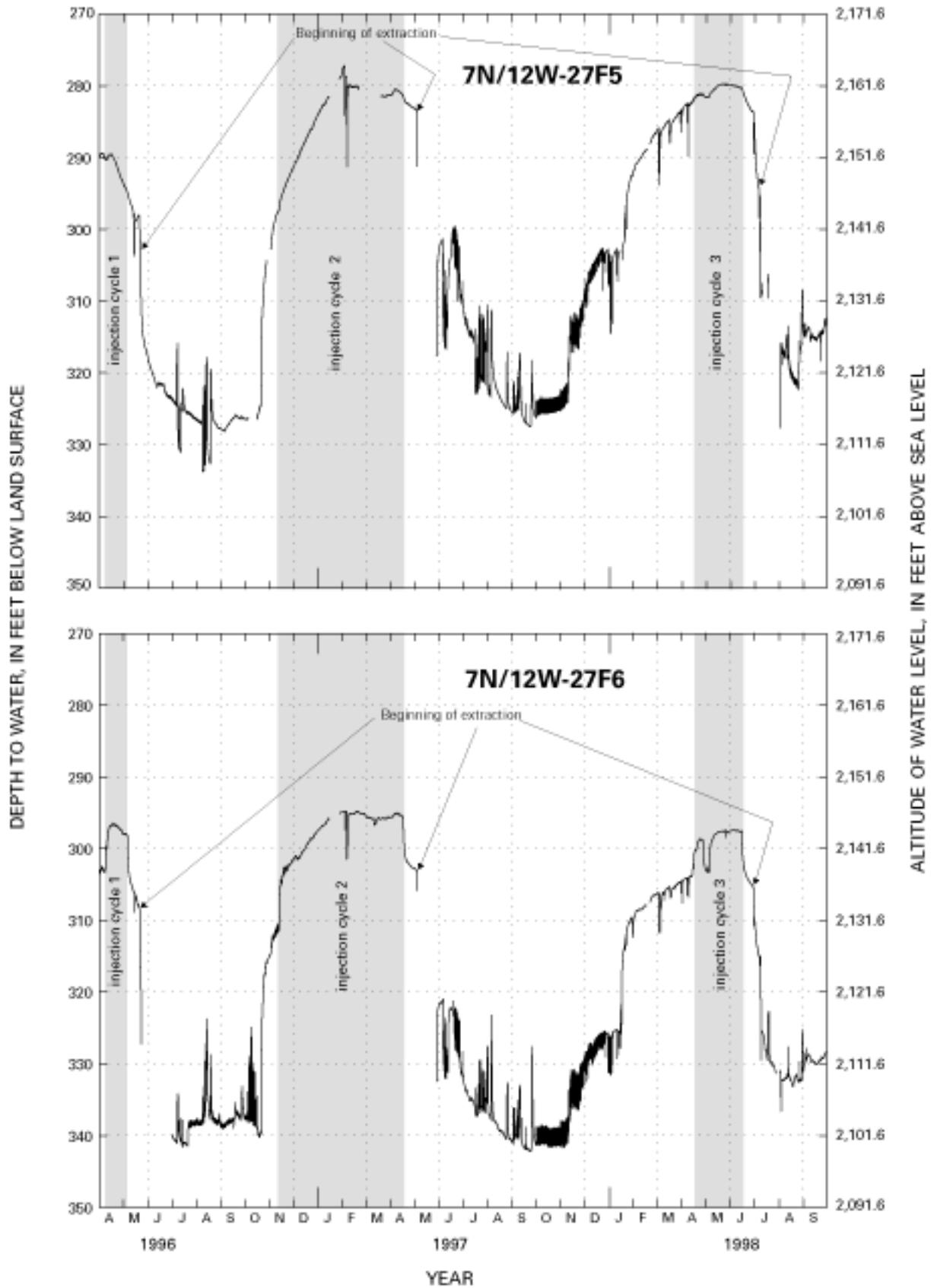
**Figure 15.** Ground-water levels recorded in piezometers 7N/12W-27F5–8 at the extensometer site in Lancaster, Antelope Valley, California, April 1996 through September 1998.
