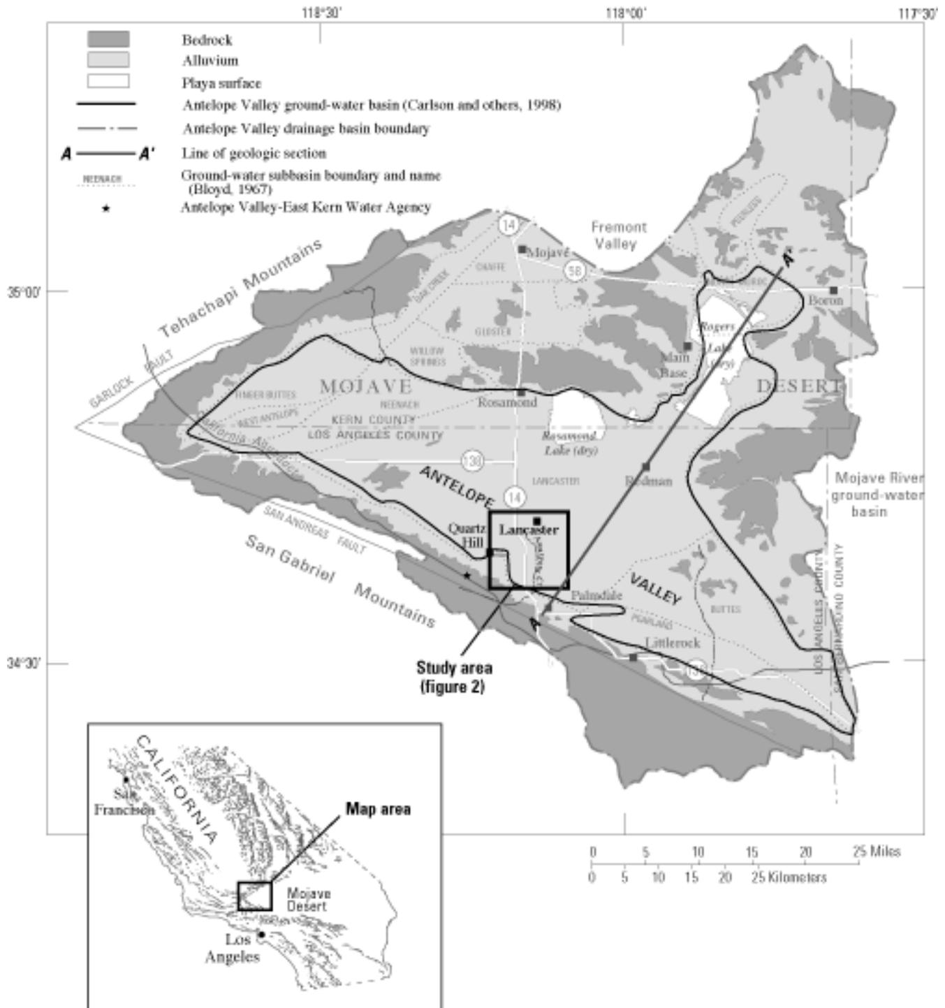
**Figure 1.** Generalized surficial geology and location of study area and of ground-water basin and subbasins in the Antelope Valley, California. (Modified from Carlson and others, 1998)
