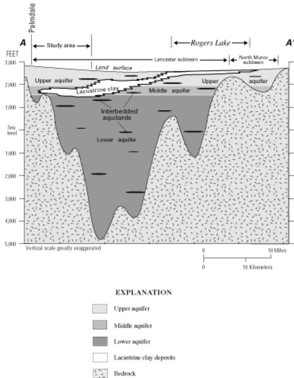
**Figure 2.** Generalized geologic section showing relation of lacustrine clay deposits to younger and older alluvium and aquifers in the Lancaster and North Muroc subbasins in the Antelope Valley ground-water basin, California (modified from Londquist and others, 1993). Line of section is shown on figure 1.
