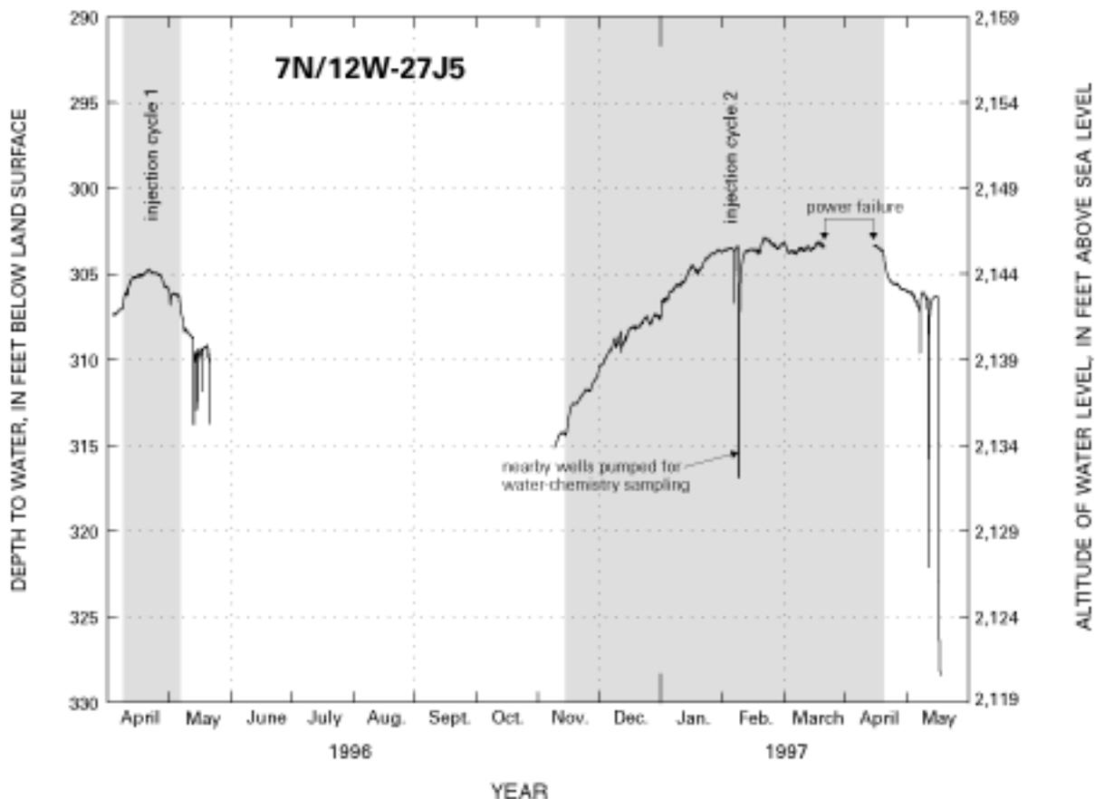
**Figure 17.** Ground-water levels recorded in abandoned production well 7N/12W-27J5 at the Avenue K-8 and Division Street well field in Lancaster, Antelope Valley, California, April 1996 through May 1997.
