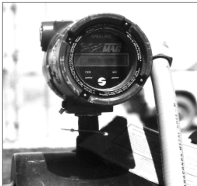
Figure 38. Flowmeter used to measure injection and extraction flow rates at injection well 7N/12W-27P3 in Lancaster, Antelope Valley, California.
