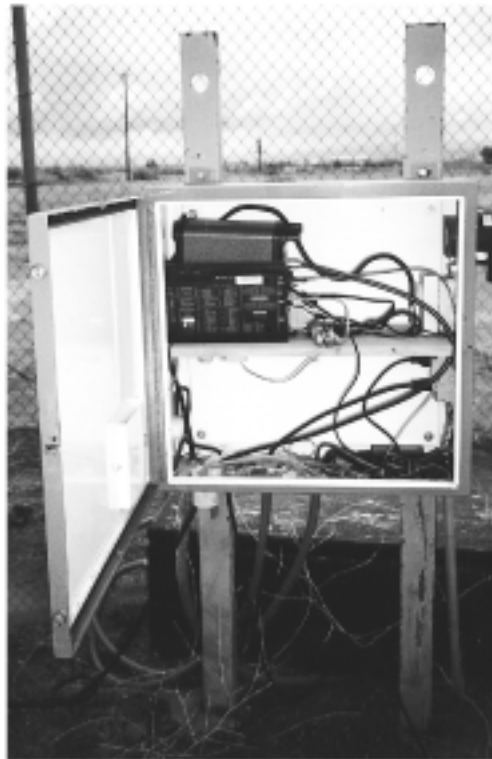
Figure 30. Permanent Global Positioning System (GPS) station at the injection site in Lancaster, Antelope Valley, California. A. Antenna (photographed in September 1998). B. Receiver with modem.
