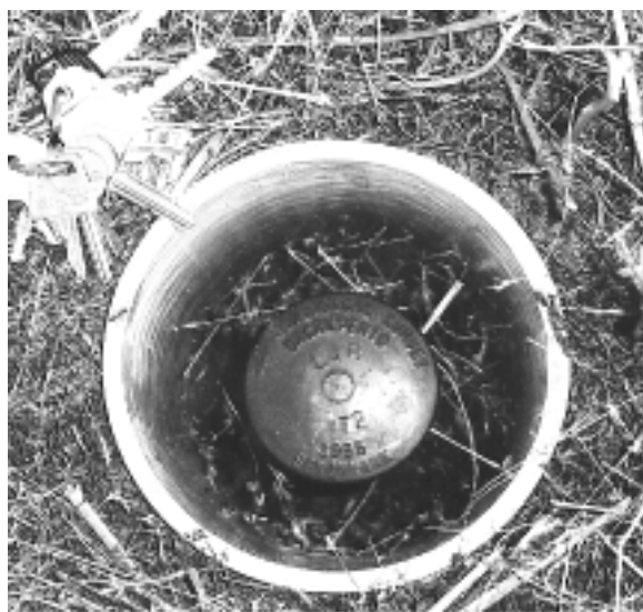
Figure 24. Typical vertical-control bench mark used for differential-leveling surveys.
