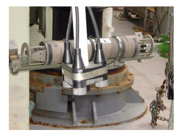
Figure 8A. The sensor of the 3 frequency (1, 2.5 and 5 mHz) Acoustic Backscatter System (ABS).
