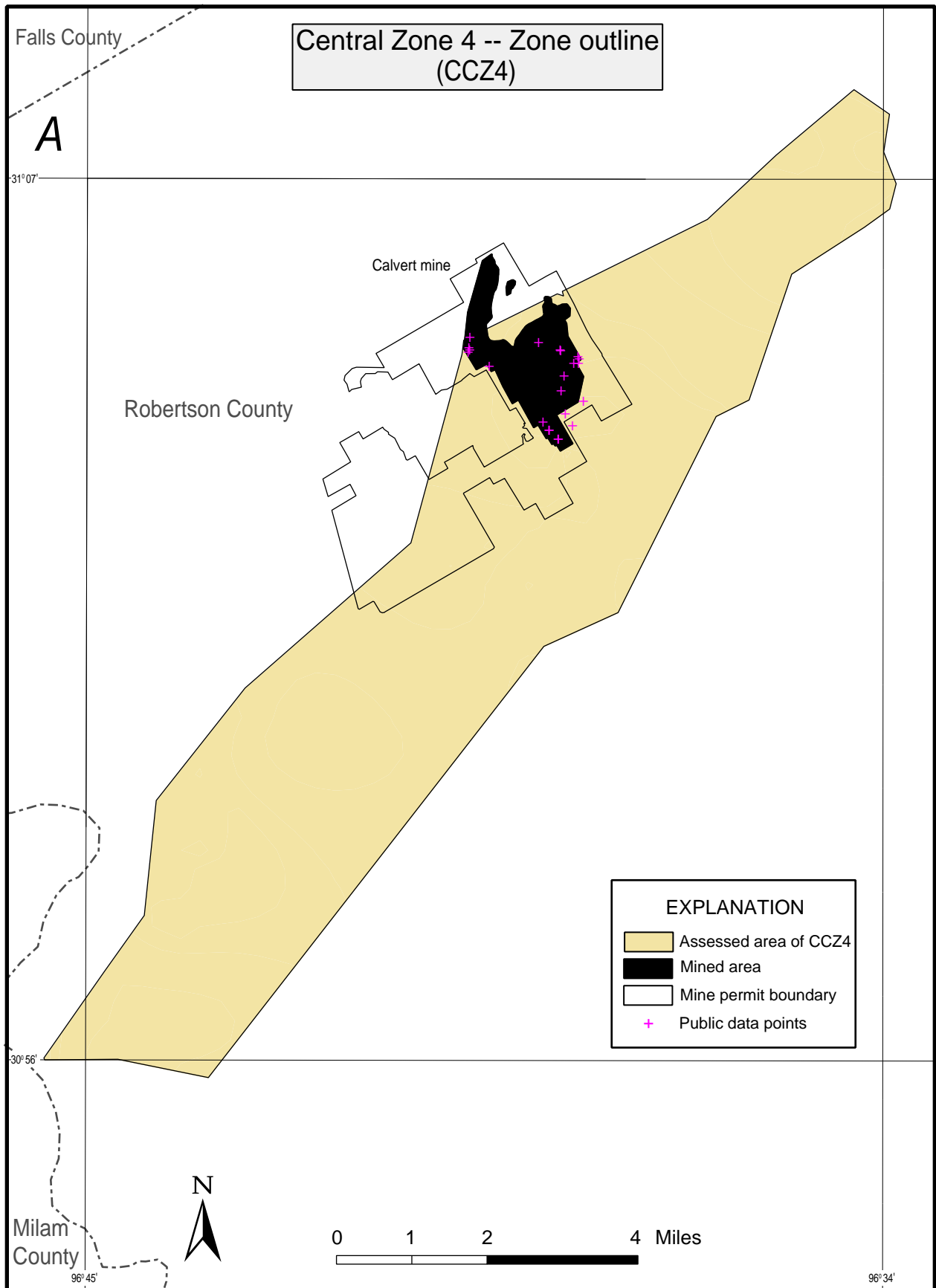
Fig. 13. Geology of central Coal Zone 4 (CCZ4). a) Outline of Zone 4 showing coal mine permit locations mined areas, and county boundaries. b) Structure contour map of the stratigraphic top of Zone 4. c) Map of overburden thickness for Zone 4. d) Map of the cumulative coal bed thicknesses that compose Zone 4.
