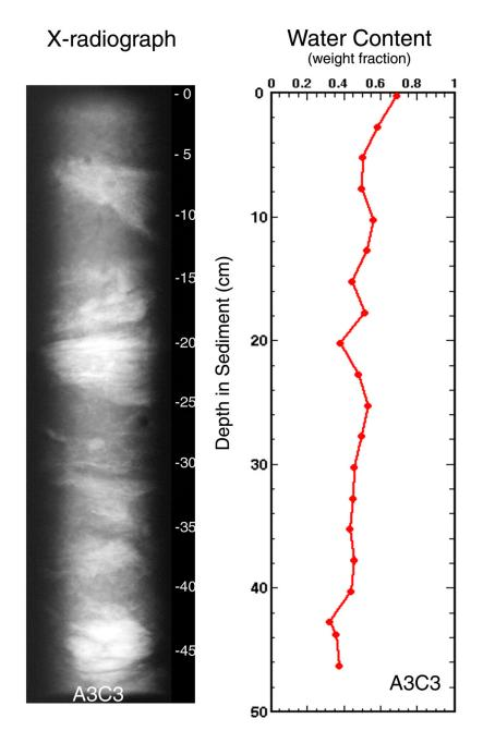
Core A3C3 was taken on June 18, 1996 in 18 meters of water. The core measured 48 cm in length, was x-rayed on June 26, 1996 and was subsampled on October 15, 1996 at 0.5 cm intervals down the whole core. Features noted are seen in the x-ray and water content profiles above and include slightly mottled sediment, angled wispy sand layering, and some biological features such as small shells. No textural analysis is intended for this core.
