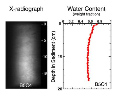
Core B5C4 was taken on June 19, 1996 in 26 meters of water. The core measured 17-17.5 cm in length, was x-rayed on June 26, 1996 and was subsampled on April 2, 1997 at 0.5 cm intervals down the whole core. Features noted are seen in the x-ray and water content profiles above and include mottled sediment, wispy deposits, gas cracks, and some biological features such as small shells. No textural analysis is intended for this core.
