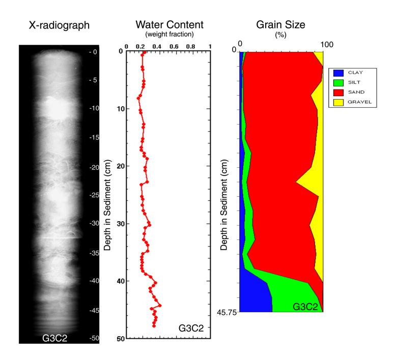
Core G3C2 was taken on June 21, 1996 in 46 meters of water. The core measured 49.5 cm in length, was x-rayed on June 26, 1996 and was subsampled on October 31, 1996 at 0.5 cm intervals down the whole core. Features noted are seen in the x-ray, water content, and texture profiles above and include sand and mud ribbons, mottled sediment, and biological features such as shell layers.
