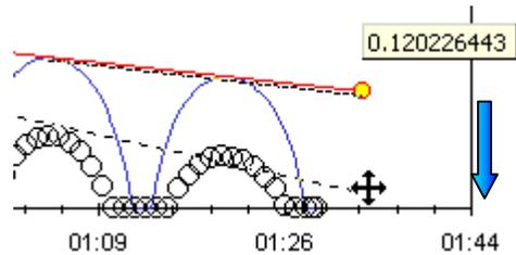
Frequency ( $\omega$ ) is estimated by fitting the red crosses in the displacement chart to the measured peaks. The vertical position of the 2 crosses does not affect estimates of  $T$ , but can be adjusted for convenience by moving the right cross without a yellow ball.
