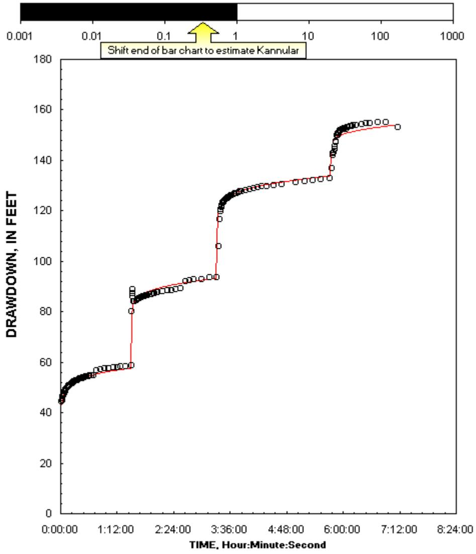
Figure 5. Graph used for estimating hydraulic conductivity of annular space and skin.
