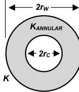
The relation between **skin** and the reduction of hydraulic conductivity around the wellbore is best illustrated by example. For an annular ring of damaged material where  $r_w = 2r_c$ , **skin** values of 1, 2, and 4 yield  $K/K_{ANNULAR}$  values of 0.41, 0.26, and 0.15.
