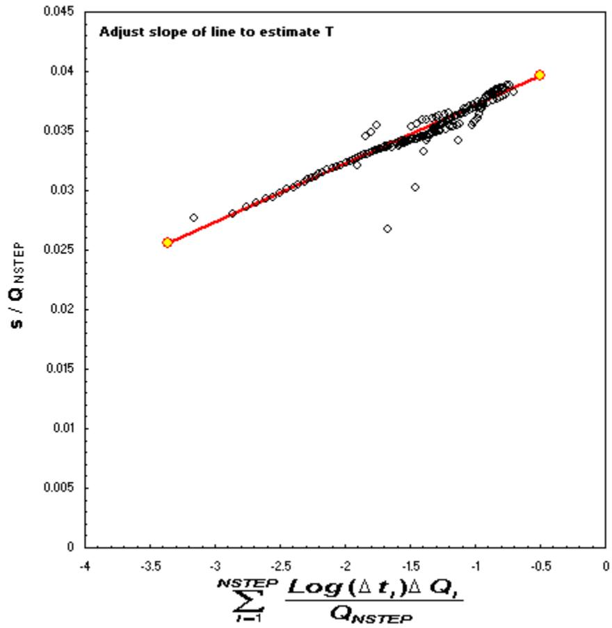
Figure 4. Plot used to estimate transmissivity from the step-drawdown spreadsheet.
