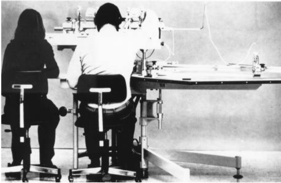
5.2 -- Figure 4. - - The Kern PG-2 Photogrammetric Plotter.
