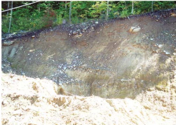
Fig. 50- B) Excavation along Rt.19 east of Soco Gap exposes diamicton about 10 m thick. Large boulder right of center is 2 m diameter. Upper center is a cross section of a channel with concentrated boulders of metasandstone (elev = 3640 ft, Bunches Bald quadrangle).
