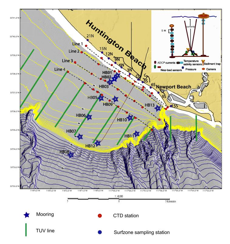
**Figure 1a.** Map of the region, the mooring sites and surfzone sampling stations. Sediment transport instruments are deployed at HB03, HB05, HB07, and HB11. The meteorological buoy is at HB07. Inset shows instrumentations of a typical mooring.
