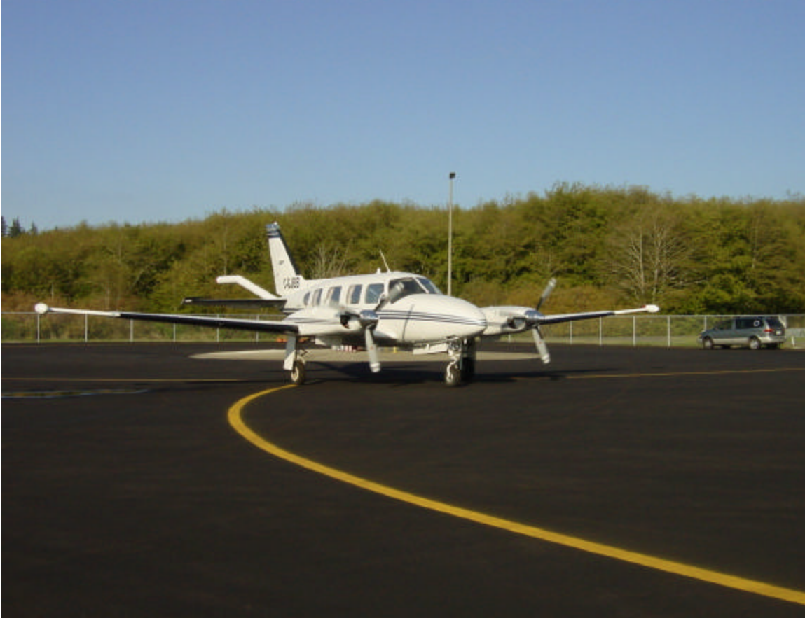
Illustration - PA-31 Navajo C-GJBB in Horizontal Gradient Survey Configuration
