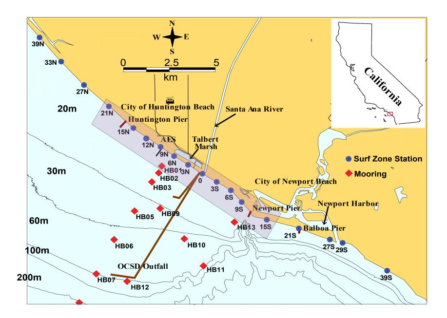
**Figure 11-1.** Map of the coastal zone surrounding Huntington Beach, California. The blue dots show the location of the surfzone sampling stations from 39N to 39S. The outfall is shown leaving the coast near station 0. The diffuser of the outfall is located near stations HB07 and HB12. Station 12S is located at Newport Pier.
