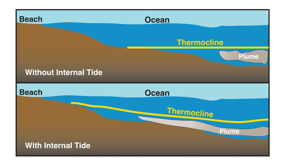
Figure 7-1. Schematic of cross-shore transport of the plume from the outfall by internal tidal currents.
