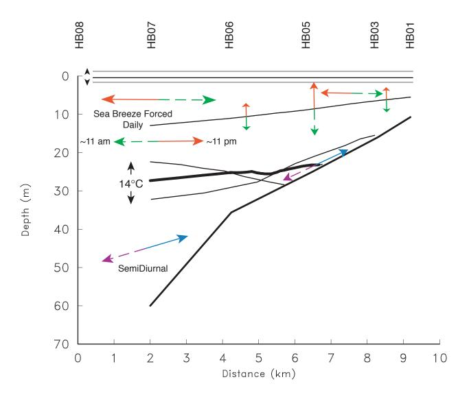
**Figure 7-11.** Conceptual model of the cross-shelf current and temperature fluctuations caused by the sea breeze and semidiurnal tide. Solid and dashed arrows represent maximum velocities a half-cycle apart. Red and green, and blue and purple arrows, are 24- and 12.42-hour oscillations, respectively.
