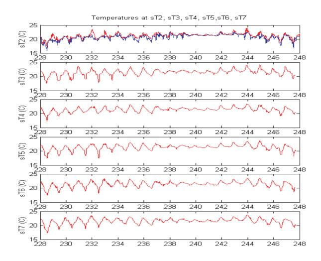
**Figure 9-13.** Surfzone temperature (lower 5 panels) at 5 locations alongshore, and surface and bottom temperature at sT2 (2.5-m isobath; top panel), deployed offshore of surfzone site sT6 (second bottom panel).
