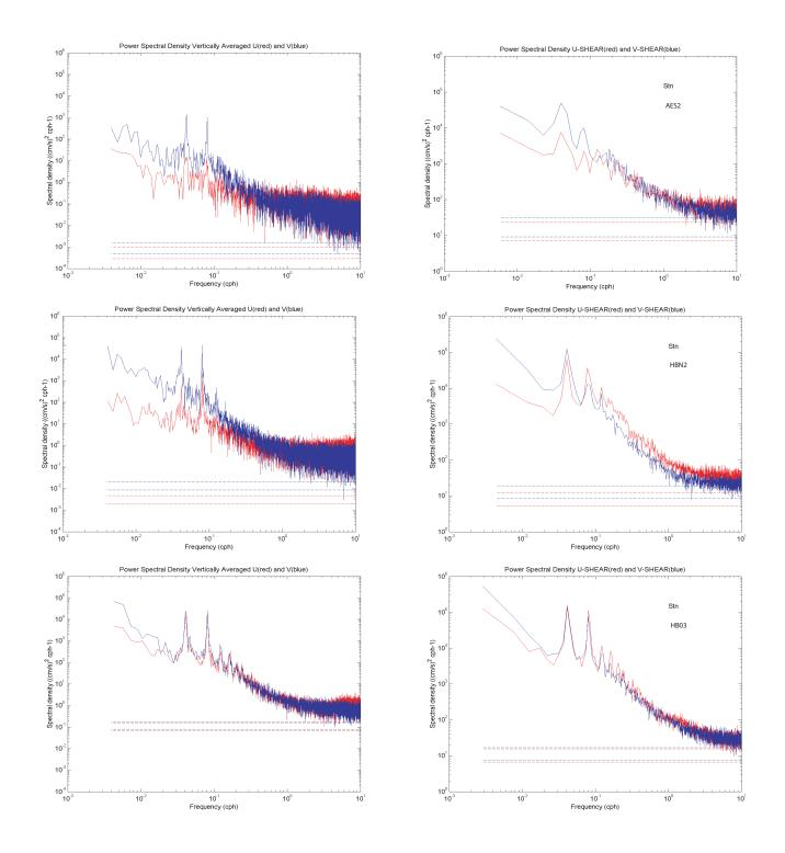
**Figure 9-3a.** Spectra of depth-averaged near-bottom velocities (left panels) and sheared flow (top-bottom difference, right panels) for moorings AES2 (top row), HBN2 (middle row), and HB03 (bottom row). Alongshore currents are blue, cross-shore currents are red. The 95% confidence interval is shown.
